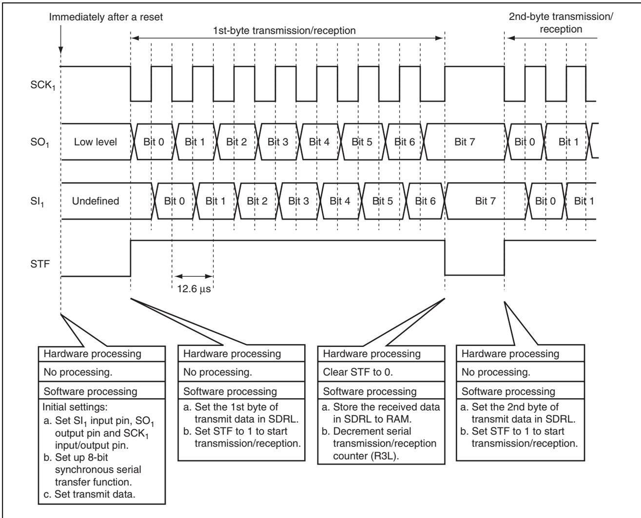
Figure 3.1 Operation Principles of Simultaneous Transmission/Reception in Synchronous Mode
