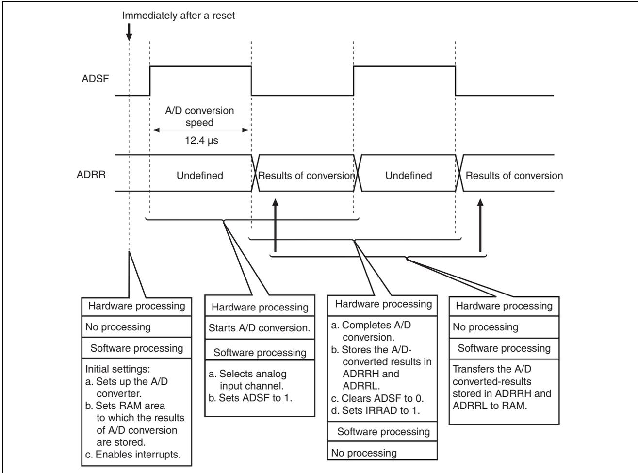
Figure 3.1 Operation Principle of Voltage Measurement by 4-Channel A/D Conversion
