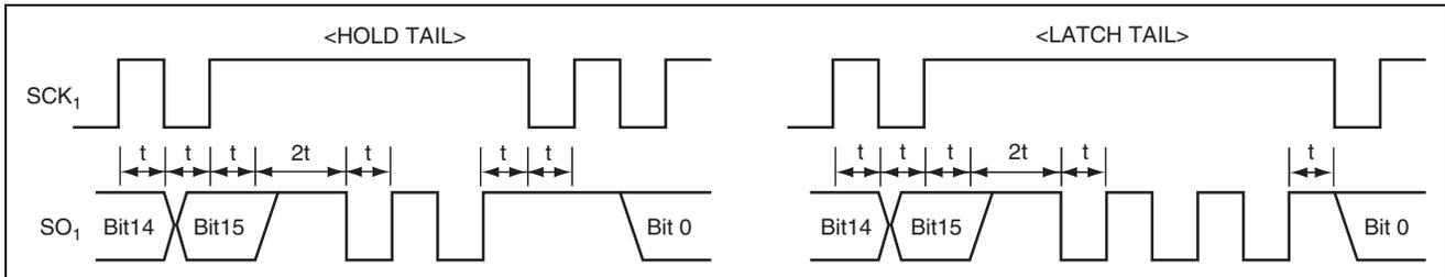
**Figure 2.3 Hold and Latch Tail Output Waveforms**
