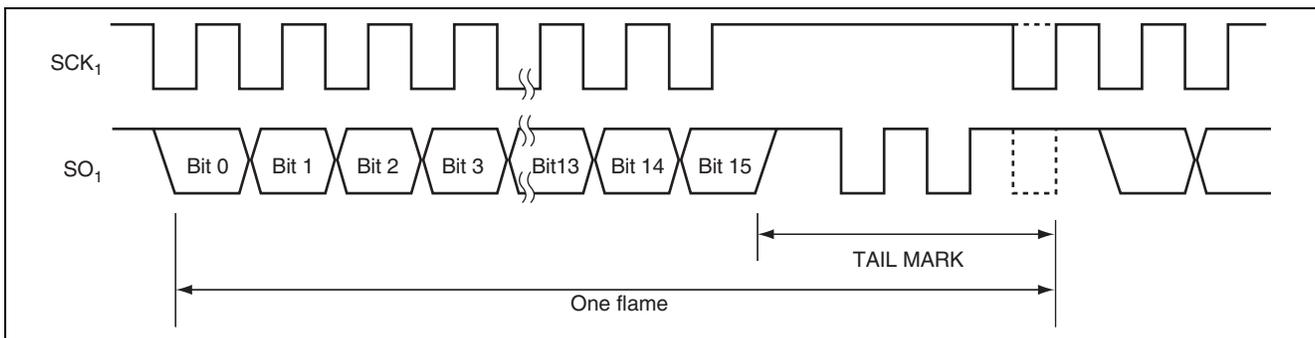
Figure 2.2 Transfer Format (When  $SNC1 = 0, SNC0 = 1$  and  $MRKON = 1$ )
