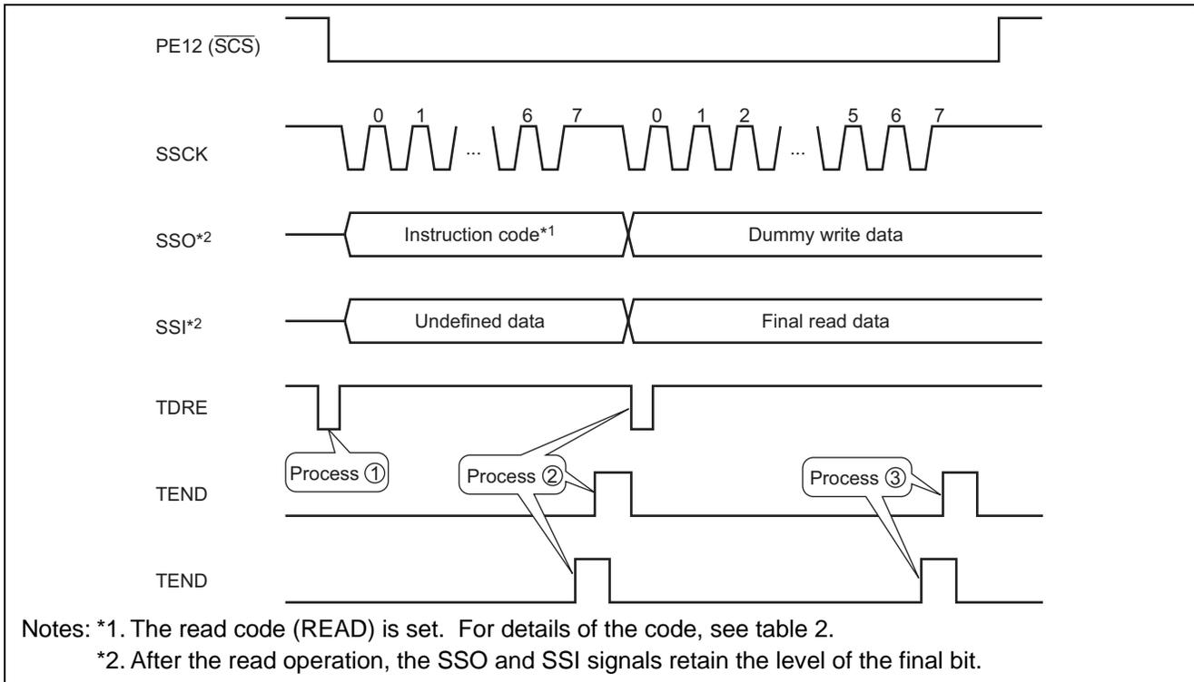
Figure 4 Operations for Reading Data
