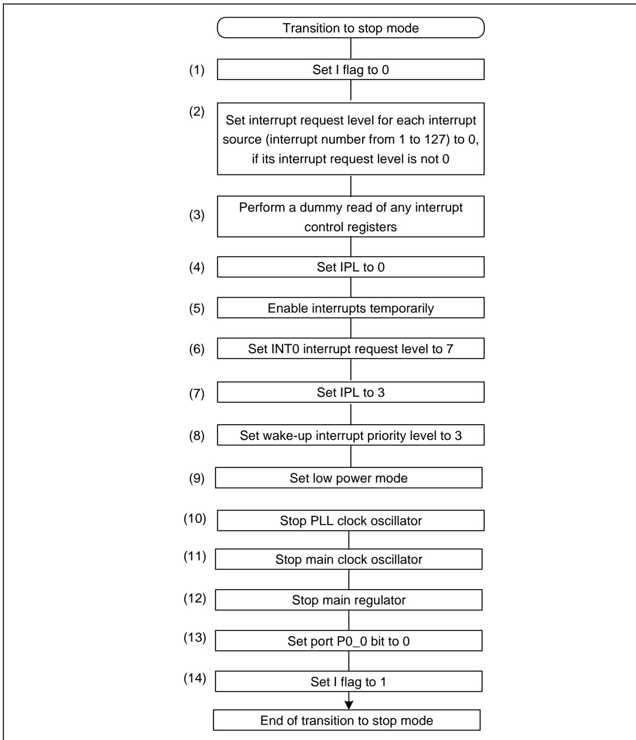
Figure 5.5 Stop Mode Transition Flowchart
