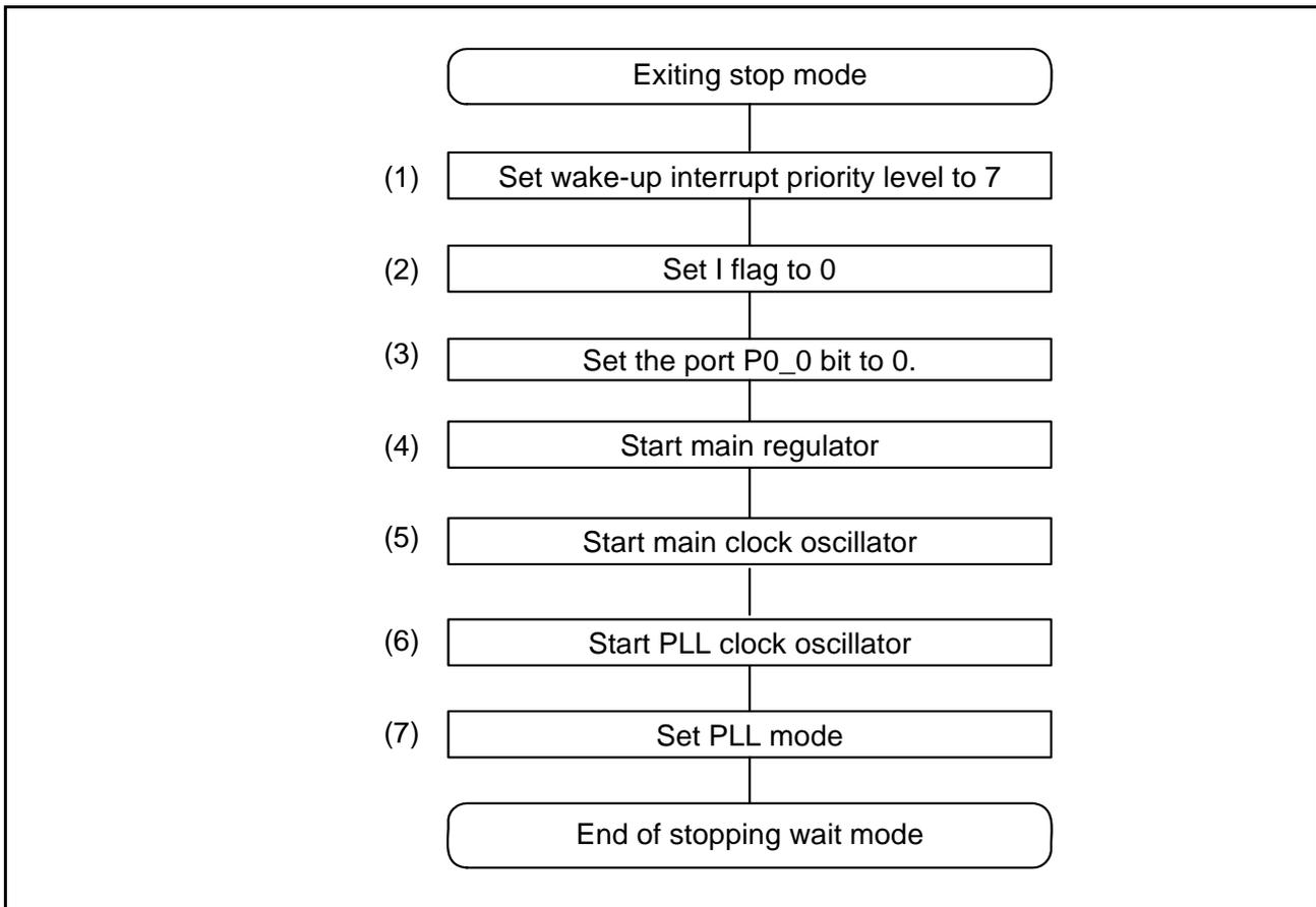
Figure 5.6 Exit Stop Mode Flowchart
