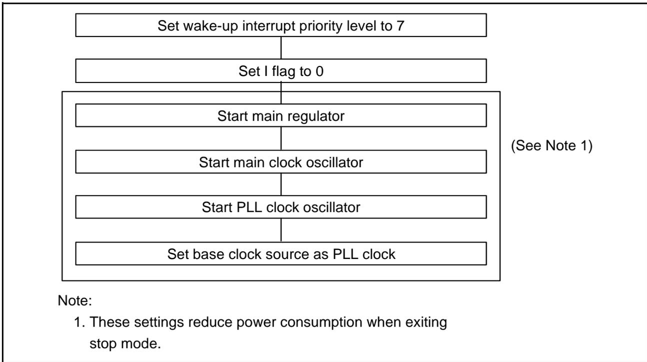
**Figure 4.5 Procedure for Exiting Stop Mode**
