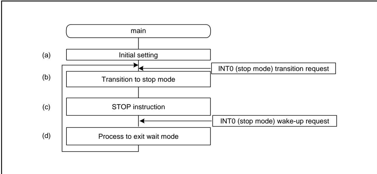
Figure 5.4 Main Function Flowchart
