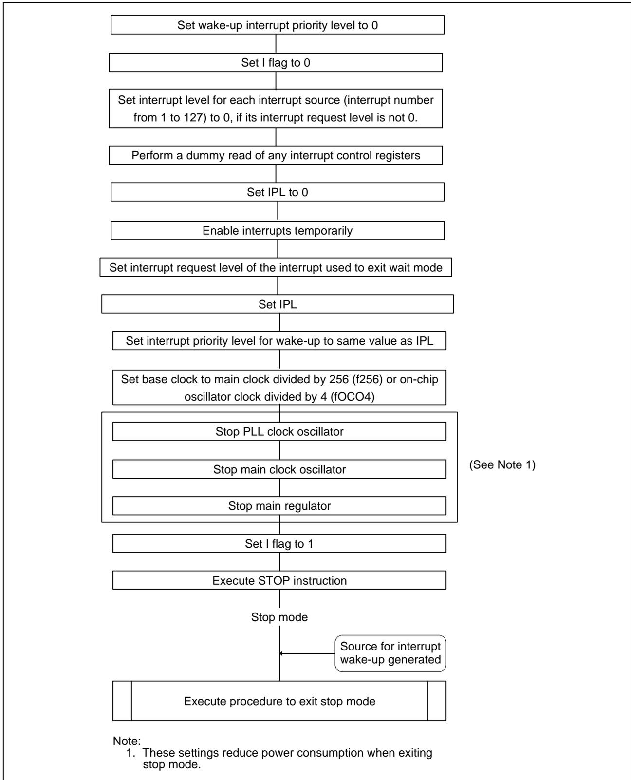
Figure 4.4 Procedure for Entering Stop Mode
