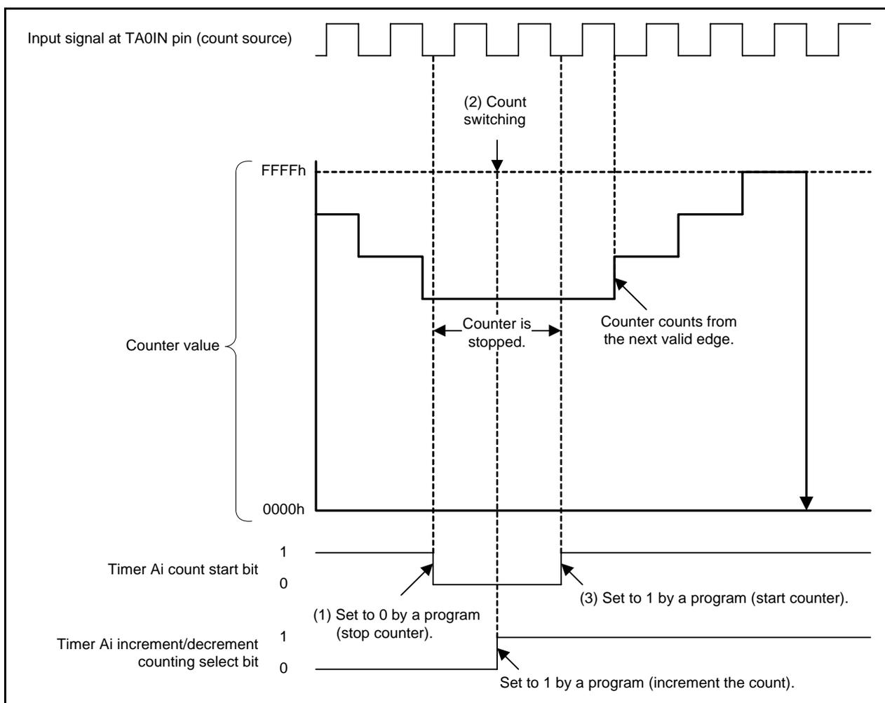
Figure 6.1 Operation Example of Switching Between Incrementing and Decrementing
