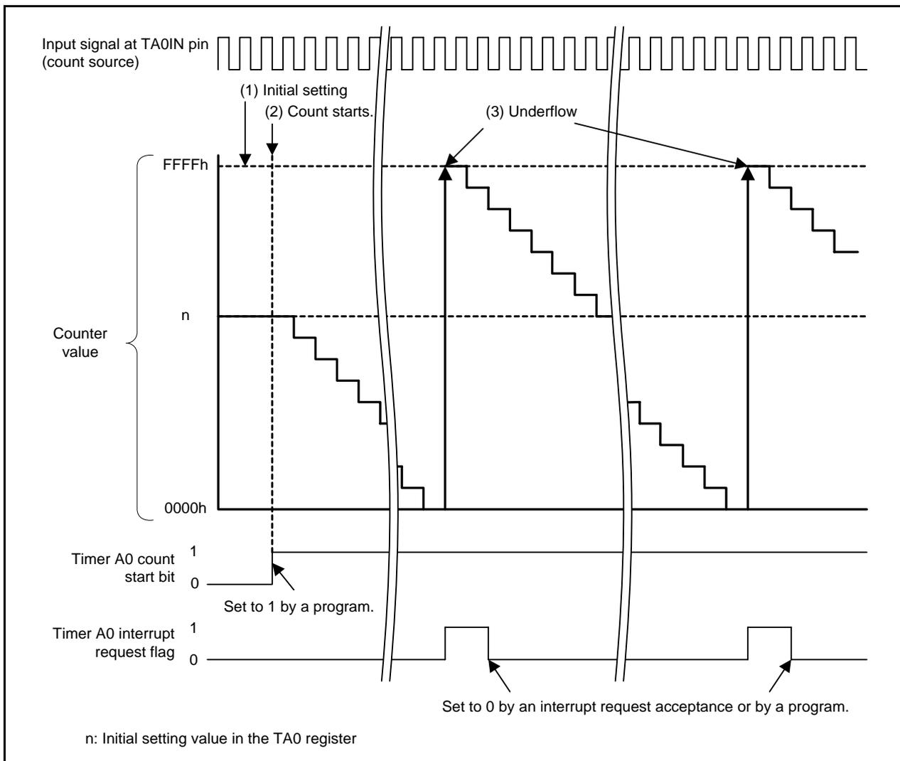
Figure 5.1 Timer A0 Operation in Event Counter Mode Using Free-running Count Operation
