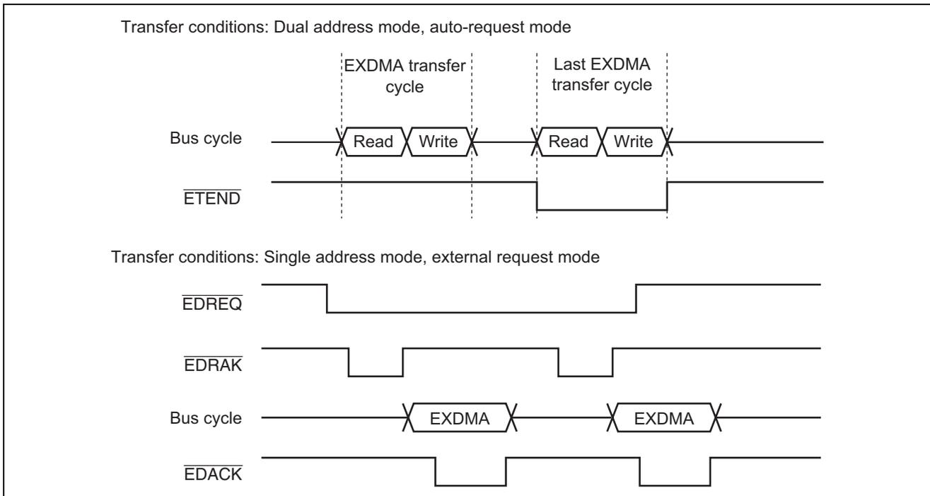
Figure 4 Example of Timing in Normal Transfer Mode
