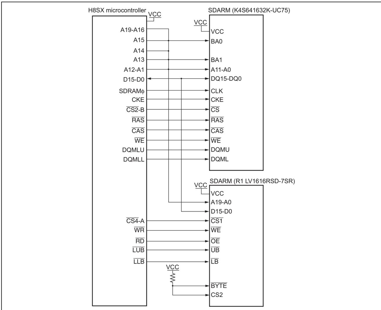
**Figure 2 Connections between External Memory and CPU**
