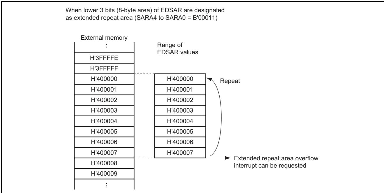
Figure 6 Example of Extended Repeat Area Function Operation
