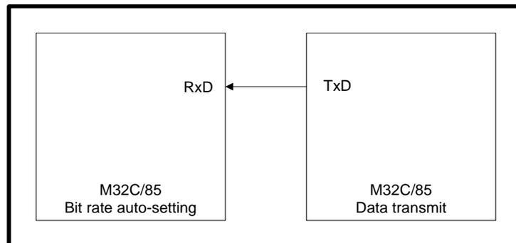
Figure 1. Circuit Connection for UART auto bit-rate setting
