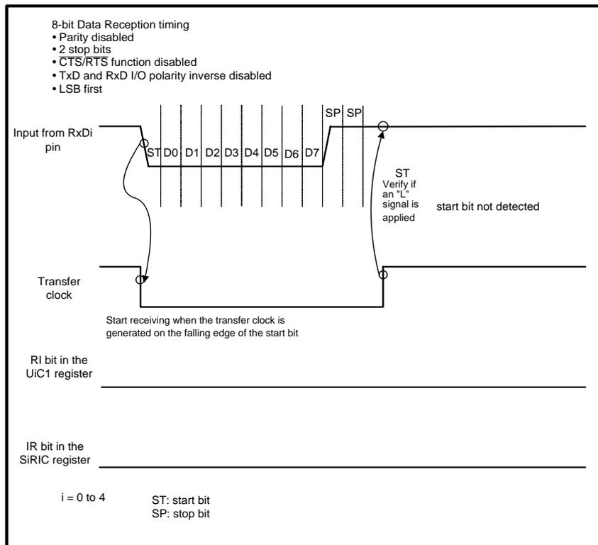
Figure 8. Negotiation Data Start Bit Undetected Timing
