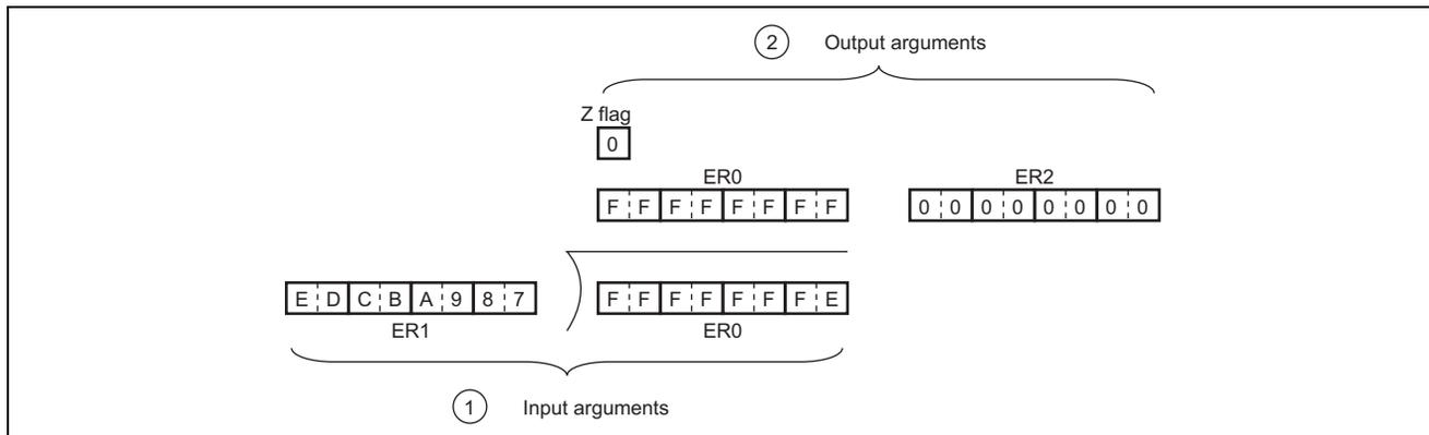
Figure 1 Example of Software DIVIDE64
