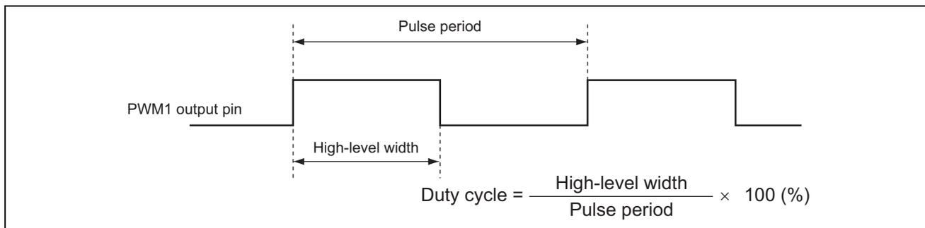
**Figure 1 Variable Duty-Cycle Pulse Output by 10-Bit PWM Function**
