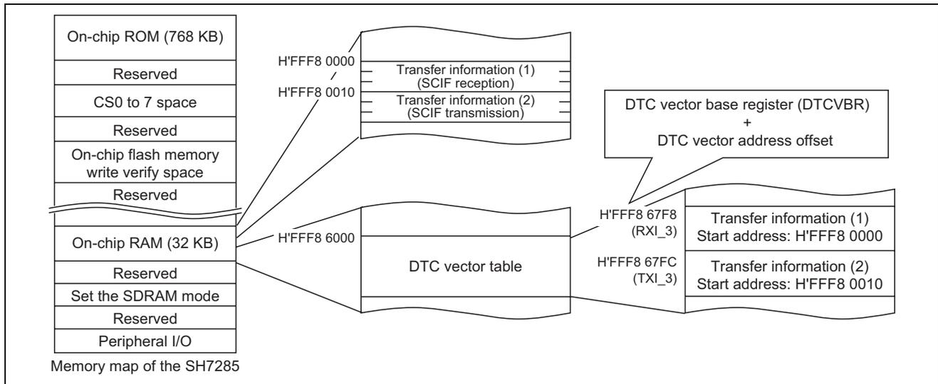
**Figure 6 Image of Arrangement of Transfer Information in Memory**
