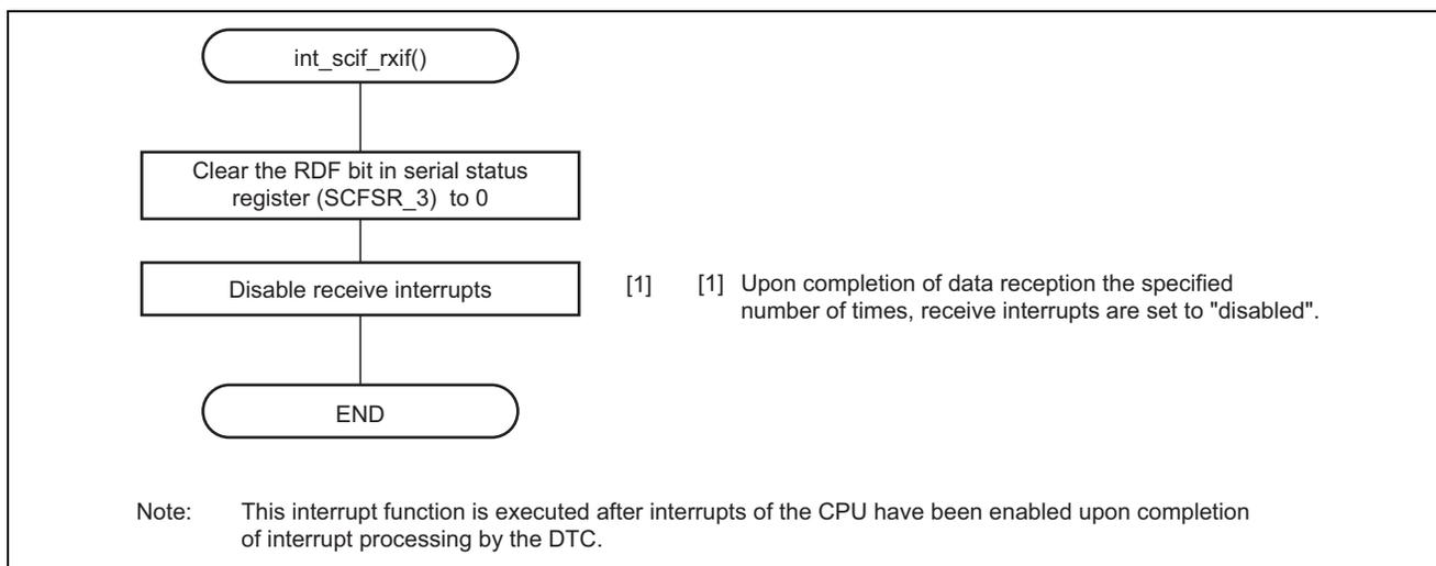
**Figure 15 Flow for Handling Receive Interrupts in Asynchronous Mode**
