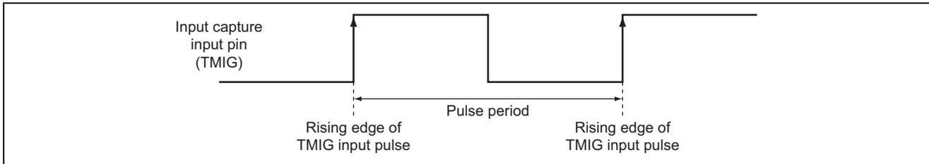
Figure 1 Measurement of Input Pulse Period
