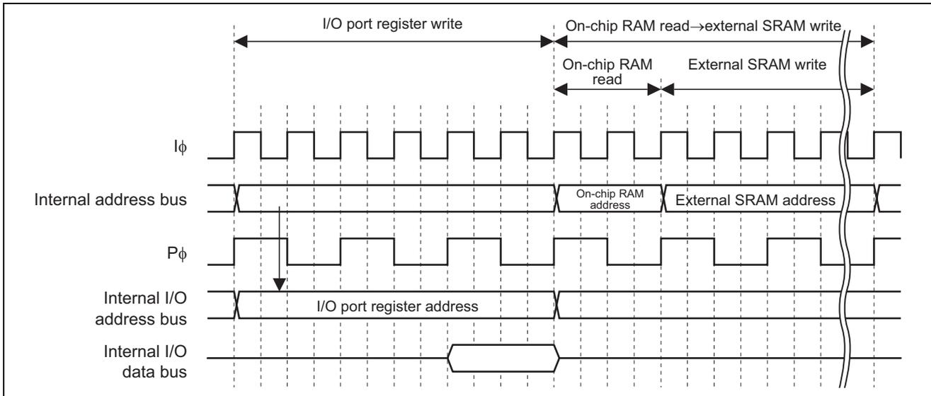
**Figure 2 Example of Timing of Operations with the Write Data Buffer Function for Peripheral Modules not in Use (PWDBE = 0)**
