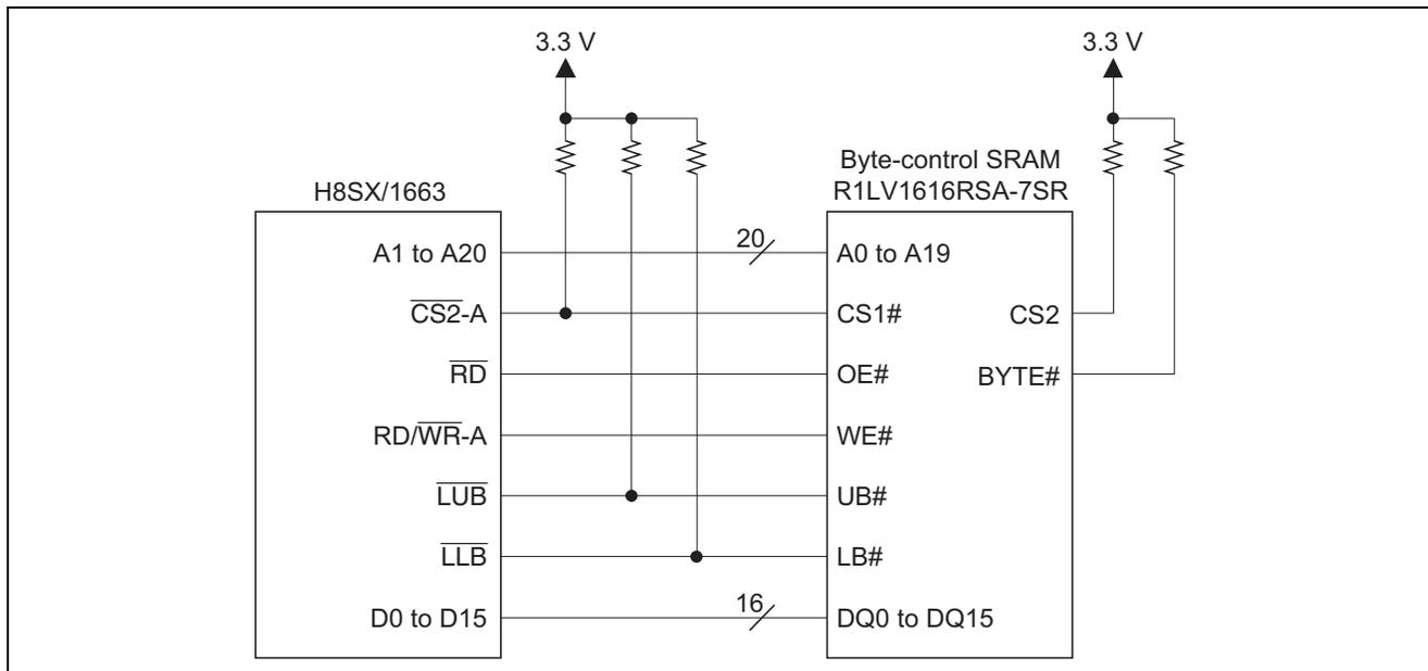
**Figure 1 Example of Connection of an SRAM with Byte Control**
