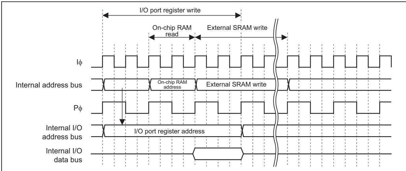
**Figure 3 Example of Timing of Operations with the Write Data Buffer Function for Peripheral Modules in Use (PWDBE = 1)**
