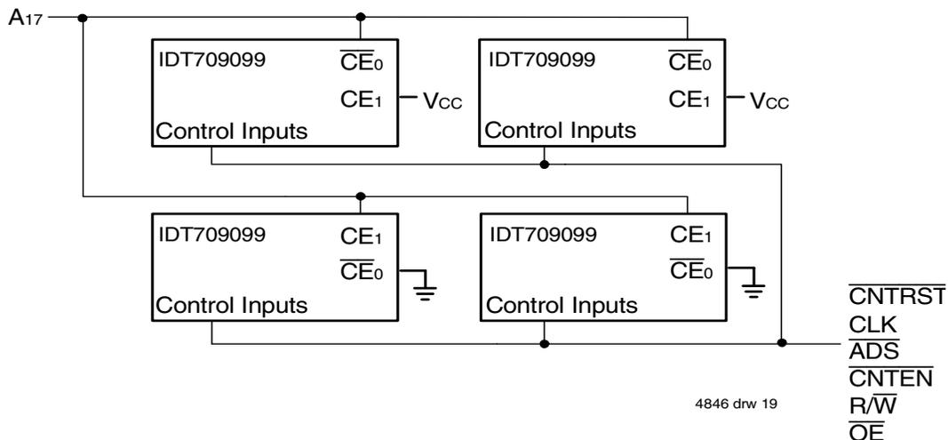
Figure 4. Depth and Width Expansion with IDT709099
