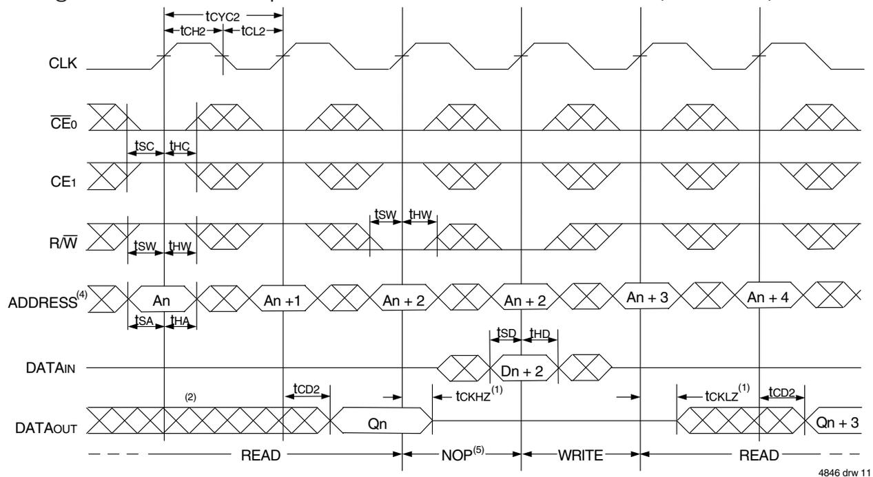
Timing Waveform of Pipelined Read-to-Write-to-Read ( $\overline{OE}$  Controlled)<sup>(3)</sup>
