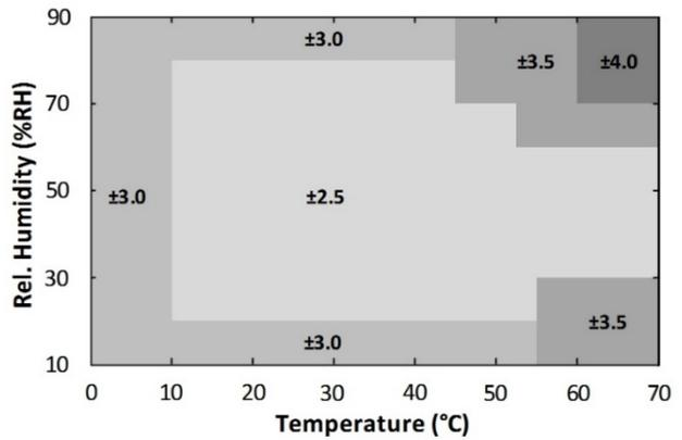
Figure 5. HS41x3 RH Accuracy over Temperature
