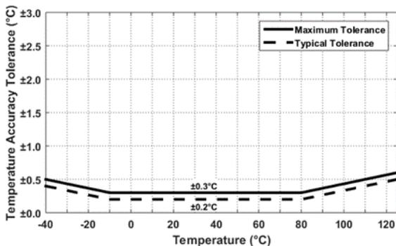
Figure 6. HS41x1 Temperature Sensor Accuracy Tolerance
