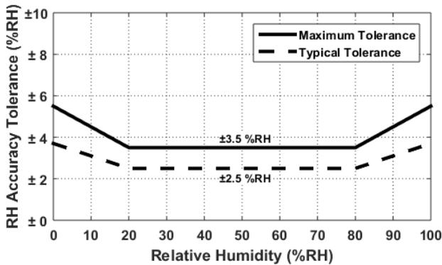
Figure 4. HS41x3 RH Accuracy Tolerance at 25°C
