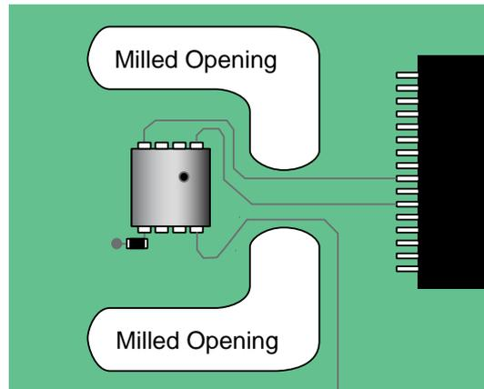
Figure 12. Milled PCB Openings for Thermal Isolation
