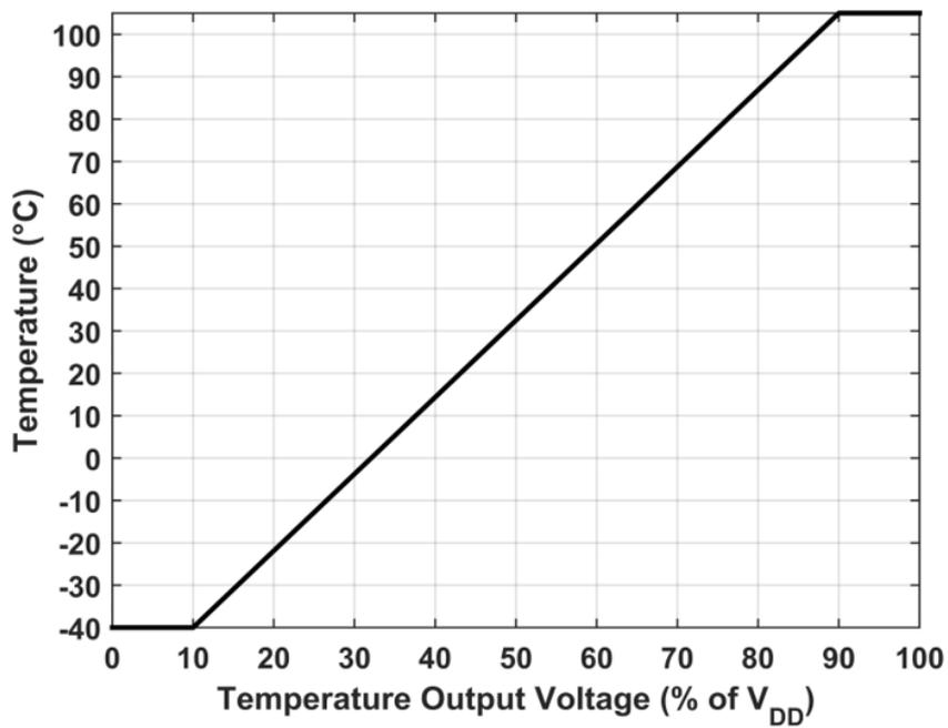
Figure 10. Temperature vs. VT Output Analog Voltage
