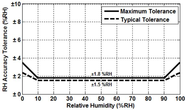
Figure 2. HS41x1 RH Accuracy Tolerance at 25°C
