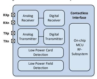
Figure 6: Contactless Interface
