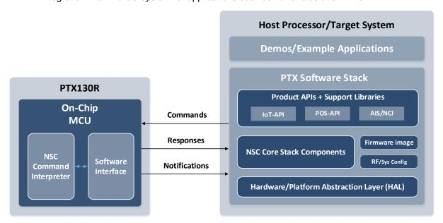
Figure 9: PTX130R SW Stack Integration View
