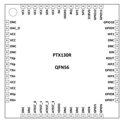
Figure 2: Pin Diagram
