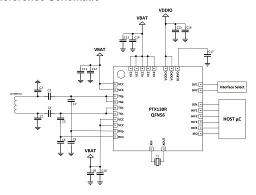
Figure 10: Exemplary Reference Schematic
