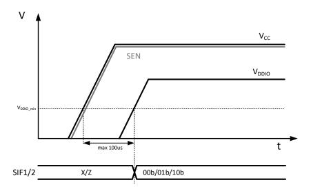
Figure 5: Supply Ramp Up (SEN==VCC)
