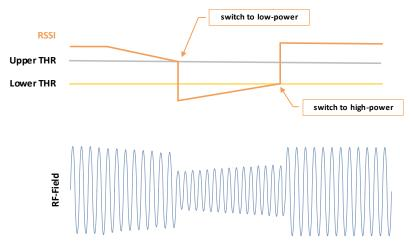
Figure 7: Dynamic Digital Power Control (DDPC)
