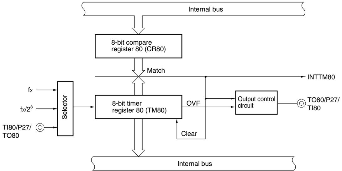
Figure 5-4. Watch Timer Block Diagram
