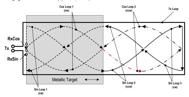
Figure 3. Coil Design for a Linear Motion Sensor
