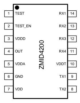
Figure 1. Pin Assignments for 14-TSSOP Package – Top View
