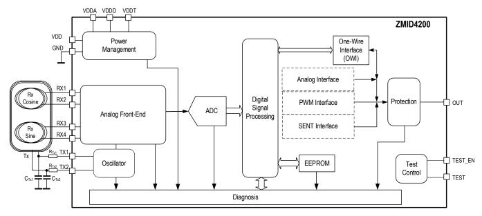
Figure 4. Block Diagram
