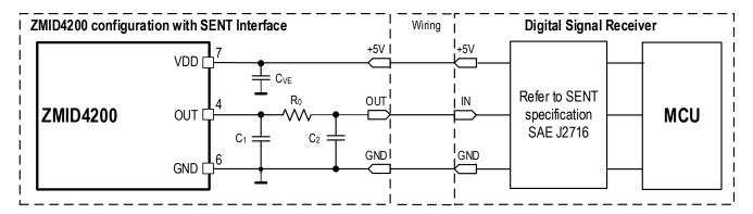
Figure 12. External Components for ZMID4200 SENT Interface
