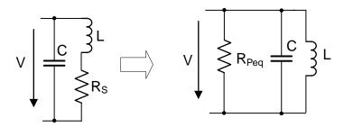
Figure 2. Parallel Resonator Circuit
