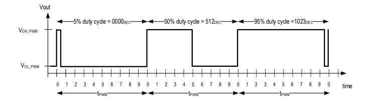
Figure 10. Example of PWM Output Signal
