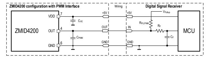
Figure 8. External Components for ZMID4200 PWM Interface with Pull-Up Resistor
