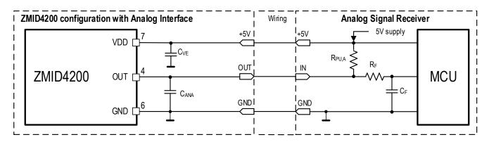
Figure 6. External Components for ZMID4200 Analog Interface with Pull-up Resistor
