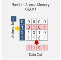
RAM: Input the address and output the data
