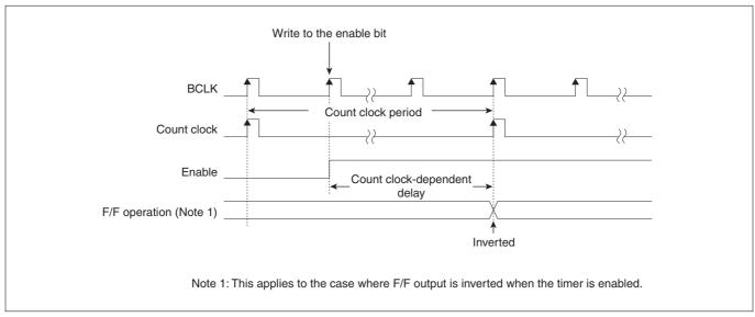
Figure 10.4.2 Count Clock Dependent Delay
