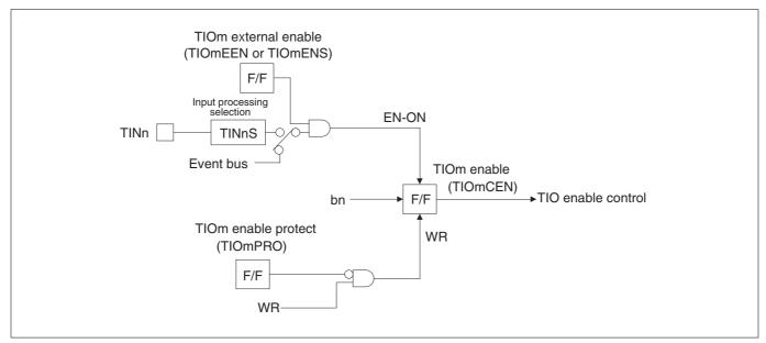
Figure 10.4.5 Configuration of the TIO Enable Circuit
