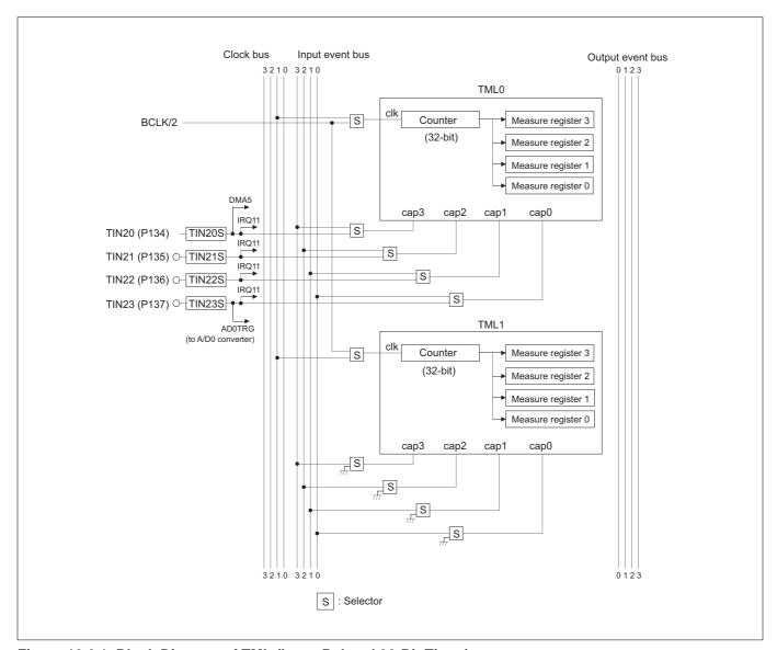
Figure 10.6.1 Block Diagram of TML (Input-Related 32-Bit Timer)
