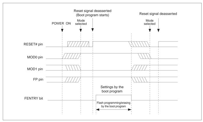
Figure 6.5.3 Internal Flash Memory Write/Erase Timing (when the flash write/erase program does not exist in it)
