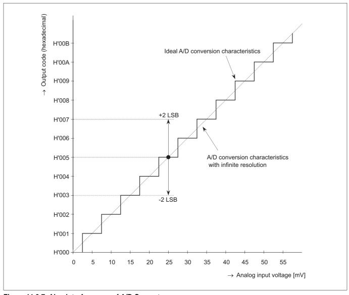
Figure 11.3.7 Absolute Accuracy of A/D Converter
