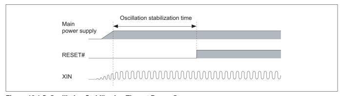
Figure 18.1.5 Oscillation Stabilization Time at Power-On
