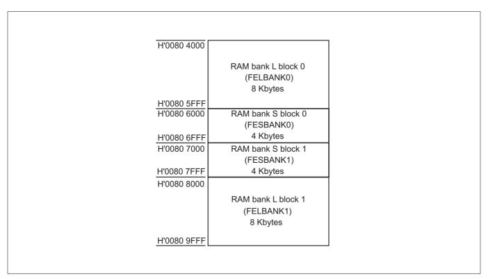
Figure 6.6.1 Internal RAM Bank Configuration of the M32176
