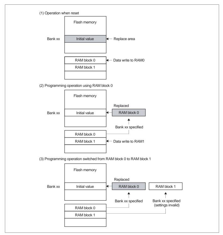
Figure 6.6.15 Application Example of Virtual Flash Emulation Mode (1/2)
