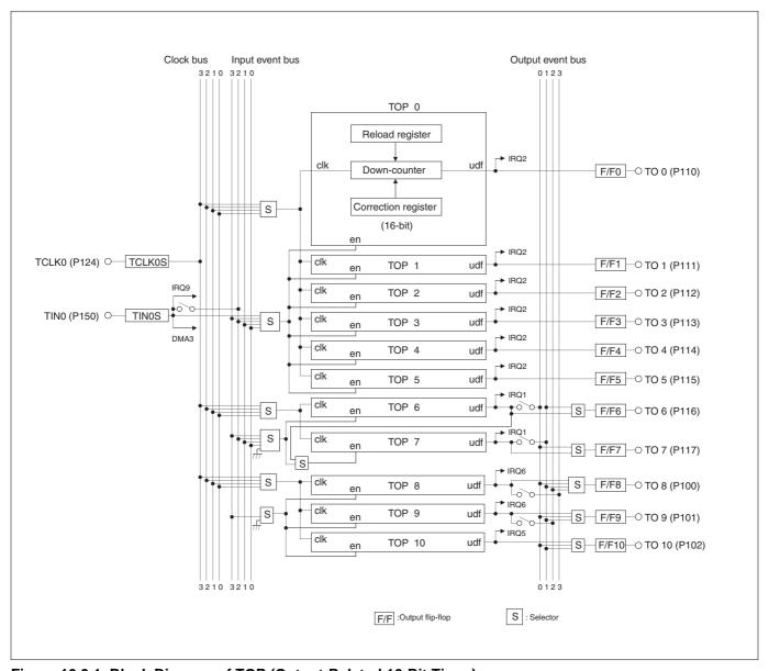
Figure 10.3.1 Block Diagram of TOP (Output-Related 16-Bit Timer)
