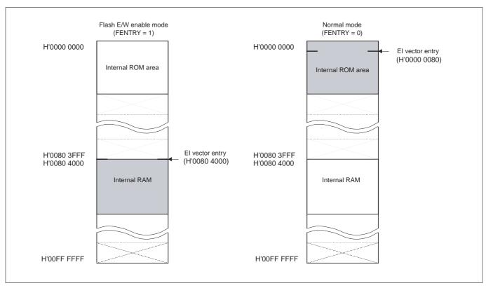
Figure 6.5.1 El Vector Entry during Flash E/W Enable Mode
