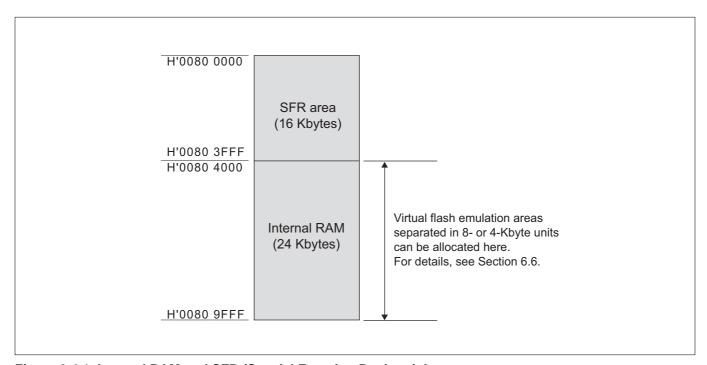
Figure 3.4.1 Internal RAM and SFR (Special Function Register) Areas
