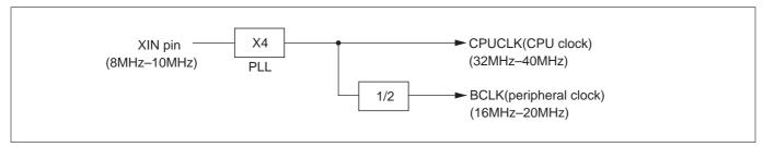
Figure 18.2.1 Conceptual Diagram of Clock Generation
