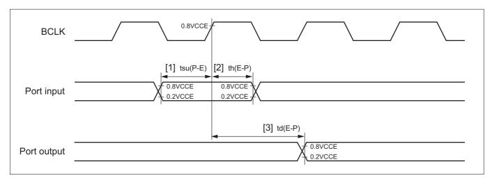
Figure 21.8.2 Input/Output Port Timing
