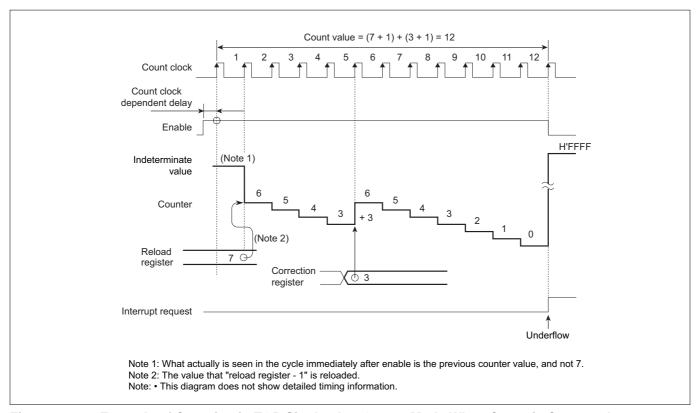
Figure 10.3.9 Example of Counting in TOP Single-shot Output Mode When Count is Corrected
