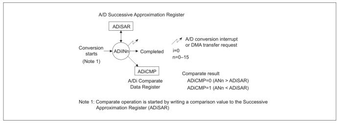
Figure 11.1.3 Operation in Single Mode (Comparate)
