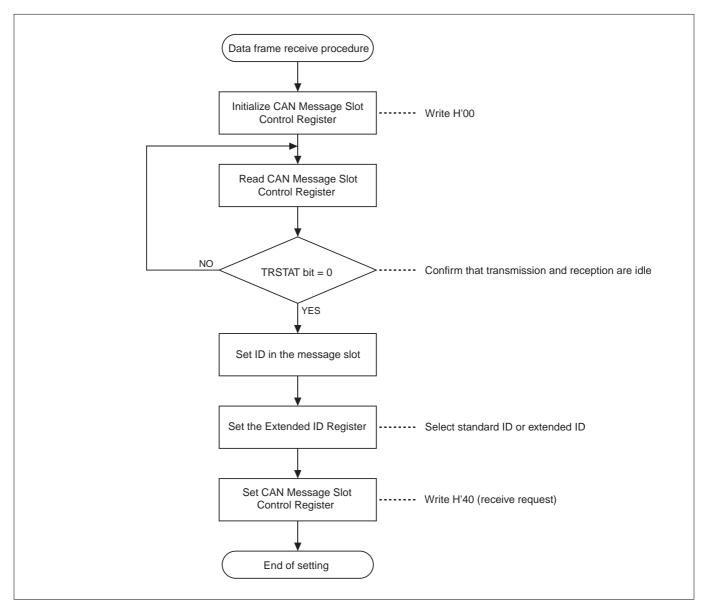
Figure 13.6.1 Data Frame Receive Procedure
