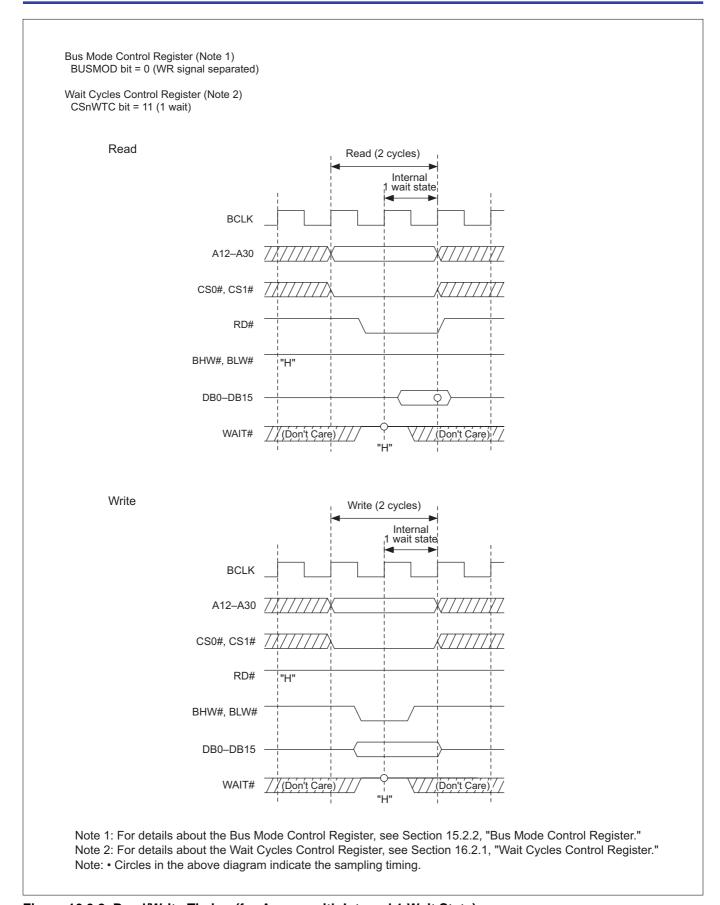
Figure 16.3.2 Read/Write Timing (for Access with Internal 1 Wait State)
