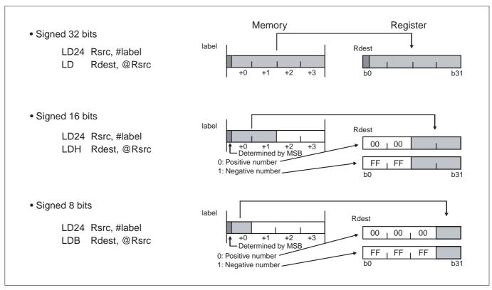
Figure 2.6.7 Transfer from Memory (Signed) to Registers
