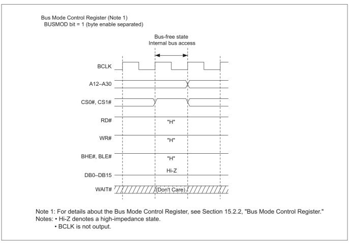
Figure 15.3.4 Internal Bus Access during Bus Free State
