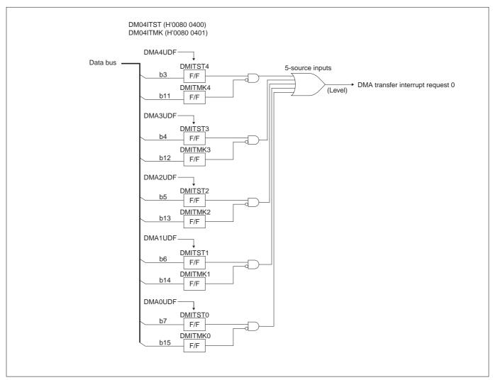
Figure 9.2.3 Block Diagram of DMA Transfer Interrupt Request 0
