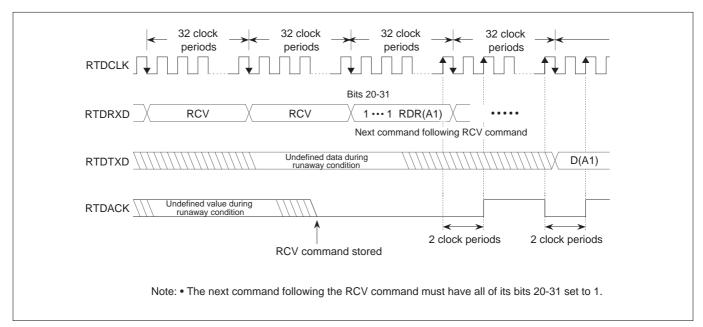
Figure 14.4.11 Operation of RCV Command
