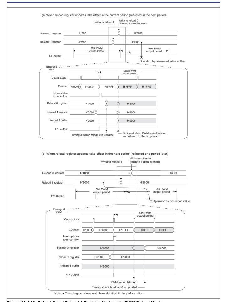
Figure 10.4.12 Reload 0 and Reload 1 Register Updates in PWM Output Mode
