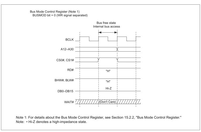
Figure 16.3.1 Internal Bus Access during Bus Free State
