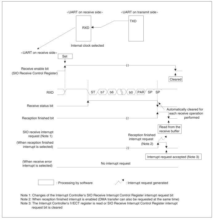
Figure 12.7.3 Example of UART Reception (When Received Normally)
