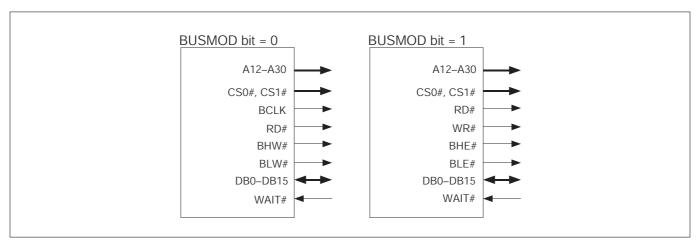
Figure 15.2.1 Pin Functions when External Bus Modes are Changed
