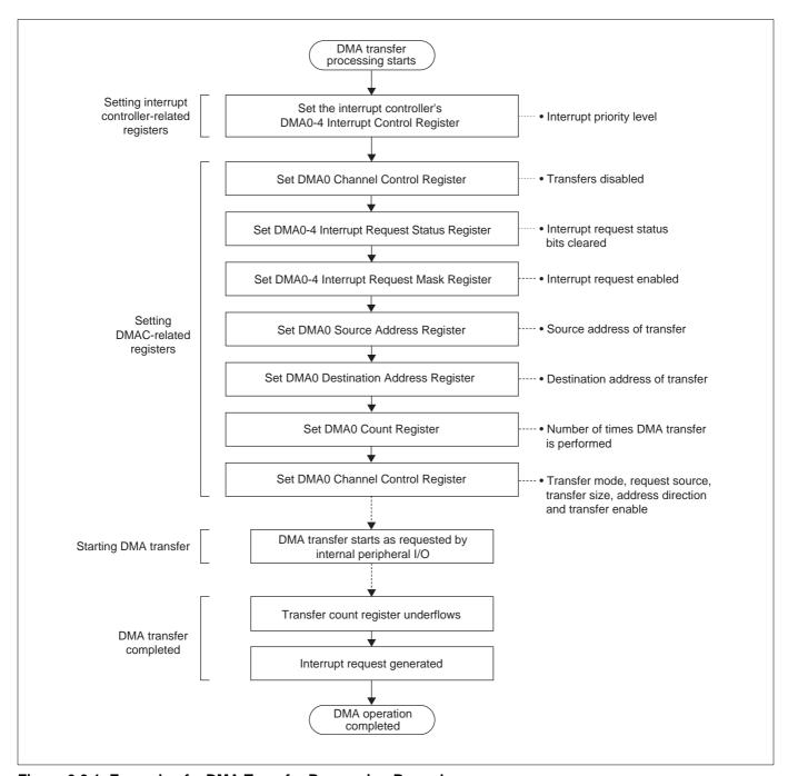
Figure 9.3.1 Example of a DMA Transfer Processing Procedure
