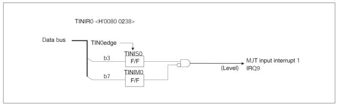
Figure 10.2.12 Block Diagram of MJT Input Interrupt 1
