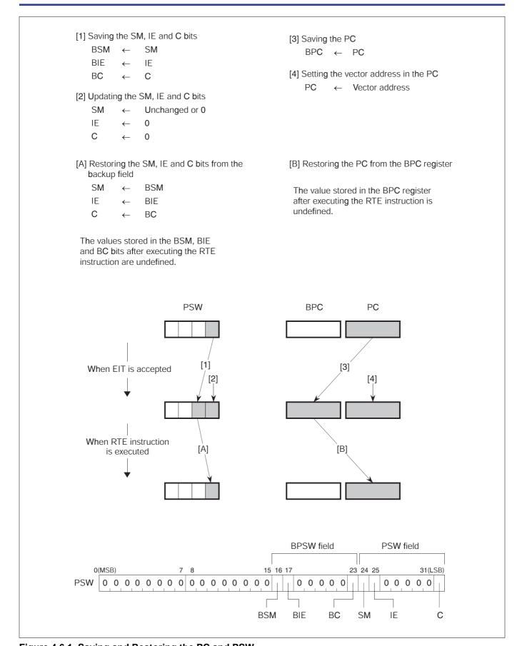
Figure 4.6.1 Saving and Restoring the PC and PSW
