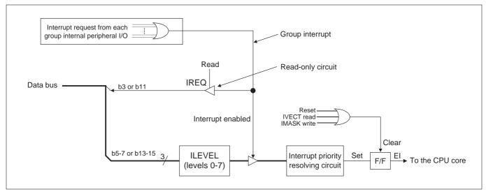
Figure 5.2.2 Configuration of the Interrupt Control Register (Level-recognized Type)
