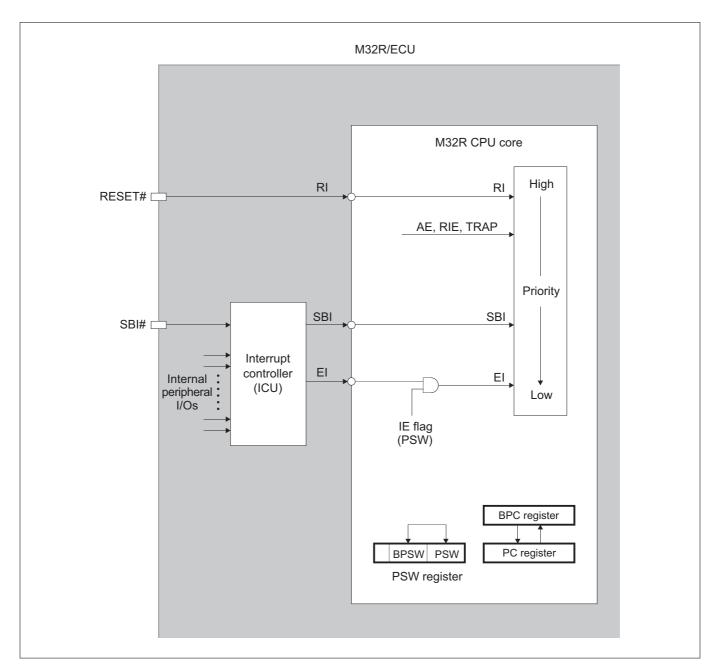
Figure 4.4.1 EIT Processing Mechanism
