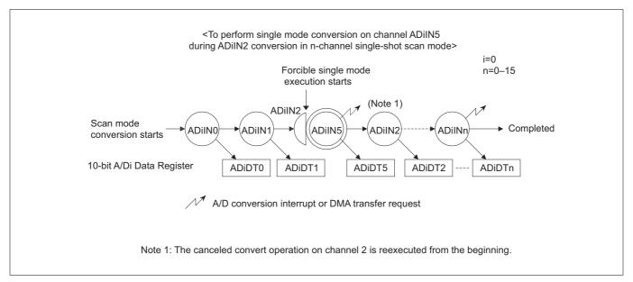
Figure 11.1.5 Forcible Single Mode Execution during Scan Mode
