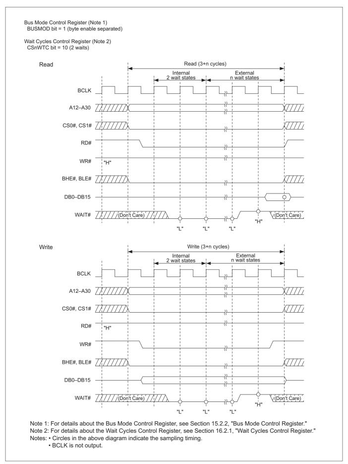
Figure 16.3.14 Read/Write Timing (for Access with Internal 2 and External n Wait States)
