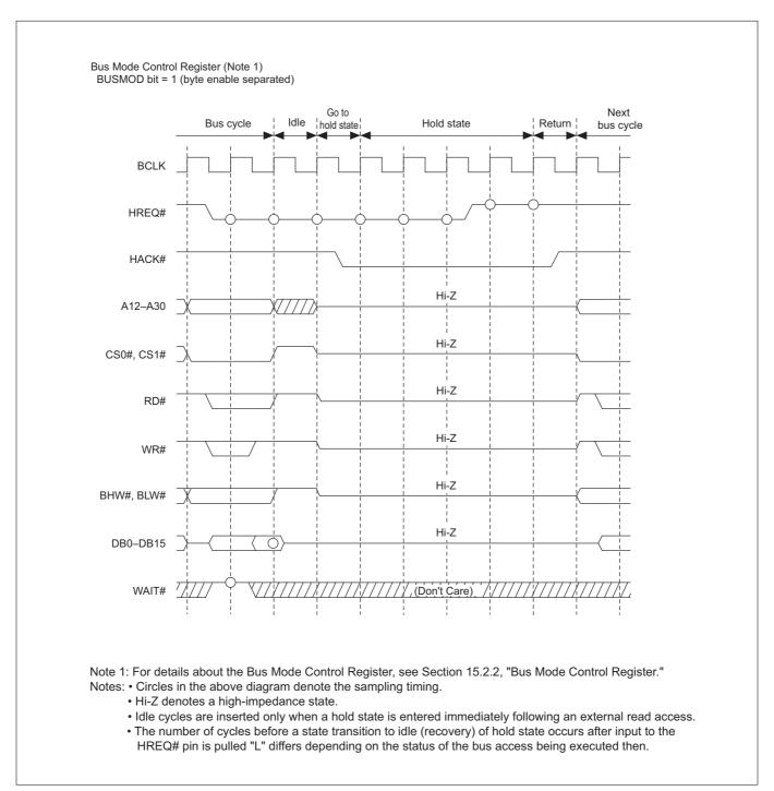
Figure 15.4.2 Bus Arbitration Timing
