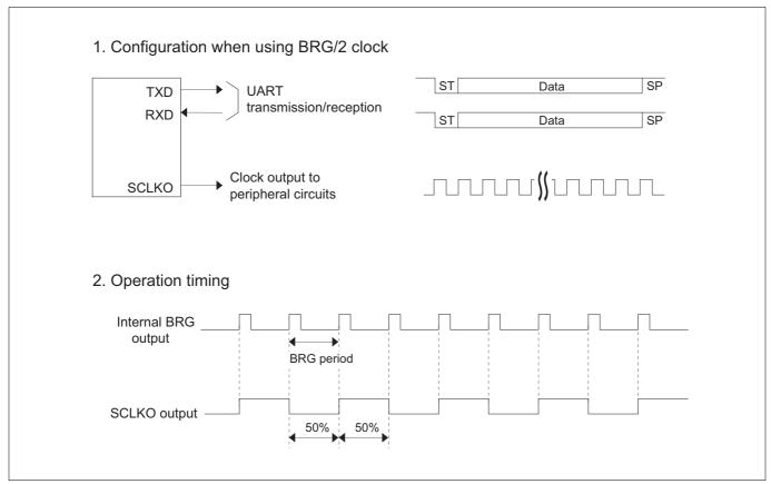
Figure 12.8.1 Example of Fixed Period Clock Output
