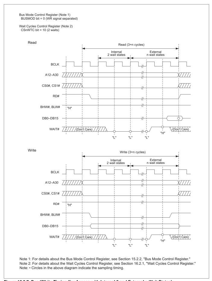
Figure 16.3.7 Read/Write Timing (for Access with Internal 2 and External n Wait States)
