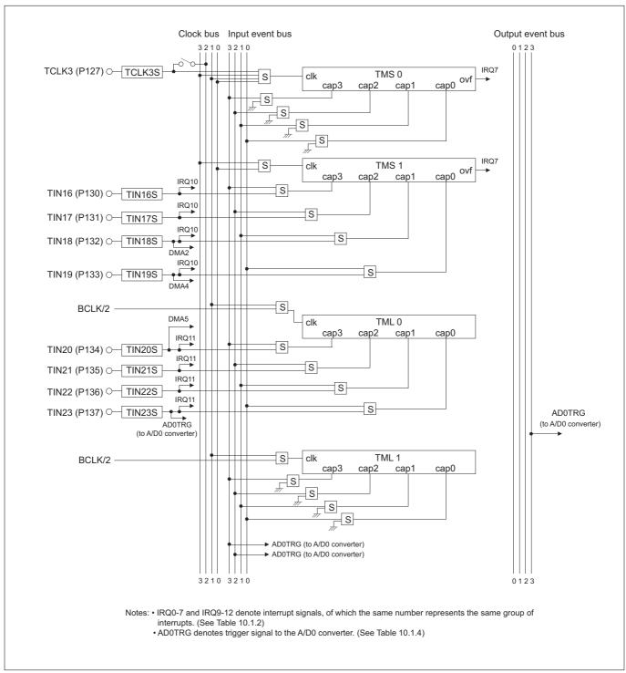
Figure 10.1.2 Block Diagram of MJT (2/3)
