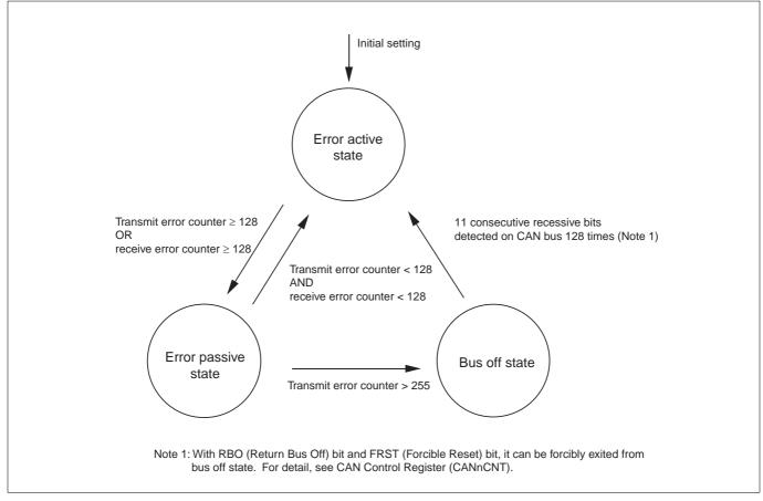
Figure 13.3.4 CAN Controller Error States
