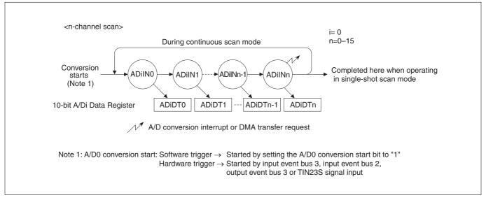
Figure 11.1.4 Operation of A/D Conversion in Scan Mode
