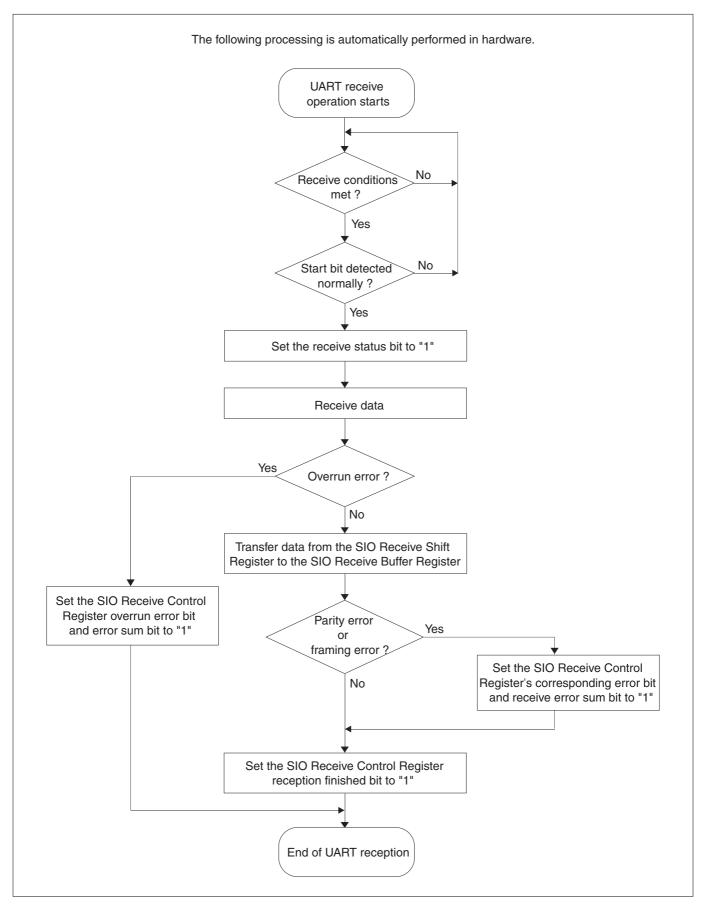
Figure 12.7.2 Receive Operation during UART Mode (Hardware Processing)
