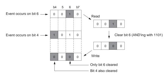
Figure 13.2.2 Example for Clearing Interrupt Request Status
