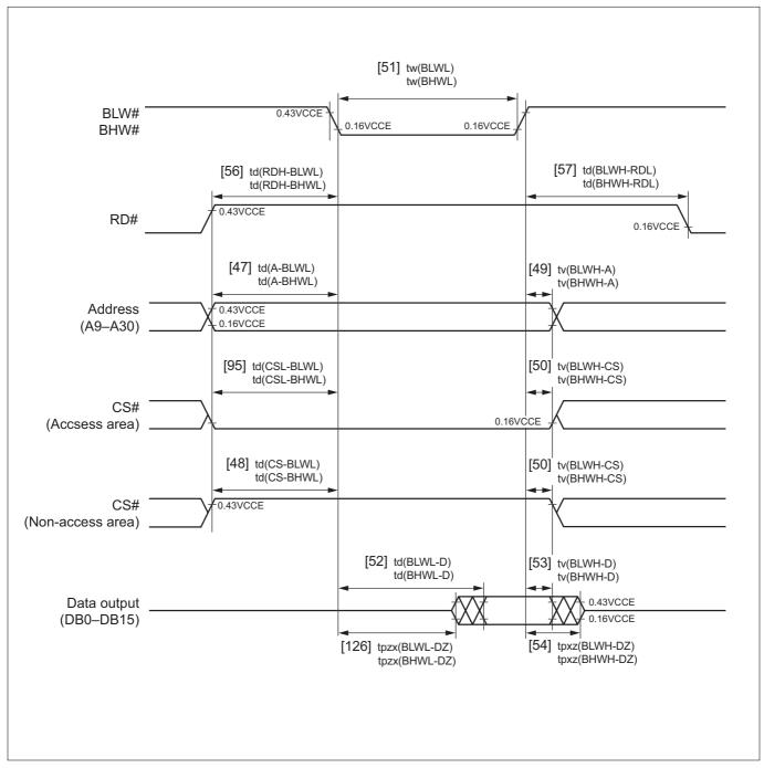
Figure 21.8.11 Write Timing (Relative to Write pulse)
