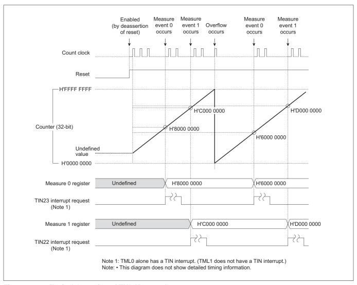
Figure 10.6.2 Typical Operation of TML Measure Input
