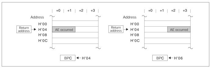
Figure 4.8.2 Example of a Return Address for Address Exception (AE)
