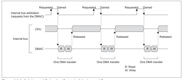
Figure 9.3.2 Gaining and Releasing Control of the Internal Bus
