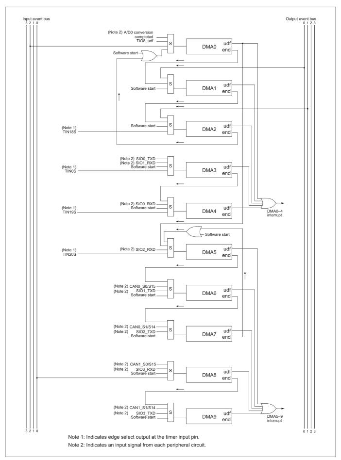
Figure 9.1.1 Block Diagram of the DMAC
