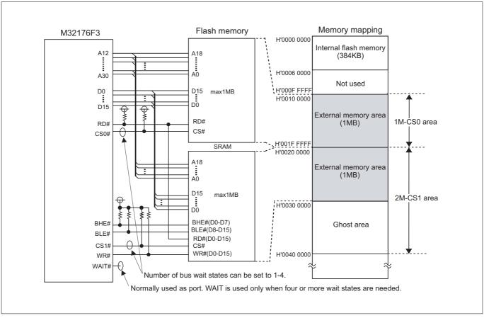
Figure 15.5.2 Typical Connection of External Extension Memory (when BUSMOD bit = "1")
