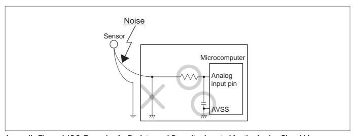
Appendix Figure 4.15.5 Example of a Resistor and Capacitor Inserted for the Analog Signal Line
