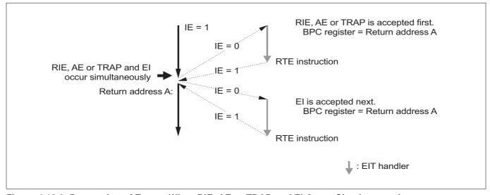
Figure 4.12.2 Processing of Events When RIE, AE or TRAP and El Occur Simultaneously
