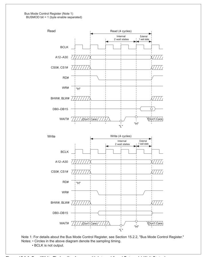
Figure 15.3.6 Read/Write Timing (for Access with Internal 2 and External 1 Wait States)
