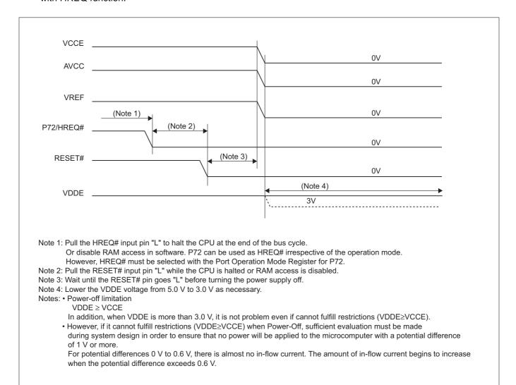
Figure 20.3.2 Power-Off Sequence when Using RAM Backup (VCCE = 5.0 V or 3.3 V)
