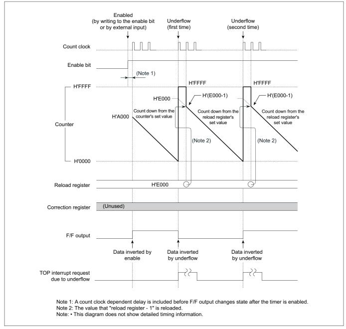
Figure 10.3.18 Typical Operation in TOP Continuous Output Mode
