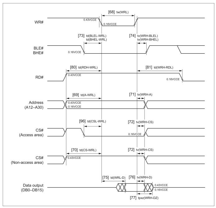
Figure 21.9.13 Write Timing (Byte Enable Mode)
