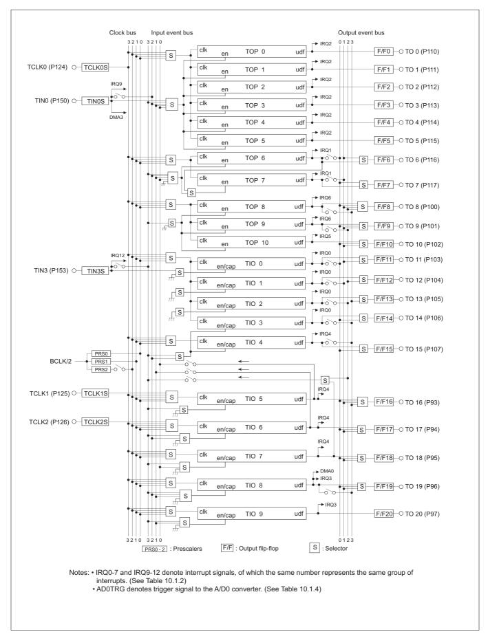
Figure 10.1.1 Block Diagram of MJT (1/3)
