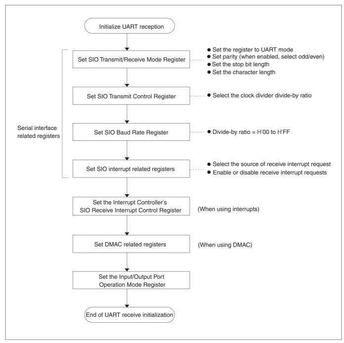
Figure 12.7.1 Procedure for Initializing UART Reception
