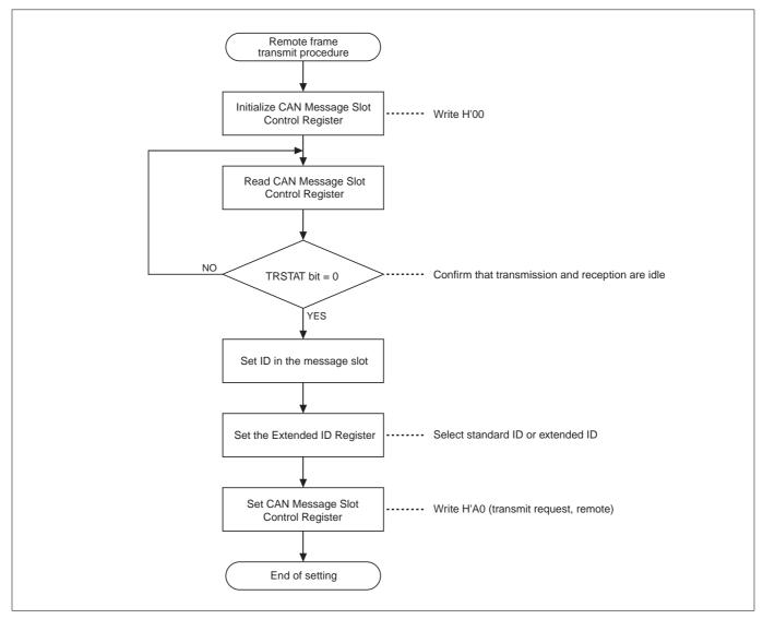
Figure 13.7.1 Remote Frame Transmit Procedure
