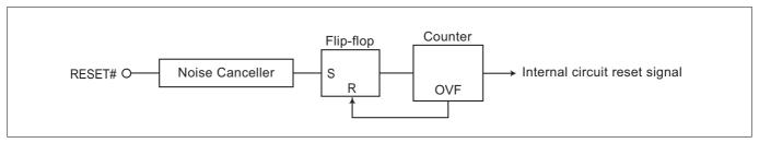
Figure 7.2.1 Reset Circuit
