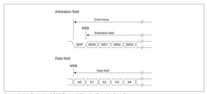
Figure 13.3.3 Example of CAN Transmit/Receive Transfer Data Format
