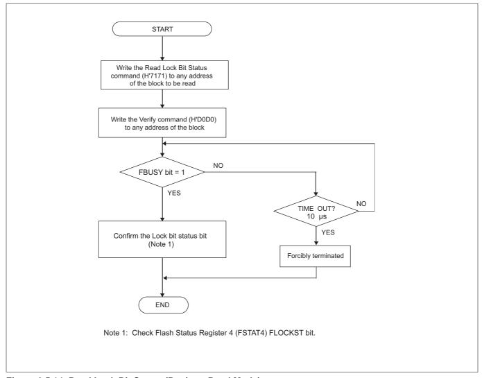
Figure 6.5.14 Read Lock Bit Status (Register Read Mode)
