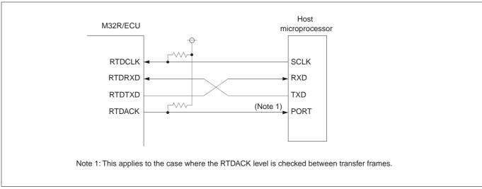
Figure 14.5.1 Connecting the RTD and Host
