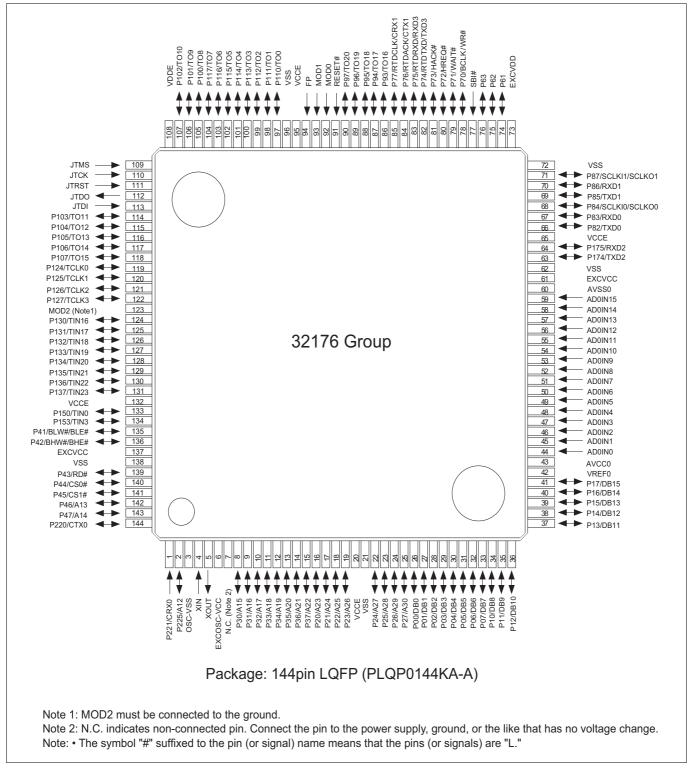
Figure 1.4.1 Pin Assignment Diagram (Top View)
