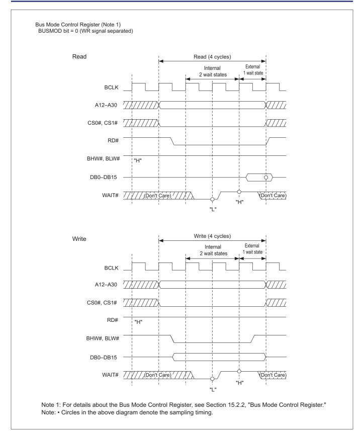
Figure 15.3.3 Read/Write Timing (for Access with Internal 2 and External 1 Wait States)
