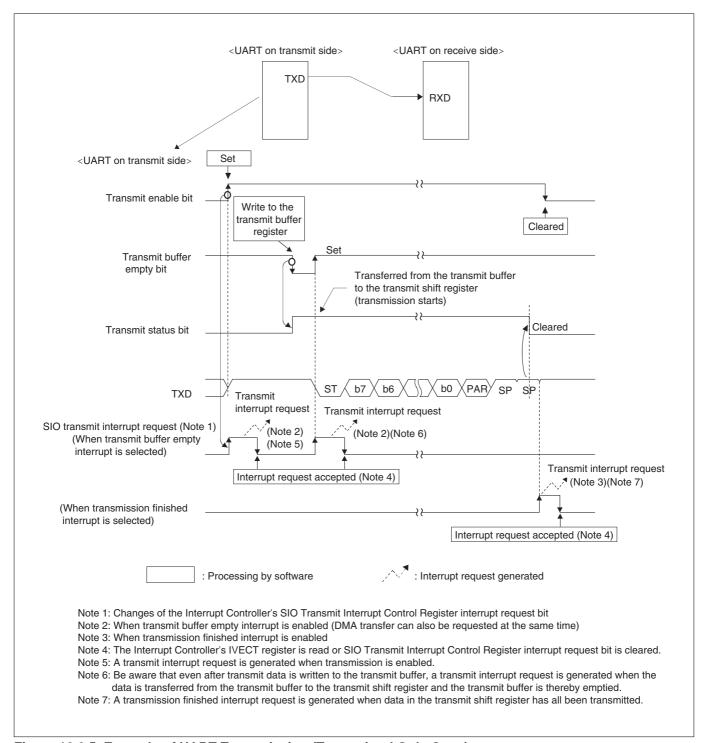
Figure 12.6.5 Example of UART Transmission (Transmitted Only Once)
