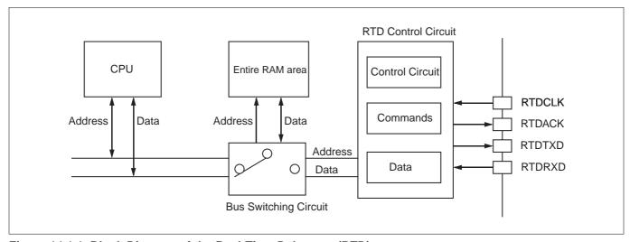
Figure 14.1.1 Block Diagram of the Real-Time Debugger (RTD)
