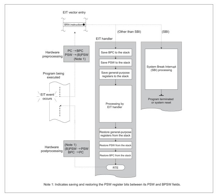
Figure 4.12.3 Example of EIT Processing
