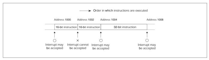
Figure 4.9.1 Timing at Which System Break Interrupt (SBI) is Accepted
