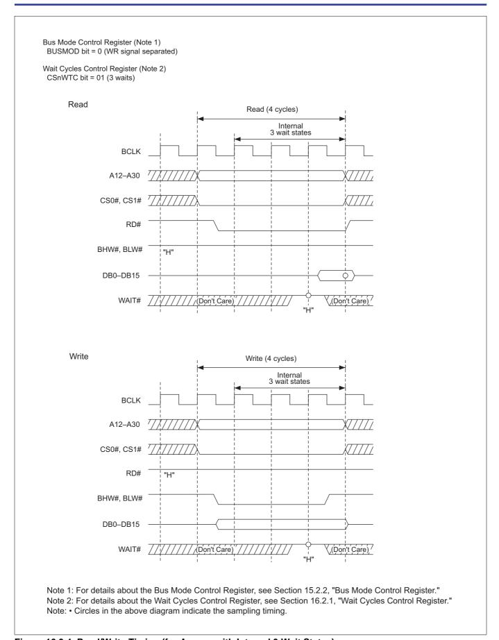
Figure 16.3.4 Read/Write Timing (for Access with Internal 3 Wait States)
