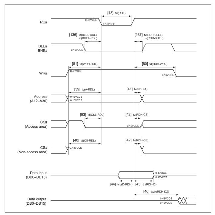
Figure 21.9.12 Read Timing (Byte Enable Mode)
