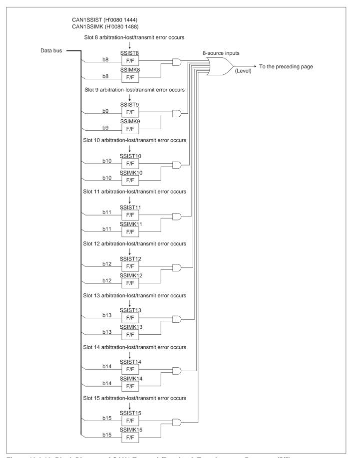
Figure 13.2.12 Block Diagram of CAN1 Transmit/Receive & Error Interrupt Requests (5/5)
