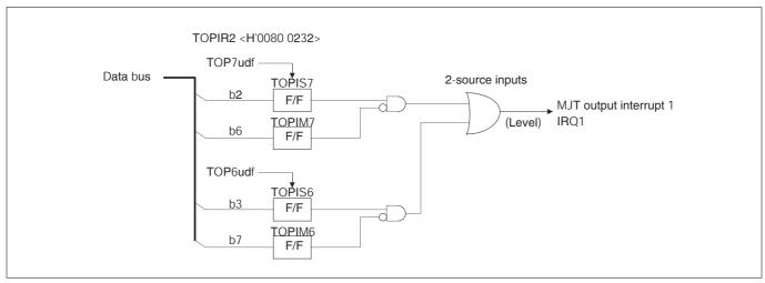
Figure 10.2.6 Block Diagram of MJT Output Interrupt 1
