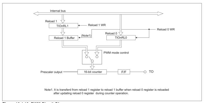
Figure 10.4.10 PWM Circuit Diagram
