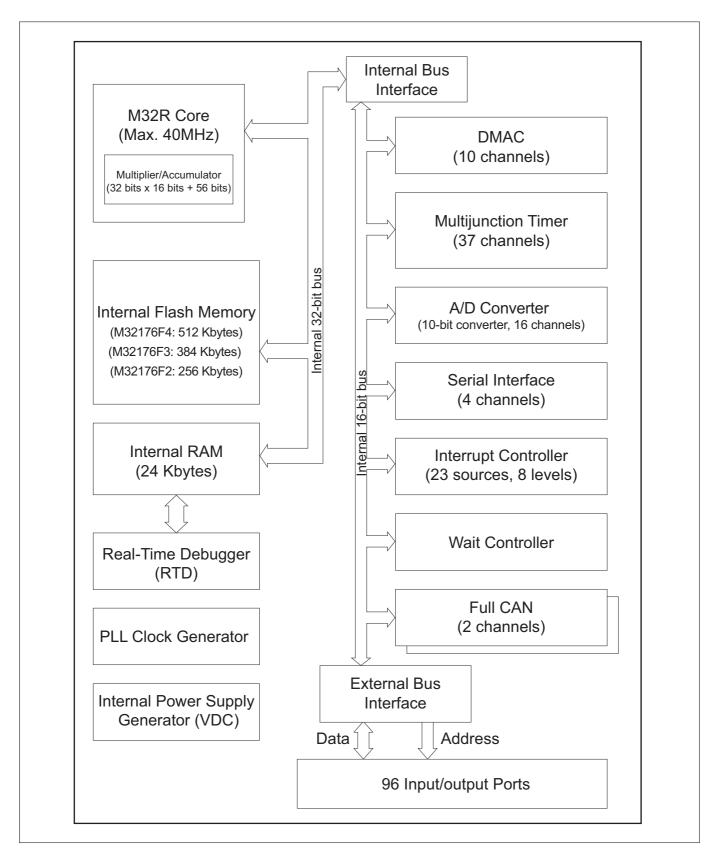
Figure 1.2.1 Block Diagram of the 32176
