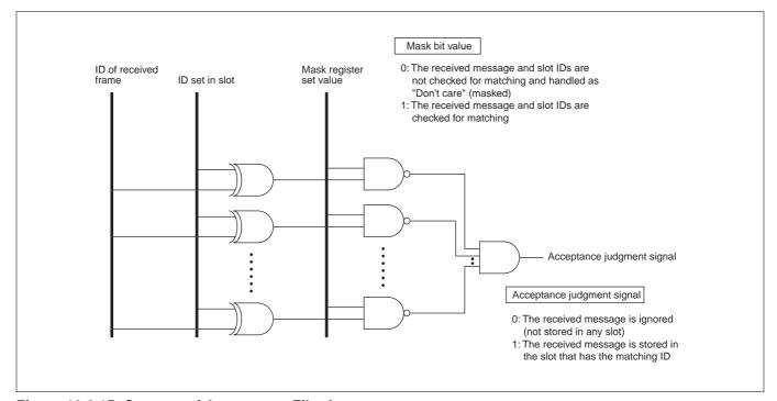
Figure 13.2.15 Concept of Acceptance Filtering
