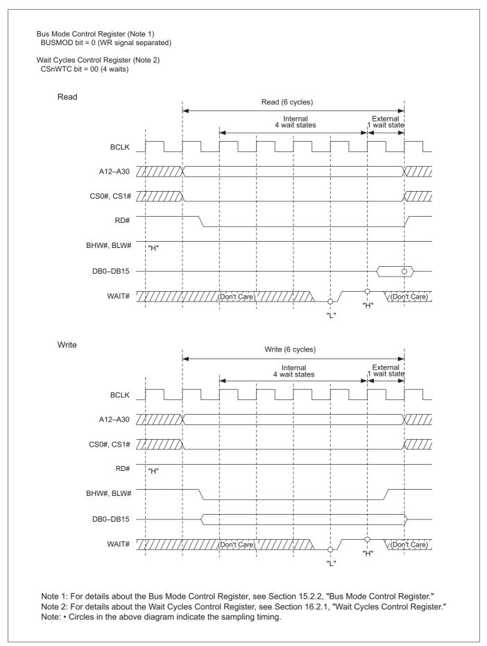
Figure 16.3.6 Read/Write Timing (for Access with Internal 4 and External 1 Wait States)
