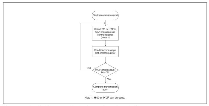
Figure 13.9.1 Opertion Flow when Aborting Remote Frame Transmission
