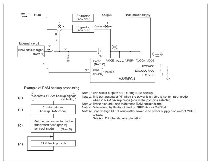
Figure 17.3.3 RAM Backup State for Low Power Operation
