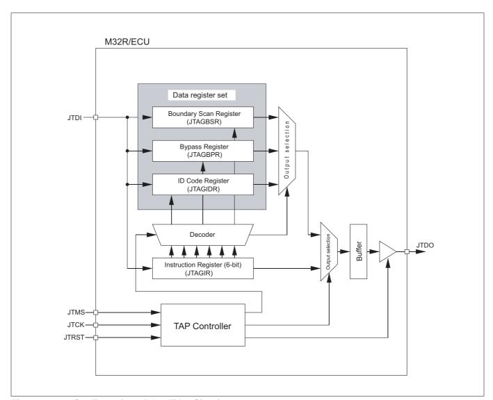
Figure 19.2.1 Configuration of the JTAG Circuit
