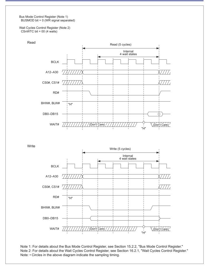
Figure 16.3.5 Read/Write Timing (for Access with Internal 4 Wait States)
