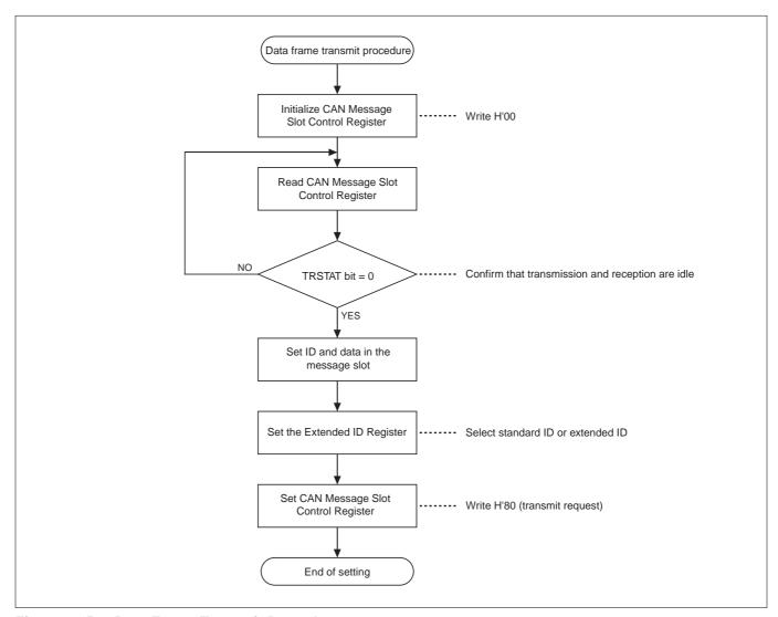
Figure 13.5.1 Data Frame Transmit Procedure
