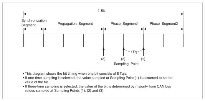
Figure 13.4.1 Example of Bit Timing
