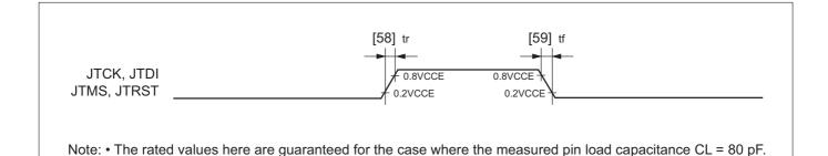
Figure 21.9.15 JTAG Pin Input Transition Time
