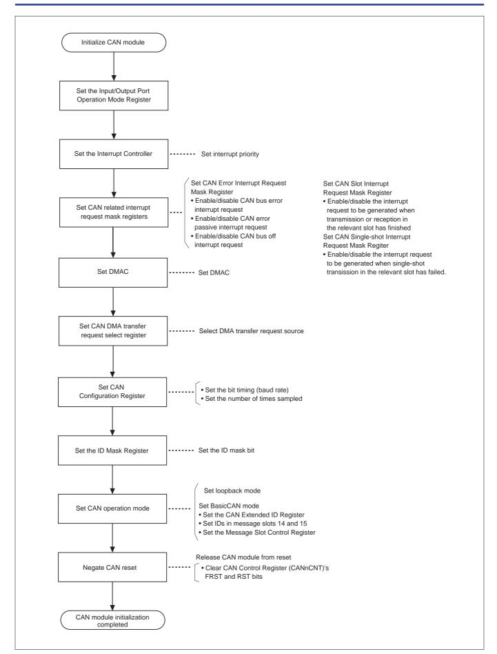
Figure 13.4.2 Initializing CAN Module
