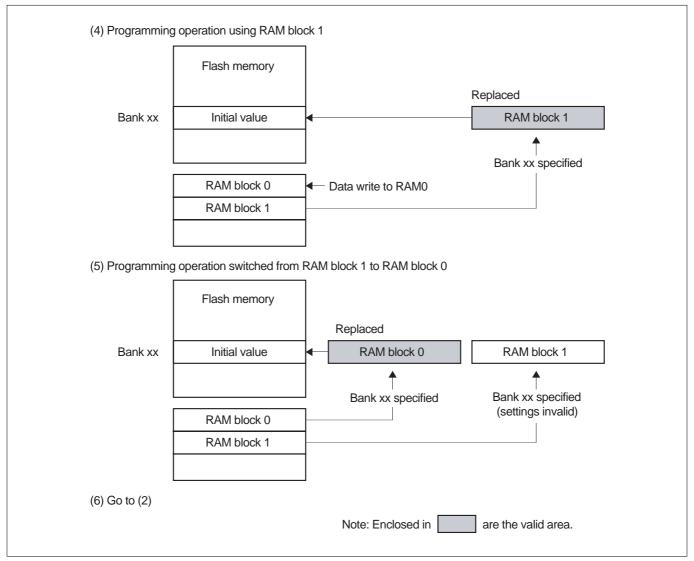
Figure 6.6.16 Application Example of Virtual Flash Emulation Mode (2/2)
