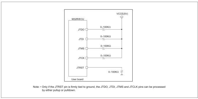
Figure 19.7.1 Processing Pins when Not Using JTAG
