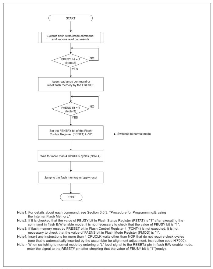
Figure 6.5.7 Procedure for switching to normal mode
