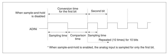
Figure 11.5.2 A/D Conversion Timing Diagram
