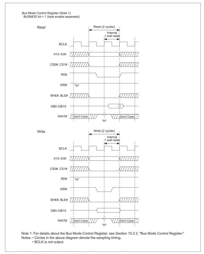
Figure 15.3.5 Read/Write Timing (for Shortest External Access)
