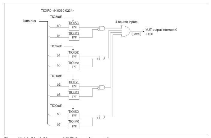
Figure 10.2.8 Block Diagram of MJT Output Interrupt 0
