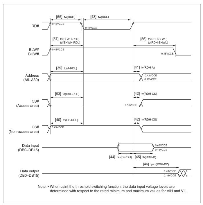
Figure 21.9.10 Read Timing (Relative to Read Pulse)
