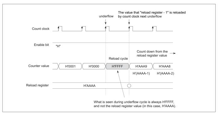
Figure 10.3.16 Counter Value Immediately after Underflow
