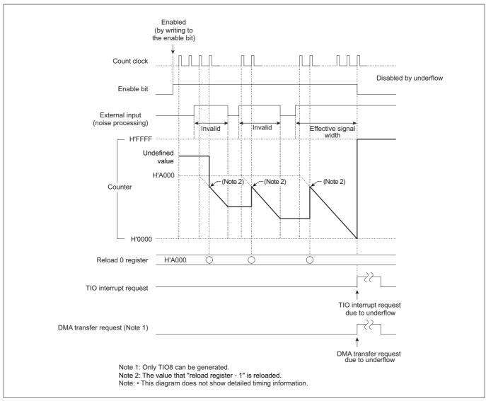
Figure 10.4.8 Typical Operation in Noise Processing Input Mode
