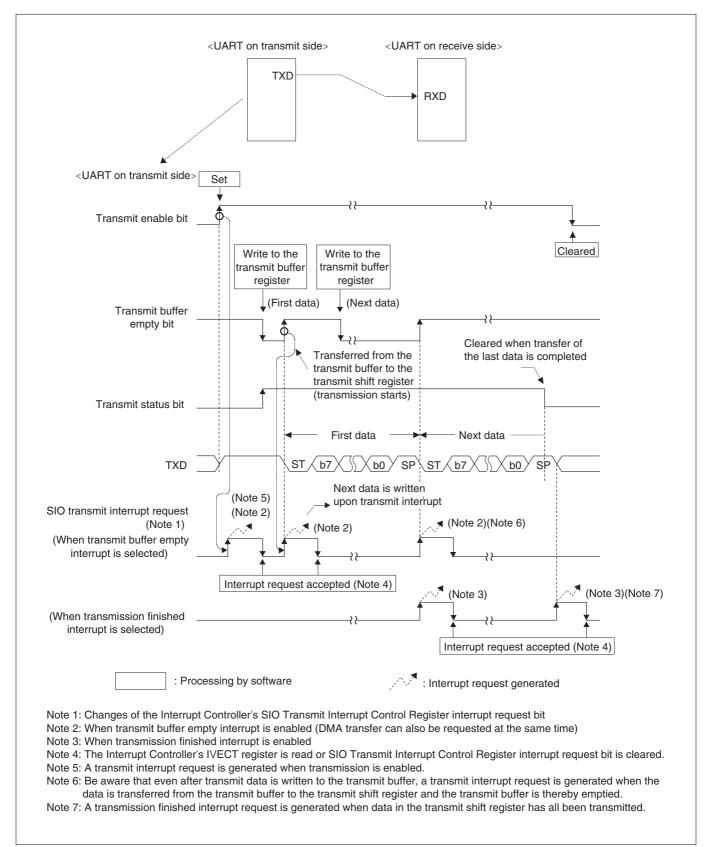
Figure 12.6.6 Example of UART Transmission (Transmitted Successively)
