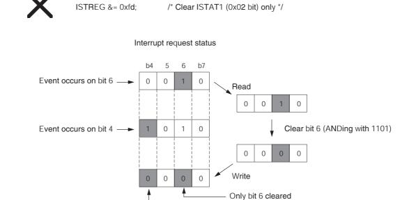
Figure 10.2.4 Example for Clearing Interrupt Request Status
