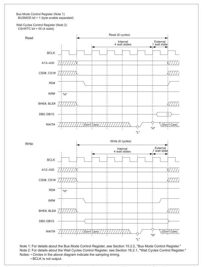
Figure 16.3.13 Read/Write Timing (for Access with Internal 4 and External 1 Wait States)
