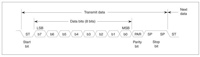
Figure 12.6.1 Example of a Transfer Data Format during UART Mode
