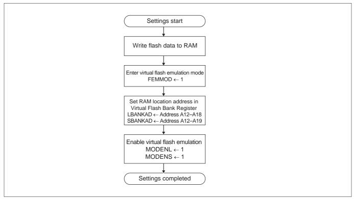
Figure 6.6.14 Virtual Flash Emulation Mode Sequence
