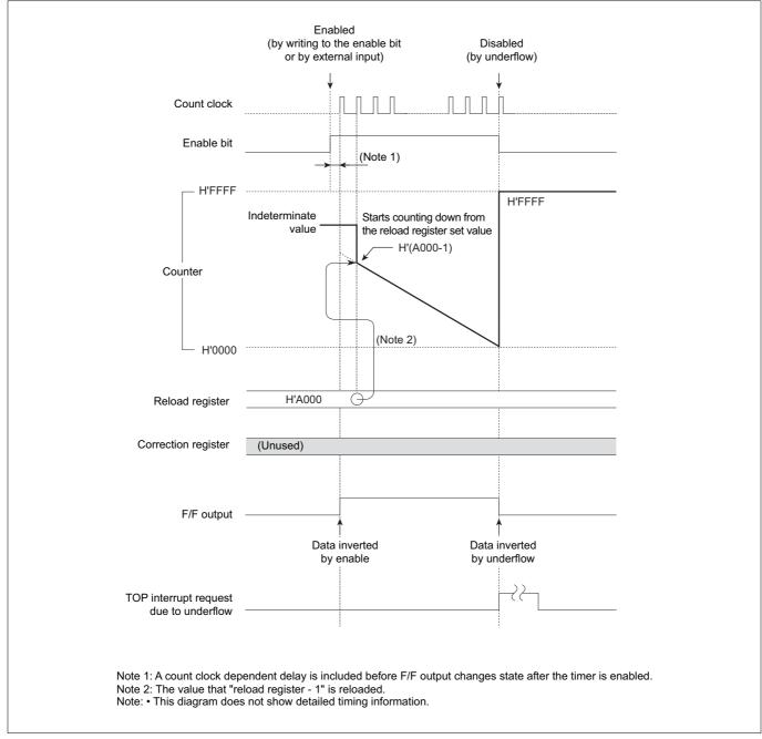
Figure 10.3.8 Typical Operation in TOP Single-shot Output Mode
