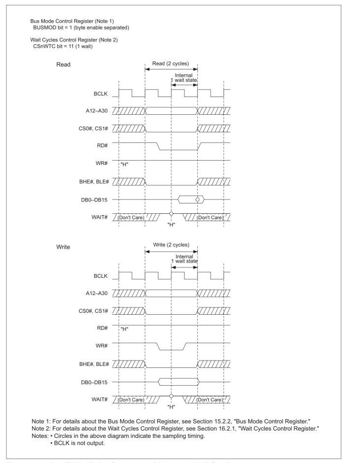
Figure 16.3.9 Read/Write Timing (for Access with Internal 1 Wait State)
