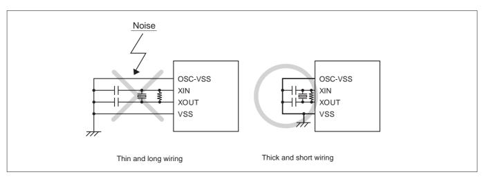
Appendix Figure 4.15.2 Example Wiring of Clock Input/Output Pins
