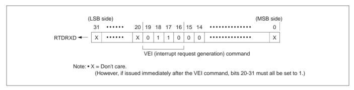
Figure 14.4.8 VEI (Interrupt Request) Command Data Format
