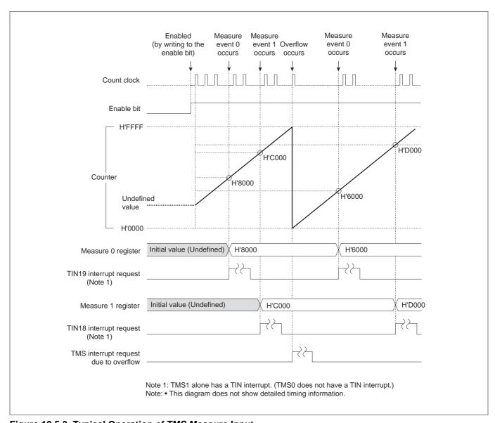
Figure 10.5.3 Typical Operation of TMS Measure Input
