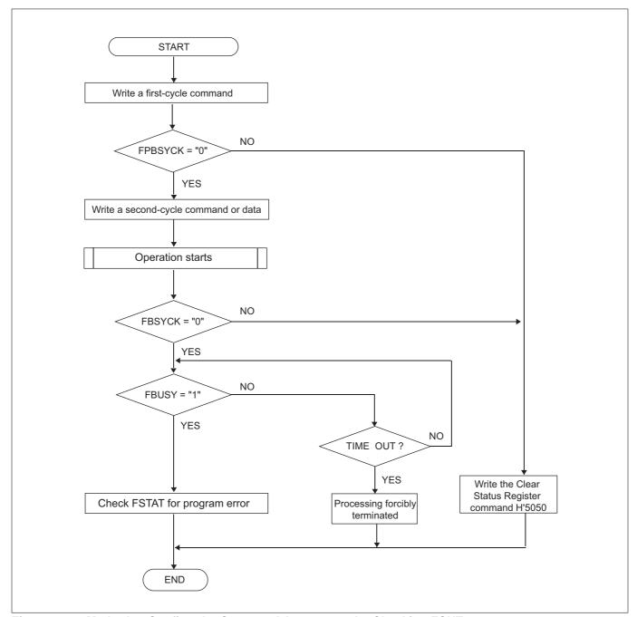
Figure 6.4.2 Method to Confirm the Command Acceptance by Checking FCNT3
