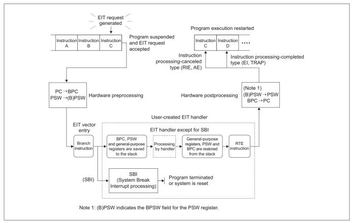
Figure 4.3.1 Outline of the EIT Processing Procedure
