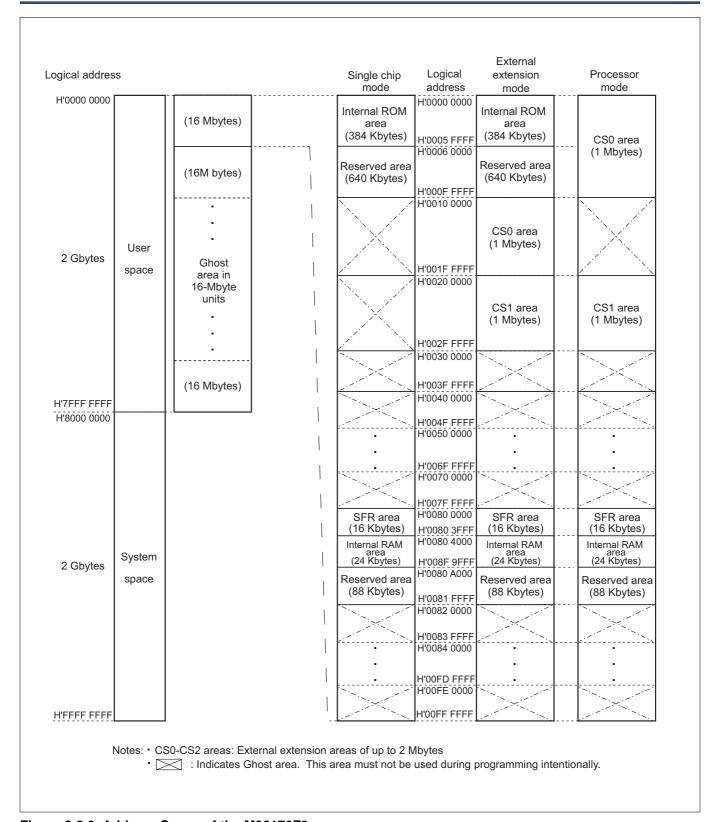
Figure 3.2.2 Address Space of the M32176F3
