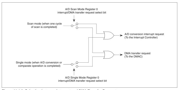
Figure 11.1.9 Selecting between Interrupt and DMA Transfer Requests
