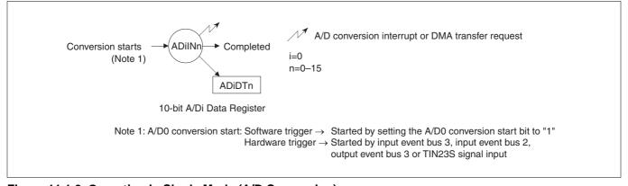
Figure 11.1.2 Operation in Single Mode (A/D Conversion)
