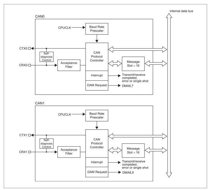
Figure 13.1.1 Block Diagram of the CAN Modules
