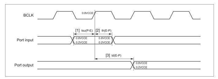
Figure 21.9.2 Input/Output Port Timing
