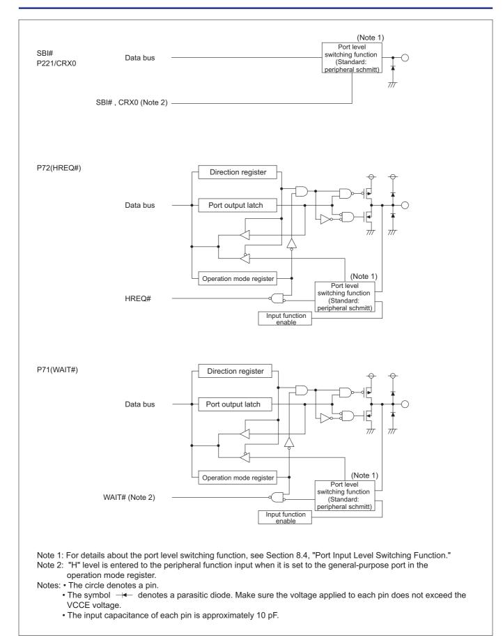
Figure 8.5.2 Port Peripheral Circuit Diagram (2)
