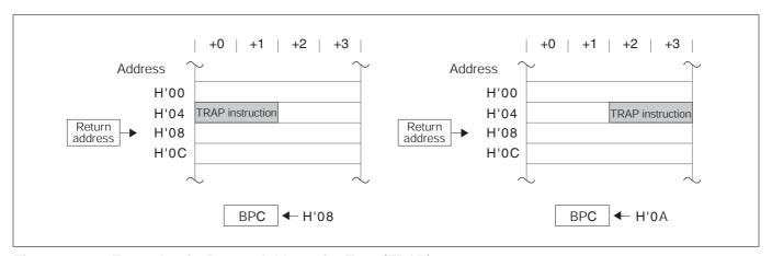
Figure 4.10.1 Example of a Return Address for Trap (TRAP)
