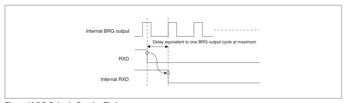
Figure 12.7.7 Delay in Receive Timing
