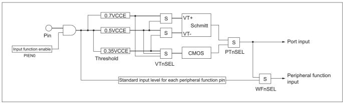
Figure 8.4.1 Port Level Switching Function
