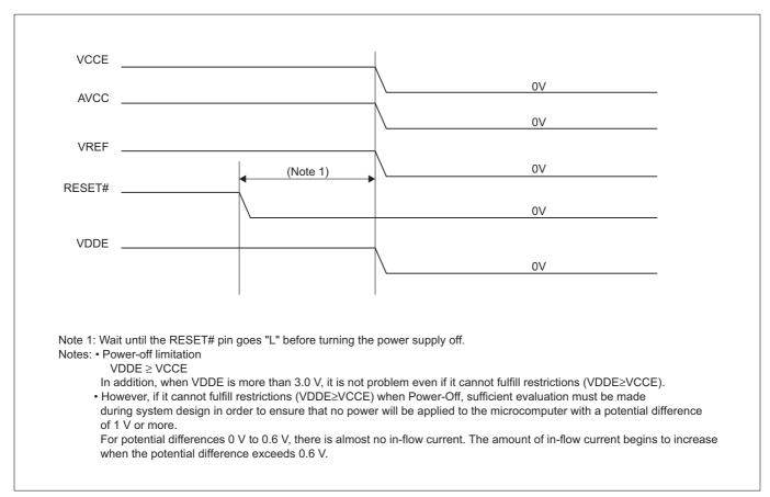
Figure 20.3.1 Power-Off Sequence when Not Using RAM Backup
