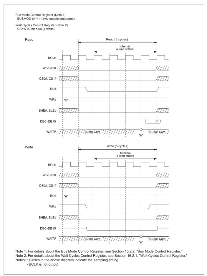
Figure 16.3.12 Read/Write Timing (for Access with Internal 4 Wait States)
