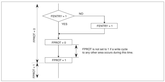
Figure 6.4.1 Protection Unlocking Flow
