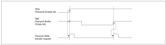
Figure 12.2.3 Transmit DMA Transfer Request
