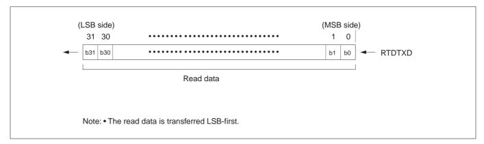
Figure 14.4.3 Read Data Transfer Format
