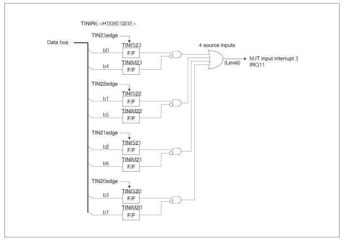
Figure 10.2.15 Block Diagram of MJT Input Interrupt 3
