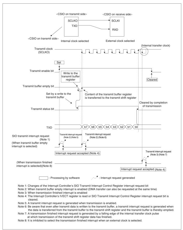
Figure 12.3.3 Example of CSIO Transmission (Transmitted Only Once)
