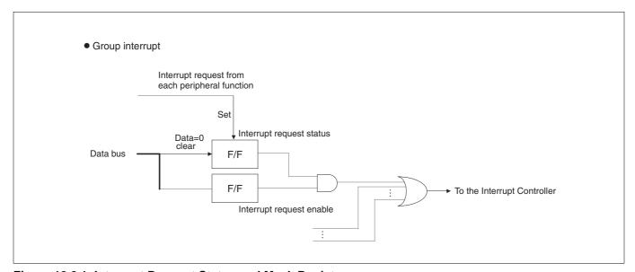
Figure 12.2.1 Interrupt Request Status and Mask Registers
