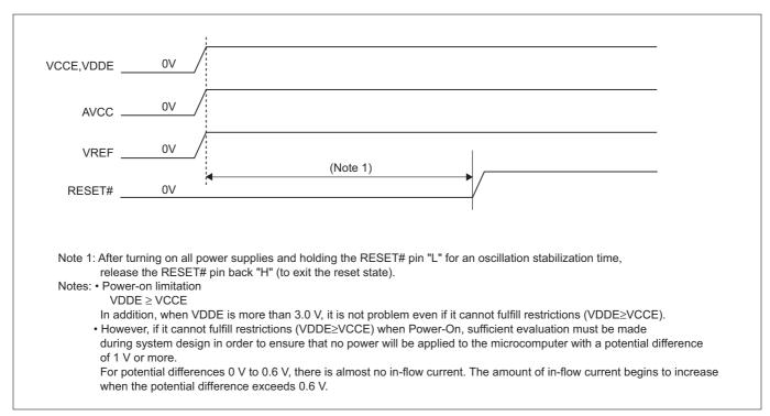
Figure 20.2.1 Power-On Sequence when Not Using RAM Backup
