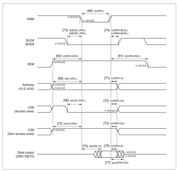
Figure 21.8.13 Write Timing (Byte Enable Mode)
