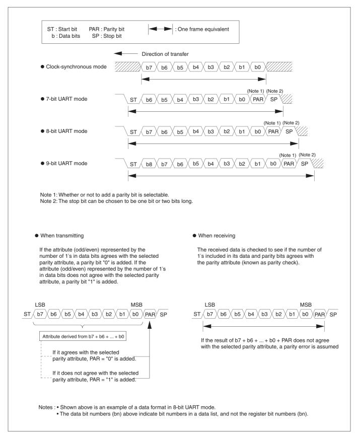
Figure 12.2.6 Data Format When Parity is Enabled
