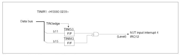
Figure 10.2.13 Block Diagram of MJT Input Interrupt 4
