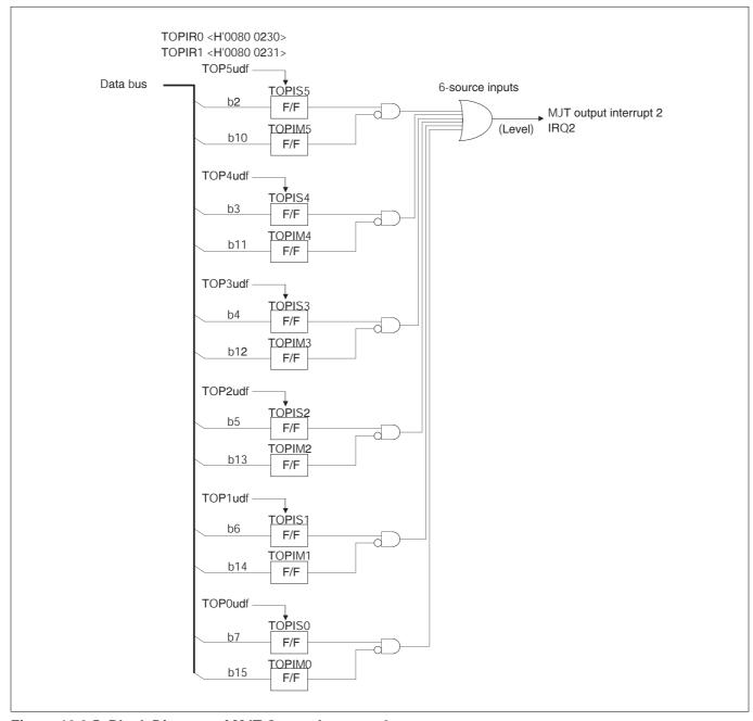
Figure 10.2.5 Block Diagram of MJT Output Interrupt 2
