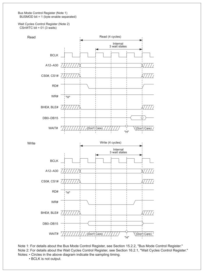
Figure 16.3.11 Read/Write Timing (for Access with Internal 3 Wait States)
