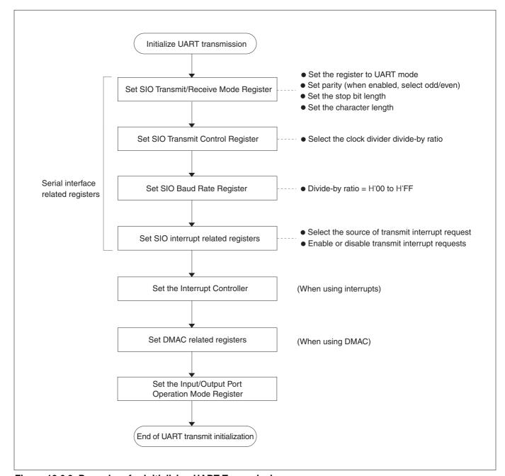
Figure 12.6.3 Procedure for Initializing UART Transmission
