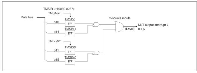
Figure 10.2.11 Block Diagram of MJT Output Interrupt 7
