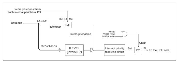
Figure 5.2.1 Configuration of the Interrupt Control Register (Edge-recognized Type)
