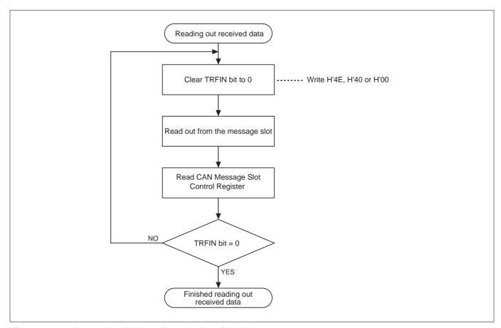
Figure 13.6.3 Procedure for Reading Out Received Data
