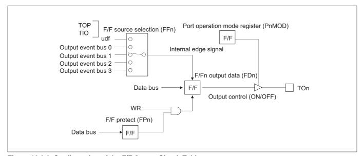
Figure 10.2.2 Configuration of the F/F Output Circuit Table
