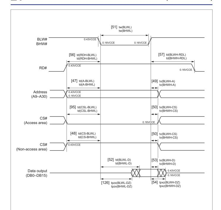
Figure 21.9.11 Write Timing (Relative to Write pulse)
