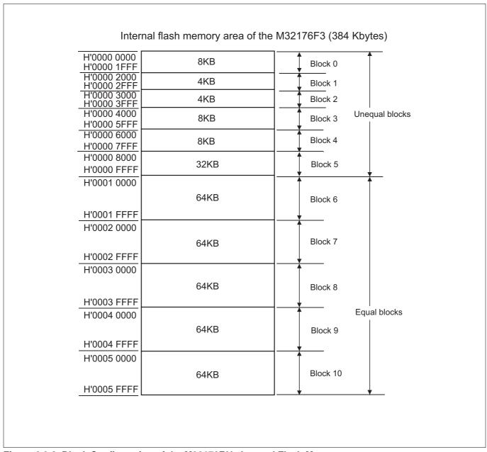
Figure 6.3.2 Block Configuration of the M32176F3's Internal Flash Memory
