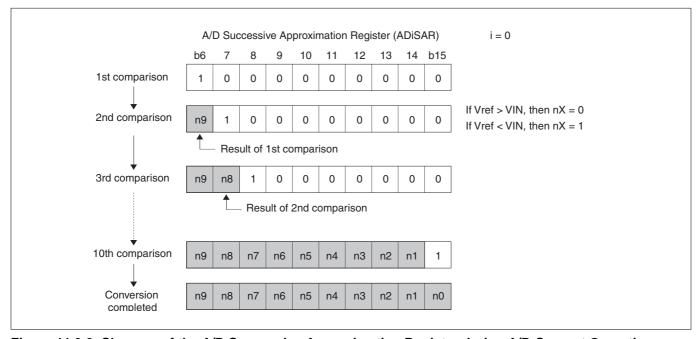
Figure 11.3.2 Changes of the A/D Successive Approximation Register during A/D Convert Operation
