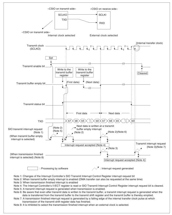
Figure 12.3.4 Example of CSIO Transmission (Transmitted Successively)
