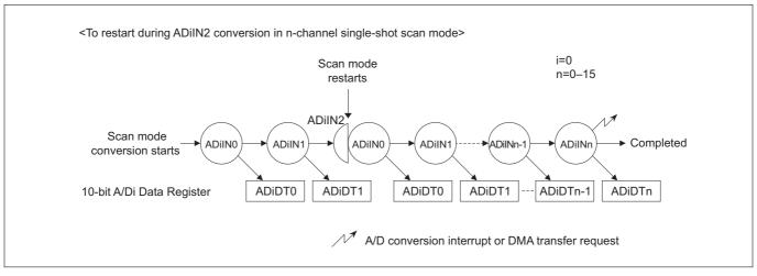
Figure 11.1.8 Conversion Restart during Scan Operation
