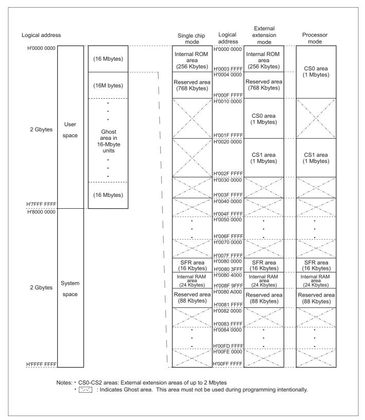
Figure 3.2.3 Address Space of the M32176F2
