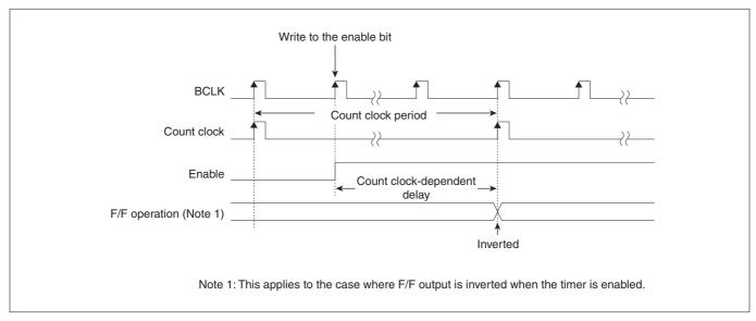
Figure 10.3.2 Count Clock Dependent Delay
