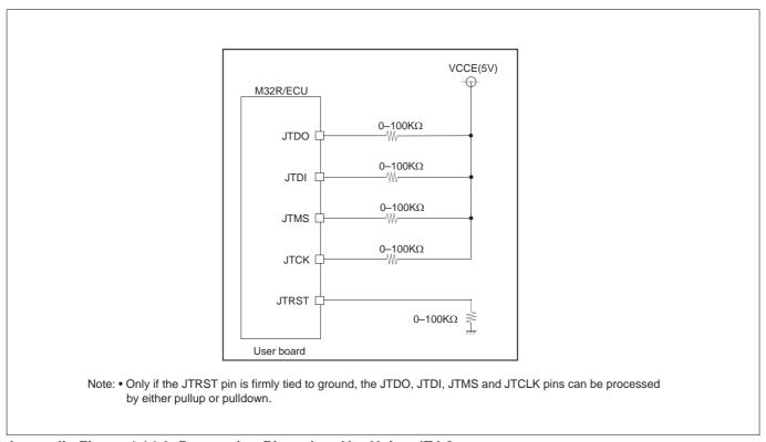
Appendix Figure 4.14.2 Processing Pins when Not Using JTAG
