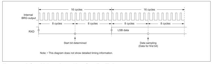
Figure 12.7.5 Start Bit Detection and Data Sampling Timing
