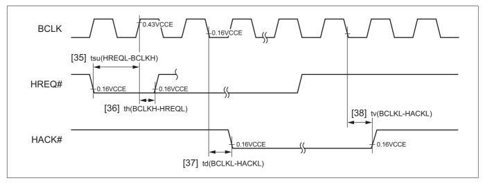
Figure 21.9.14 Bus Arbitration Timing
