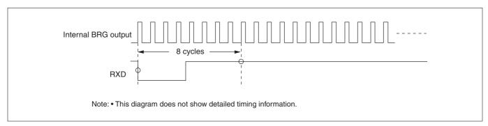
Figure 12.7.6 Example of an Invalid Start Bit (Not Received)
