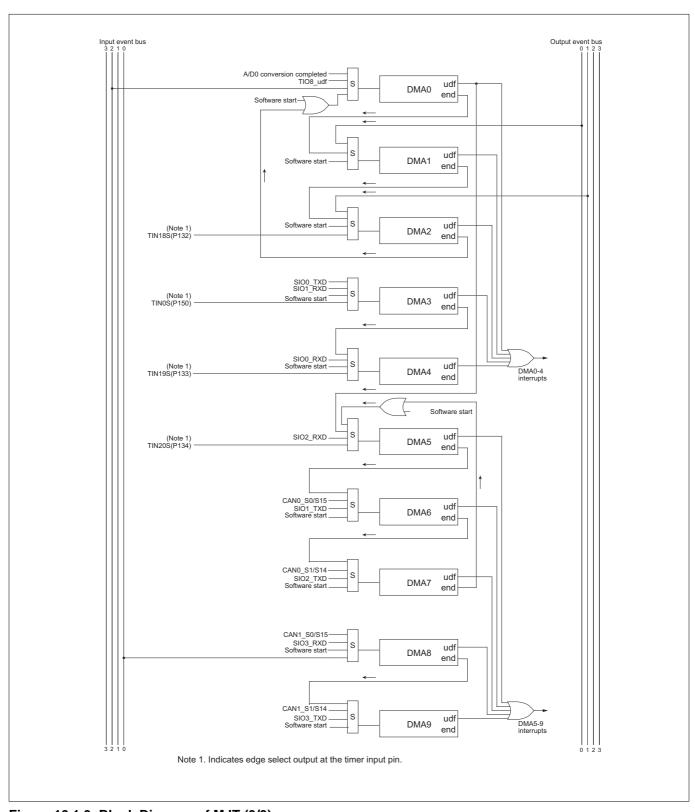
Figure 10.1.3 Block Diagram of MJT (3/3)
