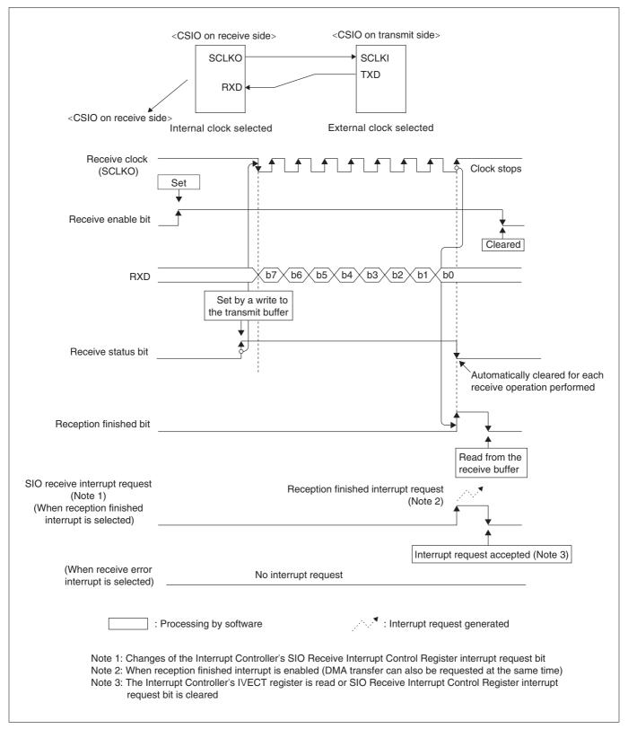
Figure 12.4.3 Example of CSIO Reception (When Received Normally)
