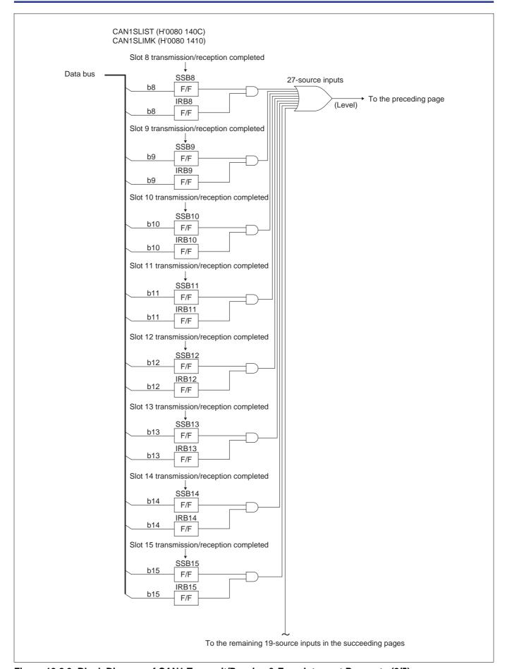
Figure 13.2.9 Block Diagram of CAN1 Transmit/Receive & Error Interrupt Requests (2/5)
