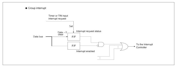
Figure 10.2.3 Interrupt Request Status and Mask Registers
