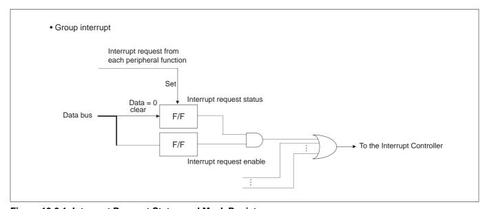
Figure 13.2.1 Interrupt Request Status and Mask Registers
