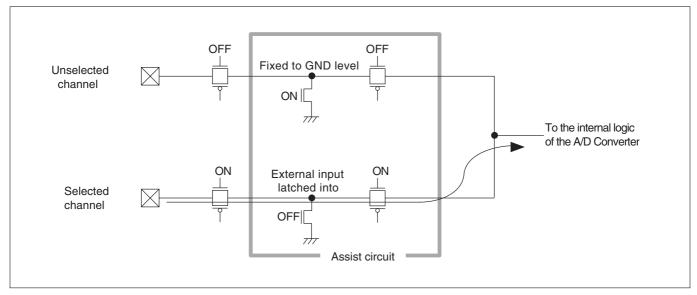
Figure 11.4.1 Configuration of the Inflow Current Bypass Circuit
