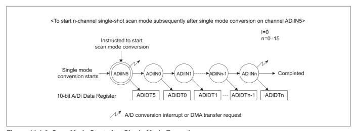
Figure 11.1.6 Scan Mode Start after Single Mode Execution
