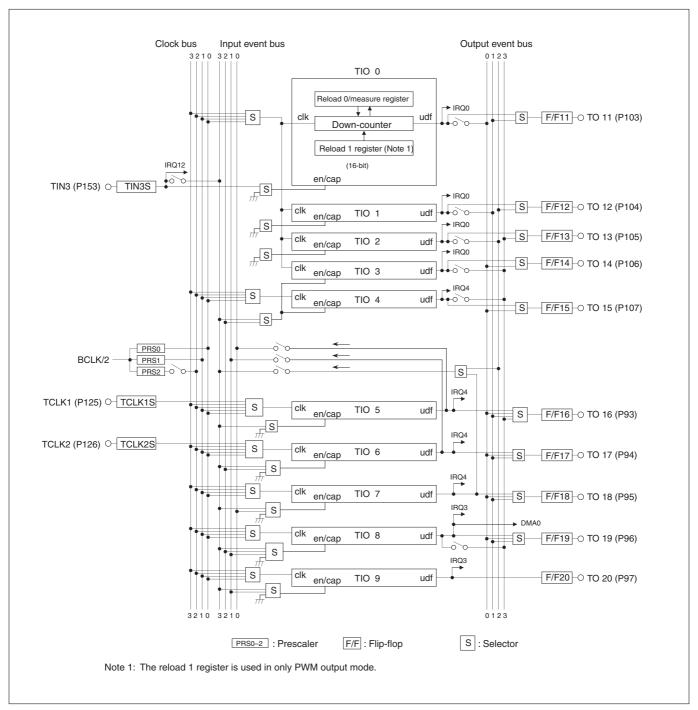
Figure 10.4.1 Block Diagram of TIO (Input/Output-Related 16-Bit Timer)
