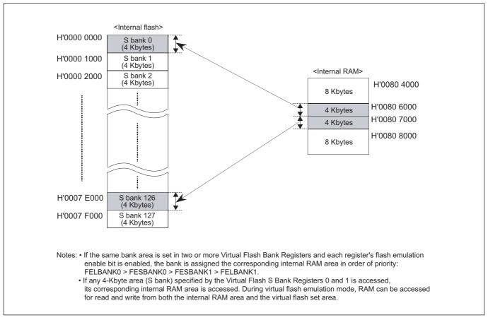
Figure 6.6.3 M32176F4 Virtual Flash Emulation Area divided in 4-Kbyte units
