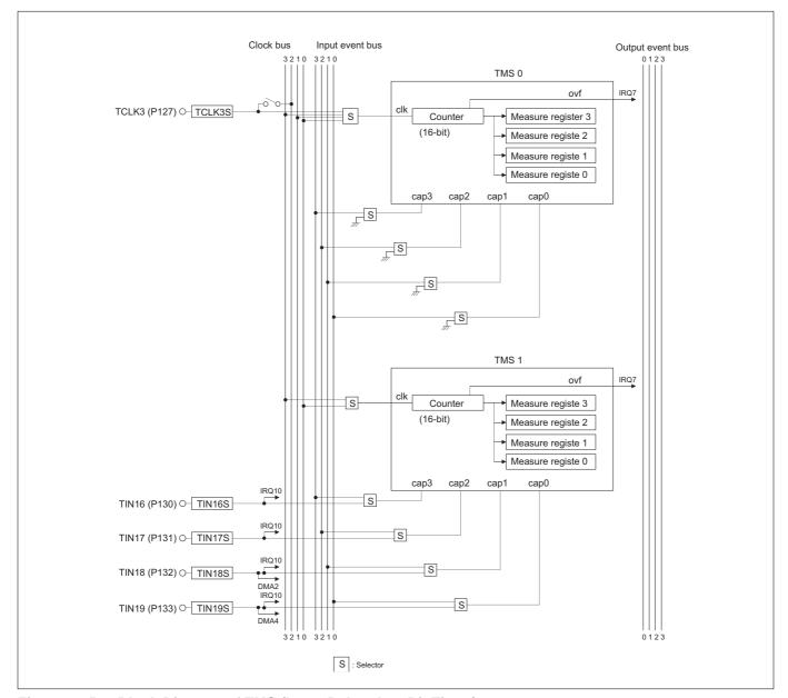
Figure 10.5.1 Block Diagram of TMS (Input-Related 16-Bit Timer)
