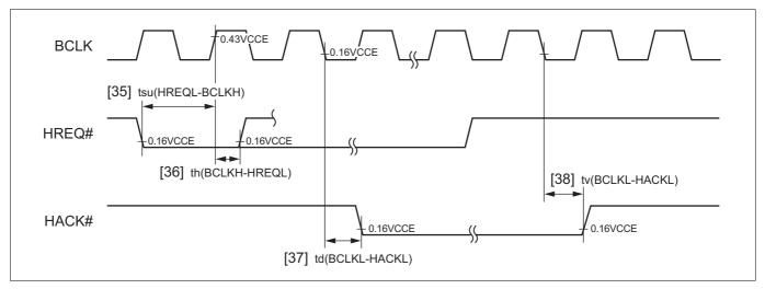
Figure 21.8.14 Bus Arbitration Timing
