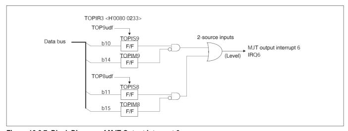
Figure 10.2.7 Block Diagram of MJT Output Interrupt 6
