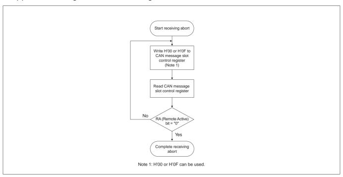
Figure 13.9.2 Opertion Flow when Canceling Remote Frame Receiving
