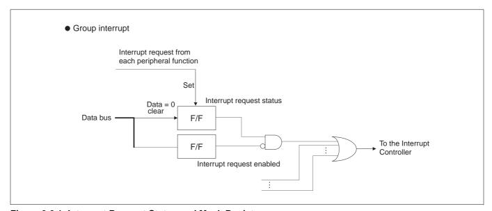
Figure 9.2.1 Interrupt Request Status and Mask Registers
