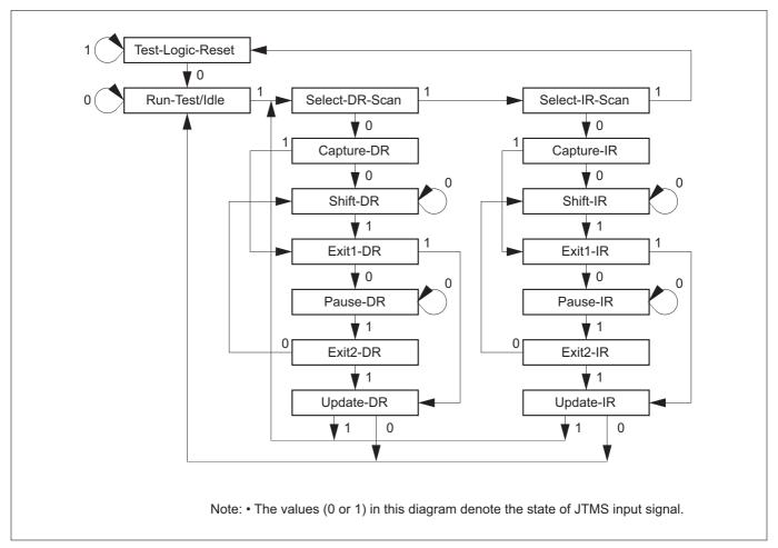
Figure 19.4.1 TAP Controller State Transition
