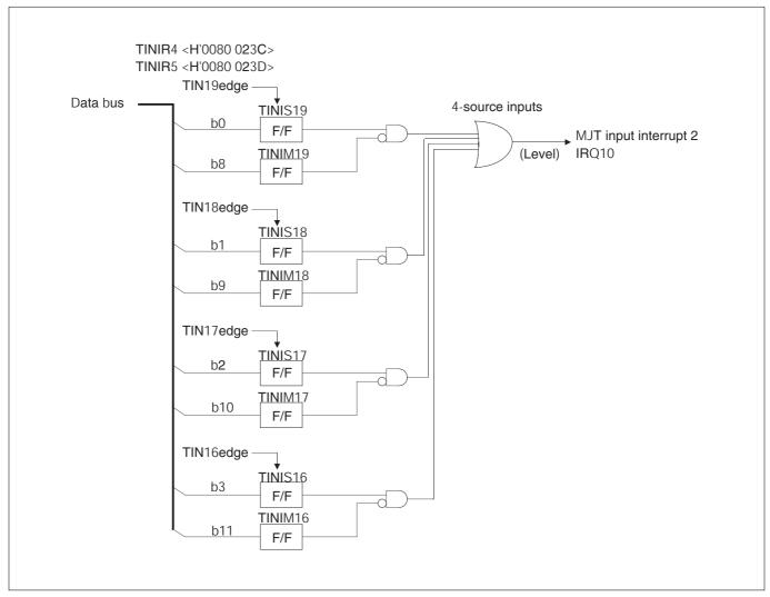
Figure 10.2.14 Block Diagram of MJT Input Interrupt 2
