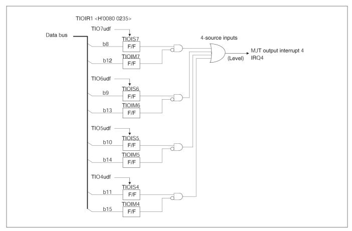
Figure 10.2.9 Block Diagram of MJT Output Interrupt 4
