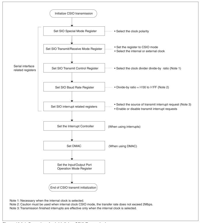
Figure 12.3.1 Procedure for Initializing CSIO Transmission
