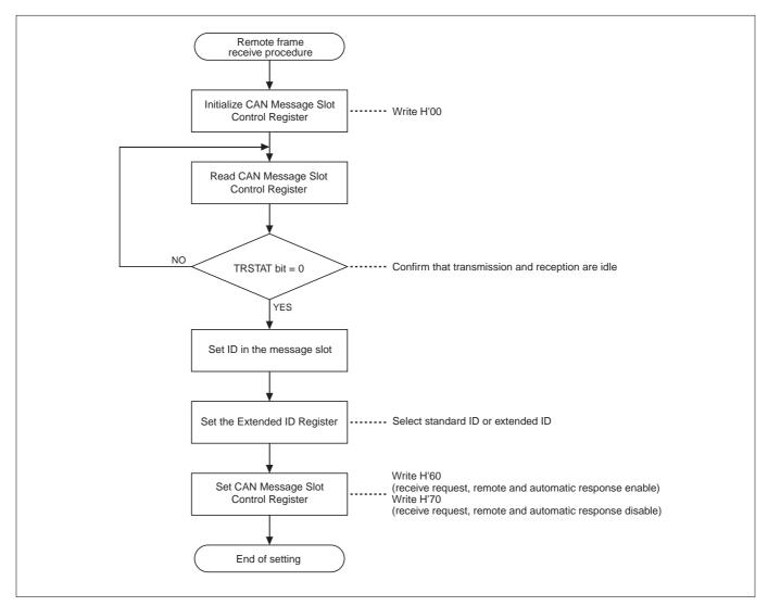
Figure 13.8.1 Remote Frame Receive Procedure
