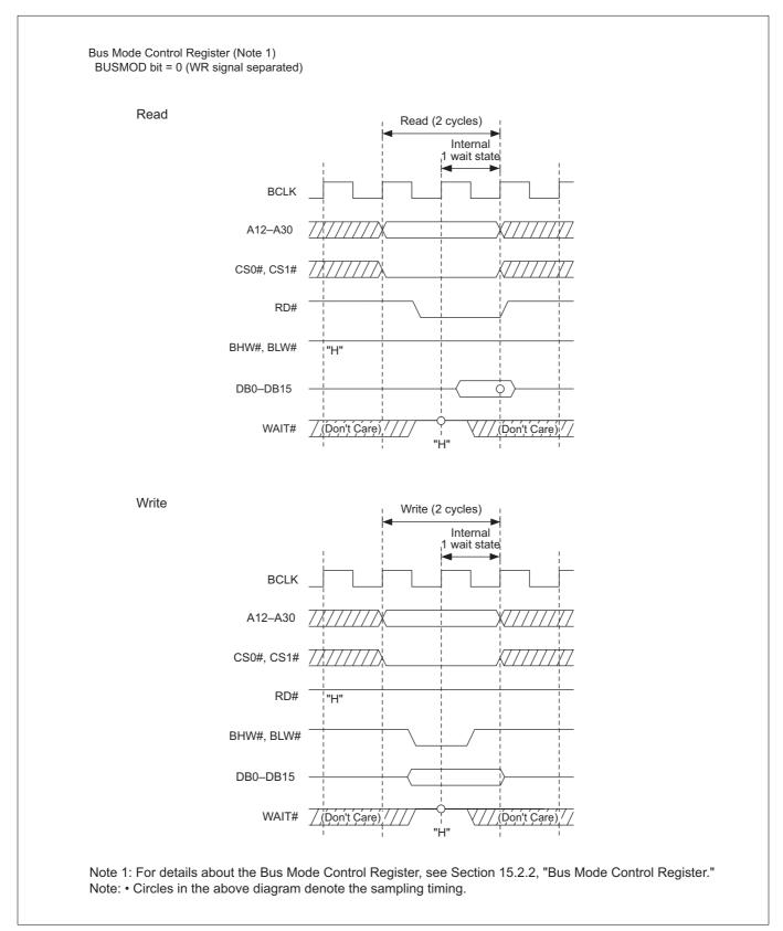
Figure 15.3.2 Read/Write Timing (for Shortest External Access)
