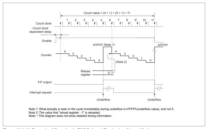
Figure 10.3.12 Example of Counting in TOP Delayed Single-shot Output Mode
