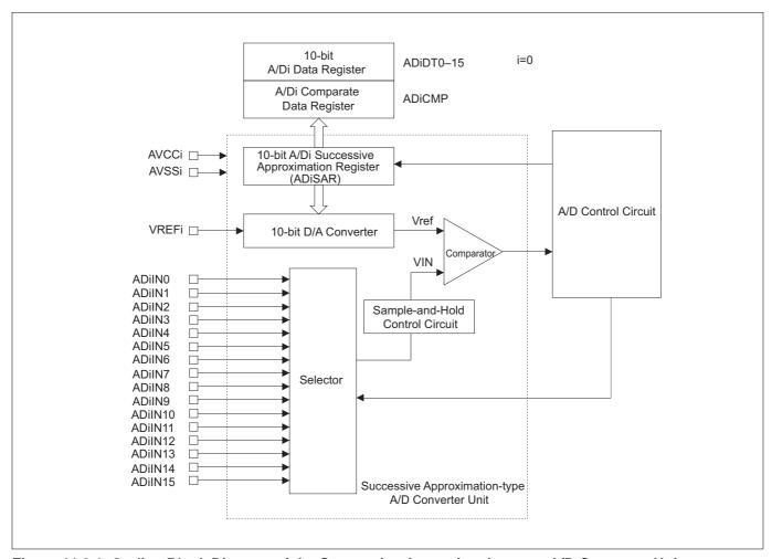
Figure 11.3.1 Outline Block Diagram of the Successive Approximation-type A/D Converter Unit
