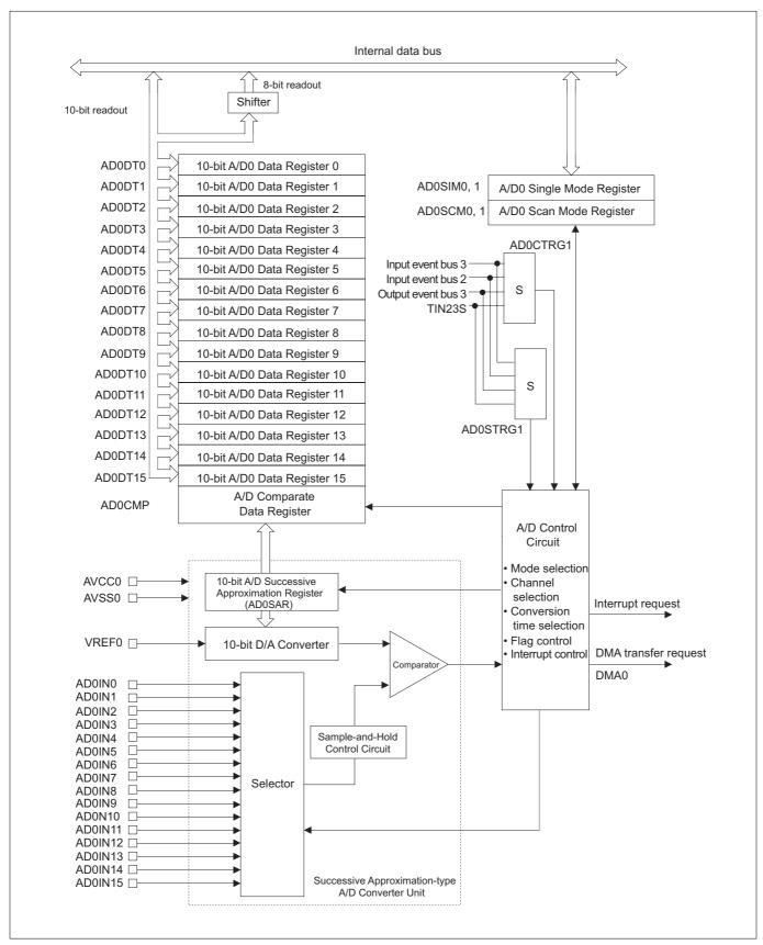
Figure 11.1.1 Block Diagram of the A/D0 Converter
