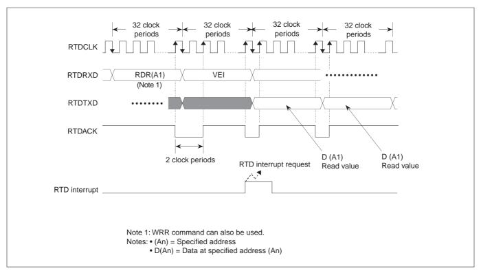
Figure 14.4.9 Operation of VEI (Interrupt Request) Command
