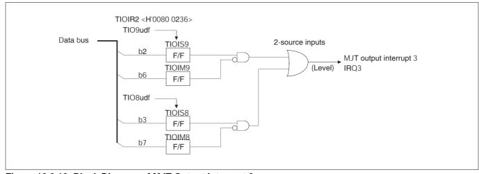
Figure 10.2.10 Block Diagram of MJT Output Interrupt 3
