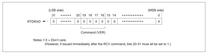
Figure 14.4.6 VER (Continuous Monitor) Command Data Format
