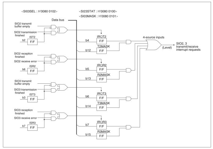
Figure 12.2.5 Block Diagram of SIO2,3 Transmit/Receive Interrupt Requests
