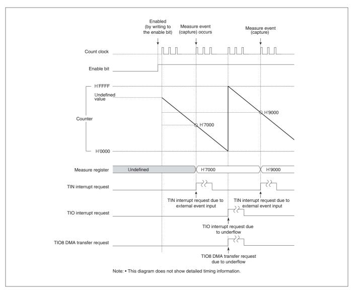
Figure 10.4.6 Typical Operation in Measure Free-Run Input Mode
