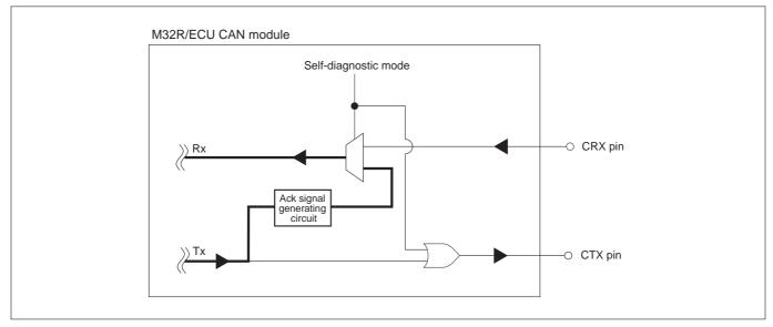
Figure 13.2.13 Conceptual Diagram of Self-Diagnostic Mode
