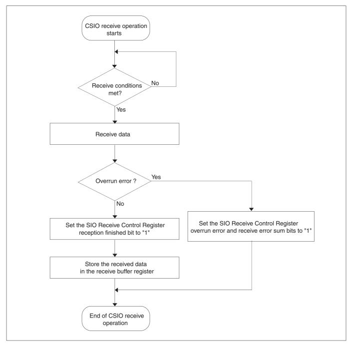
Figure 12.4.2 Receive Operation during CSIO Mode (Hardware Processing)
