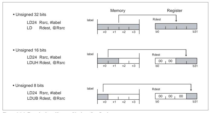
Figure 2.6.8 Transfer from Memory (Unsigned) to Registers
