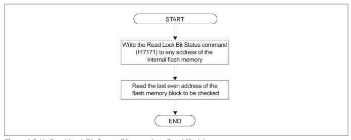
Figure 6.5.13 Read Lock Bit Status (Memory Area Read Mode)
