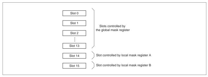
Figure 13.2.14 Relationship between the Mask Registers and the Controlled Slots
