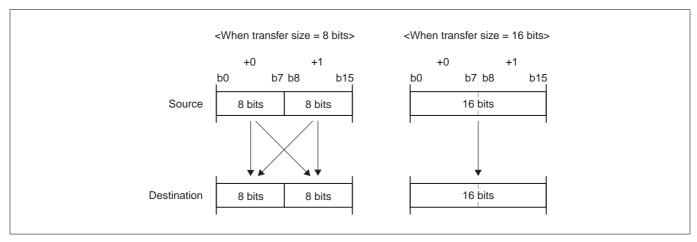
Figure 9.3.3 Transfer Byte Positions
