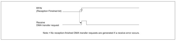
Figure 12.2.4 Reception-finished DMA Transfer Request
