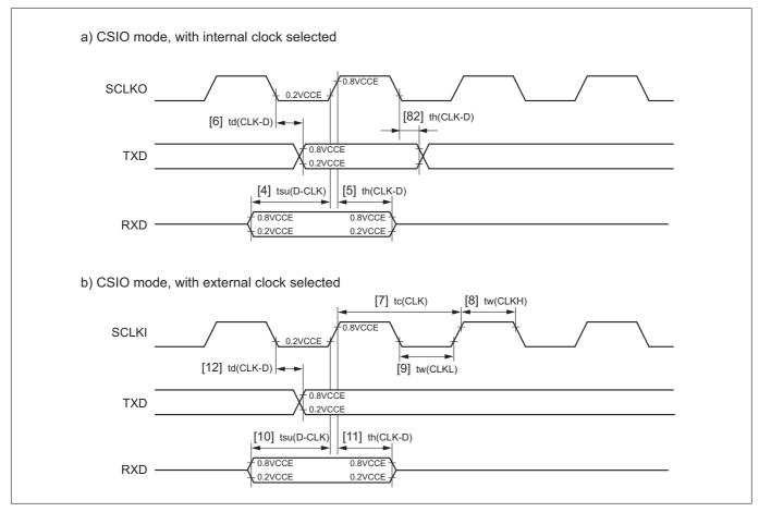
Figure 21.9.3 Serial Interface Timing
