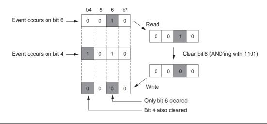
Figure 9.2.2 Example for Clearing Interrupt Request Status
