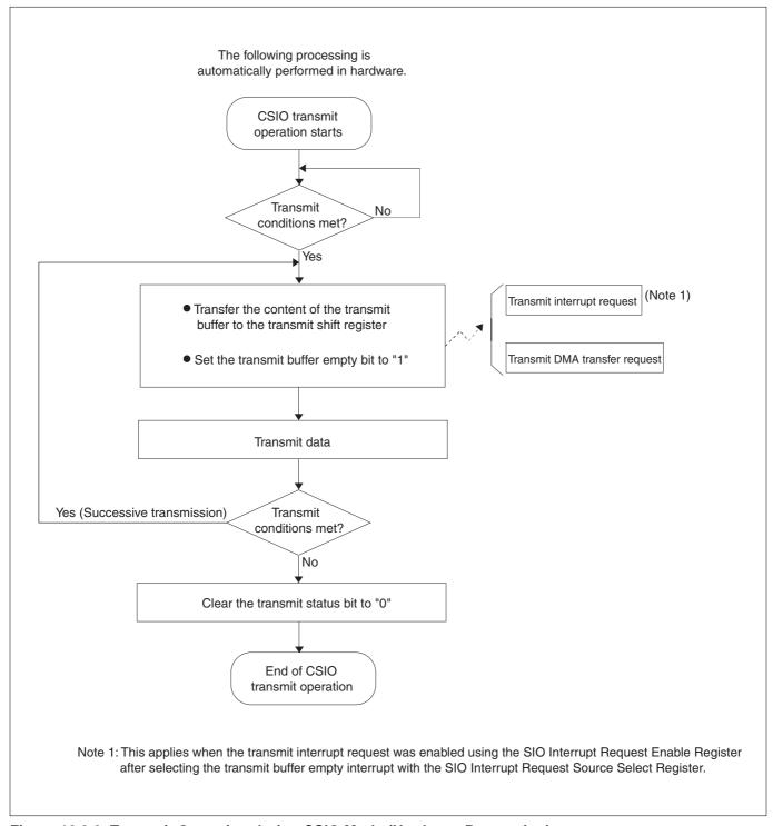
Figure 12.3.2 Transmit Operation during CSIO Mode (Hardware Processing)
