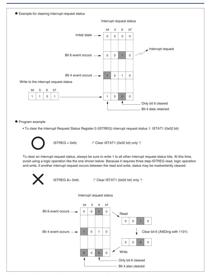
Figure 12.2.2 Example for Clearing Interrupt Request Status
