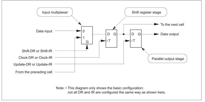
Figure 19.4.2 Basic Configuration of the JTAG Related Registers
