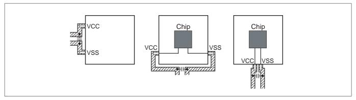
Appendix Figure 4.15.4 Example of a Bypass Capacitor Inserted between VSS and VCC Lines
