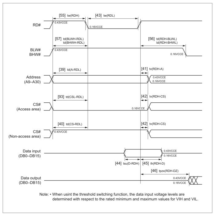
Figure 21.8.10 Read Timing (Relative to Read Pulse)
