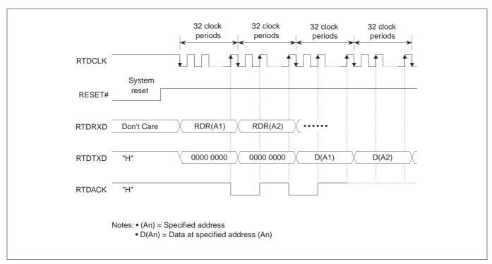
Figure 14.4.13 Command Transfer to RTD after System Reset
