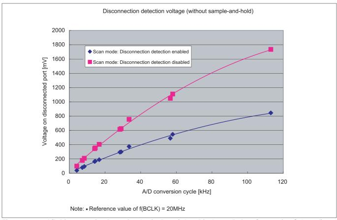
Figure 11.2.3 A/D Disconnection Detection Assist Data (when Discharge Before Conversion Selected)
