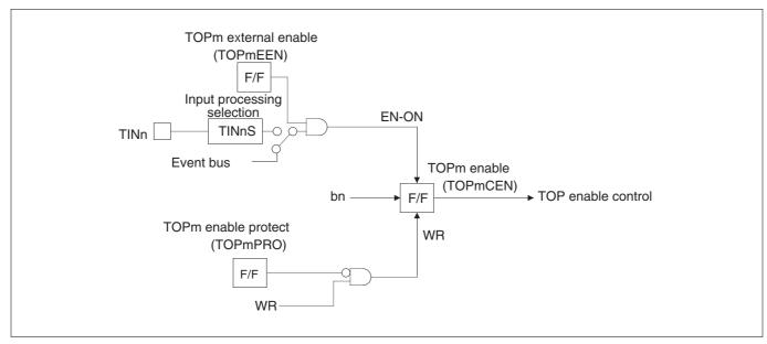
Figure 10.3.6 Configuration of the TOP Enable Circuit
