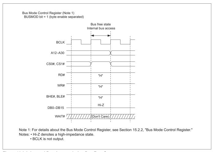
Figure 16.3.8 Internal Bus Access during Bus Free State
