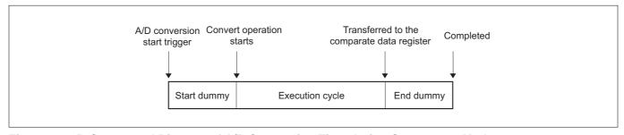
Figure 11.3.5 Conceptual Diagram of A/D Conversion Time during Comparator Mode
