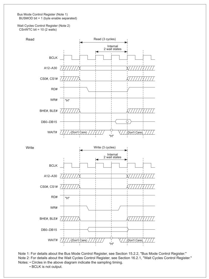
Figure 16.3.10 Read/Write Timing (for Access with Internal 2 Wait States)
