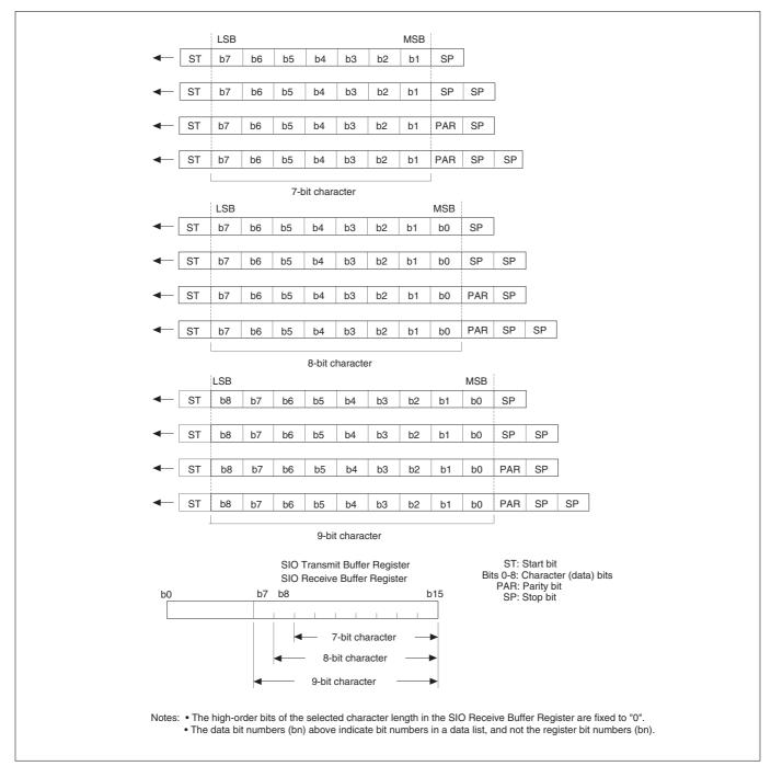
Figure 12.6.2 Selectable Data Formats during UART Mode
