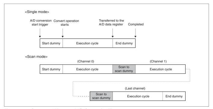
Figure 11.3.3 Conceptual Diagram of A/D Conversion Time
