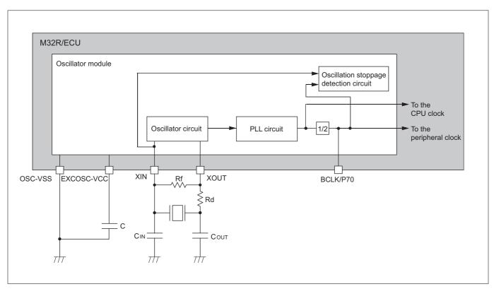
Figure 18.1.1 Example of an Oscillator Circuit
