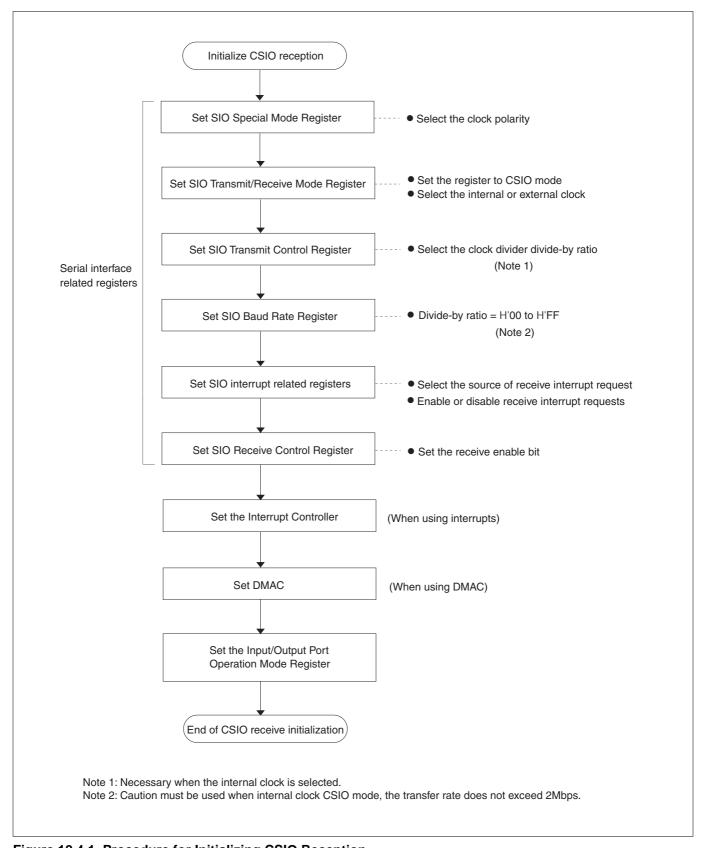
Figure 12.4.1 Procedure for Initializing CSIO Reception
