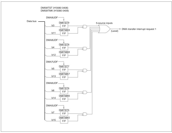
Figure 9.2.4 Block Diagram of DMA Transfer Interrupt Request 1
