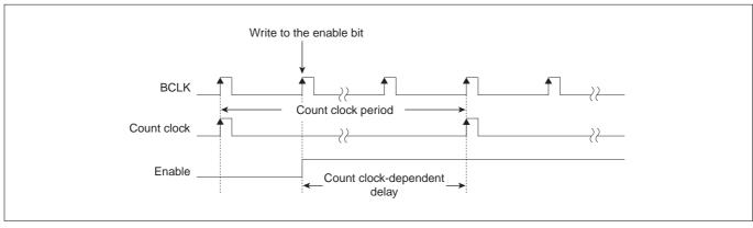
Figure 10.5.2 Count Clock-Dependent Delay
