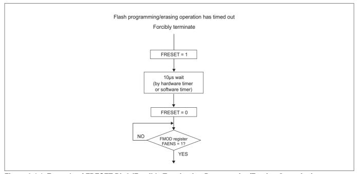
Figure 6.4.4 Example of FRESET Bit 2 (Forcibly Terminating Programming/Erasing Operation)
