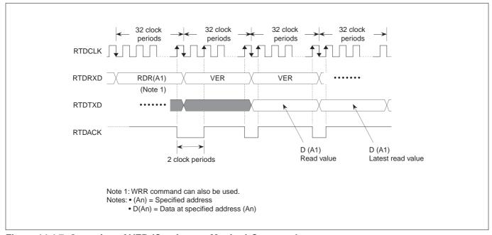
Figure 14.4.7 Operation of VER (Continuous Monitor) Command
