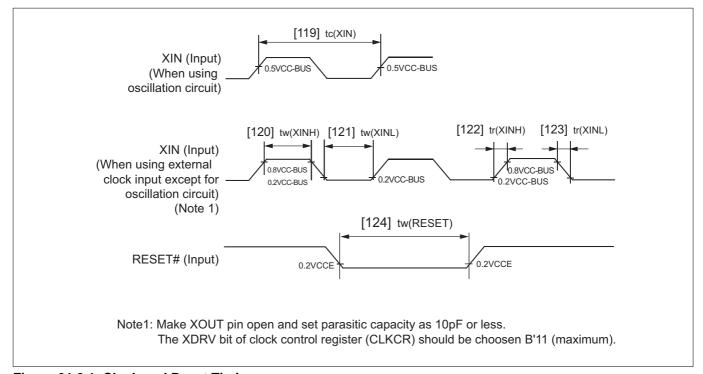
Figure 21.8.1 Clock and Reset Timing
