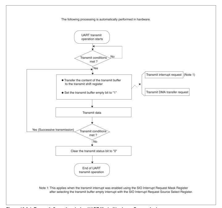
Figure 12.6.4 Transmit Operation during UART Mode (Hardware Processing)
