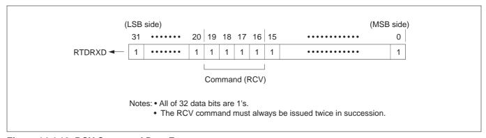
Figure 14.4.10 RCV Command Data Format
