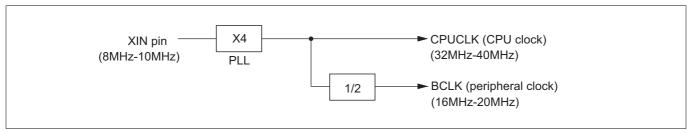
Figure 1.1.1 Conceptual Diagram of the Clock Frequency Multiplier
