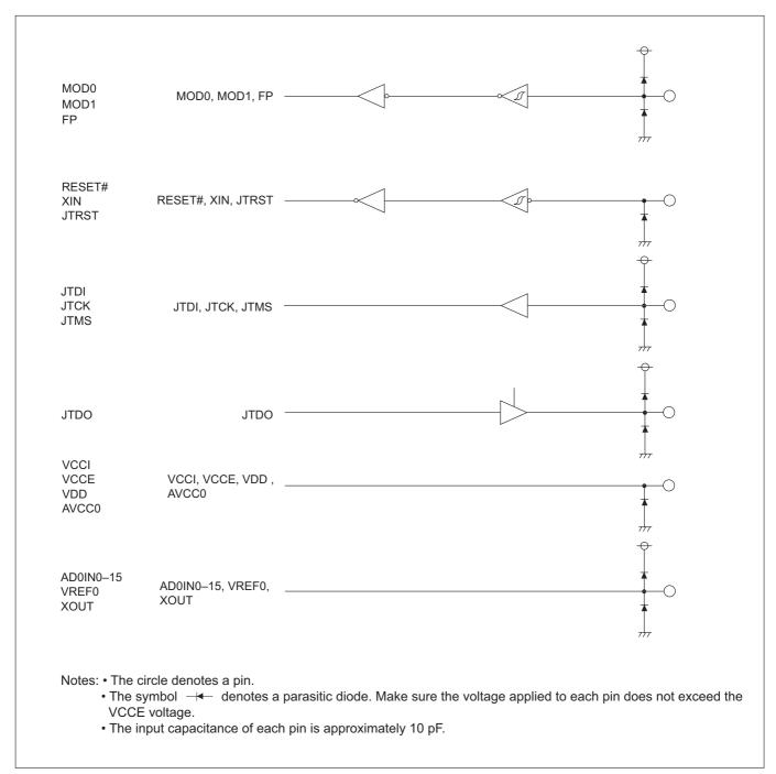
Figure 8.5.5 Port Peripheral Circuit Diagram (5)
