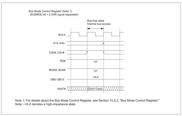
Figure 15.3.1 Internal Bus Access during Bus Free State
