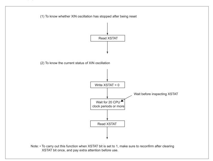
Figure 18.1.3 Procedure for Setting XSTAT
