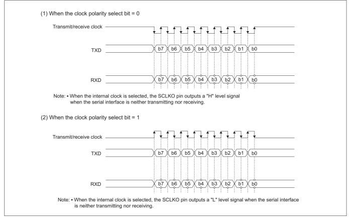
Figure 12.2.7 Selecting the Transmit/receive Clock Polarity
