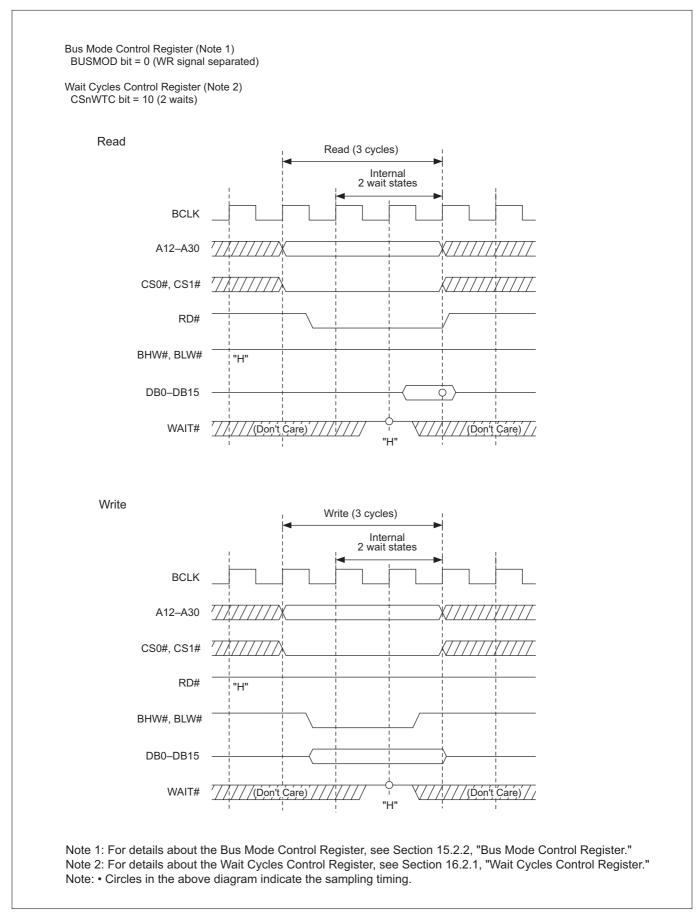
Figure 16.3.3 Read/Write Timing (for Access with Internal 2 Wait States)
