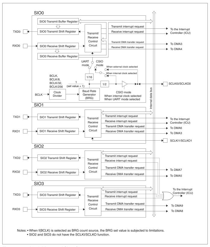
Figure 12.1.1 Block Diagram of SIO0-SIO3
