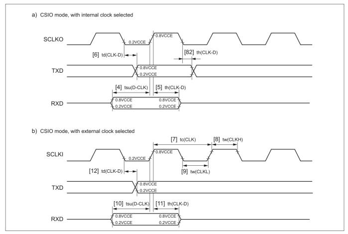
Figure 21.8.3 Serial Interface Timing
