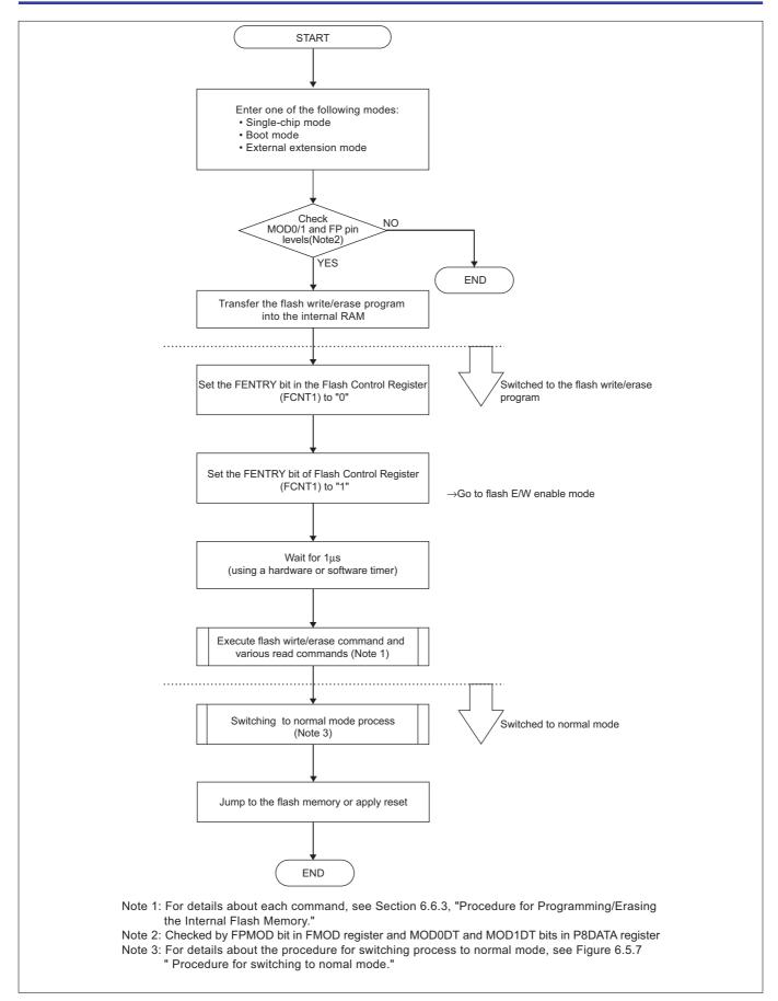
Figure 6.5.6 Procedure for Entering Flash E/W Enable Mode
