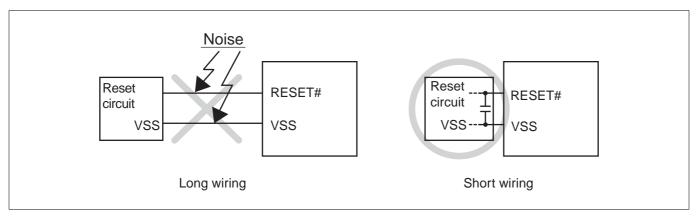
Appendix Figure 4.15.1 Example Wiring of the RESET# Pin
