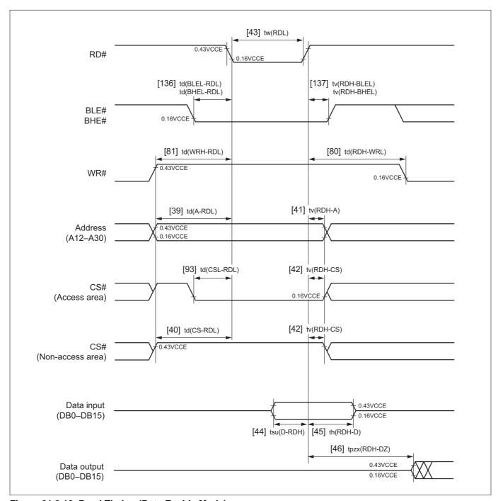
Figure 21.8.12 Read Timing (Byte Enable Mode)
