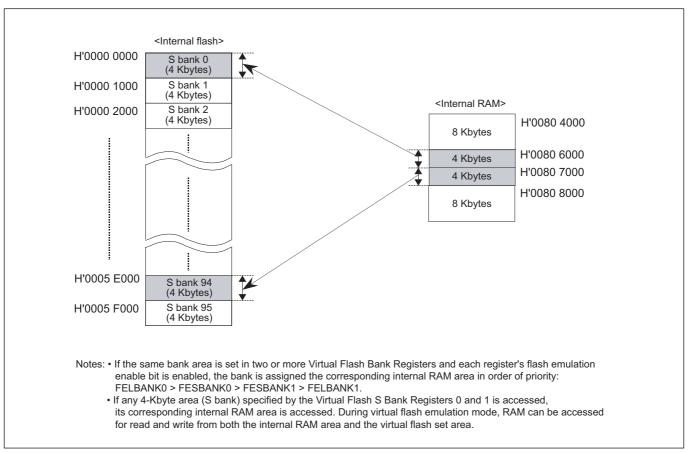
Figure 6.6.5 M32176F3 Virtual Flash Emulation Area divided in 4-Kbyte units
