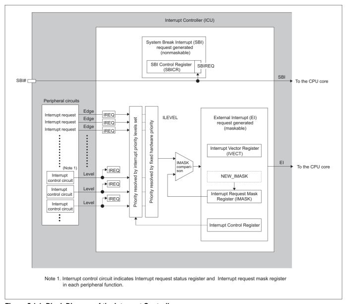
Figure 5.1.1 Block Diagram of the Interrupt Controller
