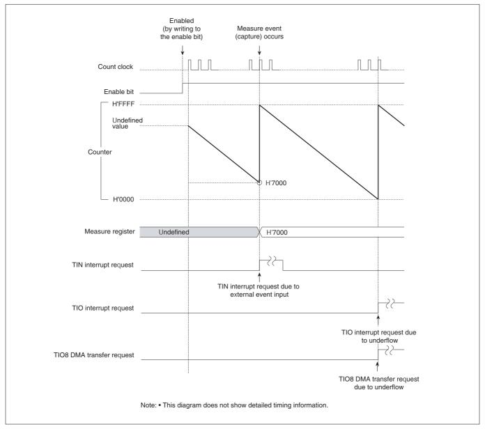
Figure 10.4.7 Typical Operation in Measure Clear Input Mode
