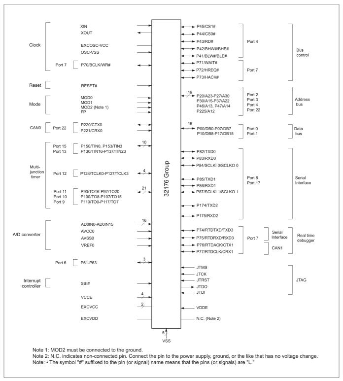
Figure 1.3.1 Pin Function Diagram
