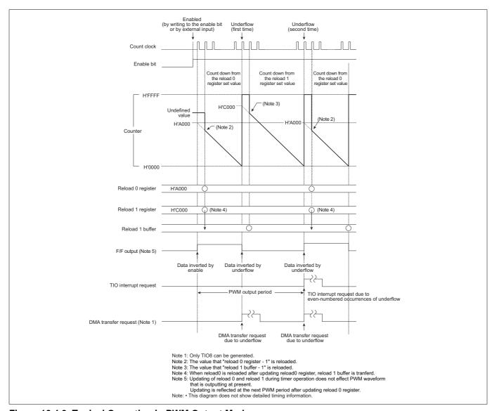
Figure 10.4.9 Typical Operation in PWM Output Mode
