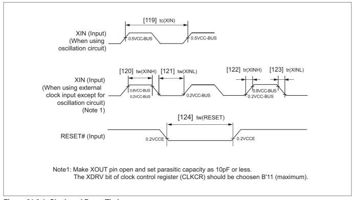
Figure 21.9.1 Clock and Reset Timing
