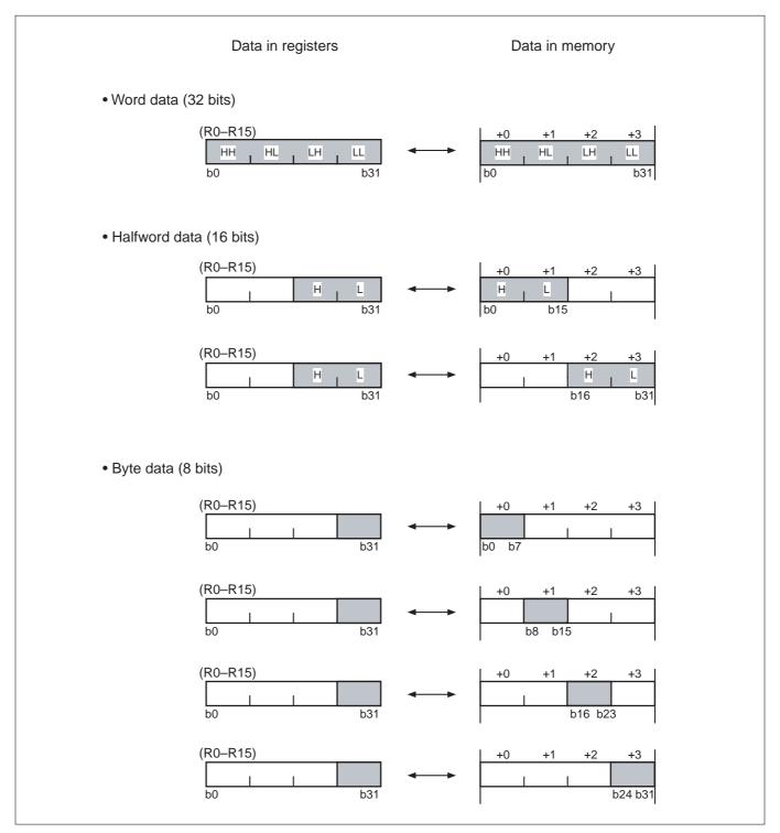
Figure 2.6.9 Difference in Data Arrangements
