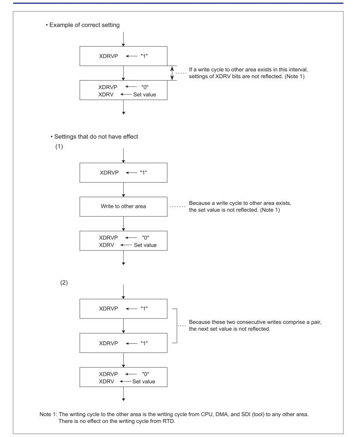
Figure 18.1.4 Procedure for Setting the Oscillation Drive Capability
