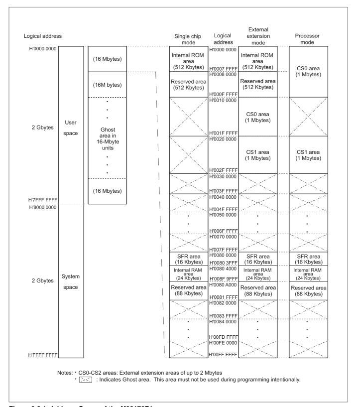
Figure 3.2.1 Address Space of the M32176F4
