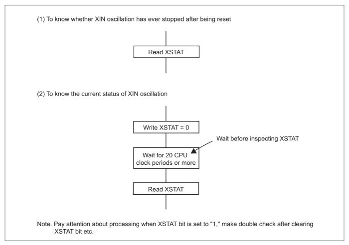
Figure 8.3.1 Procedure for Setting XSTAT
