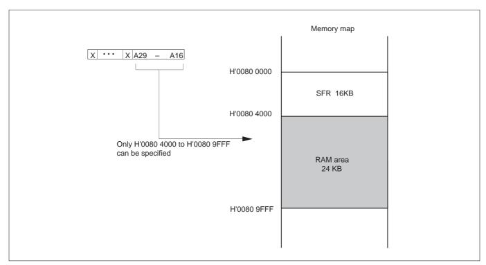
Figure 14.4.12 Setting Addresses in the Real-Time Debugger
