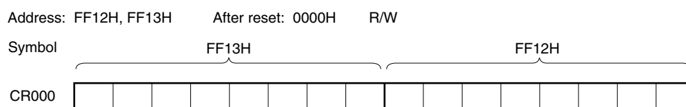
Figure 6-3. Format of 16-Bit Timer Capture/Compare Register 000 (CR000)
