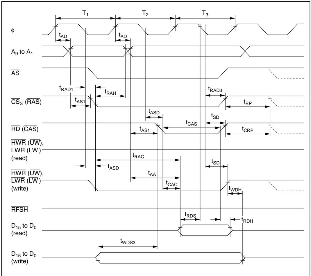
Figure 21.7 DRAM Bus Timing (Read/Write): Three-State Access
