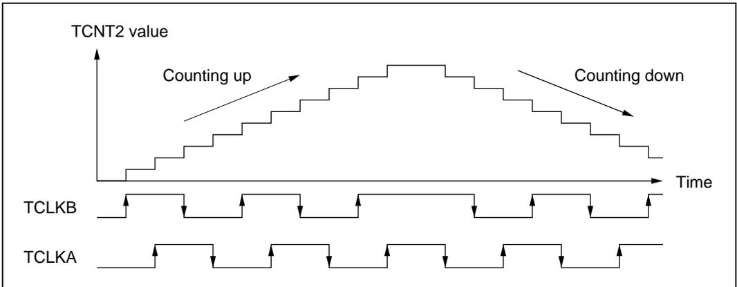
**Figure 10.44 Operation in Phase Counting Mode (Example)**
