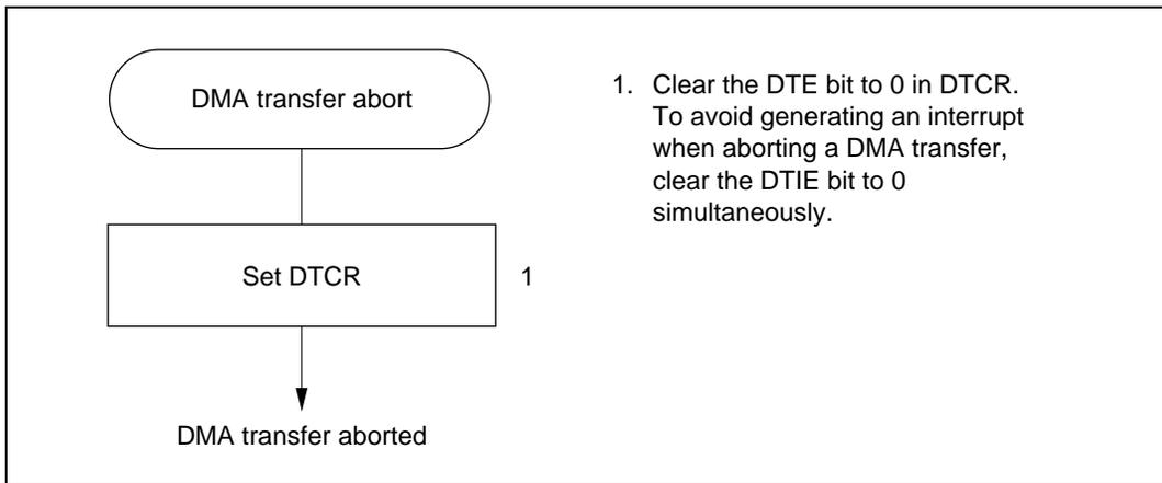
**Figure 8.22 Procedure for Aborting a DMA Transfer**
