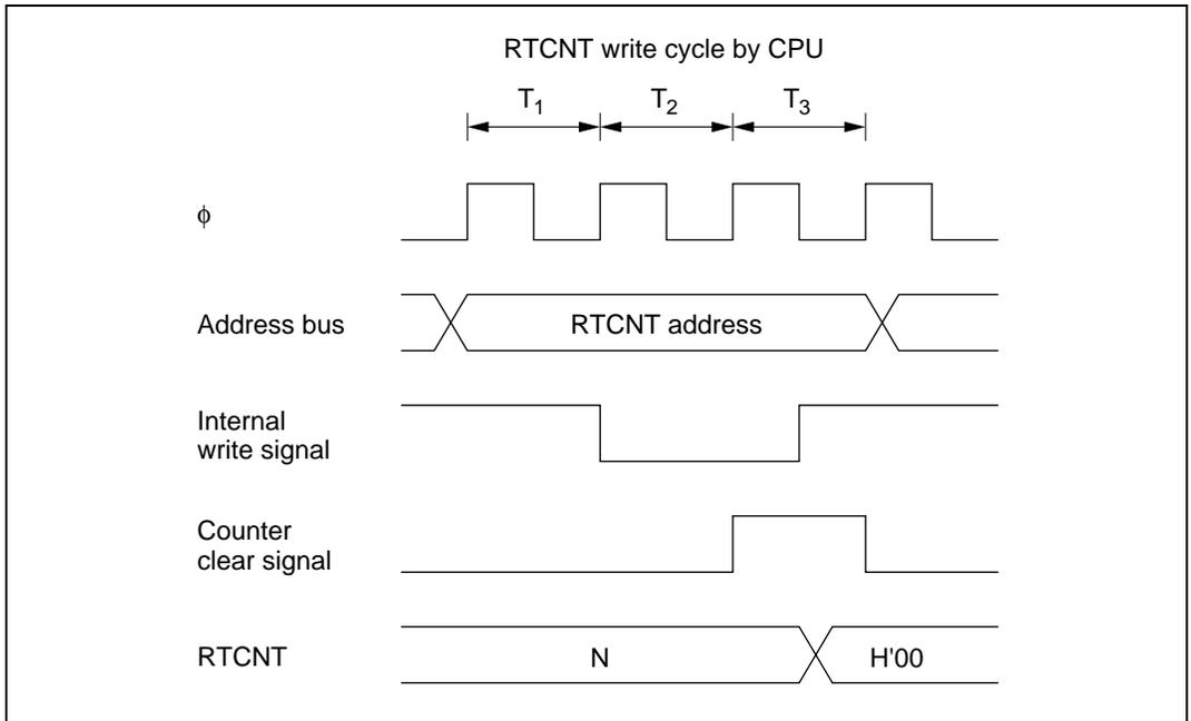
**Figure 7.20 Contention between RTCNT Write and Clear**
