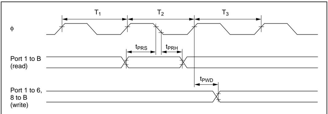
Figure 21.19 TPC and I/O Port Input/Output Timing
