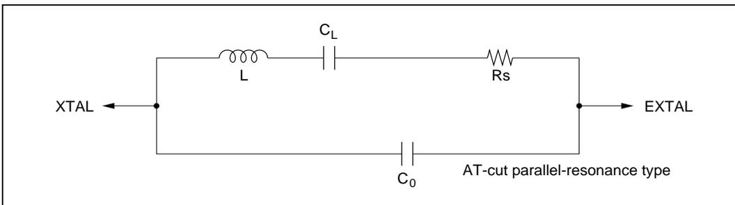
**Figure 19.3 Crystal Resonator Equivalent Circuit****Table 19.2 Crystal Resonator Parameters**
