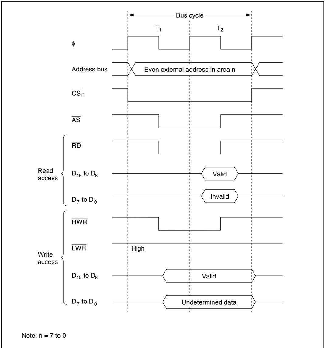
**Figure 6.9 Bus Control Signal Timing for 16-Bit, Two-State-Access Area (1)**
