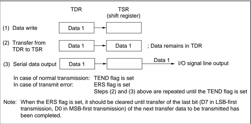
**Figure 14.5 Relation between Transmit Operation and Internal Registers**
