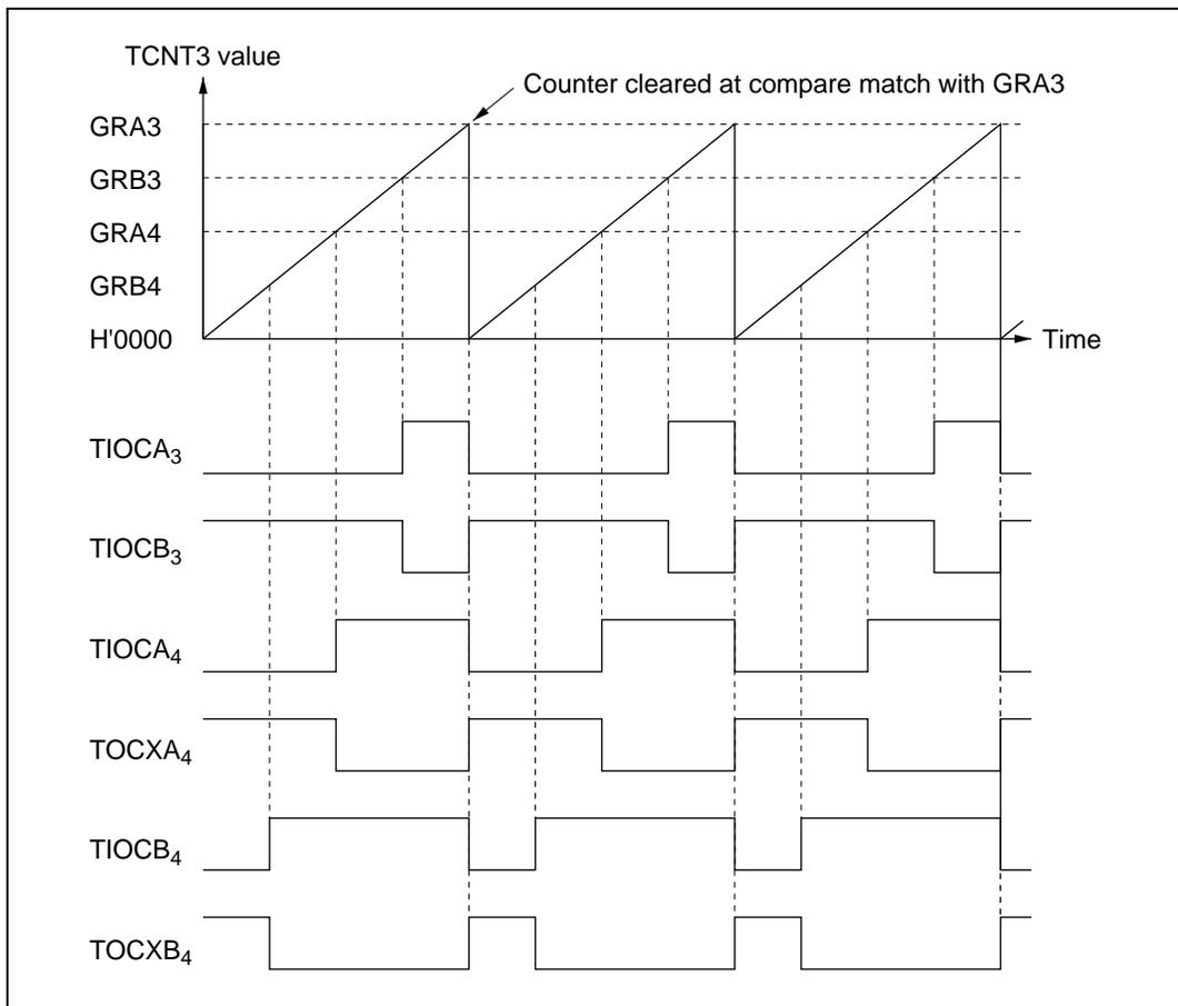
**Figure 10.32 Operation in Reset-Synchronized PWM Mode (Example)**
