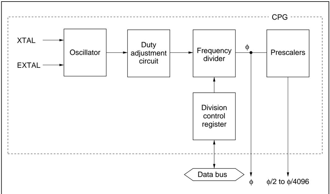
**Figure 19.1 Block Diagram of Clock Pulse Generator**
