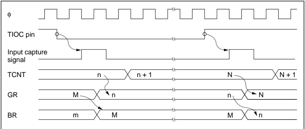
**Figure 10.52 Input Capture and Buffer Transfer Timing**
