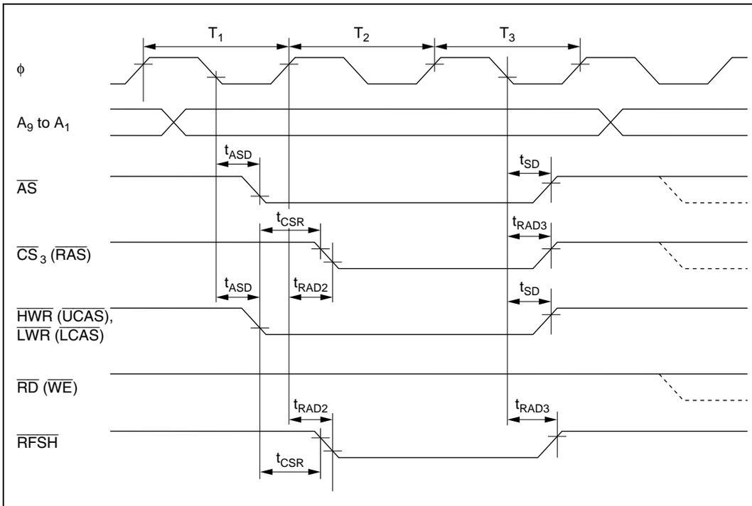
**Figure 21.11 DRAM Bus Timing (Refresh Cycle): Three-State Access**
