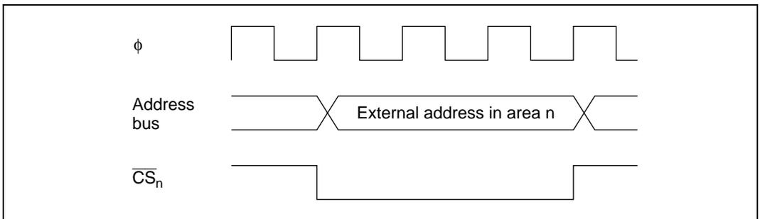
**Figure 6.3  $\overline{CS}_n$  Output Timing ( $n = 7$  to  $0$ )**
