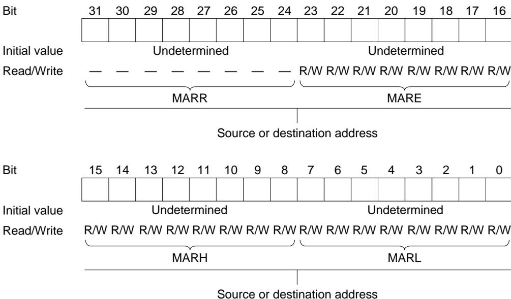
An MAR functions as a source or destination address register depending on how the DMAC is activated: as a destination address register if activation is by a receive-data-full interrupt from the serial communication interface (SCI) (channel 0), and as a source address register otherwise.
