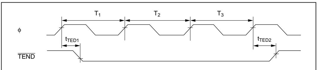
Figure 21.25 DMAC  $\overline{\text{TEND}}$  Output Timing for 3 State Access
