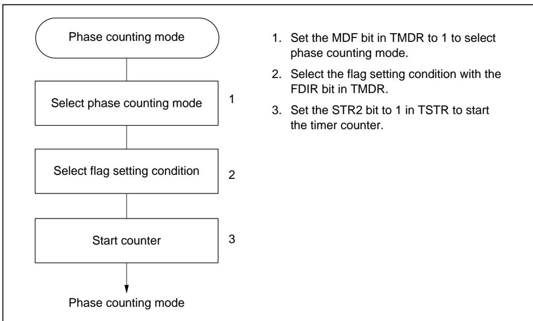
**Figure 10.43 Setup Procedure for Phase Counting Mode (Example)**
