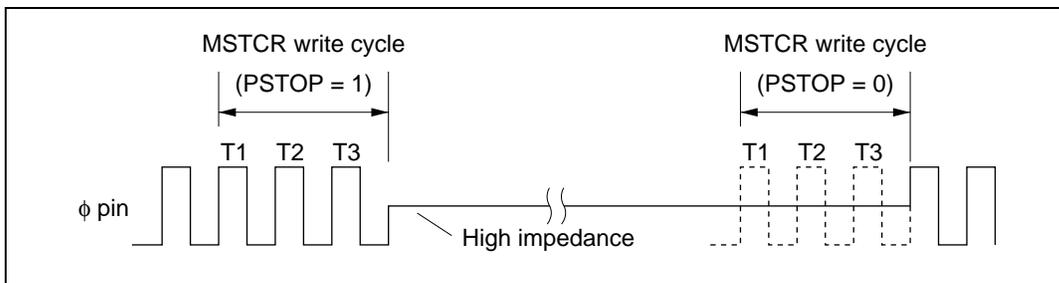
**Figure 20.3 Starting and Stopping of System Clock Output**
