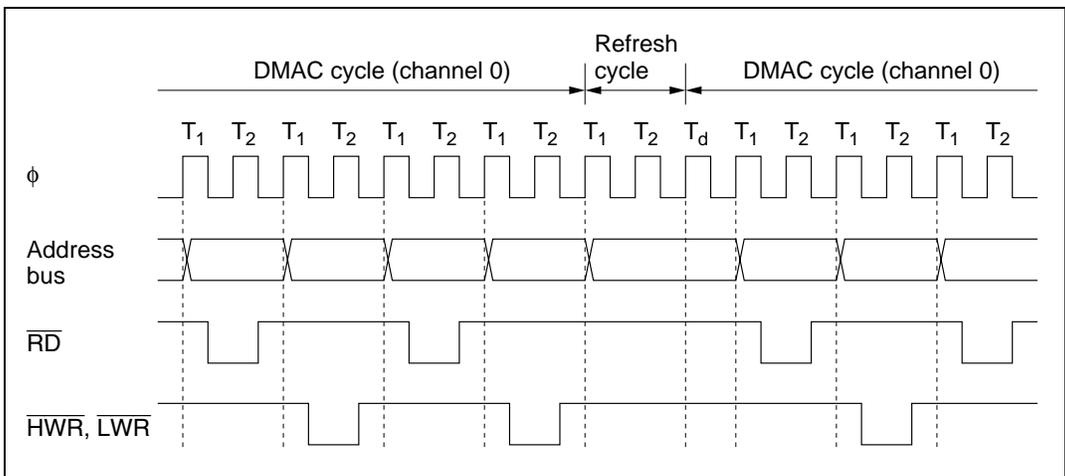
**Figure 8.20 Bus Timing of Refresh Controller and DMAC**
