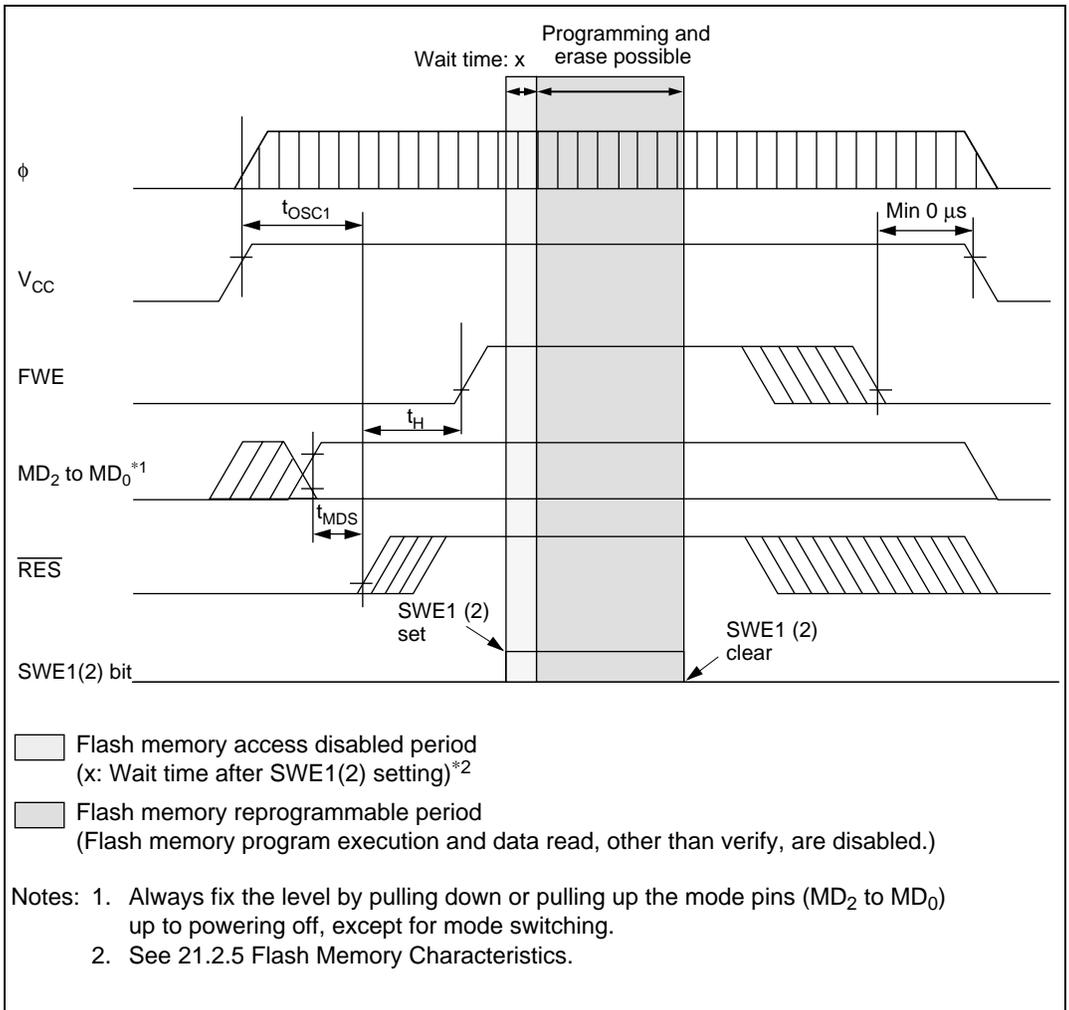
**Figure 18.19 Powering On/Off Timing (User Program Mode)**
