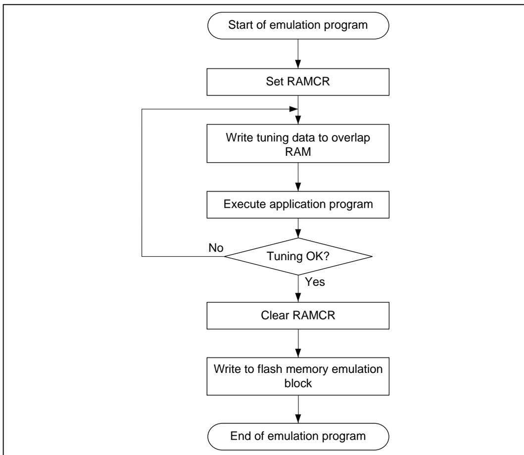
Figure 18.15 Flowchart for Flash Memory Emulation in RAM
