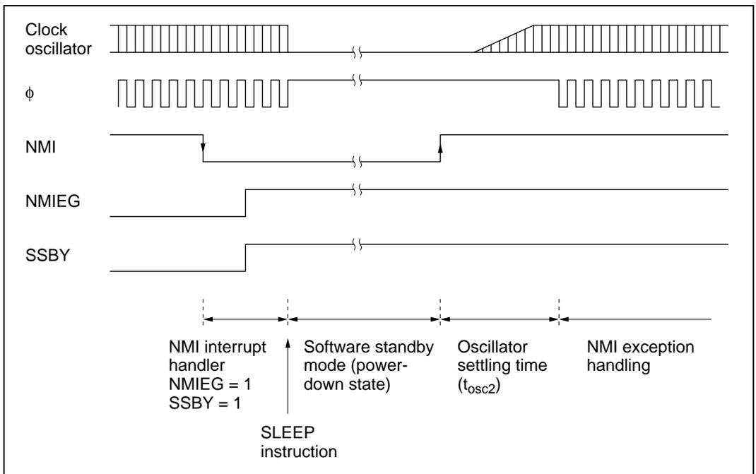
**Figure 20.1 NMI Timing for Software Standby Mode (Example)**
