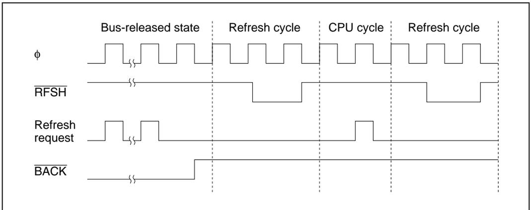
**Figure 7.24 Refresh Cycles when Bus Is Released**
