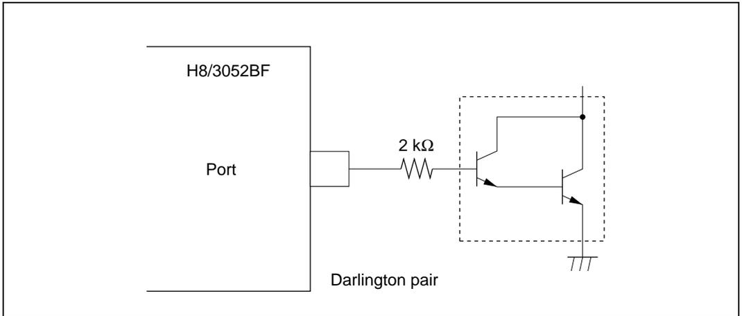
**Figure 21.1 Darlington Pair Drive Circuit (Example)**
