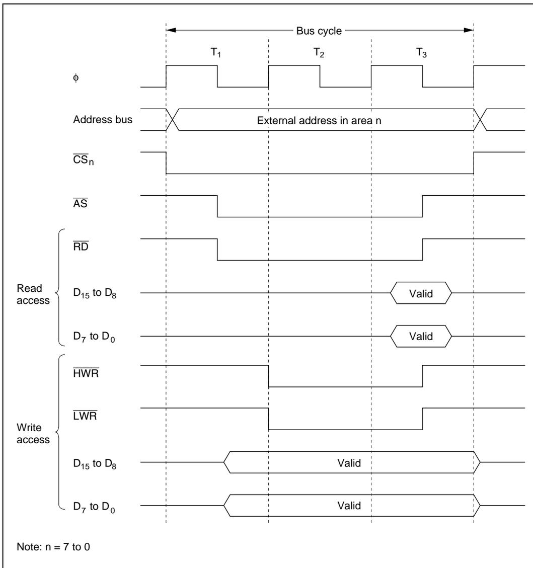
**Figure 6.8 Bus Control Signal Timing for 16-Bit, Three-State-Access Area (3)
