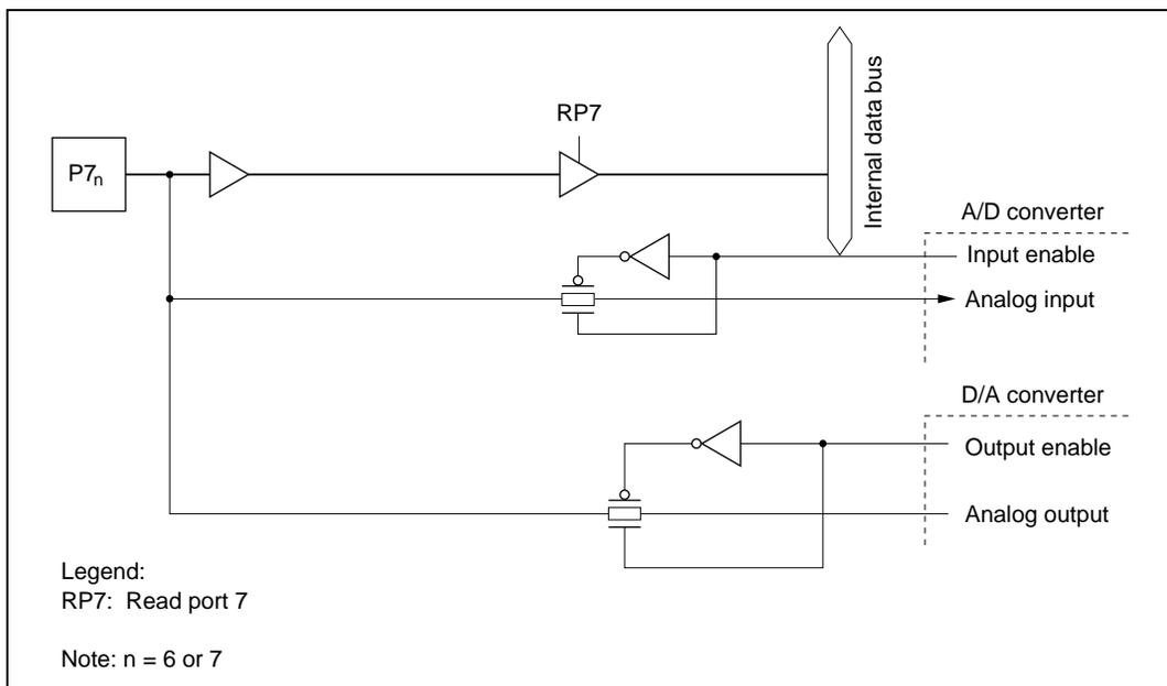
Figure C.7 (b) Port 7 Block Diagram (Pins P7<sub>6</sub>, P7<sub>7</sub>)
