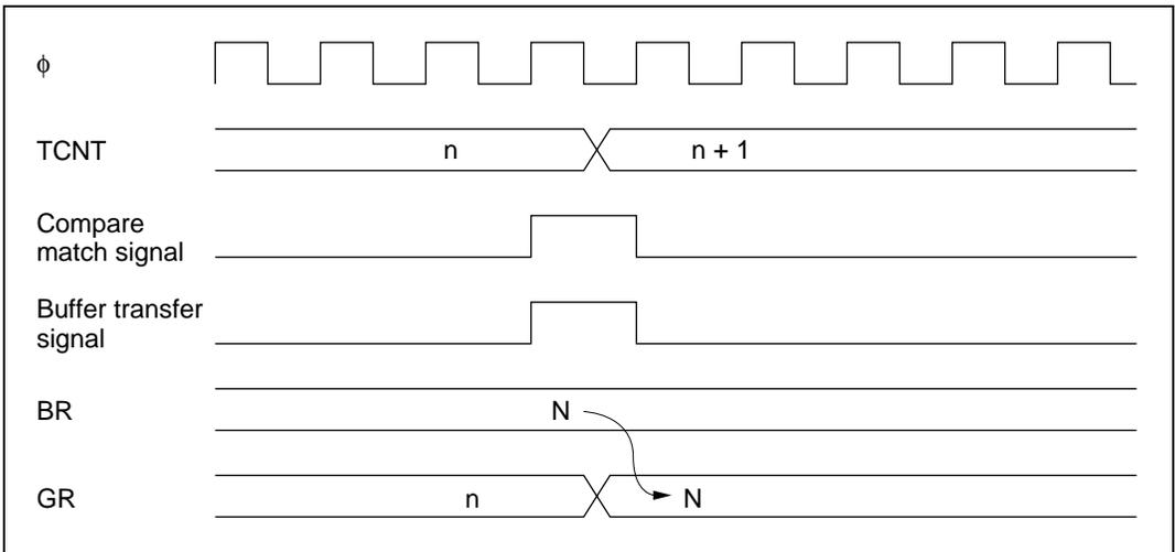
**Figure 10.50 Compare Match and Buffer Transfer Timing (Example)**
