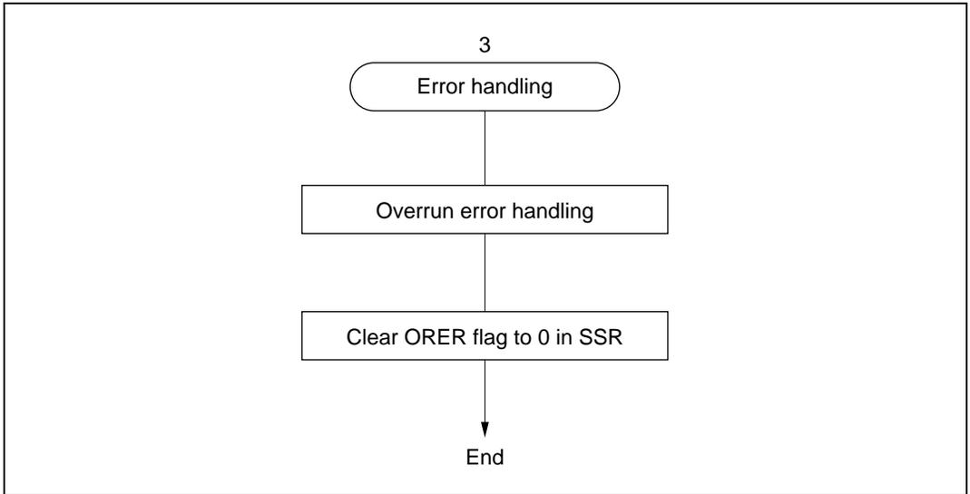
**Figure 13.18 Sample Flowchart for Serial Receiving (2)**
