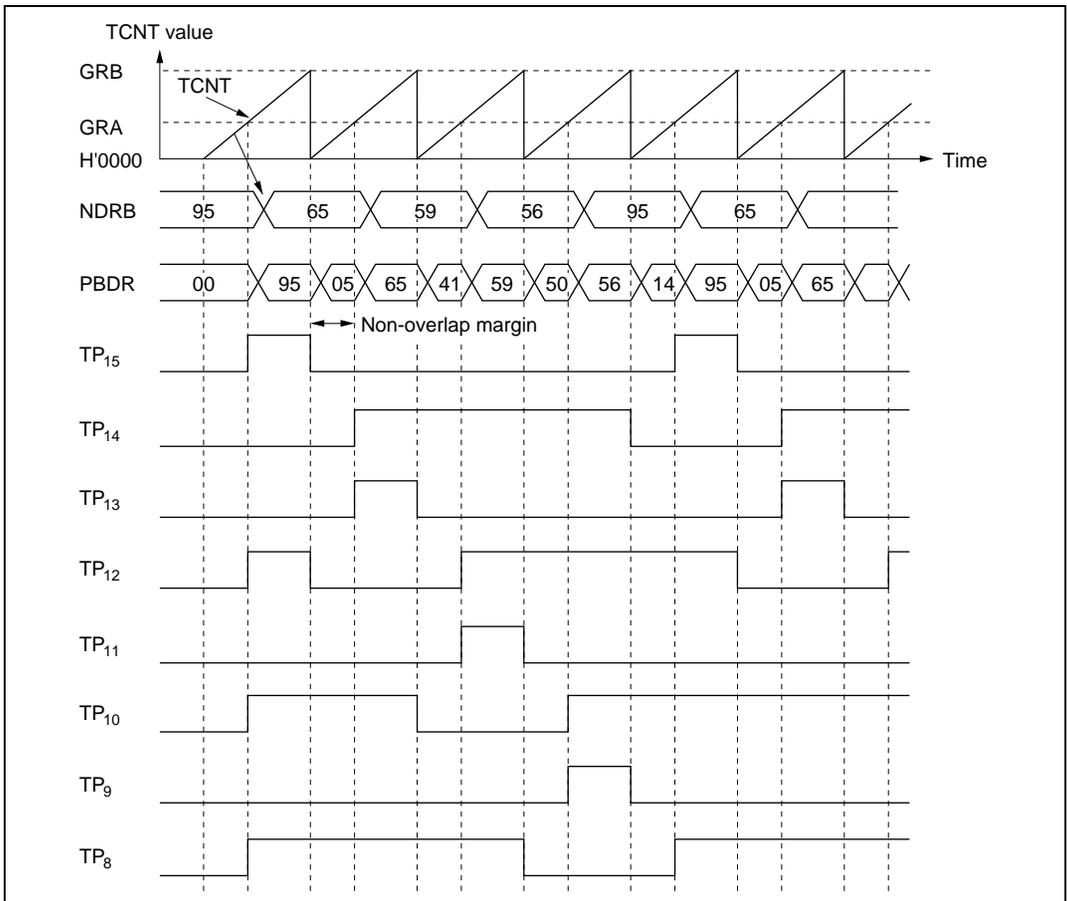
**Figure 11.7 Non-Overlapping TPC Output Example
