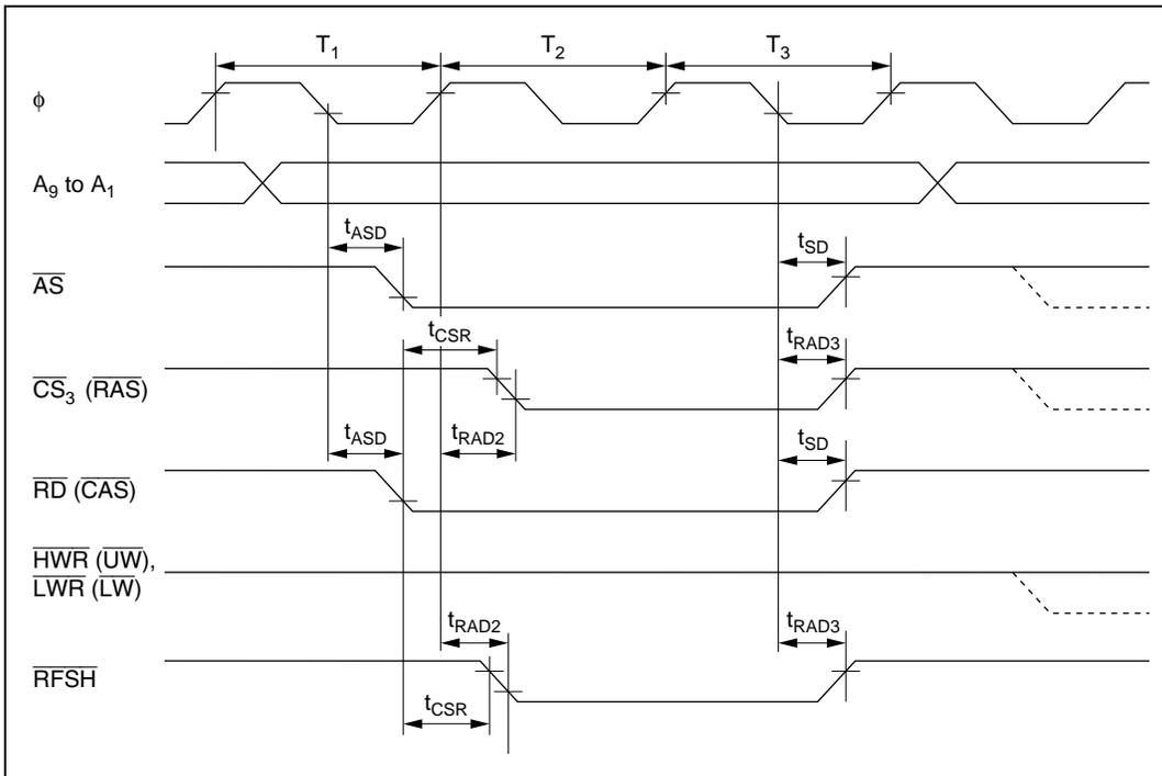
**Figure 21.8 DRAM Bus Timing (Refresh Cycle): Three-State Access**
