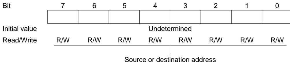
An IOAR functions as a source or destination address register depending on how the DMAC is activated: as a source address register if activation is by a receive-data-full interrupt from the SCI (channel 0), and as a destination address register otherwise.
