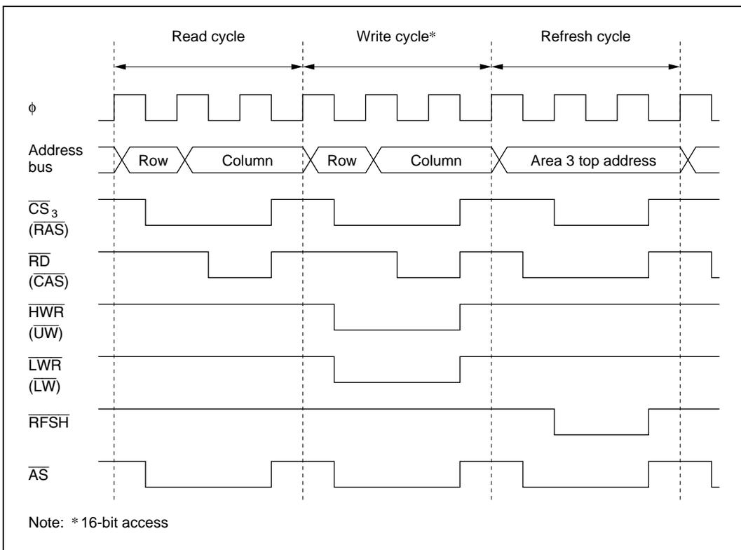
**Figure 7.5 DRAM Control Signal Output Timing (1) ( $2\overline{\text{WE}}$  Mode)**
