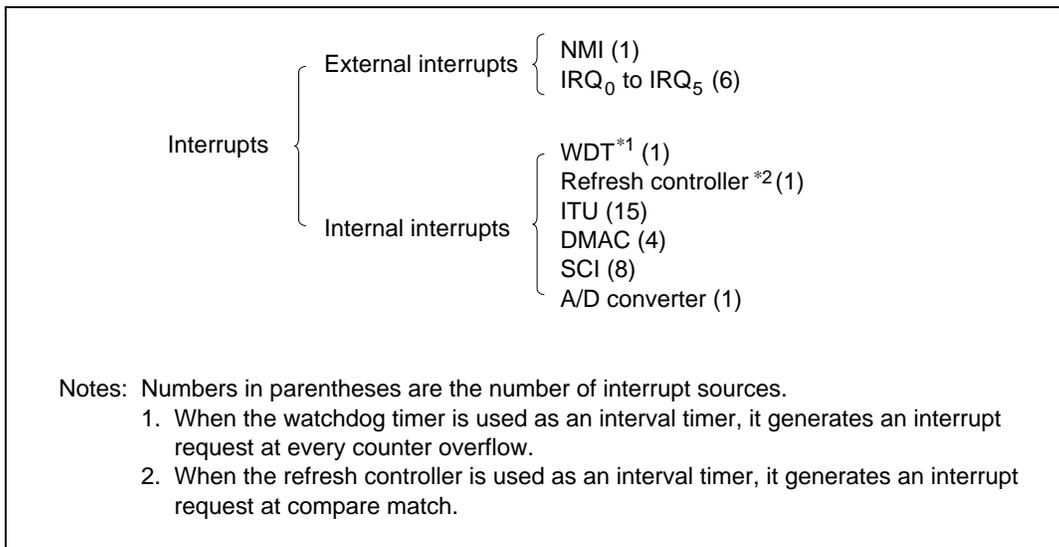
**Figure 4.5 Interrupt Sources and Number of Interrupts**
