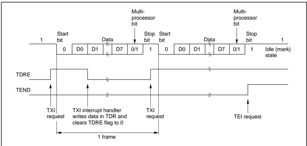
**Figure 13.11 Example of SCI Transmit Operation
