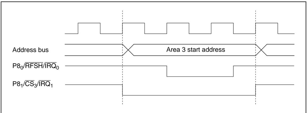
**Figure 7.23 Operation when DRAM/PSRAM Connection Is Switched**
