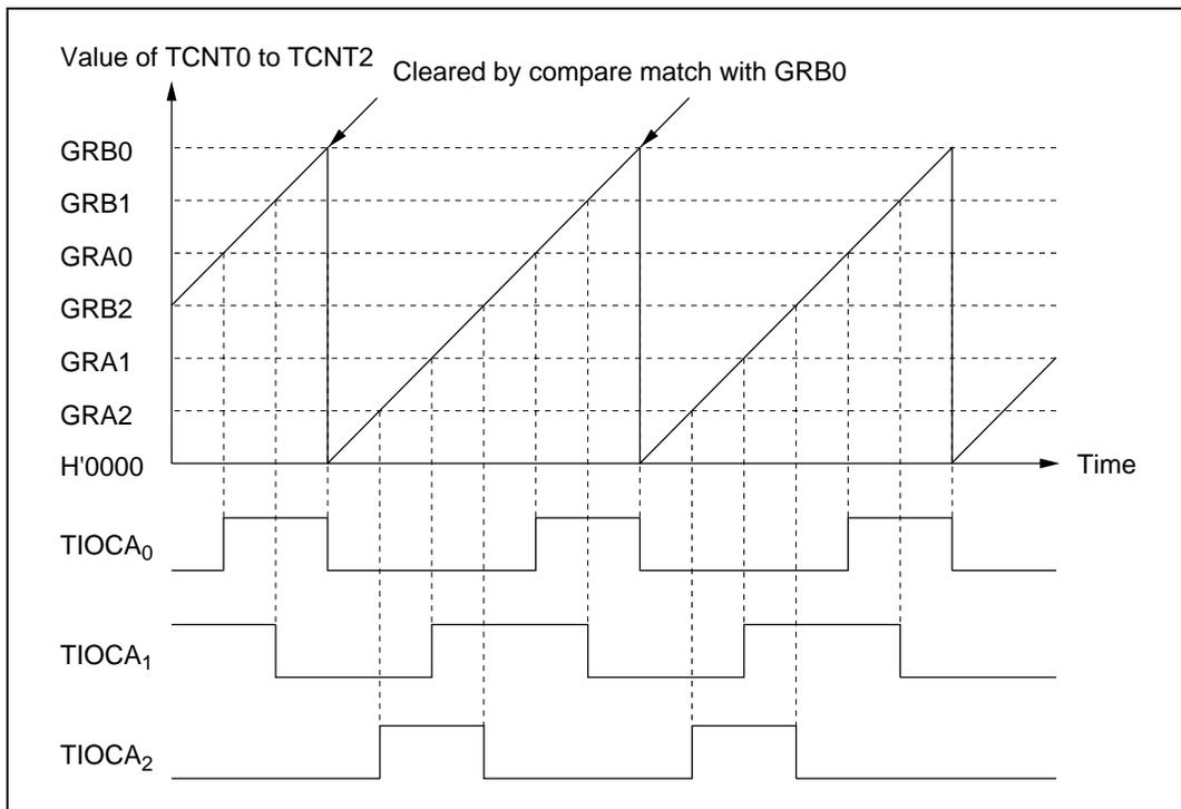
**Figure 10.27 Synchronization (Example)**
