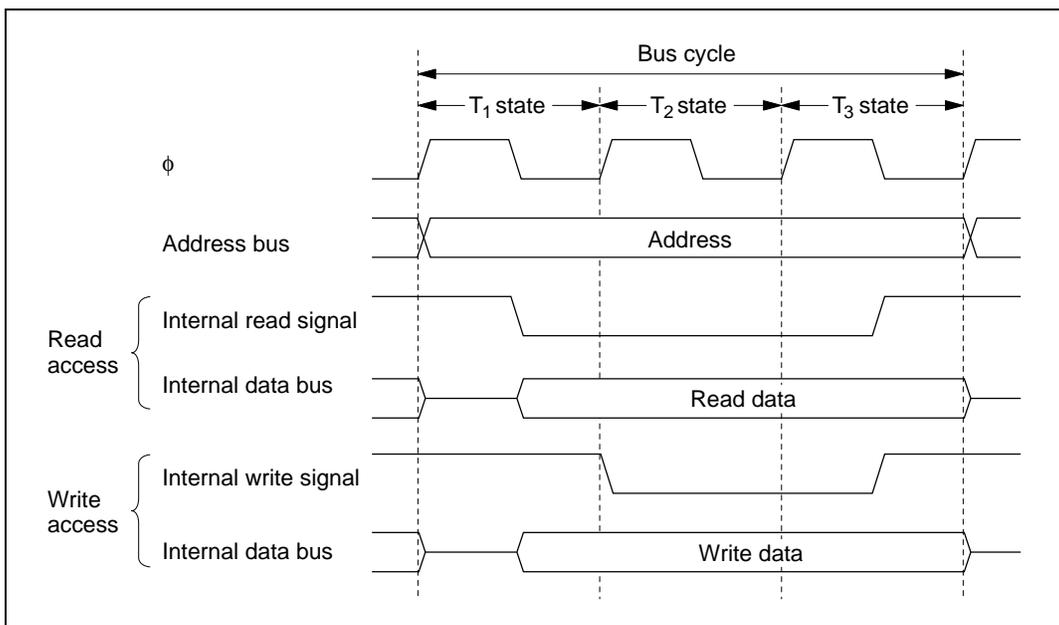
**Figure 2.16 Access Cycle for On-Chip Supporting Modules**
