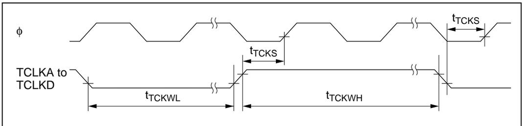
**Figure 21.21 ITU External Clock Input Timing**
