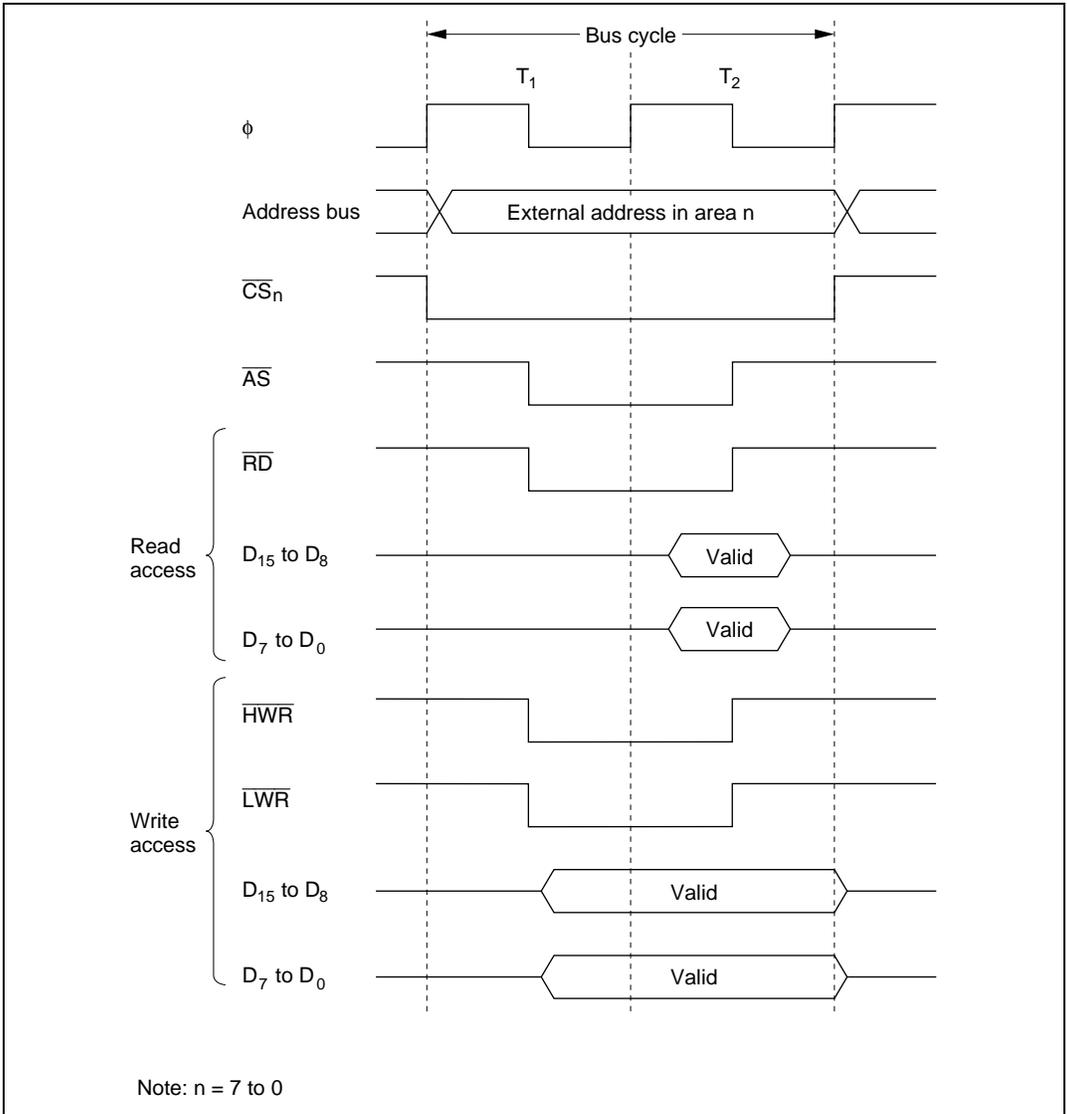
**Figure 6.11 Bus Control Signal Timing for 16-Bit, Two-State-Access Area (3)
