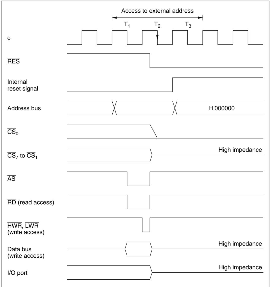
**Figure D.2 Reset during Memory Access (Reset during T<sub>2</sub> State)**
