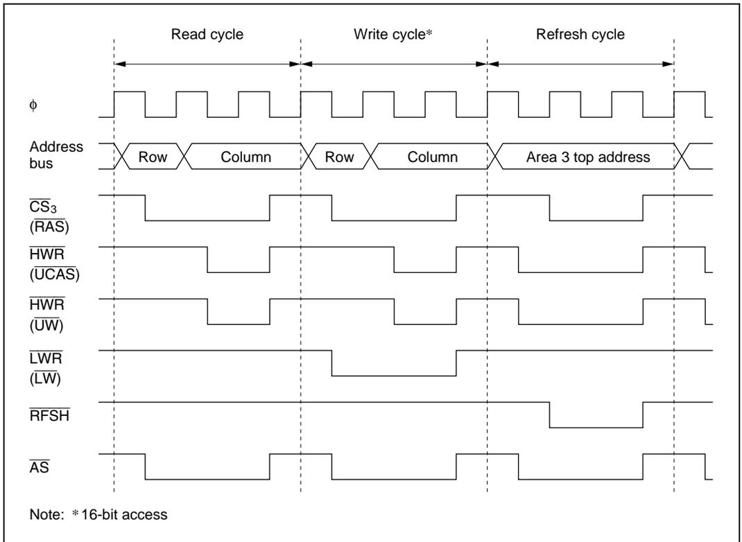
**Figure 7.5 DRAM Control Signal Output Timing (2) ( $\overline{2CAS}$  Mode)**
