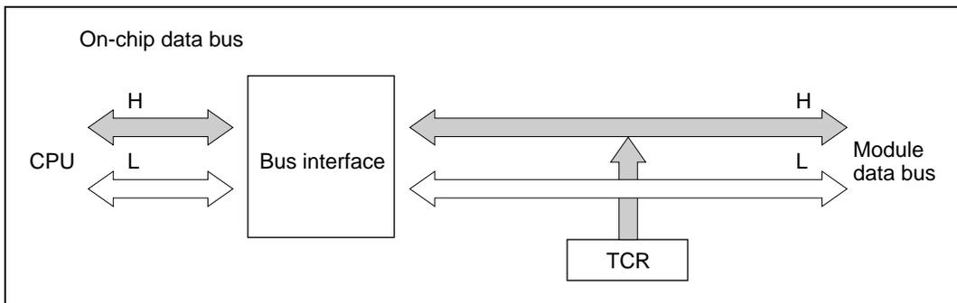
**Figure 10.13 Access to Timer Counter (CPU Reads TCR)**
