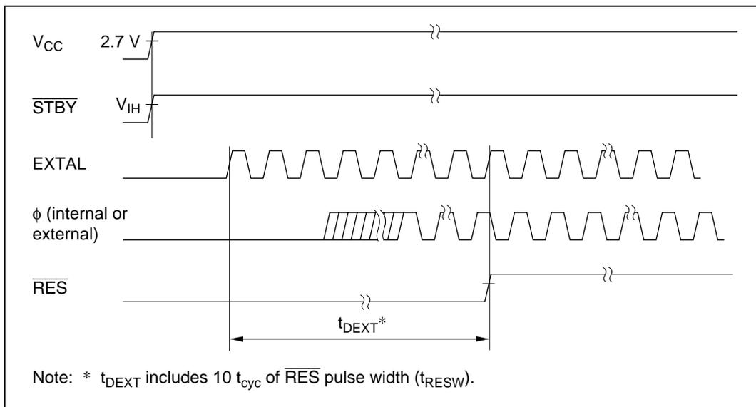
**Figure 19.7 External Clock Output Settling Delay Timing**
