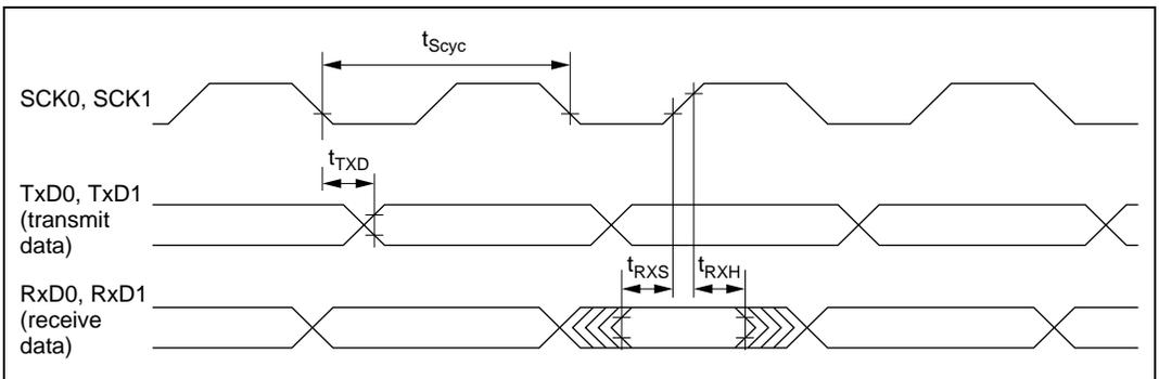
**Figure 21.23 SCI Input/Output Timing in Synchronous Mode**
