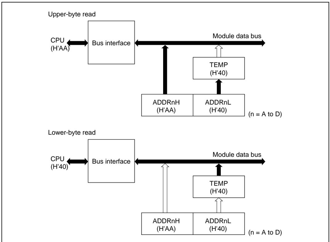
**Figure 15.2 A/D Data Register Access Operation (Reading H'AA40)**
