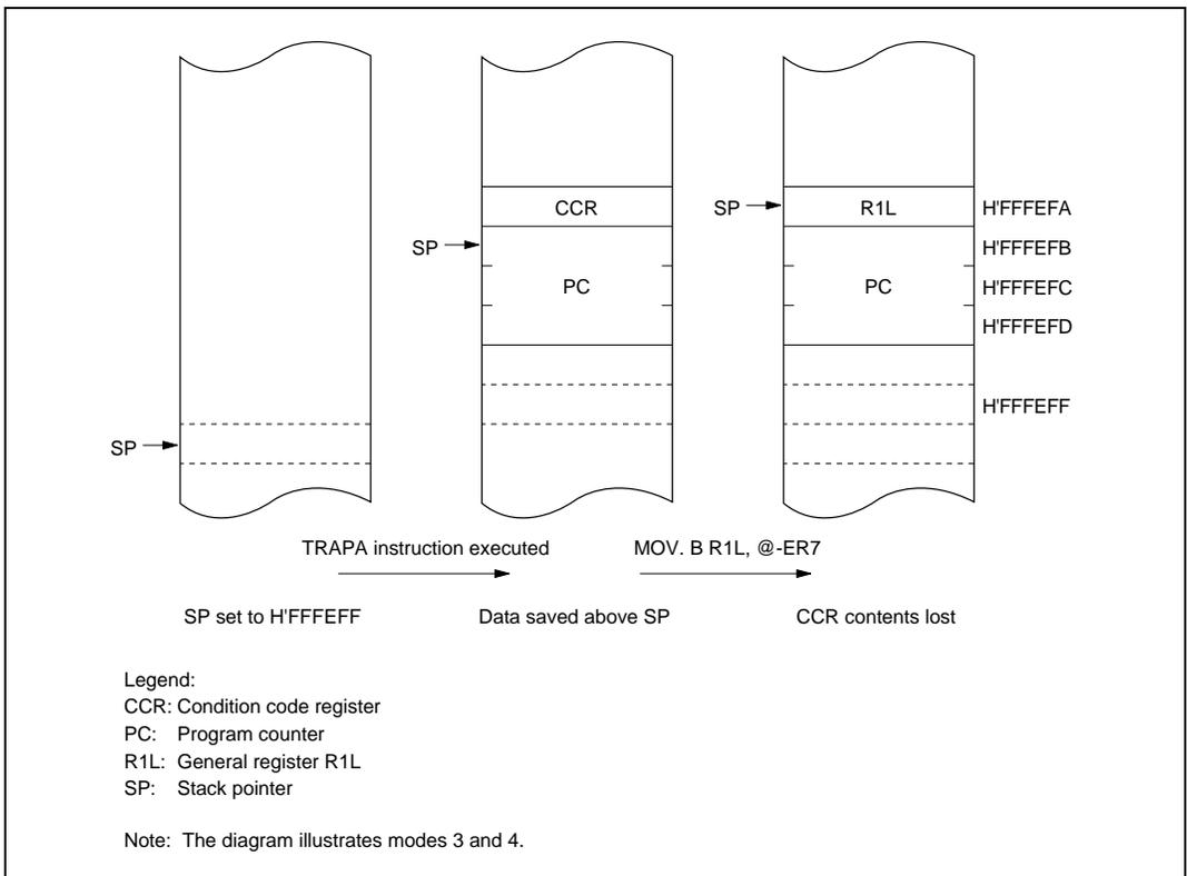
**Figure 4.7 Operation when SP Value Is Odd**
