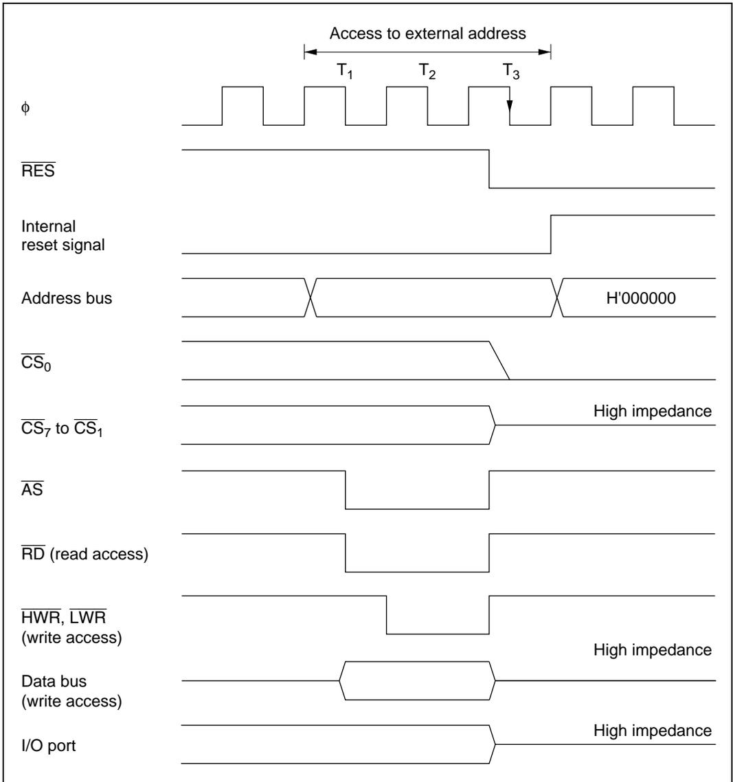
**Figure D.3 Reset during Memory Access (Reset during T<sub>3</sub> State)**
