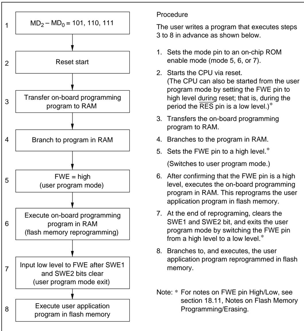
**Figure 18.10 User Program Mode Execution Procedure (Example)**
