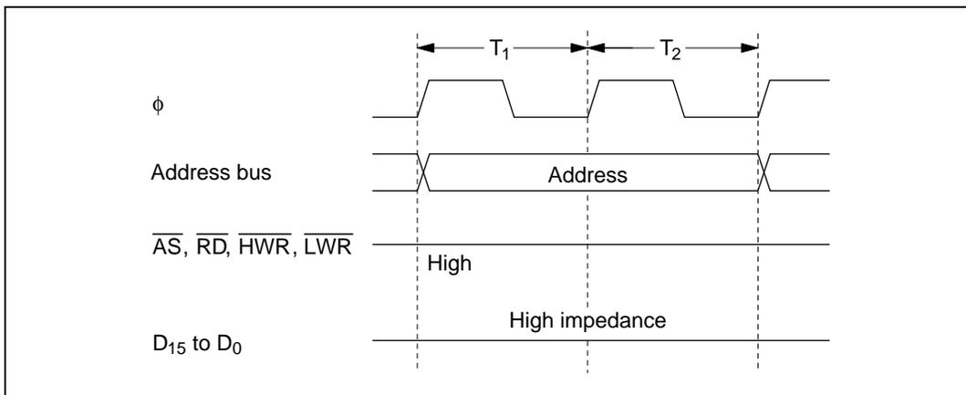
**Figure 2.15 Pin States during On-Chip Memory Access**
