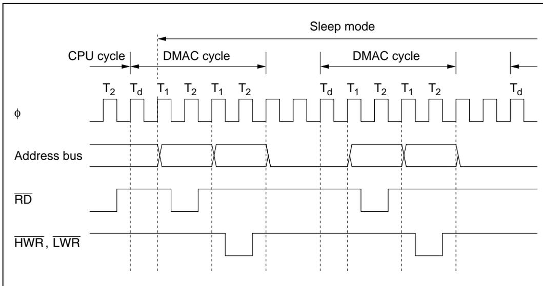
**Figure 8.24 Timing of Cycle-Steal Transfer in Sleep Mode**
