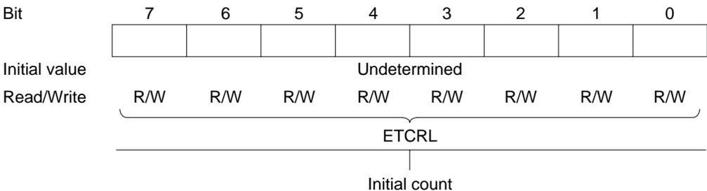
In repeat mode, ETCRH functions as an 8-bit transfer counter and ETCRL holds the initial transfer count. ETCRH is decremented by 1 each time one transfer is executed. When ETCRH reaches H'00, the value in ETCRL is reloaded into ETCRH and the same operation is repeated. The ETCRs are not initialized by a reset or in standby mode.
