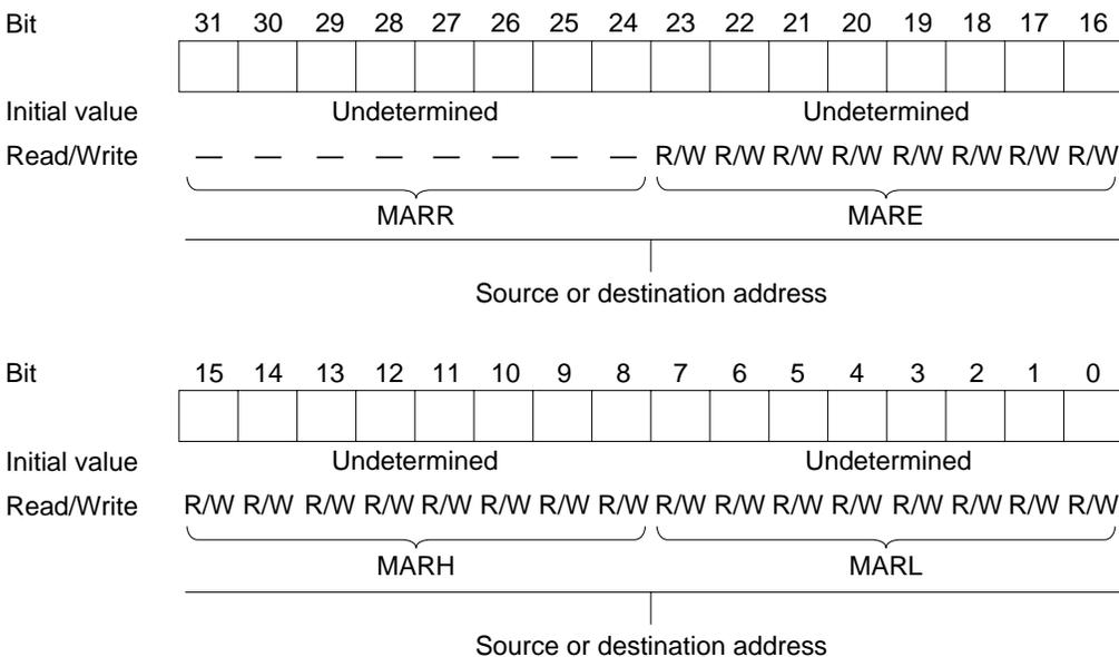
The MAR value is incremented or decremented each time one byte or word is transferred, automatically updating the source or destination memory address. For details, see section 8.3.4, Data Transfer Control Registers (DTCR).
