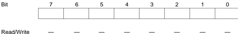
The SCI loads transmit data from TDR into TSR, then transmits the data serially from the TxD pin, LSB (bit 0) first. After transmitting one data byte, the SCI automatically loads the next transmit data from TDR into TSR and starts transmitting it. If the TDRE flag is set to 1 in SSR, however, the SCI does not load the TDR contents into TSR. The CPU cannot read or write TSR directly.
