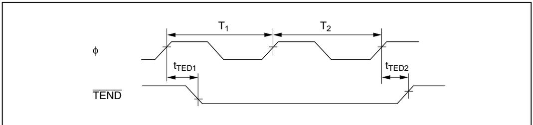
Figure 21.24 DMAC  $\overline{\text{TEND}}$  Output Timing for 2 State Access
