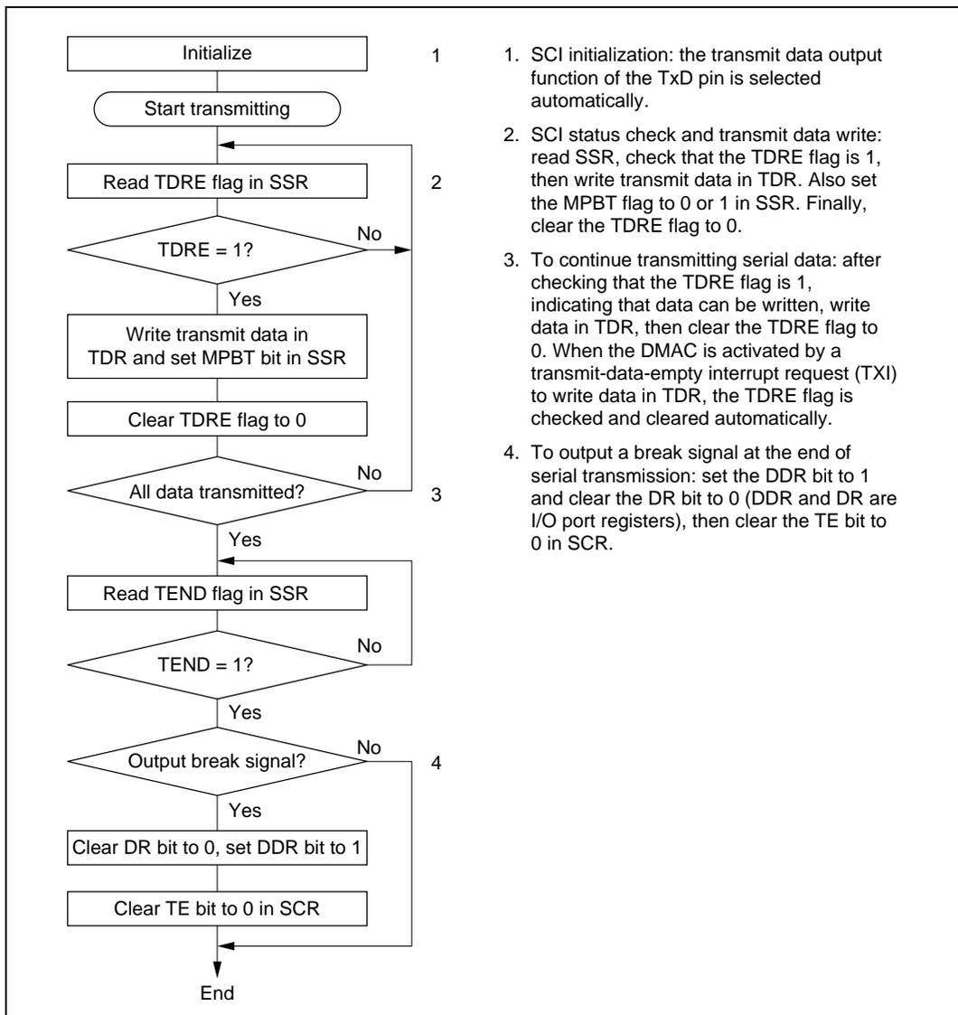
Figure 13.10 Sample Flowchart for Transmitting Multiprocessor Serial Data
