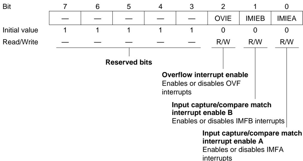
Each TIER is an 8-bit readable/writable register that enables and disables overflow interrupt requests and general register input capture and compare match interrupt requests.
