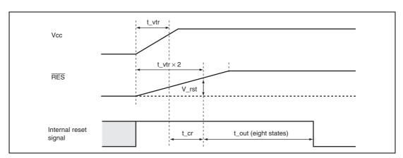
Figure 23.1 Power-On Reset Circuit Reset Timing
