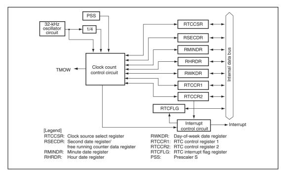
Figure 10.1 Block Diagram of RTC
