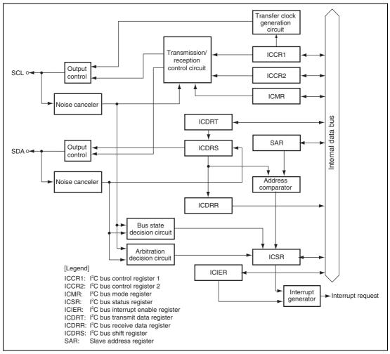
Figure 19.1 Block Diagram of I<sup>2</sup>C Bus Interface 2
