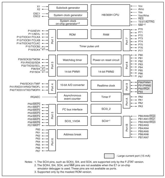
Figure 1.2 Block Diagram of H8/38776 Group
