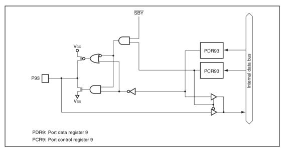
Figure B.8 (a) Port 9 Block Diagram (P93)
