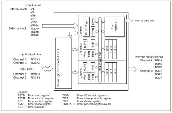
Figure 12.1 Block Diagram of TPU
