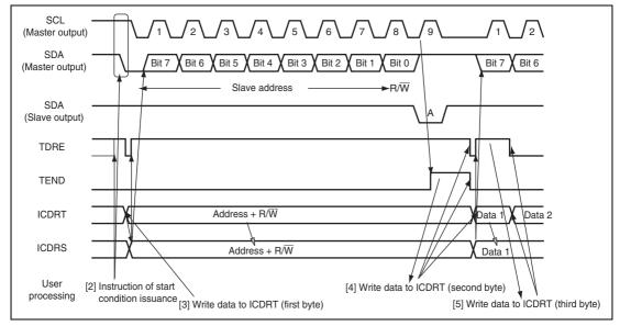
Figure 19.5 Master Transmit Mode Operation Timing (1)
