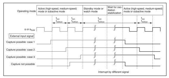
Figure 6.3 External Input Signal Capture when Signal Changes before/after Standby Mode or Watch Mode
