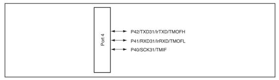
Figure 9.3 Port 4 Pin Configuration
