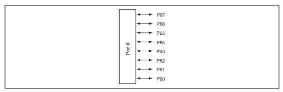
Figure 9.5 Port 6 Pin Configuration
