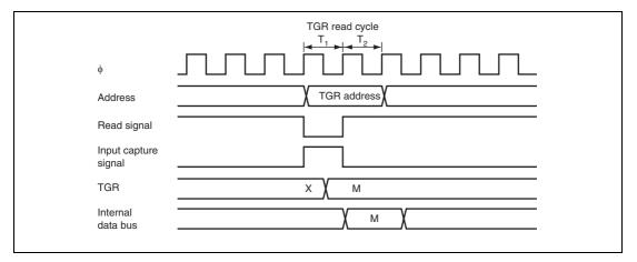
Figure 12.35 Contention between TGR Read and Input Capture
