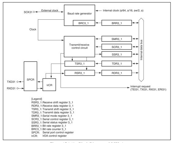
Figure 15.1 (1) Block Diagram of SCI3\_1
