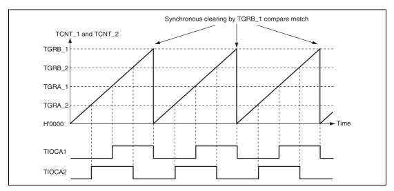
Figure 12.15 Example of Synchronous Operation
