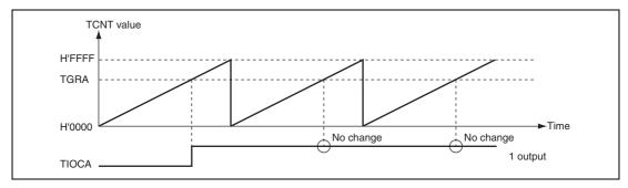
Figure 12.10 Example of 0 Output/1 Output Operation
