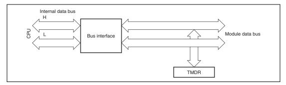
Figure 12.4 8-Bit Register Access Operation [CPU ↔ TMDR (Lower 8 Bits)]
