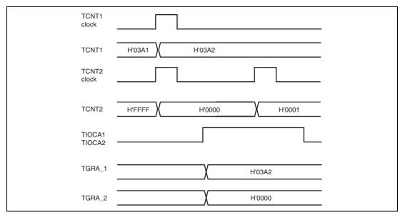
Figure 12.17 Example of Operation with Cascaded Connection
