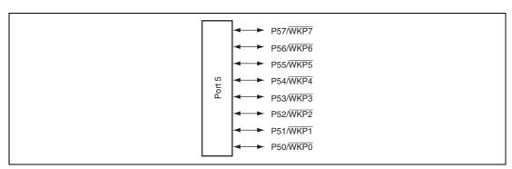
Figure 9.4 Port 5 Pin Configuration
