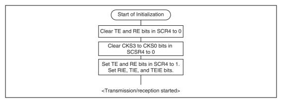
Figure 16.3 Flowchart Example of SCI4 Initialization
