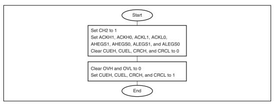
Figure 13.3 Software Procedure when Using ECH and ECL as 8-Bit Event Counters
