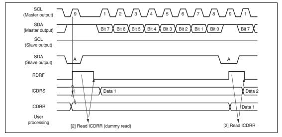
Figure 19.11 Slave Receive Mode Operation Timing (1)
