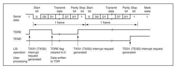
Figure 15.5 Example SCI3 Operation in Transmission in Asynchronous Mode (8-Bit Data, Parity, One Stop Bit)
