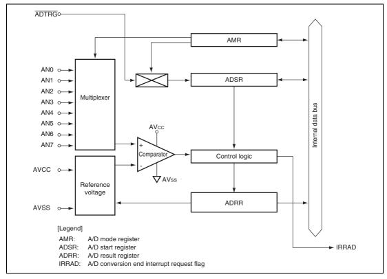
Figure 18.1 Block Diagram of A/D Converter
