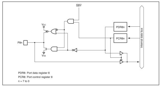
Figure B.7 Port 8 Block Diagram
