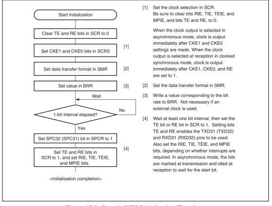
Figure 15.4 Sample SCI3 Initialization Flowchart
