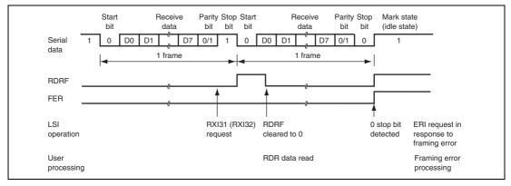
Figure 15.7 Example SCI3 Operation in Reception in Asynchronous Mode (8-Bit Data, Parity, One Stop Bit)
