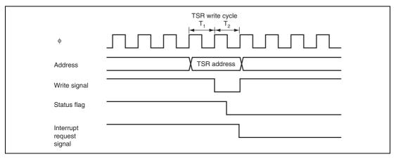
Figure 12.31 Timing for Status Flag Clearing by CPU
