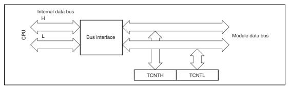
Figure 12.2 16-Bit Register Access Operation [CPU ↔ TCNT (16 Bits)]
