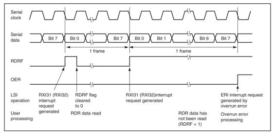
Figure 15.12 Example of SCI3 Reception Operation in Clock Synchronous Mode
