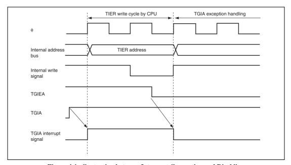
Figure 4.4 Contention between Interrupt Generation and Disabling
