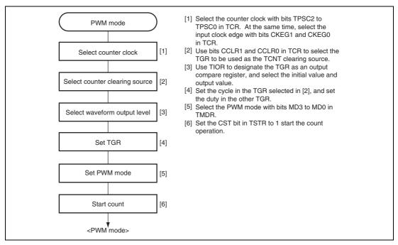
Figure 12.18 Example of PWM Mode Setting Procedure
