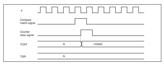
Figure 12.26 Counter Clear Timing (Compare Match)
