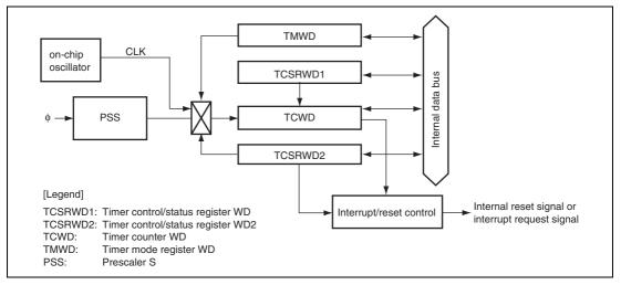
Figure 14.1 Block Diagram of Watchdog Timer
