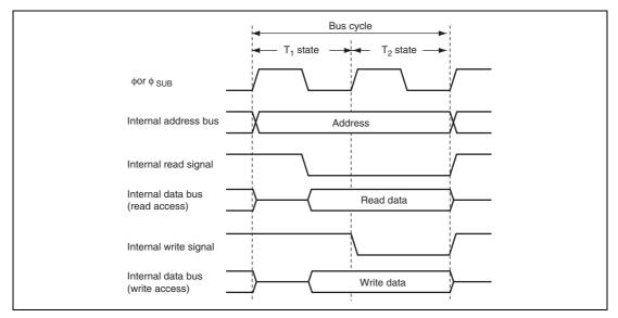
Figure 2.9 On-Chip Memory Access Cycle
