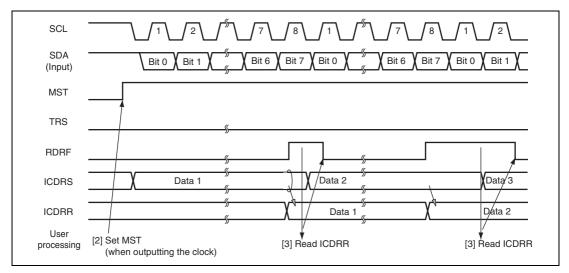
Figure 19.15 Receive Mode Operation Timing
