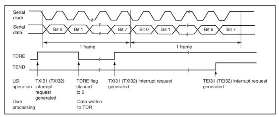
Figure 15.10 Example of SCI3 Operation in Transmission in Clock Synchronous Mode
