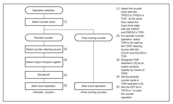
Figure 12.6 Example of Counter Operation Setting Procedure
