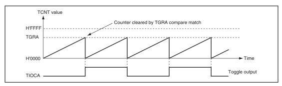
Figure 12.11 Example of Toggle Output Operation
