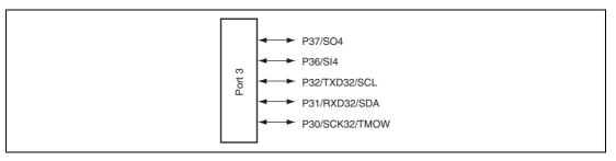
Figure 9.2 Port 3 Pin Configuration
