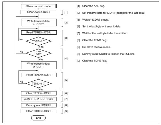
Figure 19.19 Sample Flowchart for Slave Transmit Mode
