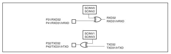
Figure 9.11 Input/Output Data Inversion Function
