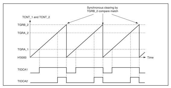
Figure 12.20 Example of PWM Mode Operation (2)
