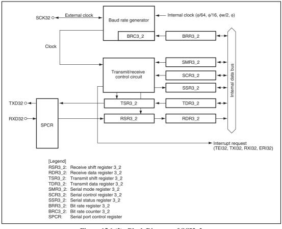
Figure 15.1 (2) Block Diagram of SCI3\_2
