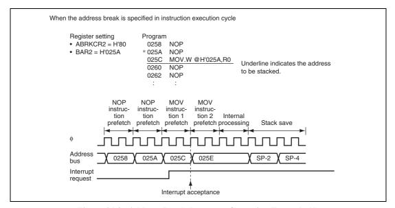
Figure 21.2 Address Break Interrupt Operation Example (1)
