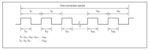
Figure 17.3 Waveform Output by PWM
