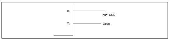
Figure 5.7 Pin Connection when not Using Subclock
