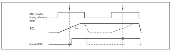
Figure 19.21 Timing of Bit Synchronous Circuit
