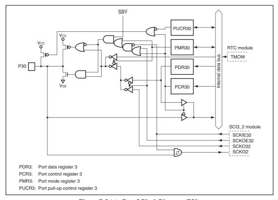
Figure B.2 (g) Port 3 Block Diagram (P30)
