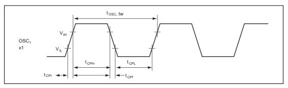
Figure 23.2 Clock Input Timing
