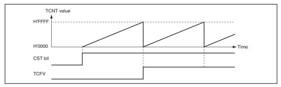
Figure 12.7 Free-Running Counter Operation
