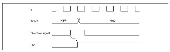
Figure 14.4 Timing of OVF Flag Setting
