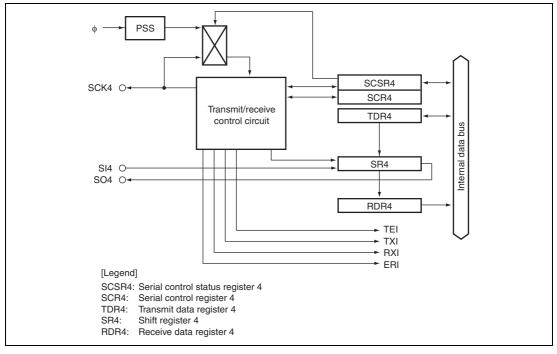
Figure 16.1 Block Diagram of SCI4
