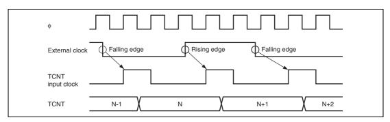
Figure 12.23 Count Timing in External Clock Operation
