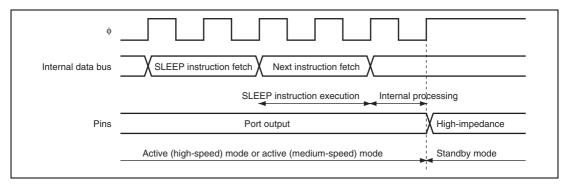
Figure 6.2 Standby Mode Transition and Pin States
