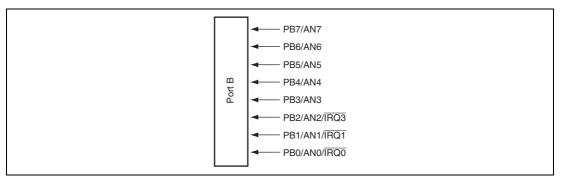
Figure 9.10 Port B Pin Configuration
