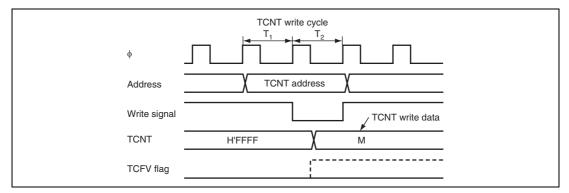
Figure 12.38 Contention between TCNT Write and Overflow
