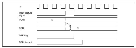
Figure 12.29 TGI Interrupt Timing (Input Capture)
