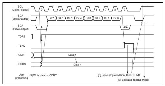
Figure 19.6 Master Transmit Mode Operation Timing (2)
