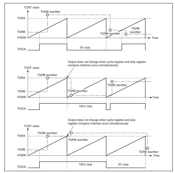
Figure 12.21 Example of PWM Mode Operation (3)
