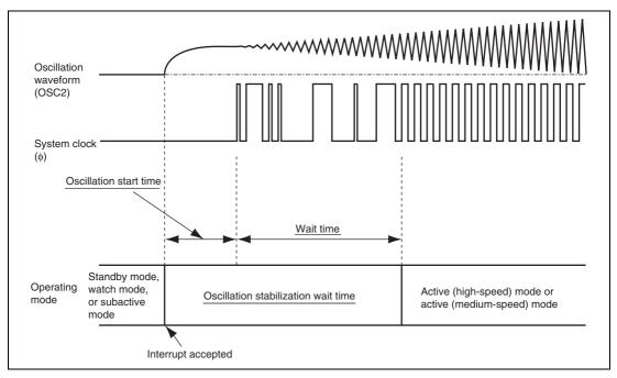
Figure 5.12 Oscillation Stabilization Wait Time
