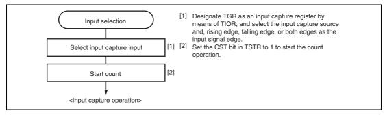
Figure 12.12 Example of Setting Procedure for Input Capture Operation
