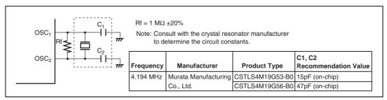
Figure 5.3 Typical Connection to Ceramic Resonator
