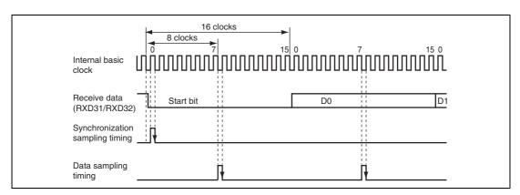
Figure 15.18 Receive Data Sampling Timing in Asynchronous Mode
