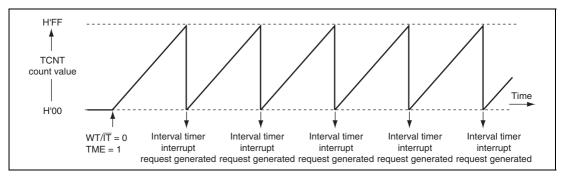
Figure 14.3 Interval Timer Mode Operation
