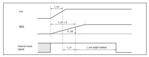
Figure 20.2 Power-On Reset Circuit Operation Timing
