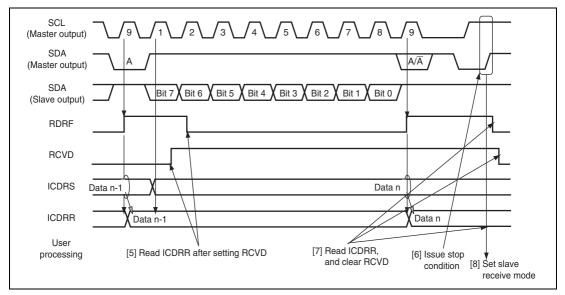
Figure 19.8 Master Receive Mode Operation Timing (2)
