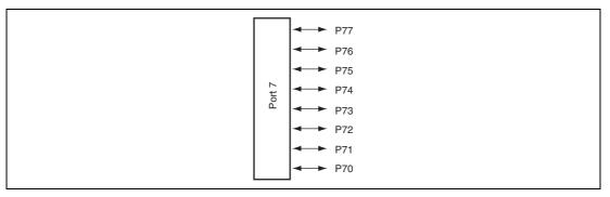
Figure 9.6 Port 7 Pin Configuration
