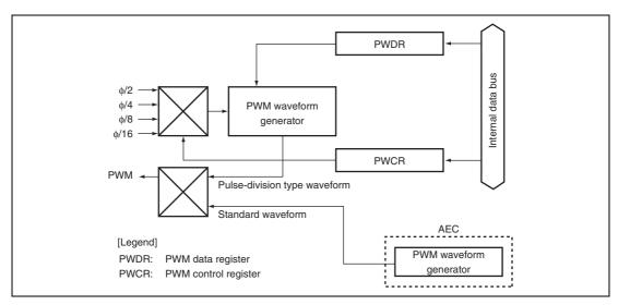
Figure 17.1 Block Diagram of 14-Bit PWM
