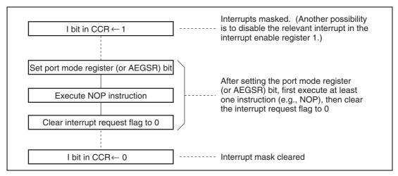
Figure 3.5 Port Mode Register (or AEGSR) Setting and Interrupt Request Flag Clearing Procedure
