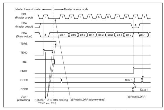
Figure 19.7 Master Receive Mode Operation Timing (1)
