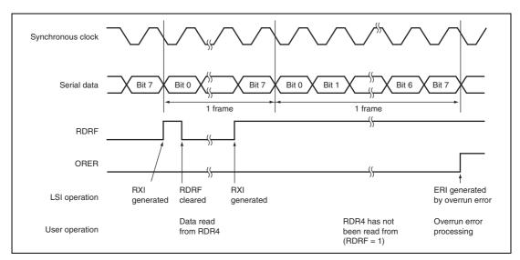
Figure 16.7 Receive Operation Example
