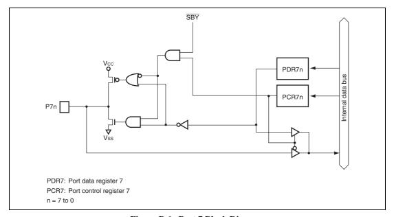
Figure B.6 Port 7 Block Diagram
