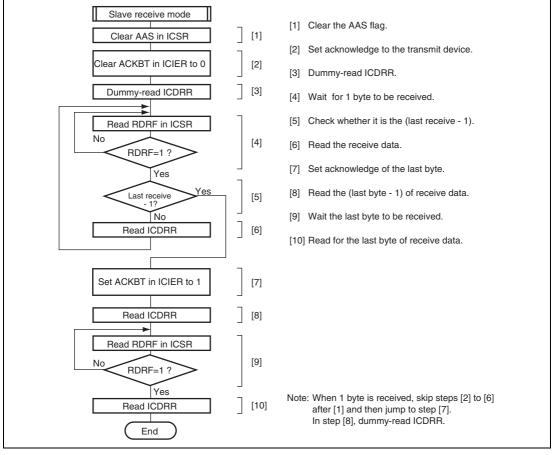
Figure 19.20 Sample Flowchart for Slave Receive Mode
