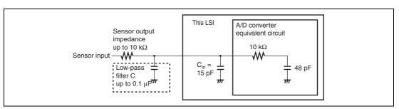
Figure 18.8 Example of Analog Input Circuit
