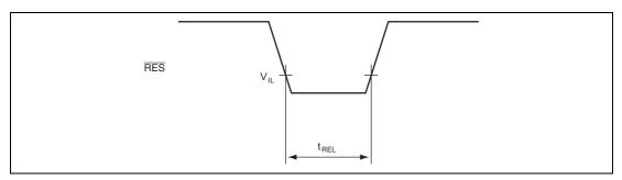
Figure 23.3 RES Low Width Timing
