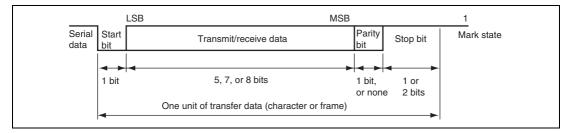
Figure 15.2 Data Format in Asynchronous Communication
