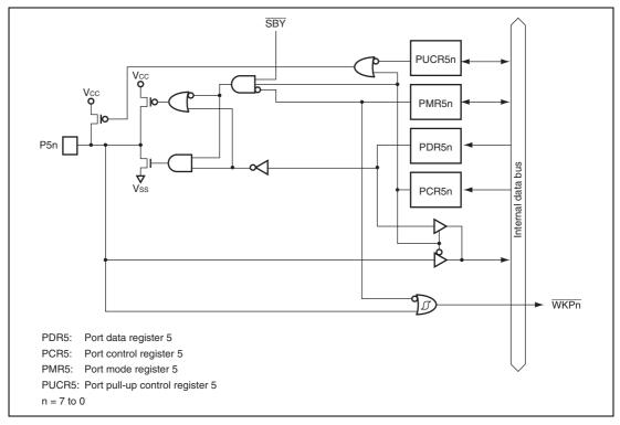
Figure B.4 Port 5 Block Diagram
