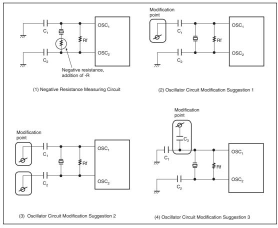
Figure 5.10 Negative Resistance Measurement and Circuit Modification Suggestions
