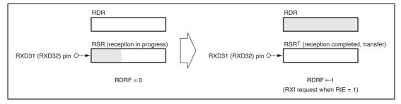
Figure 15.17 (a) RDRF Setting and RXI Interrupt
