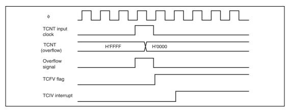
Figure 12.30 TCIV Interrupt Setting Timing
