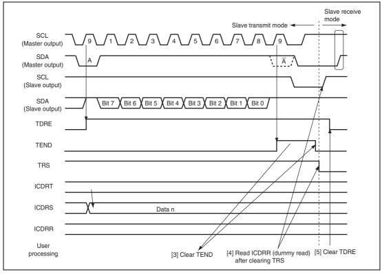
Figure 19.10 Slave Transmit Mode Operation Timing (2)
