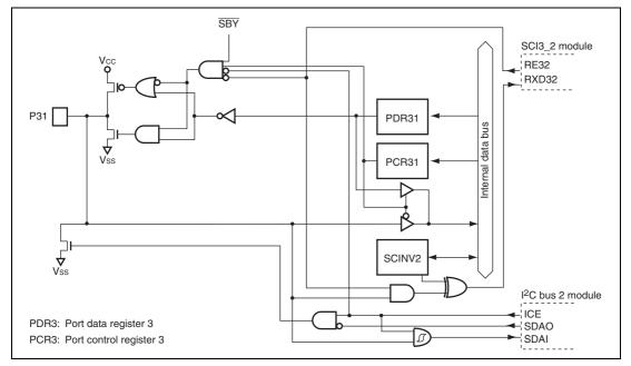
Figure B.2 (f) Port 3 Block Diagram (P31)
