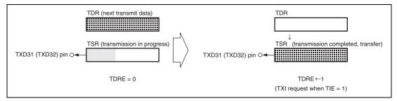
Figure 15.17 (b) TDRE Setting and TXI Interrupt
