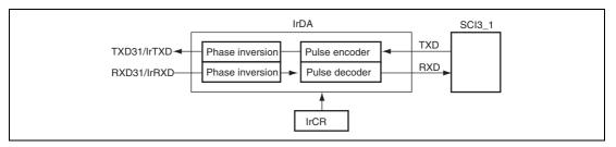
Figure 15.15 IrDA Block Diagram
