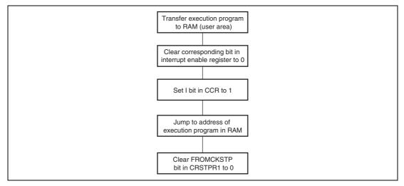
Figure 7.5 Module Standby Mode Setting
