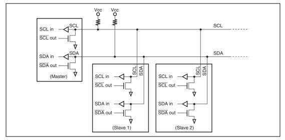
Figure 19.2 External Circuit Connections of I/O Pins
