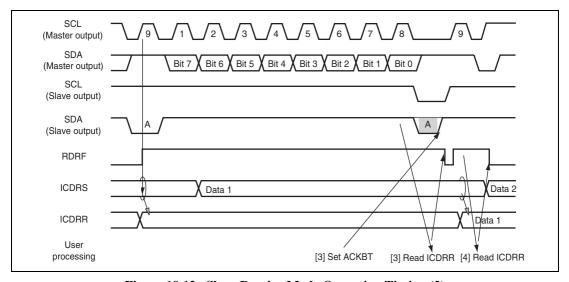
Figure 19.12 Slave Receive Mode Operation Timing (2)
