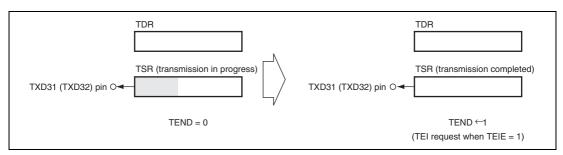
Figure 15.17 (c) TEND Setting and TEI Interrupt
