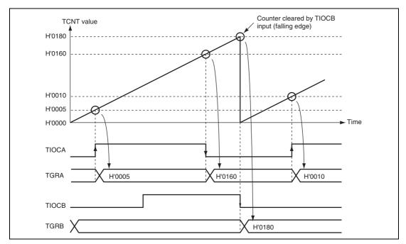
Figure 12.13 Example of Input Capture Operation
