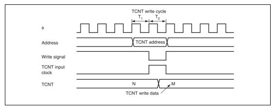
Figure 12.33 Contention between TCNT Write and Increment Operation
