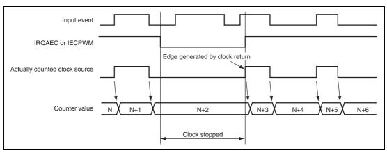
Figure 13.5 Example of Clock Control Operation
