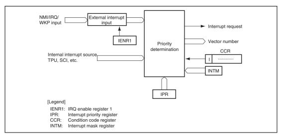
Figure 4.1 Block Diagram of Interrupt Controller
