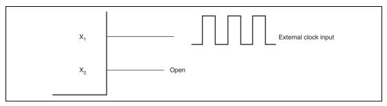
Figure 5.8 Pin Connection when Inputting External Clock
