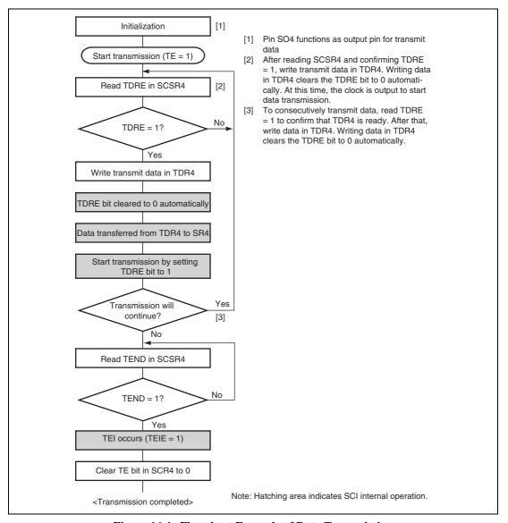
Figure 16.4 Flowchart Example of Data Transmission
