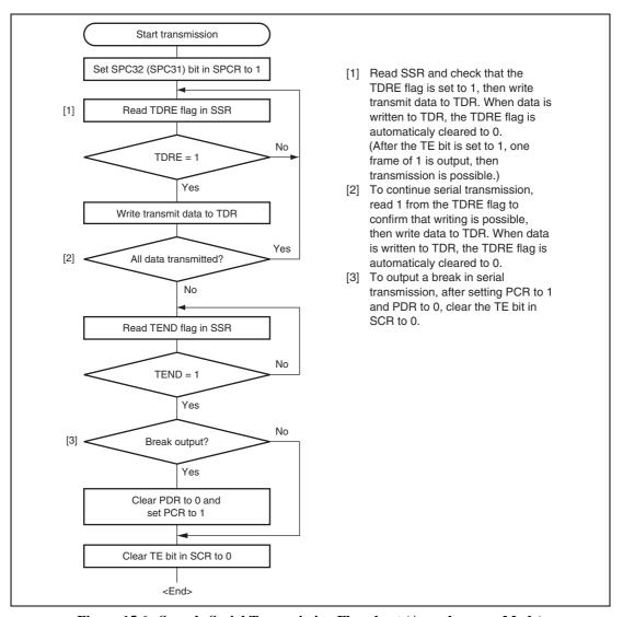
Figure 15.6 Sample Serial Transmission Flowchart (Asynchronous Mode)
