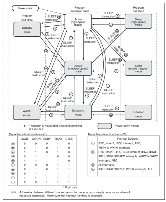
Figure 6.1 Mode Transition Diagram
