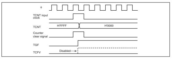
Figure 12.37 Contention between Overflow and Counter Clearing
