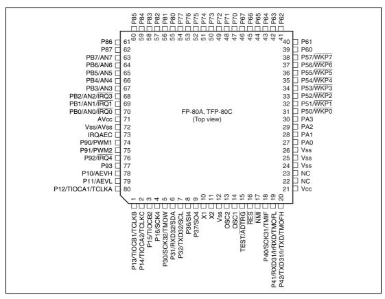
Figure 1.3 Pin Assignment of H8/38776 Group (FP-80A, TFP-80C)
