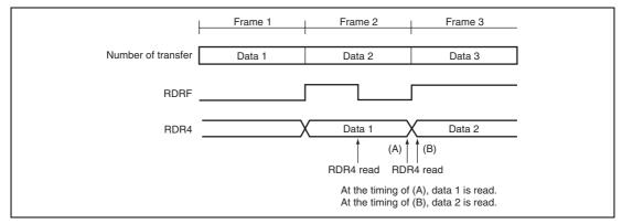
Figure 16.9 Relationship between Reading RDR4 and RDRF
