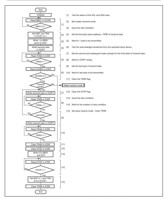
Figure 19.17 Sample Flowchart for Master Transmit Mode
