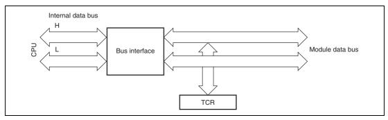
Figure 12.3 8-Bit Register Access Operation [CPU ↔ TCR (Upper 8 Bits)]
