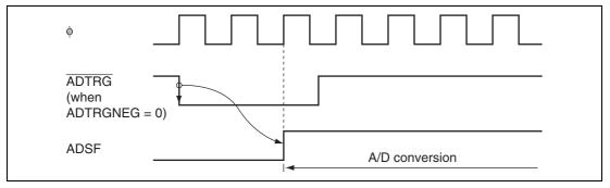
Figure 18.2 External Trigger Input Timing
