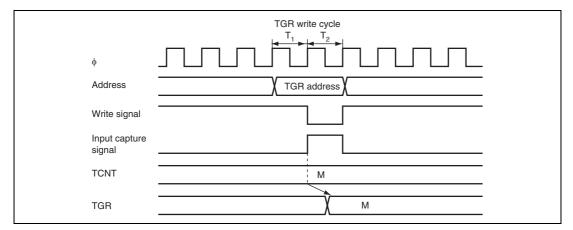
Figure 12.36 Contention between TGR Write and Input Capture
