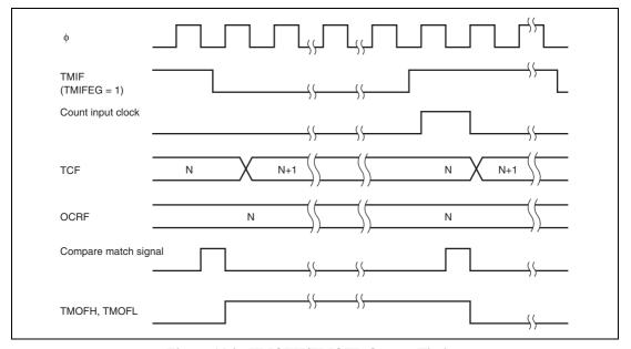
Figure 11.2 TMOFH/TMOFL Output Timing
