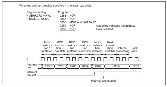
Figure 21.2 Address Break Interrupt Operation Example (2)
