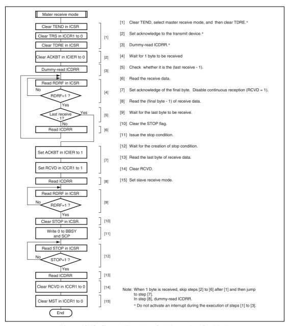
Figure 19.18 Sample Flowchart for Master Receive Mode
