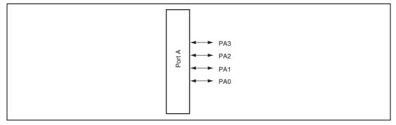
Figure 9.9 Port A Pin Configuration
