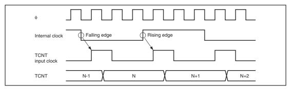
Figure 12.22 Count Timing in Internal Clock Operation
