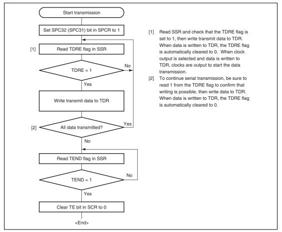
Figure 15.11 Sample Serial Transmission Flowchart (Clock Synchronous Mode)
