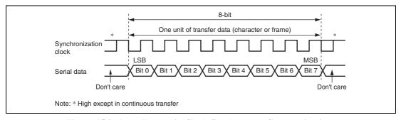
Figure 15.9 Data Format in Clock Synchronous Communications
