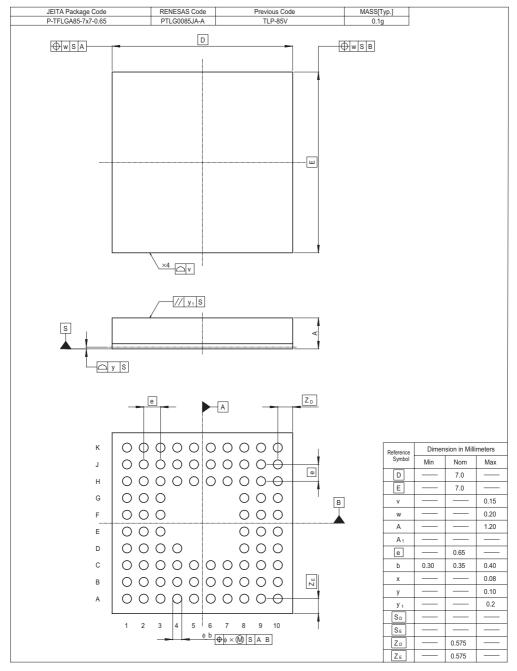
Figure D.3 Package Dimensions (TLP-85V)
