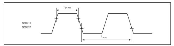
Figure 23.5 SCK3 Input Clock Timing
