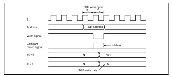
Figure 12.34 Contention between TGR Write and Compare Match
