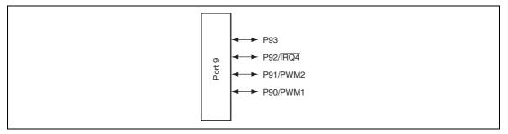
Figure 9.8 Port 9 Pin Configuration
