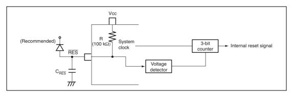
Figure 20.1 Power-On Reset Circuit
