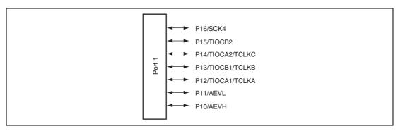
Figure 9.1 Port 1 Pin Configuration
