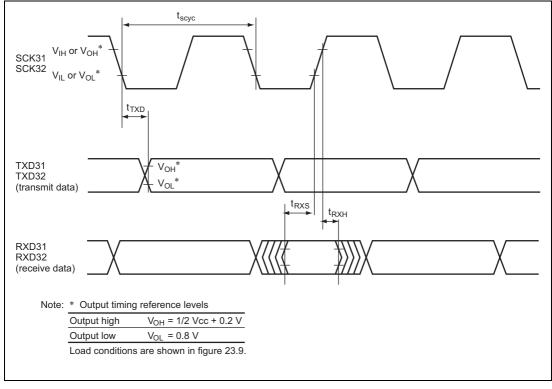
Figure 23.6 SCI3 Input/Output Timing in Clocked Synchronous Mode
