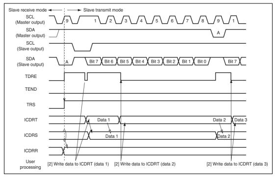
Figure 19.9 Slave Transmit Mode Operation Timing (1)
