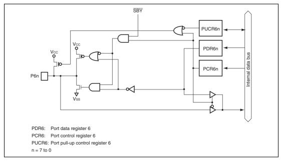
Figure B.5 Port 6 Block Diagram
