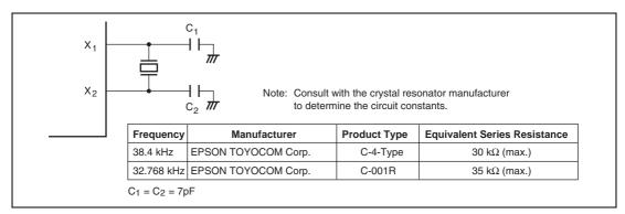
Figure 5.5 Typical Connection to 32.768-kHz/38.4-kHz Crystal Resonator
