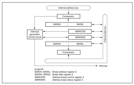
Figure 21.1 Block Diagram of Address Break
