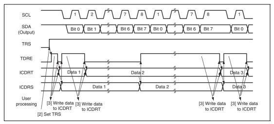
Figure 19.14 Transmit Mode Operation Timing
