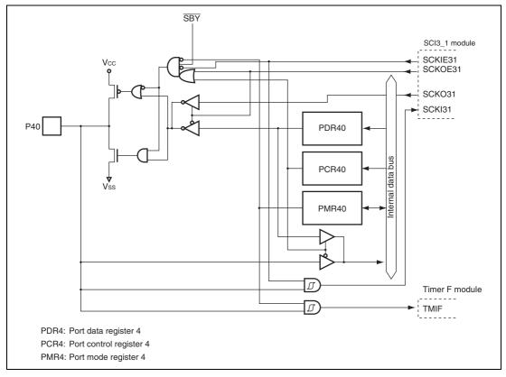
Figure B.3 (c) Port 4 Block Diagram (P40)
