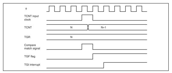
Figure 12.28 TGI Interrupt Timing (Compare Match)
