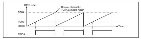
Figure 12.19 Example of PWM Mode Operation (1)
