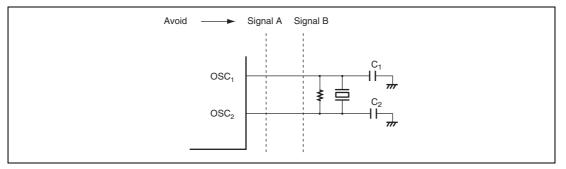
Figure 5.11 Example of Incorrect Board Design
