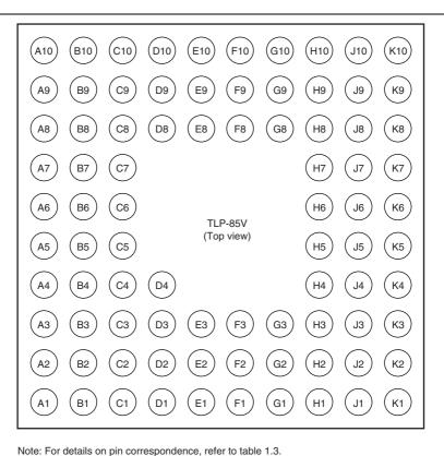
Figure 1.4 Pin Assignment of H8/38776 Group (TLP-85V)
