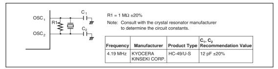
Figure 5.2 Typical Connection to Crystal Resonator
