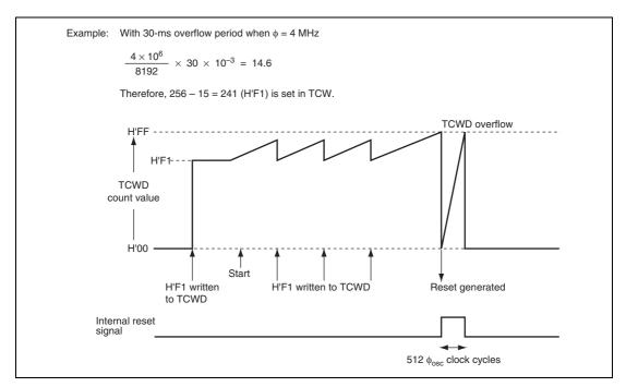
Figure 14.2 Example of Watchdog Timer Operation
