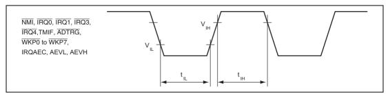
Figure 23.4 Input Timing
