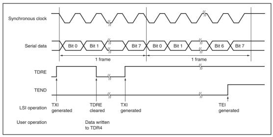
Figure 16.5 Transmit Operation Example
