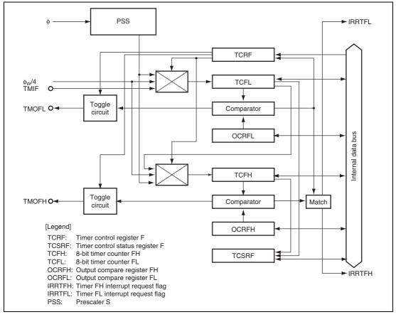
Figure 11.1 Block Diagram of Timer F
