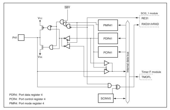
Figure B.3 (b) Port 4 Block Diagram (P41)
