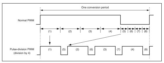
Figure 17.2 Operation of Pulse-Division-Type PWM with Division by 4
