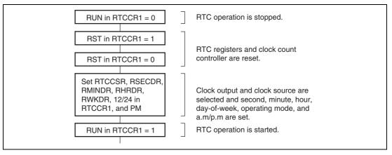
Figure 10.3 Initial Setting Procedure
