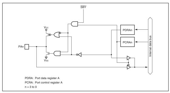
Figure B.9 Port A Block Diagram
