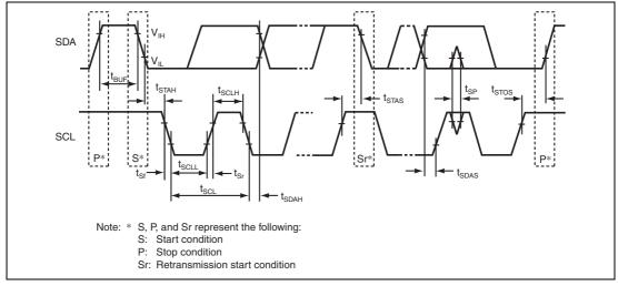
Figure 23.8 I<sup>2</sup>C Bus Interface Input/Output Timing
