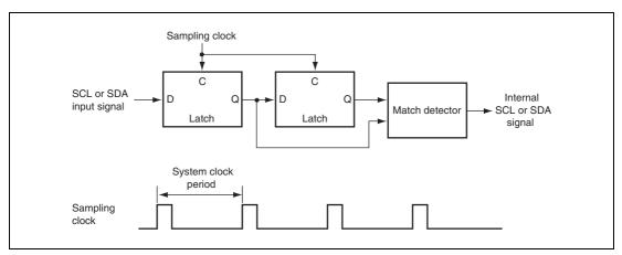
Figure 19.16 Block Diagram of Noise Conceler
