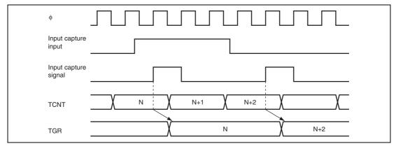
Figure 12.25 Input Capture Input Signal Timing
