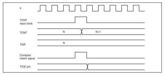
Figure 12.24 Output Compare Output Timing
