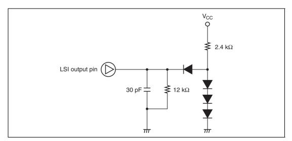
Figure 23.9 Output Load Condition
