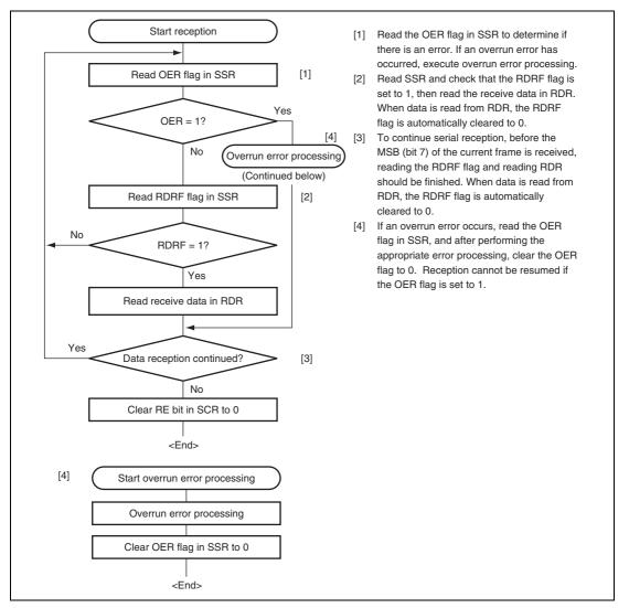
Figure 15.13 Sample Serial Reception Flowchart (Clock Synchronous Mode)
