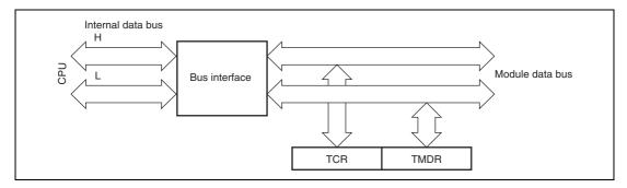
Figure 12.5 8-Bit Register Access Operation [CPU  $\leftrightarrow$  TCR and TMDR (16 Bits)]
