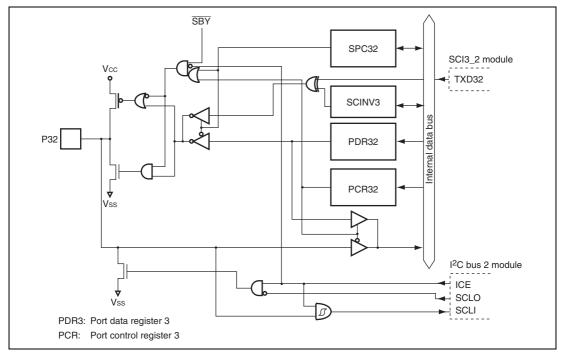
Figure B.2 (e) Port 3 Block Diagram (P32)
