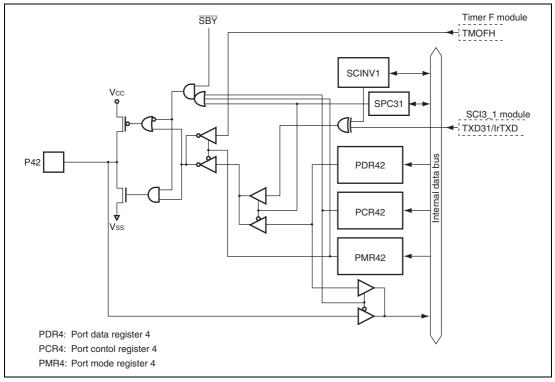
Figure B.3 (a) Port 4 Block Diagram (P42)
