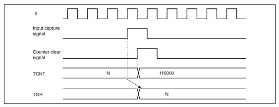
Figure 12.27 Counter Clear Timing (Input Capture)
