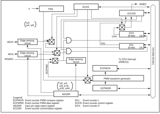
Figure 13.1 Block Diagram of the Asynchronous Event Counter
