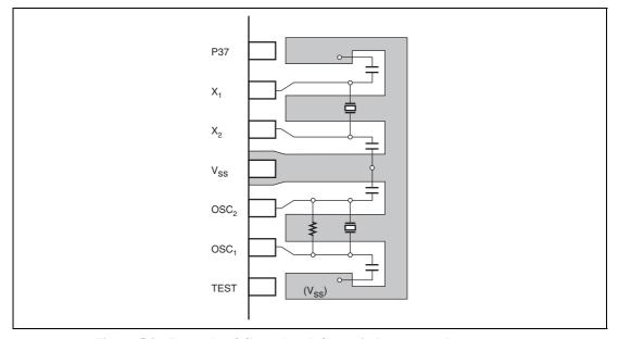
Figure 5.9 Example of Crystal and Ceramic Resonator Arrangement
