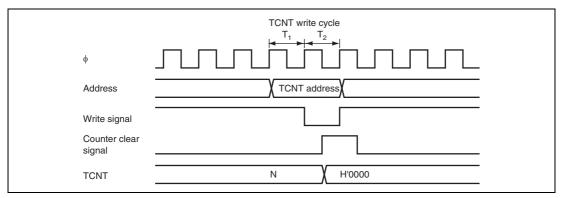
Figure 12.32 Contention between TCNT Write and Clear Operation
