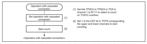
Figure 12.16 Setting Procedure for Operation with Cascaded Operation
