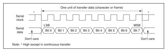
Figure 12.14 Data Format in Synchronous Communication
