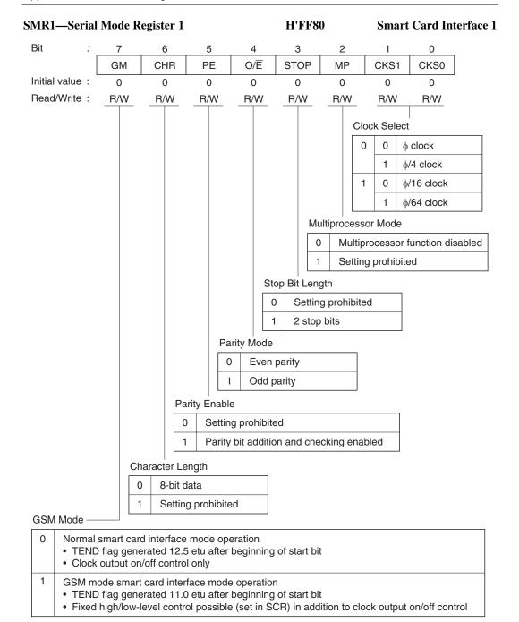
Note: etu: Elementary time unit (time for transfer of 1 bit)
