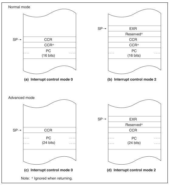
Figure 2.16 Stack Structure after Exception Handling (Examples)
