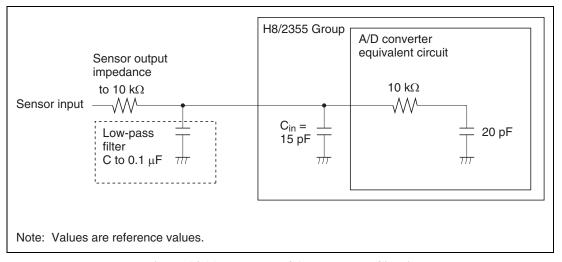
Figure 14.11 Example of Analog Input Circuit
