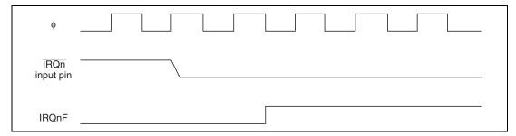
Figure 5.3 Timing of Setting IRQnF
