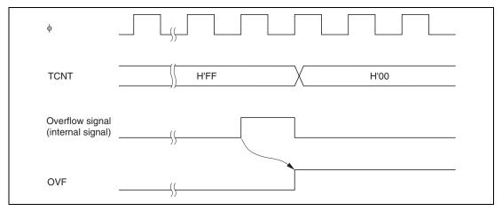
Figure 11.6 Timing of Setting of OVF
