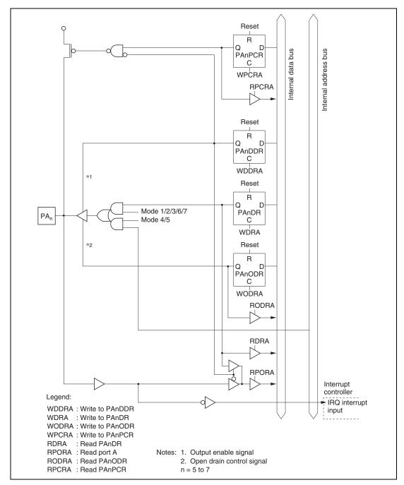
Figure C.7 (c) Port A Block Diagram (Pins PA<sub>5</sub> to PA<sub>7</sub>)
