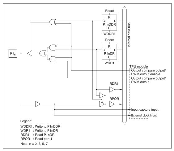
Figure C.1 (b) Port 1 Block Diagram (Pins P1<sub>2</sub>, P1<sub>3</sub>, P1<sub>5</sub>, and P1<sub>7</sub>)
