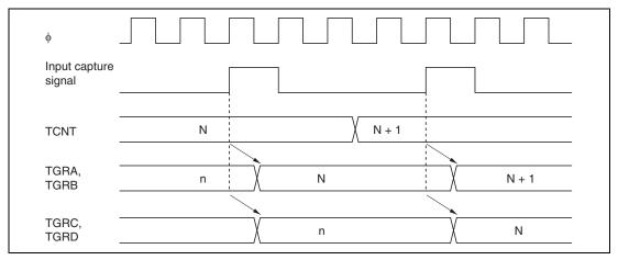
Figure 9.41 Buffer Operation Timing (Input Capture)
