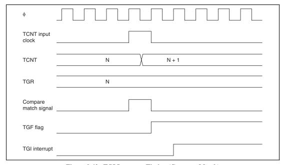
Figure 9.42 TGI Interrupt Timing (Compare Match)
