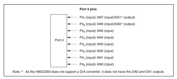
Figure 8.4 Port 4 Pin Functions
