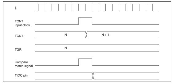
Figure 9.36 Output Compare Output Timing
