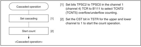
Figure 9.21 Cascaded Operation Setting Procedure
