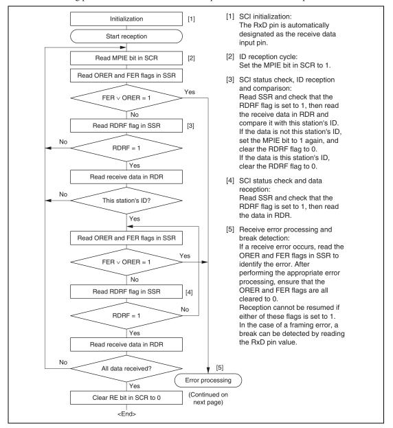
Figure 12.12 Sample Multiprocessor Serial Reception Flowchart
