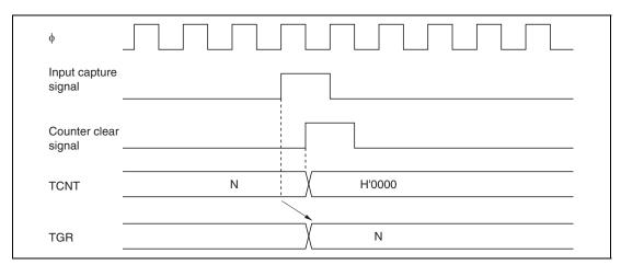
Figure 9.39 Counter Clear Timing (Input Capture)
