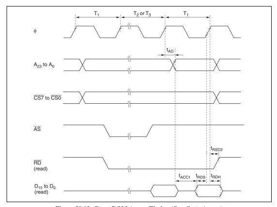
Figure 20.12 Burst ROM Access Timing (One-State Access)
