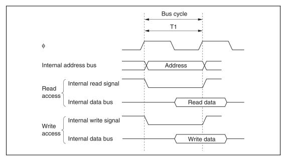
Figure 2.17 On-Chip Memory Access Cycle
