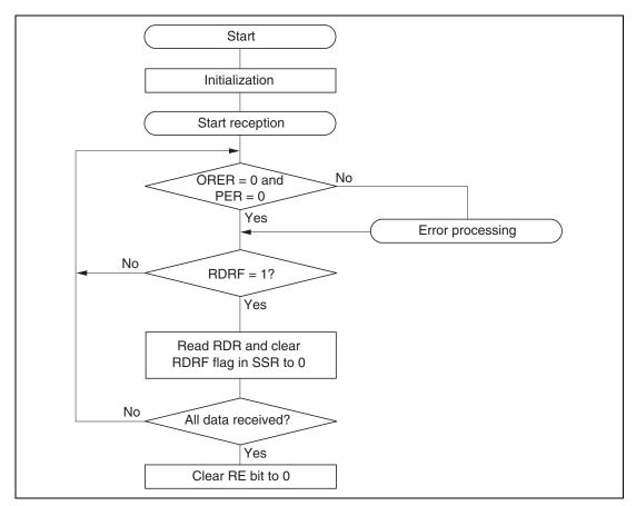
Figure 13.7 Example of Reception Processing Flow
