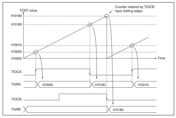
Figure 9.13 Example of Input Capture Operation
