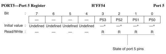
Note: \* Determined by the state of pins P5<sub>3</sub> to P5<sub>0</sub>.
