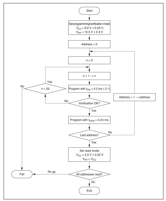
Figure 17.4 High-Speed Programming Flowchart
