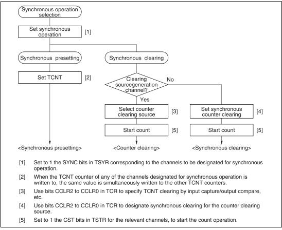
Figure 9.14 Example of Synchronous Operation Setting Procedure
