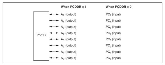
Figure 8.17 Port C Pin Functions (Modes 2 and 6)
