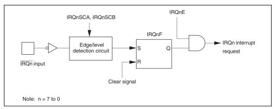
Figure 5.2 Block Diagram of Interrupts IRQ7 to IRQ0
