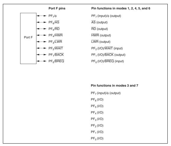
**Figure 8.25 Port F Pin Functions**
