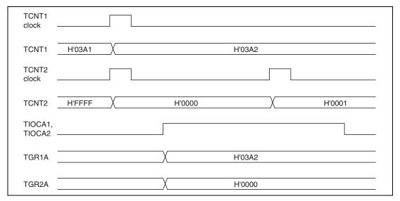
Figure 9.22 Example of Cascaded Operation (1)
