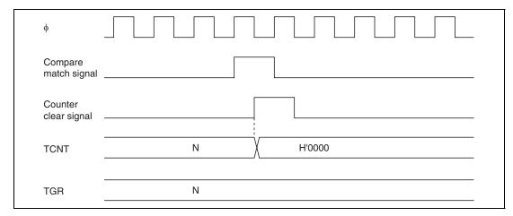
Figure 9.38 Counter Clear Timing (Compare Match)
