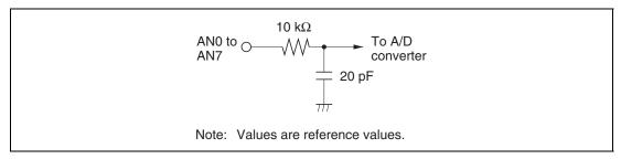
Figure 14.8 Analog Input Pin Equivalent Circuit
