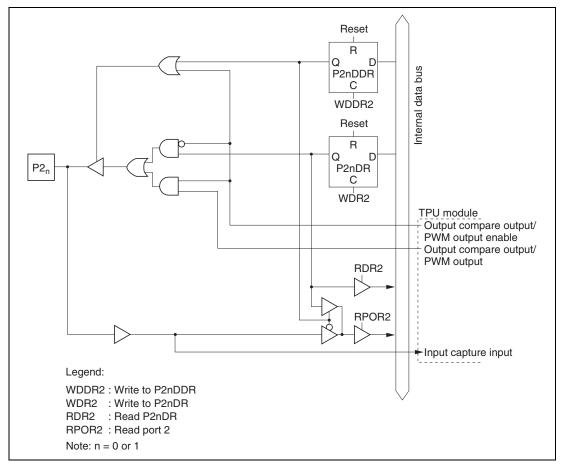
Figure C.2 (a) Port 2 Block Diagram (Pins P2, and P2,)
