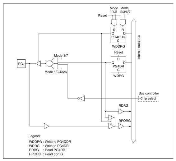
Figure C.13 (c) Port G Block Diagram (Pin  $PG_4$ )
