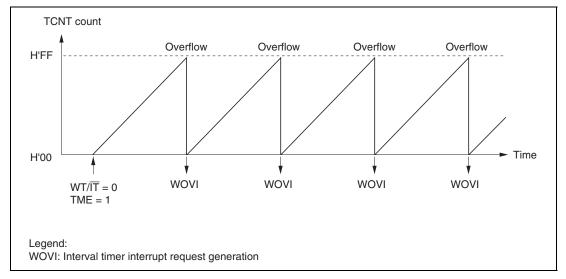
Figure 11.5 Interval Timer Operation
