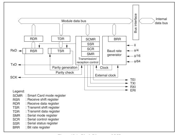
Figure 12.1 Block Diagram of SCI
