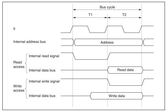
Figure 2.19 On-Chip Supporting Module Access Cycle
