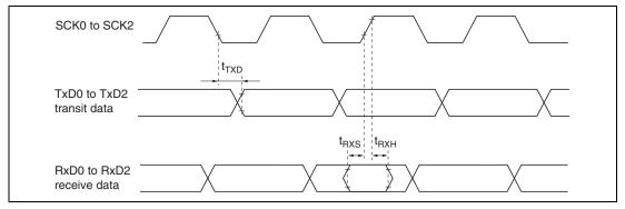
Figure 20.22 SCI Input/Output Timing (Clock Synchronous Mode)
