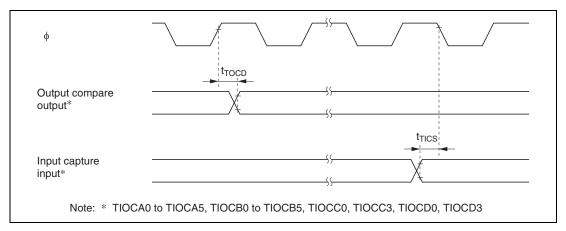
Figure 20.15 TPU Input/Output Timing
