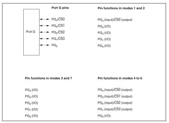
Figure 8.26 Port G Pin Functions
