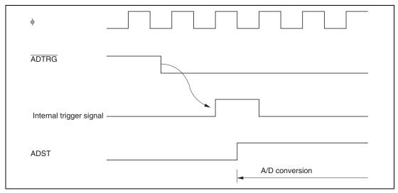
Figure 14.6 External Trigger Input Timing
