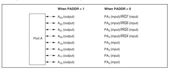
Figure 8.10 Port A Pin Functions (Mode 6)
