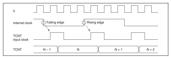
Figure 9.34 Count Timing in Internal Clock Operation
