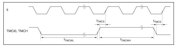
Figure 20.18 8-Bit Timer Clock Input Timing
