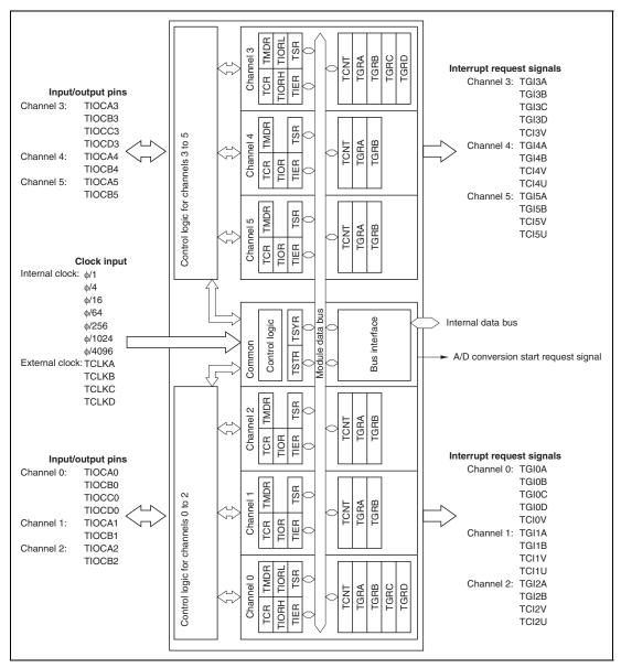
Figure 9.1 Block Diagram of TPU
