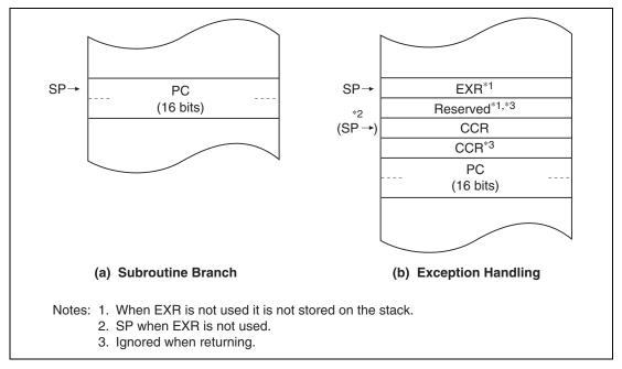
Figure 2.3 Stack Structure in Normal Mode
