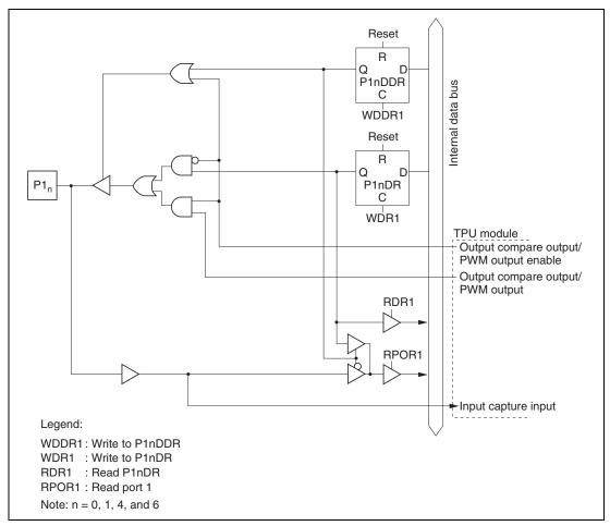
Figure C.1 (a) Port 1 Block Diagram (Pins P1, P1, P1, and P1)
