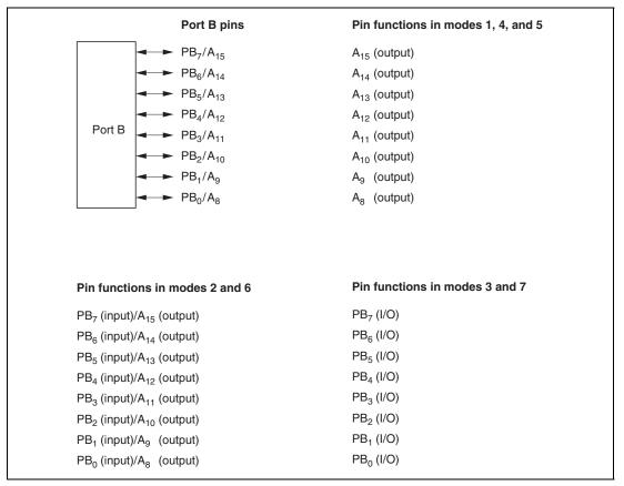
Figure 8.11 Port B Pin Functions
