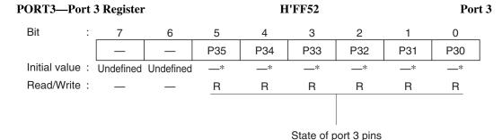
Note: \* Determined by the state of pins  $P3_5$  to  $P3_0$ .
