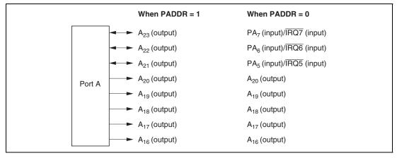
Figure 8.9 Port A Pin Functions (Modes 4 and 5)
