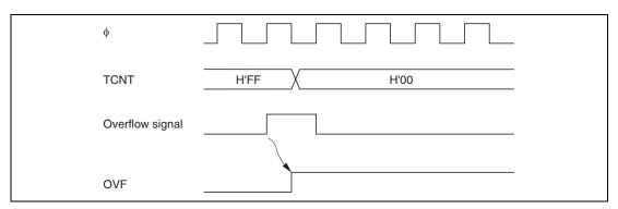
Figure 10.8 Timing of OVF Setting
