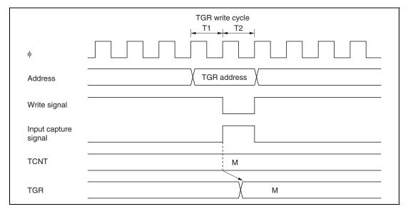
Figure 9.54 Contention between TGR Write and Input Capture
