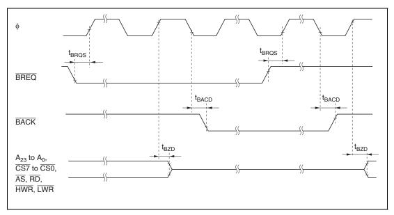
Figure 20.13 External Bus Release Timing
