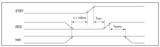
Figure F.2 Timing of Recovery from Hardware Standby Mode
