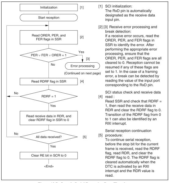
Figure 12.7 Sample Serial Reception Data Flowchart
