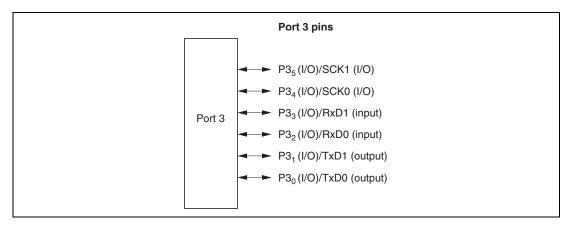
Figure 8.3 Port 3 Pin Functions
