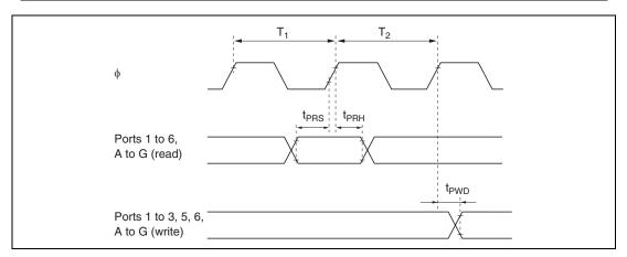
Figure 20.14 I/O Port Input/Output Timing
