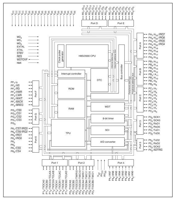
Figure 1.2 Block Diagram (H8S/2393)
