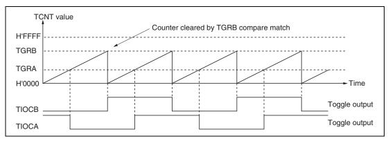
Figure 9.11 Example of Toggle Output Operation
