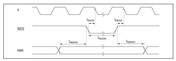
Figure 20.6 Reset Input Timing
