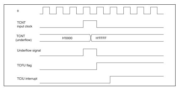
Figure 9.45 TCIU Interrupt Setting Timing
