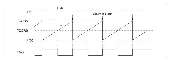
Figure 10.9 Example of Pulse Output
