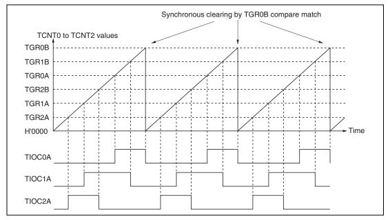
Figure 9.15 Example of Synchronous Operation
