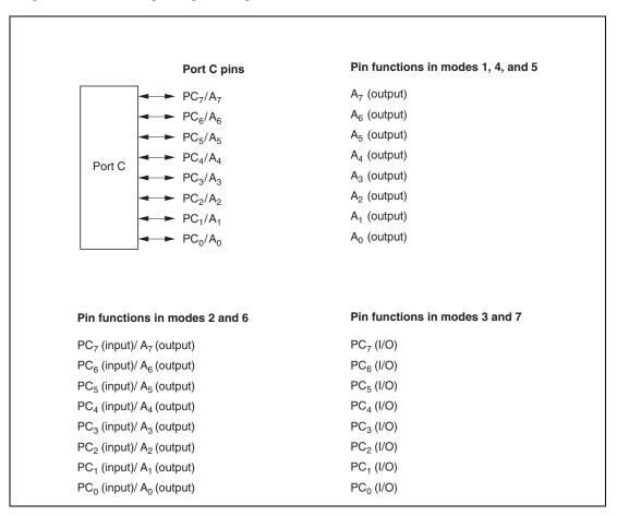
Figure 8.15 Port C Pin Functions
