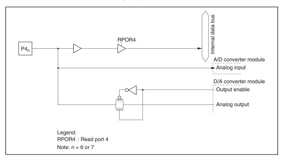
Figure C.4 (b) Port 4 Block Diagram (Pins P4<sub>6</sub> and P4<sub>7</sub> in H8S/2355 and H8S/2353)
