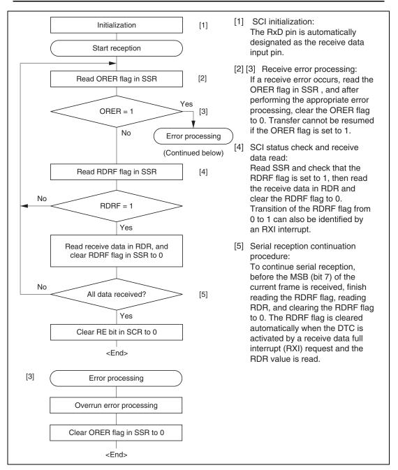
Figure 12.18 Sample Serial Reception Flowchart
