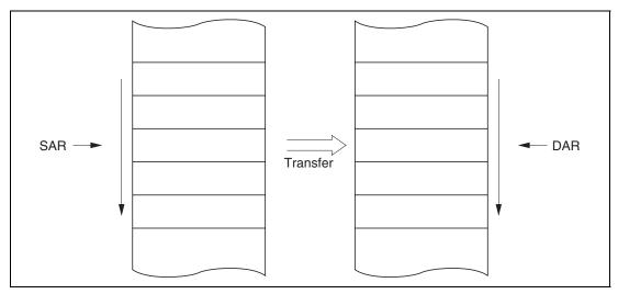
Figure 7.6 Memory Mapping in Normal Mode
