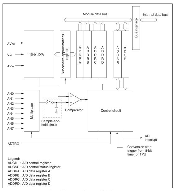
Figure 14.1 Block Diagram of A/D Converter
