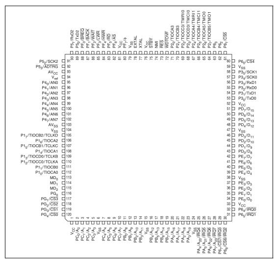
Figure 1.5 H8S/2393 Pin Arrangement (TFP-120: Top View)
