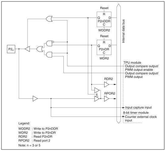
Figure C.2 (c) Port 2 Block Diagram (Pins P2, and P2,
