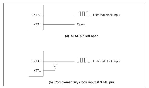
Figure 18.5 External Clock Input (Examples)
