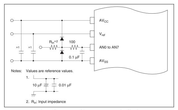
Figure 14.7 Example of Analog Input Protection Circuit
