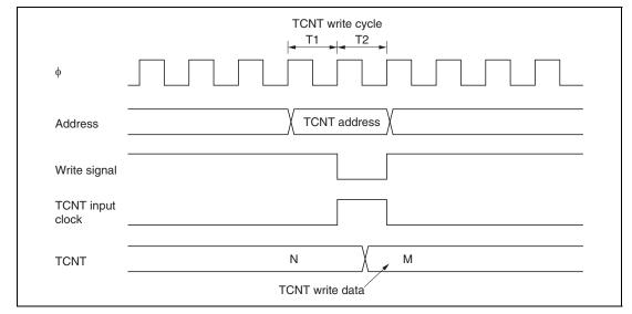
Figure 9.50 Contention between TCNT Write and Increment Operations
