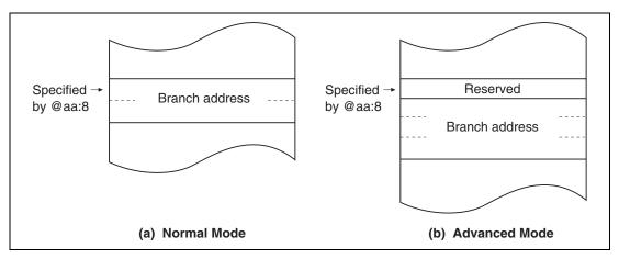
Figure 2.13 Branch Address Specification in Memory Indirect Mode
