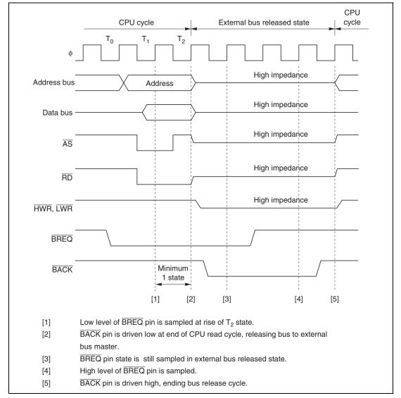
Figure 6.19 Bus-Released State Transition Timing
