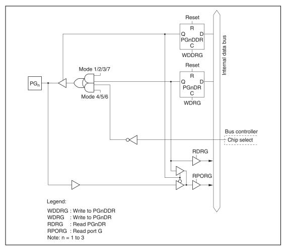
Figure C.13 (b) Port G Block Diagram (Pins PG<sub>1</sub> to PG<sub>3</sub>)
