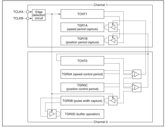
Figure 9.33 Phase Counting Mode Application Example
