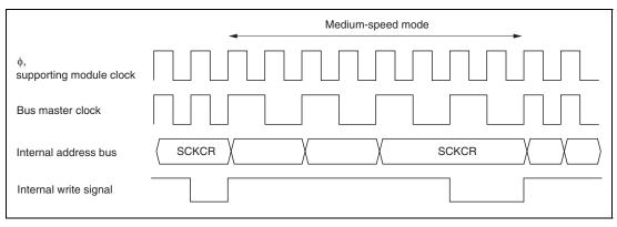
Figure 19.1 Medium-Speed Mode Transition and Clearance Timing
