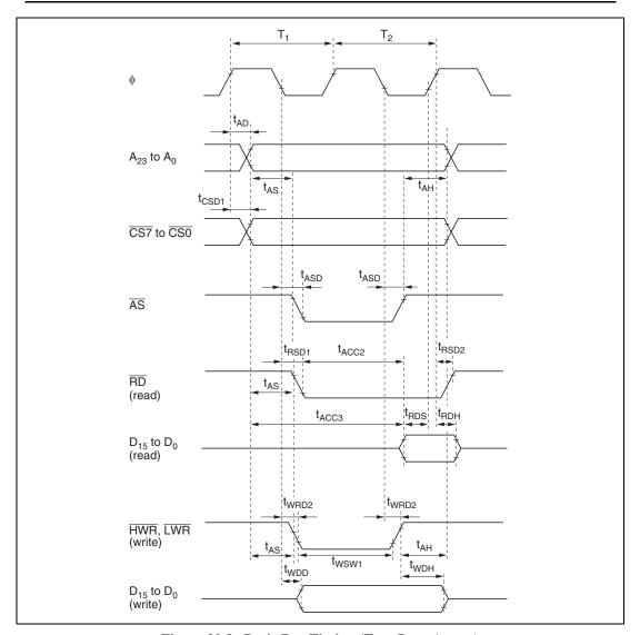
Figure 20.8 Basic Bus Timing (Two-State Access)
