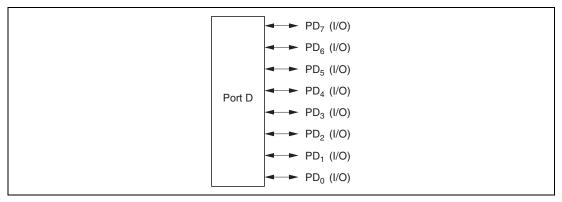
Figure 8.21 Port D Pin Functions (Modes 3 and 7)
