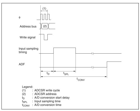
Figure 14.5 A/D Conversion Timing
