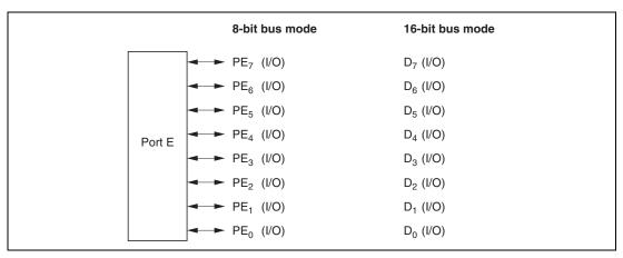
Figure 8.23 Port E Pin Functions (Modes 1, 2, 4, 5, and 6)
