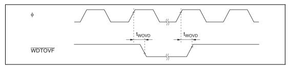
Figure 20.20 WDT Output Timing
