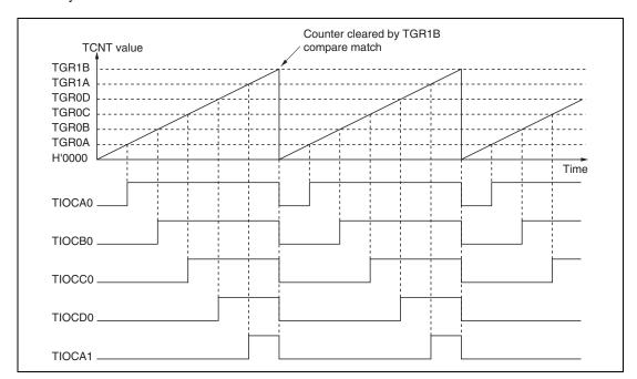
Figure 9.26 Example of PWM Mode Operation (2)
