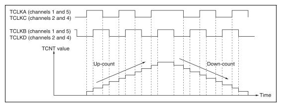
Figure 9.29 Example of Phase Counting Mode 1 Operation
