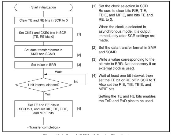
Figure 12.4 Sample SCI Initialization Flowchart
