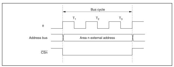
Figure 6.3  $\overline{CSn}$  Signal Output Timing (n = 0 to 7)
