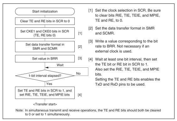
Figure 12.15 Sample SCI Initialization Flowchart
