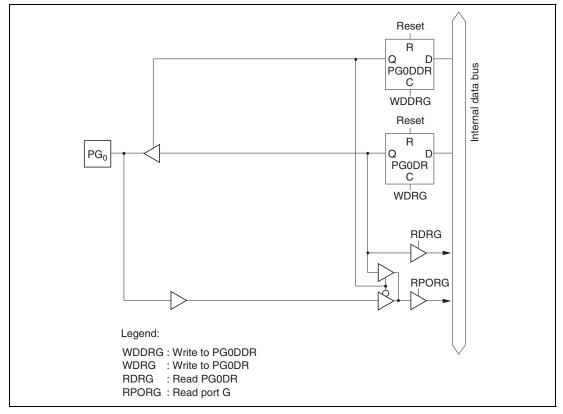
Figure C.13 (a) Port G Block Diagram (Pin  $PG_0$ )
