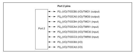
Figure 8.2 Port 2 Pin Functions
