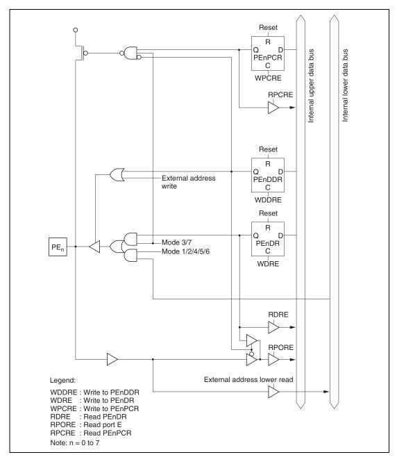
Figure C.11 Port E Block Diagram (Pin PE<sub>n</sub>)
