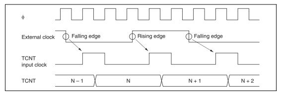
Figure 9.35 Count Timing in External Clock Operation
