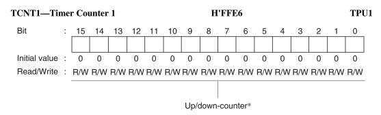
Note: \* This timer counter can be used as an up/down-counter only in phase counting mode or when performing overflow/underflow counting on another channel. In other cases it functions as an up-counter.
