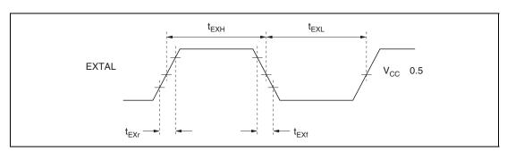
Figure 18.6 External Clock Input Timing
