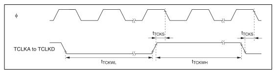
Figure 20.16 TPU Clock Input Timing
