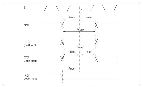
Figure 20.7 Interrupt Input Timing
