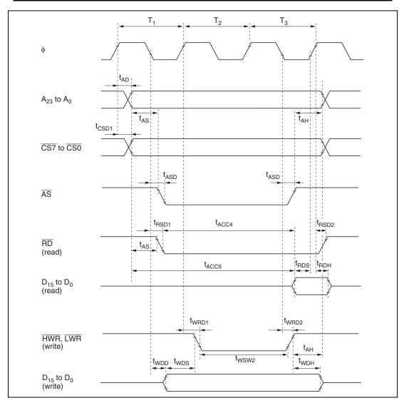
Figure 20.9 Basic Bus Timing (Three-State Access)
