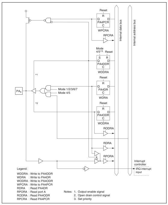
Figure C.7 (b) Port A Block Diagram (Pin PA<sub>4</sub>)
