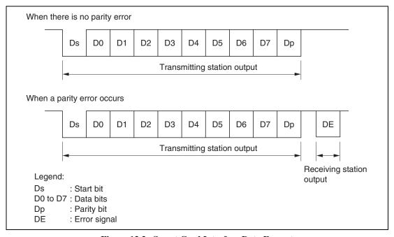
Figure 13.3 Smart Card Interface Data Format
