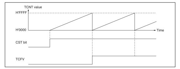
Figure 9.7 Free-Running Counter Operation
