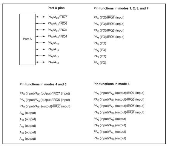
Figure 8.7 Port A Pin Functions
