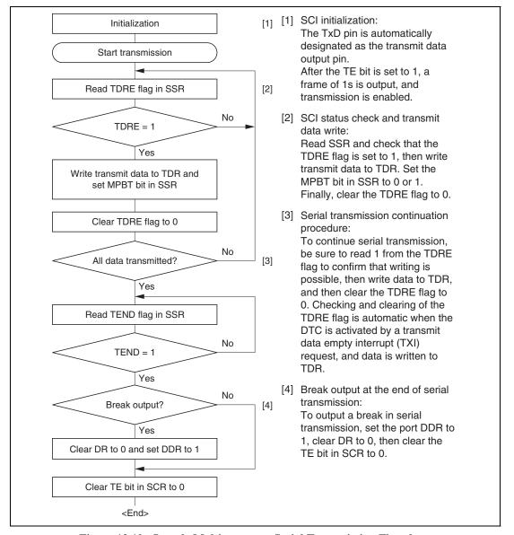
Figure 12.10 Sample Multiprocessor Serial Transmission Flowchart
