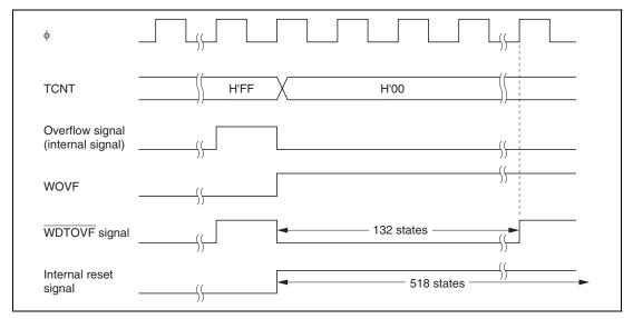
Figure 11.7 Timing of Setting of WOVF
