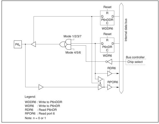
Figure C.6 (a) Port 6 Block Diagram (Pins P6, and P6,)
