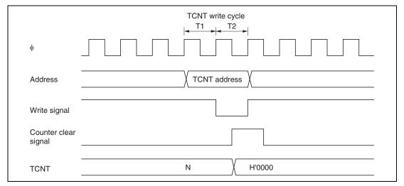
Figure 9.49 Contention between TCNT Write and Clear Operations
