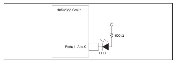
Figure 20.2 LED Drive Circuit (Example)
