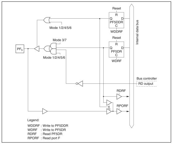
Figure C.12 (f) Port F Block Diagram (Pin PF<sub>5</sub>)
