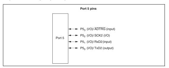
**Figure 8.5 Port 5 Pin Functions**
