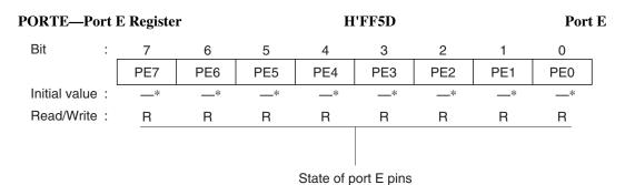
Note: \* Determined by the state of pins PE<sub>7</sub> to PE<sub>0</sub>.
