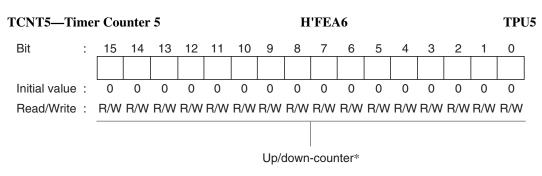
Note: \* This timer counter can be used as an up/down-counter only in phase counting mode or when performing overflow/underflow counting on another channel. In other cases it functions as an up-counter.
