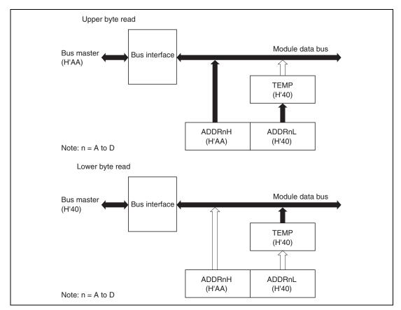
Figure 14.2 ADDR Access Operation (Reading H'AA40)
