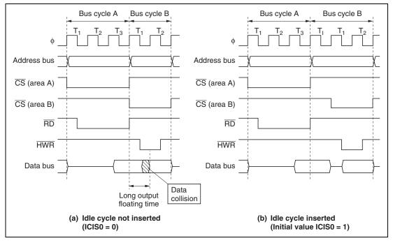
Figure 6.17 Example of Idle Cycle Operation (2)
