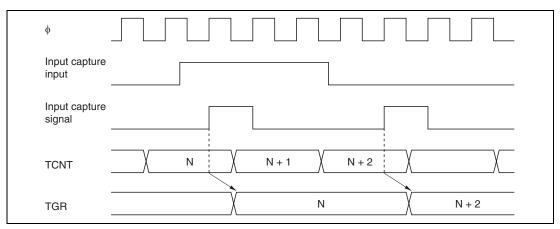
Figure 9.37 Input Capture Input Signal Timing
