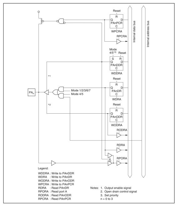
Figure C.7 (a) Port A Block Diagram (Pins PA, to PA,)
