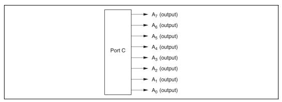
Figure 8.16 Port C Pin Functions (Modes 1, 4, and 5)
