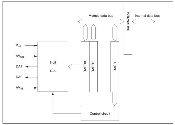
Figure 15.1 Block Diagram of D/A Converter
