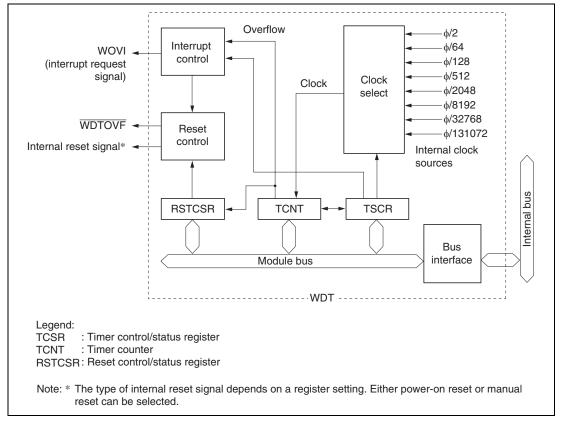
Figure 11.1 Block Diagram of WDT
