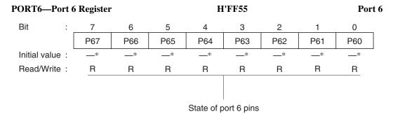
Note: \* Determined by the state of pins  $P6_7$  to  $P6_0$ .
