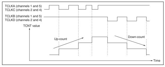
Figure 9.31 Example of Phase Counting Mode 3 Operation
