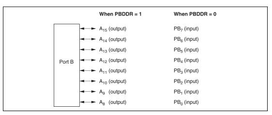
Figure 8.13 Port B Pin Functions (Modes 2 and 6)
