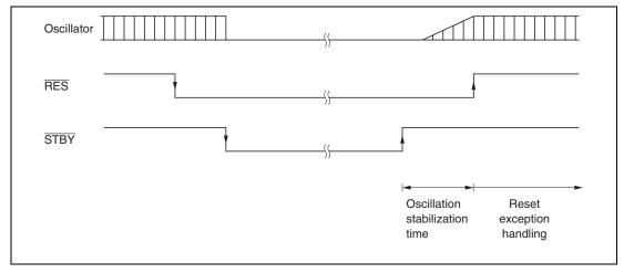
Figure 19.3 Hardware Standby Mode Timing (Example)
