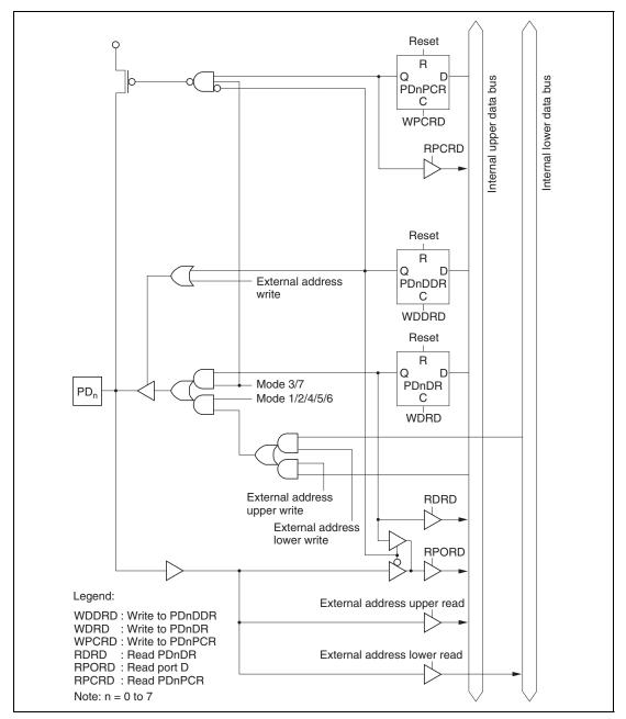
Figure C.10 Port D Block Diagram (Pin PD<sub>n</sub>)
