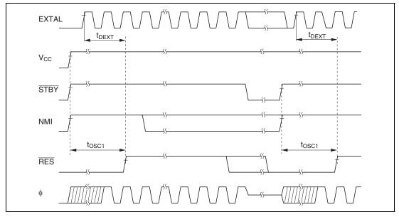
Figure 20.5 Oscillator Settling Timing
