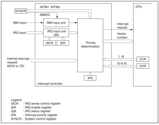
Figure 5.1 Block Diagram of Interrupt Controller
