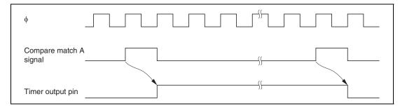
Figure 10.5 Timing of Timer Output
