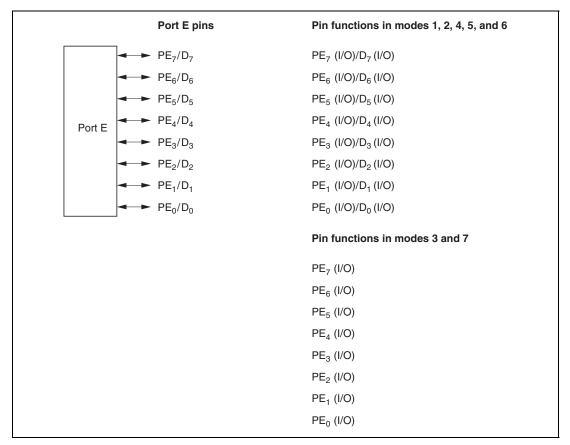
Figure 8.22 Port E Pin Functions
