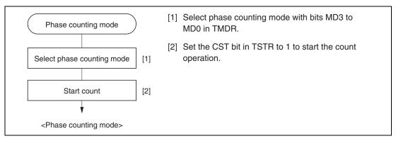
Figure 9.28 Example of Phase Counting Mode Setting Procedure
