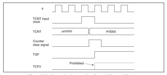
Figure 9.56 Contention between Overflow and Counter Clearing
