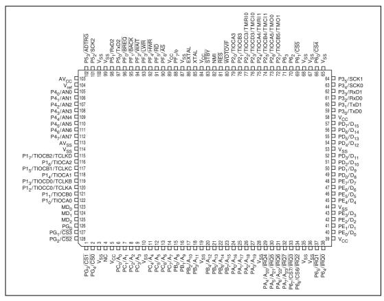
Figure 1.6 H8S/2393 Pin Arrangement (FP-128: Top View)
