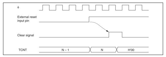
Figure 10.7 Timing of External Reset
