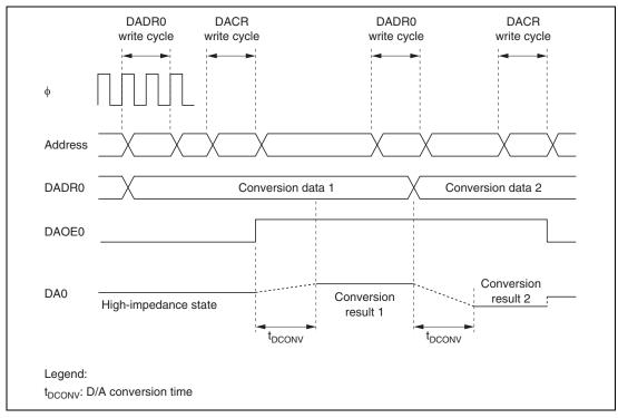
Figure 15.2 Example of D/A Converter Operation
