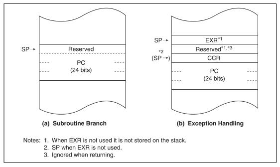
Figure 2.5 Stack Structure in Advanced Mode
