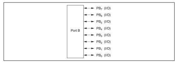
Figure 8.14 Port B Pin Functions (Modes 3 and 7)
