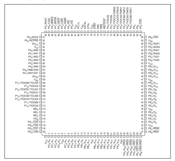
Figure 1.3 H8S/2355 and H8S/2353 Pin Arrangement (TFP-120: Top View)
