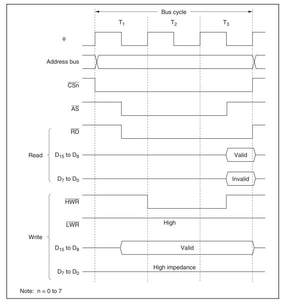
Figure 6.7 Bus Timing for 8-Bit 3-State Access Space
