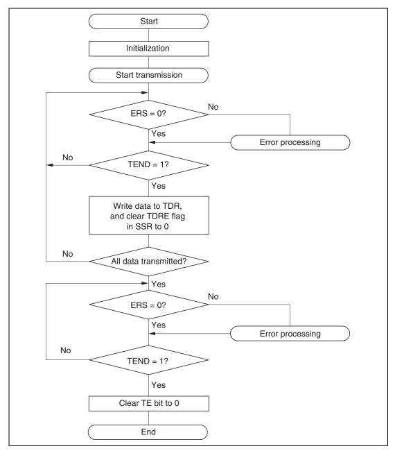
Figure 13.4 Example of Transmission Processing Flow
