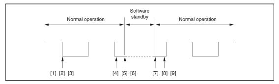
Figure 13.9 Clock Halt and Restart Procedure
