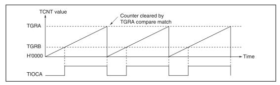
Figure 9.25 Example of PWM Mode Operation (1)
