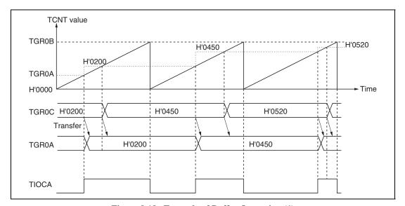
Figure 9.19 Example of Buffer Operation (1)
