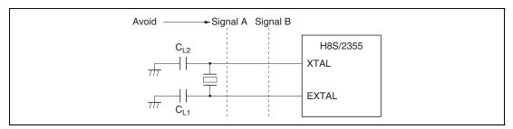
Figure 18.4 Example of Incorrect Board Design
