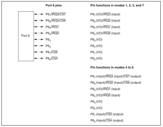
Figure 8.6 Port 6 Pin Functions
