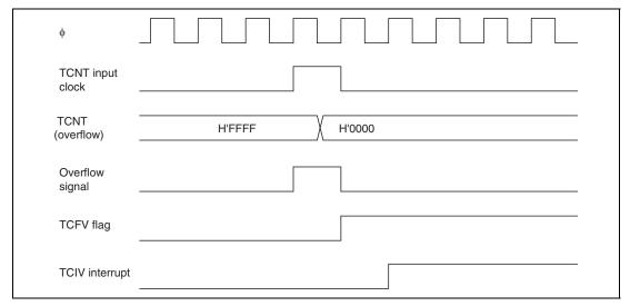
Figure 9.44 TCIV Interrupt Setting Timing
