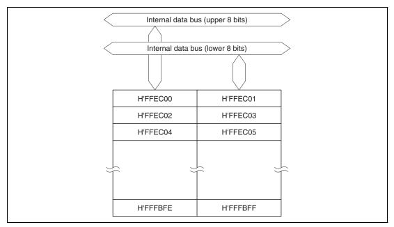
Figure 16.1 Block Diagram of RAM (H8S/2355)
