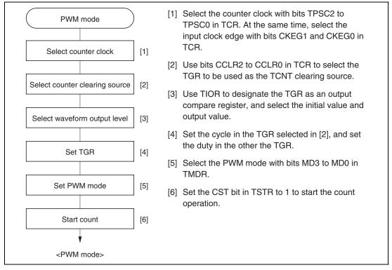
Figure 9.24 Example of PWM Mode Setting Procedure
