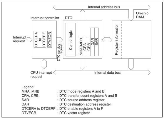
Figure 7.1 Block Diagram of DTC
