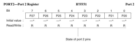
Note: \* Determined by the state of pins P2<sub>7</sub> to P2<sub>0</sub>.
