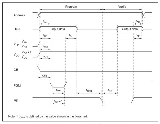
Figure 17.5 PROM Programming/Verification Timing
