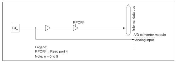
Figure C.4 (a) Port 4 Block Diagram (Pins  $P4_0$  to  $P4_5$  in H8S/2355 and H8S/2353, Pins  $P4_0$  to  $P4_7$  in H8S/2393)
