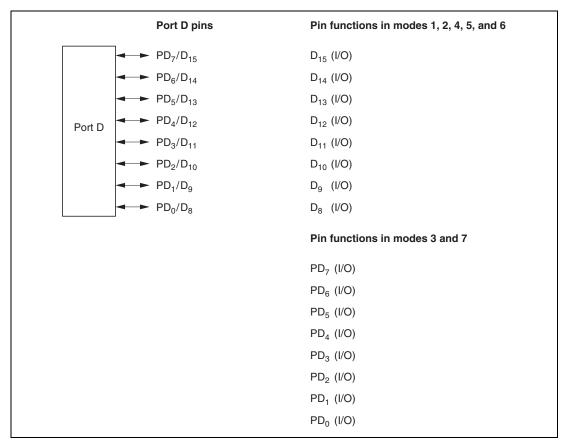
**Figure 8.19 Port D Pin Functions**
