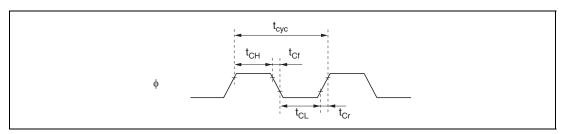
Figure 20.4 System Clock Timing
