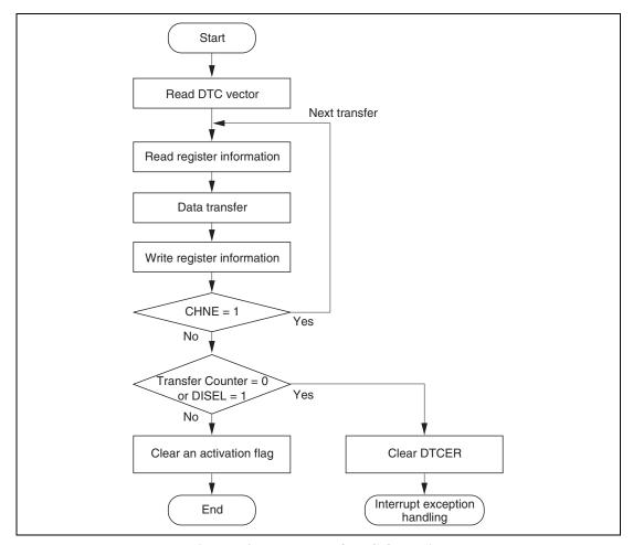
Figure 7.2 Flowchart of DTC Operation
