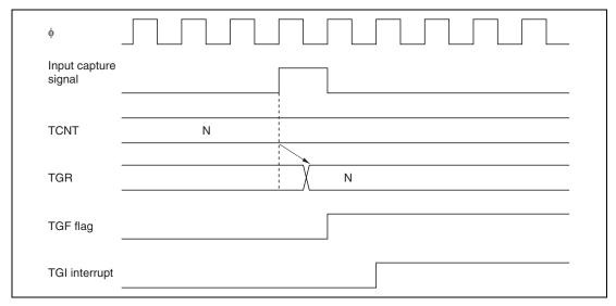
**Figure 9.43 TGI Interrupt Timing (Input Capture)**
