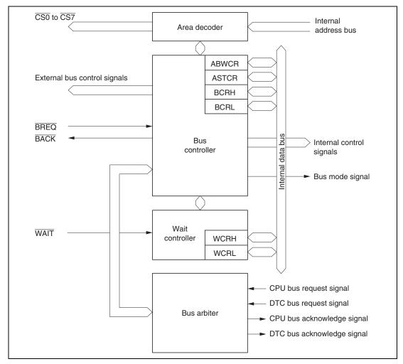
Figure 6.1 Block Diagram of Bus Controller
