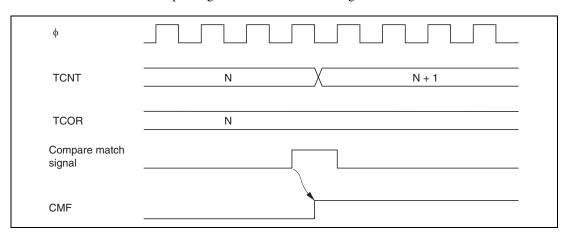
Figure 10.4 Timing of CMF Setting
