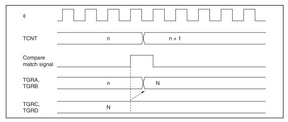
**Figure 9.40 Buffer Operation Timing (Compare Match)**
