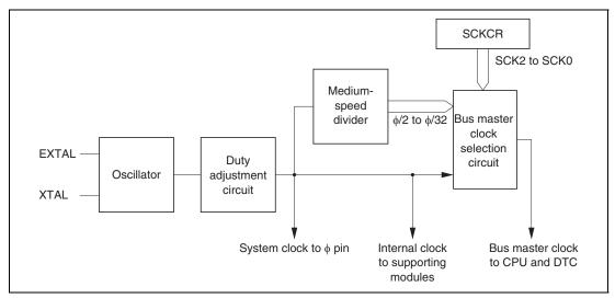
Figure 18.1 Block Diagram of Clock Pulse Generator
