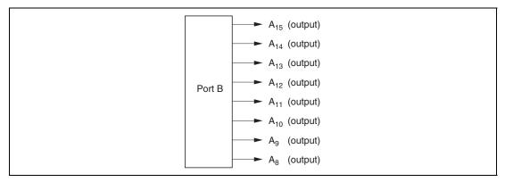
Figure 8.12 Port B Pin Functions (Modes 1, 4, and 5)
