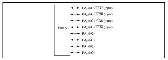
Figure 8.8 Port A Pin Functions (Modes 1, 2, 3, and 7)
