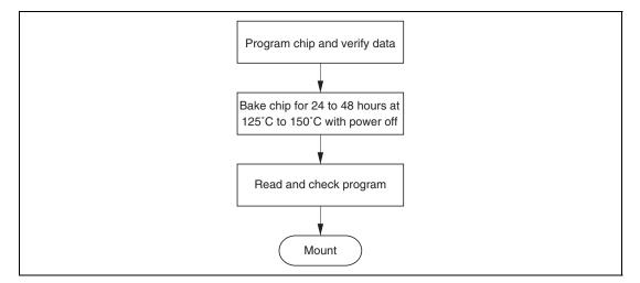
Figure 17.6 Recommended Screening Procedure
