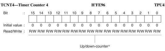
Note: \* This timer counter can be used as an up/down-counter only in phase counting mode or when performing overflow/underflow counting on another channel. In other cases it functions as an up-counter.
