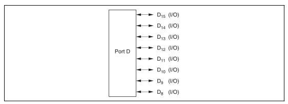
Figure 8.20 Port D Pin Functions (Modes 1, 2, 4, 5, and 6)
