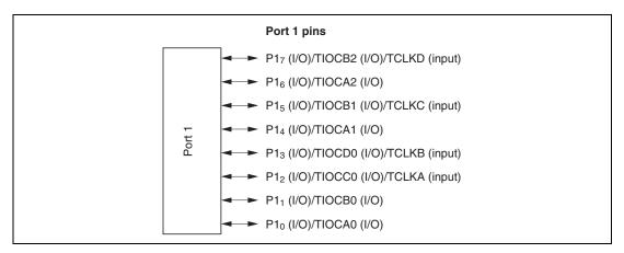
Figure 8.1 Port 1 Pin Functions
