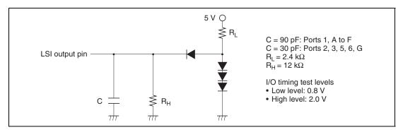
Figure 20.3 Output Load Circuit
