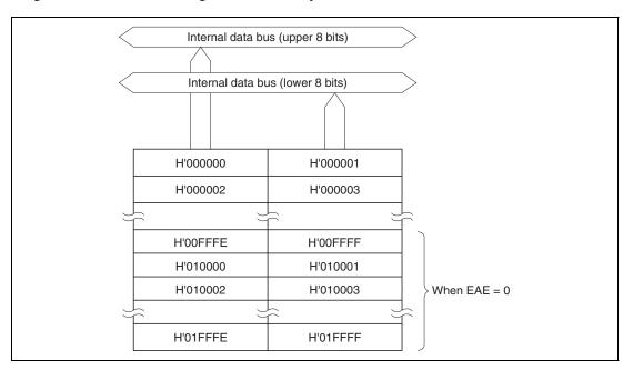
Figure 17.1 Block Diagram of ROM (H8S/2355)
