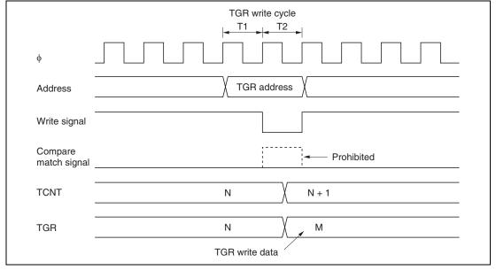
Figure 9.51 Contention between TGR Write and Compare Match
