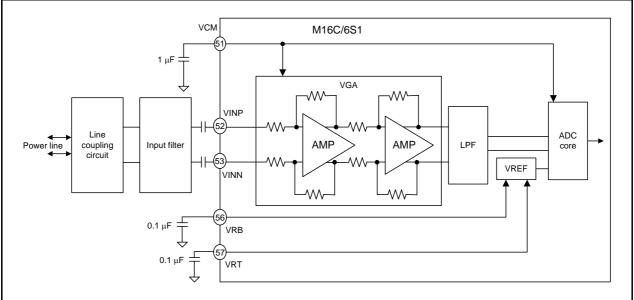
Figure 26.7 AFE Receiver Analog Circuit
