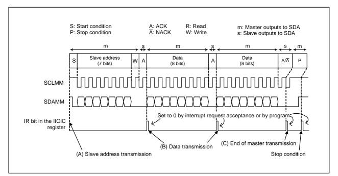
Figure 21.17 Example of Master Transmission
