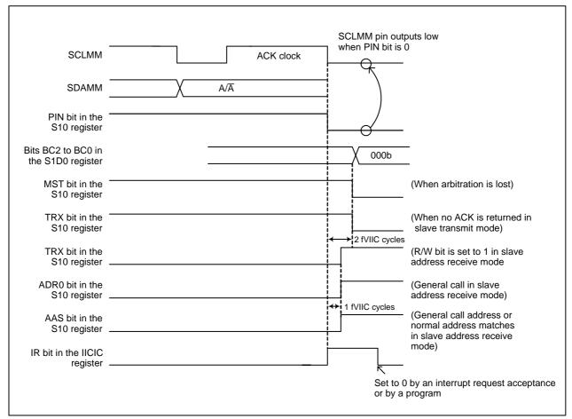
Figure 21.15 Operation After Transmitting/Receiving a Slave Address or Data
