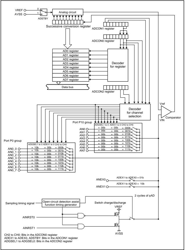
Figure 22.1 A/D Converter Block Diagram
