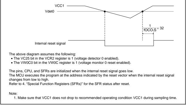
Figure 7.3 Voltage Monitor 0 Reset Operation Example
