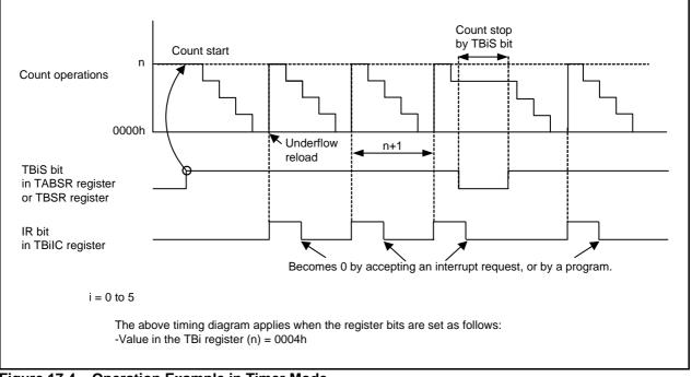
Figure 17.4 Operation Example in Timer Mode
