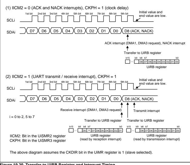
Figure 19.20 Transfer to UiRB Register and Interrupt Timing
