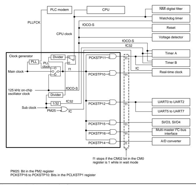
Figure 8.5 Peripheral Function Clocks
