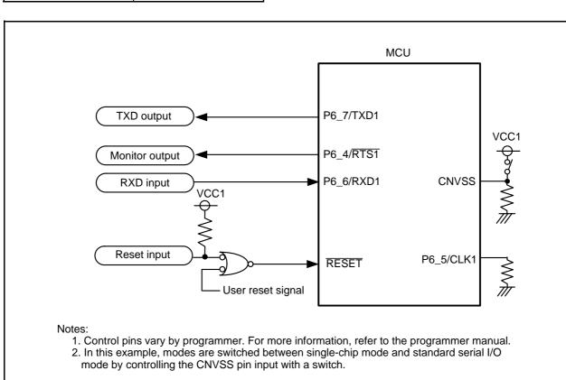
Figure 24.28 Circuit Application in Standard Serial I/O Mode 2
