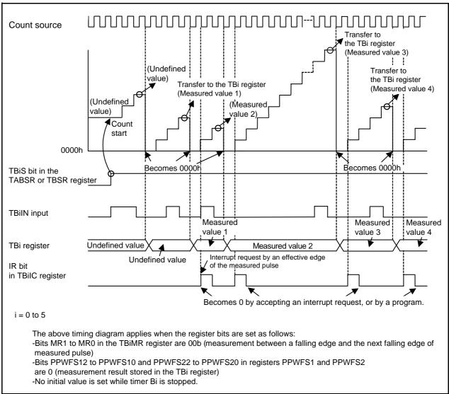
Figure 17.6 Operation Example in Pulse Period Measurement Mode
