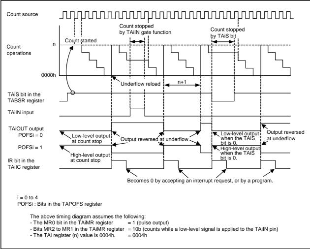
Figure 16.5 Operation Example in Timer Mode
