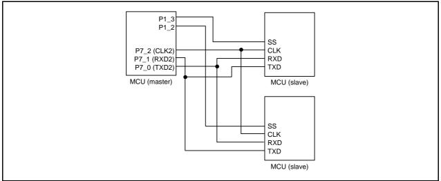
Figure 19.32 Serial Bus Communication Control Example (UART2)
