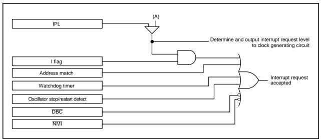
Figure 13.9 Interrupt Priority Select Circuit 2
