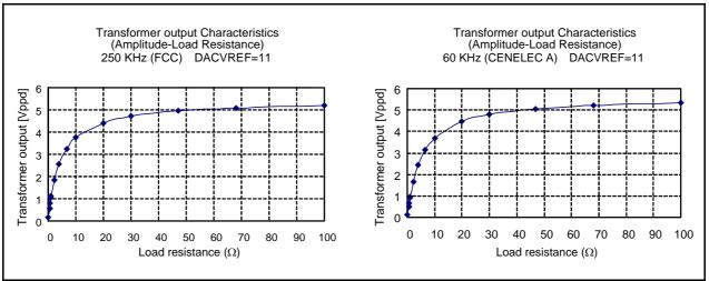
Figure 26.5 Line Driver Transfer R-V Typical Characteristics (Measuring Condition: Rout = 1  $\Omega$  as in Figure 26.3)
