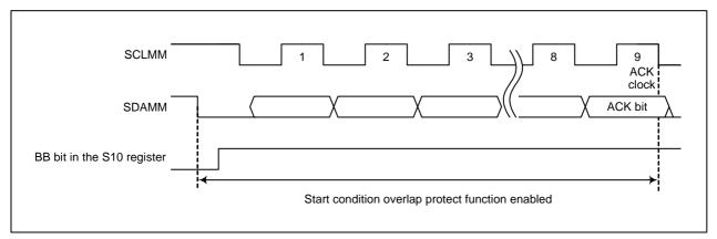
Figure 21.11 Start Condition Overlap Protect Function Enable Period
