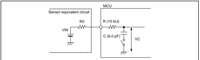
Figure 22.16 Analog Input Pin and External Sensor Equivalent Circuit
