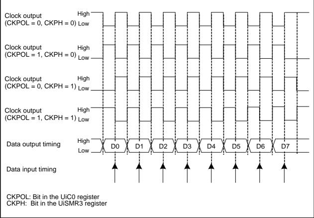
Figure 19.33 Transmit/Receive Timing in Master Mode (Internal Clock)
