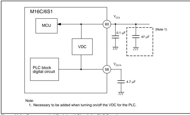
Figure 26.9 Recommended Peripheral Circuit for PLC Regulator
