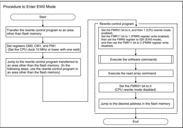
Figure 24.16 Setting and Resetting of EW0 Mode
