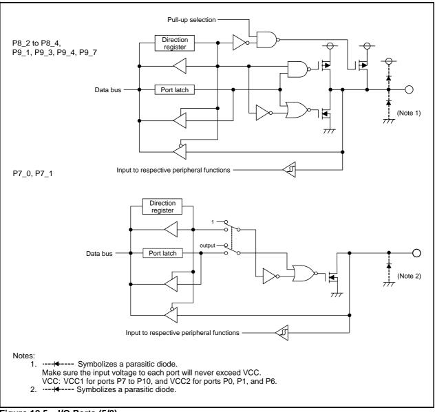
Figure 12.5 I/O Ports (5/8)
