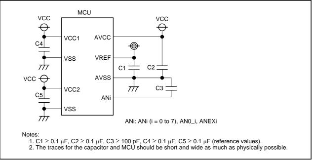
Figure 22.17 Example of Pin Configuration
