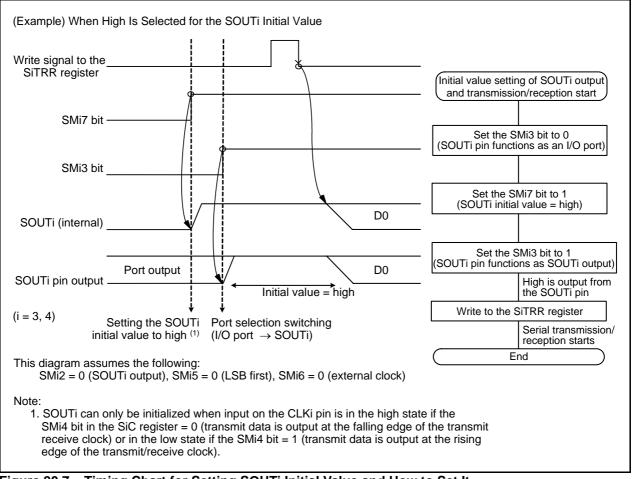
Figure 20.7 Timing Chart for Setting SOUTi Initial Value and How to Set It
