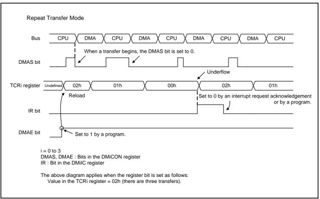
Figure 15.4 Operation Example in Repeat Transfer Mode
