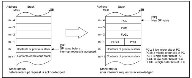
Figure 13.5 Stack Status Before and After Acceptance of Interrupt Request
