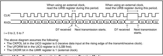
Figure 19.8 Operation Example in Continuous Receive Mode
