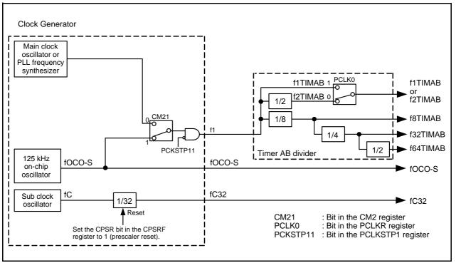
Figure 16.1 Timer A and B Count Sources
