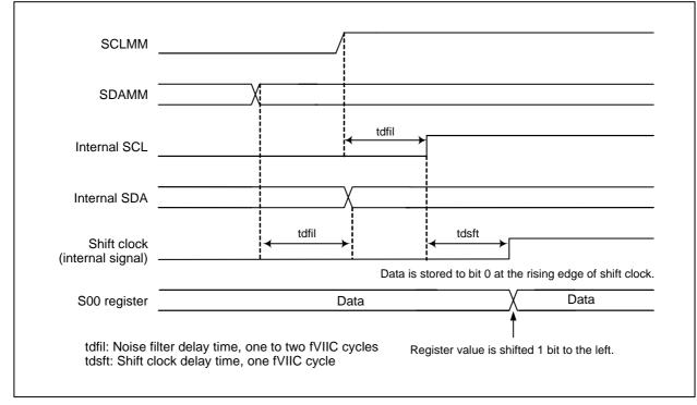
Figure 21.2 Timing to Store Received Data to the S00 Register
