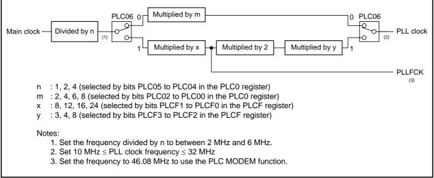
Figure 8.3 Relation between Main Clock and PLL Clock
