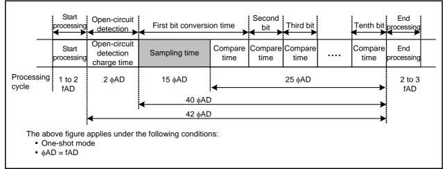
Figure 22.3 A/D Conversion Timing
