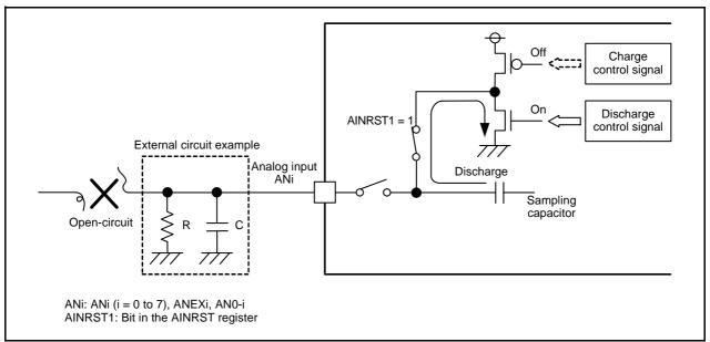
Figure 22.8 A/D Open-Circuit Detection Example on AVSS (Preconversion Discharge)
