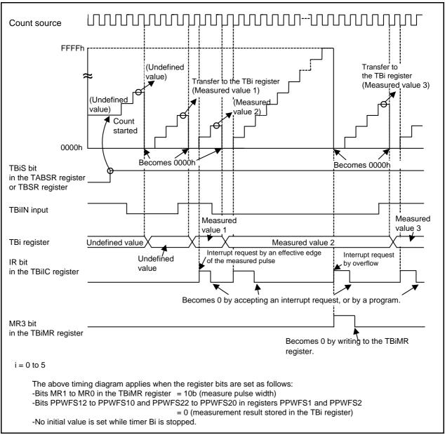
Figure 17.7 Operation Example in Pulse Width Measurement Mode
