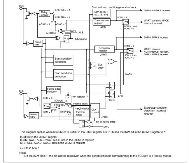
Figure 19.18 I<sup>2</sup>C Mode Block Diagram
