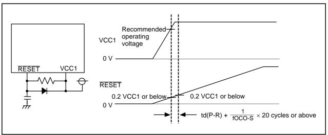
Figure 6.4 Reset Circuit Example
