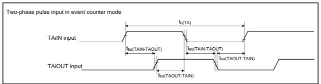
Figure 27.6 Timer A Input (Two-Phase Pulse Input in Event Counter Mode)
