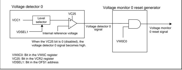
Figure 7.2 Voltage Monitor 0 Reset Generator Block Diagram
