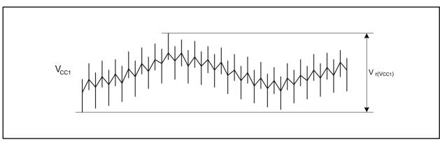
Figure 27.1 Ripple Waveform
