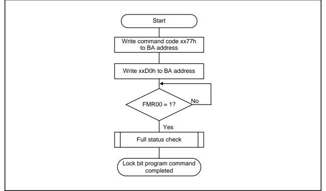
Figure 24.12 Lock Bit Program Command (Suspend Function Disabled)
