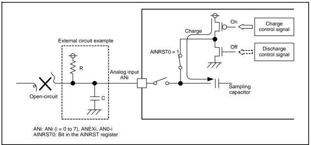
Figure 22.6 A/D Open-Circuit Detection Example on AVCC (Preconversion Charge)
