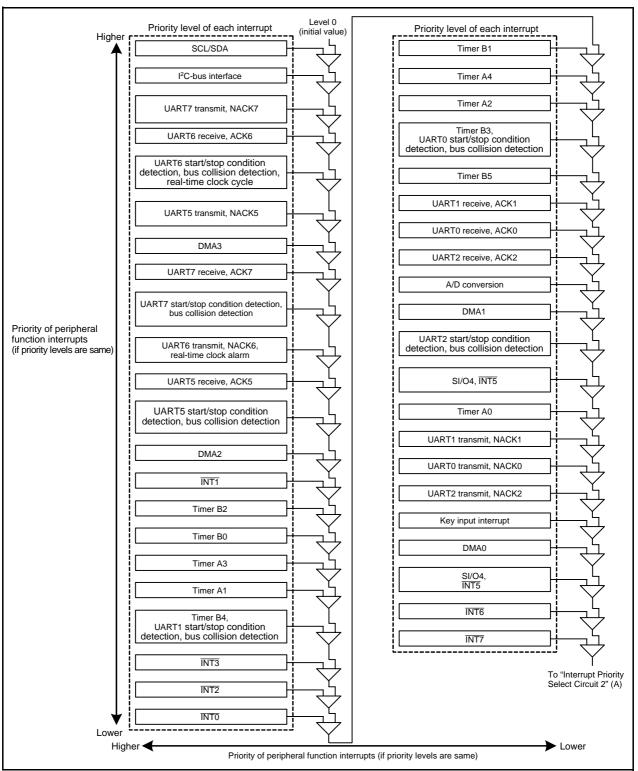
Figure 13.8 Interrupt Priority Select Circuit 1
