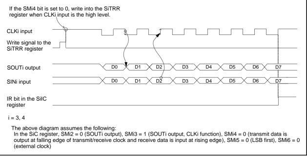
Figure 20.6 SI/Oi Operation Timing (External Clock)
