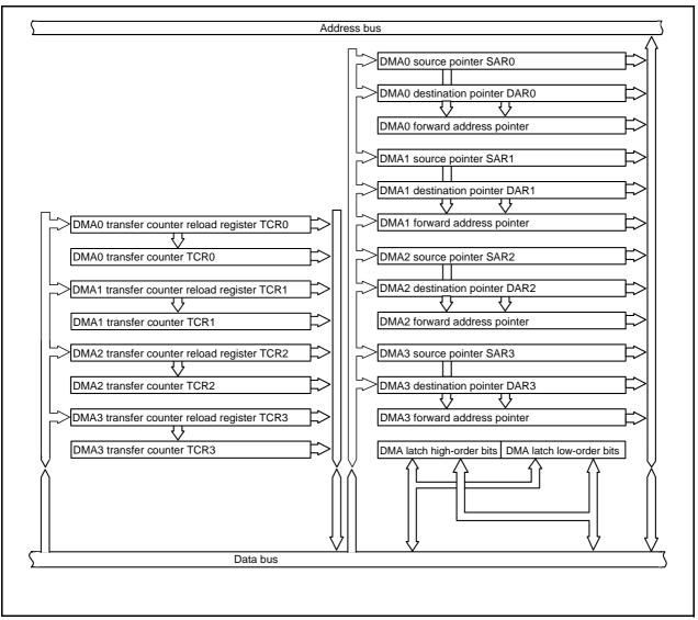
Figure 15.1 DMAC Block Diagram
