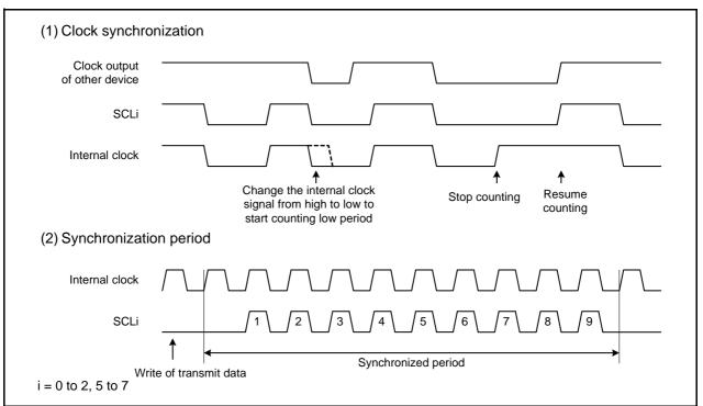
Figure 19.25 Clock Synchronization
