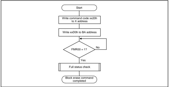
Figure 24.11 Block Erase Command (Suspend Function Disabled)
