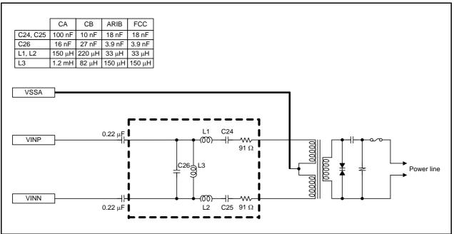
Figure 26.8 Recommended Input Filter
