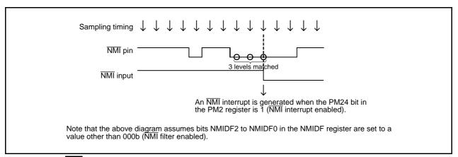
Figure 12.11 NMI Digital Filter Operation Example
