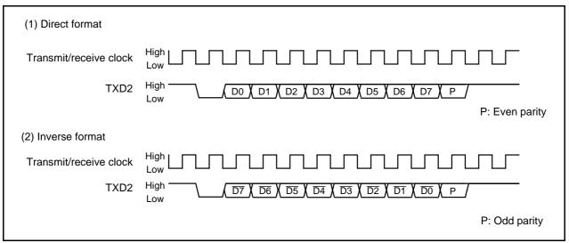
Figure 19.38 SIM Interface Format
