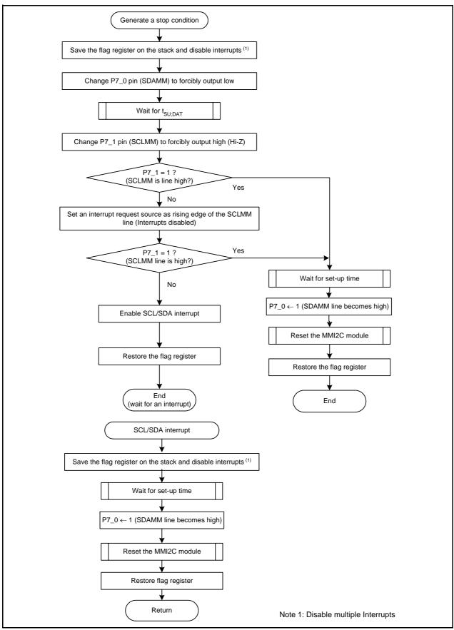
Figure 28.12 Generating a Stop Condition
