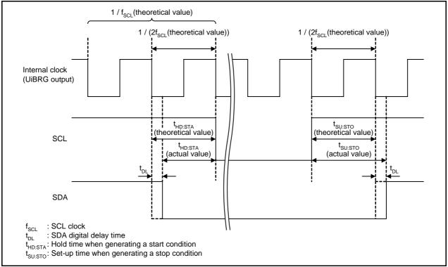
Figure 28.10 Setup and Hold Times When Generating Start and Stop Conditions
