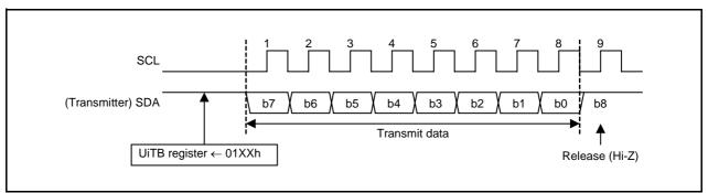
Figure 19.28 Byte Data Transmission
