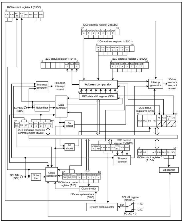
Figure 21.1 Multi-master I<sup>2</sup>C-bus Interface Block Diagram
