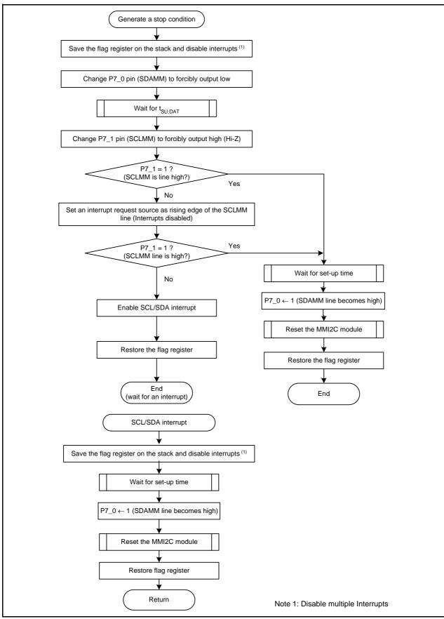
Figure 21.23 Generating a Stop Condition
