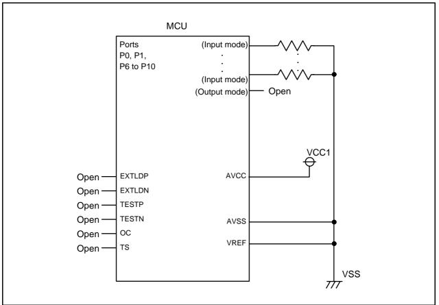
Figure 12.12 Unassigned Pin Handling
