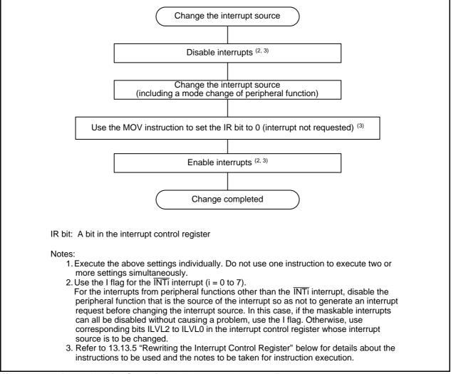
Figure 28.8 Procedure for Changing the Interrupt Generate Factor
