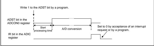
Figure 28.14 ADST Bit Operation
