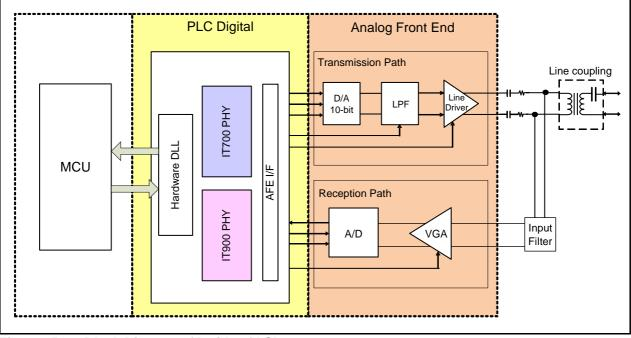
Figure 25.1 Block Diagram of Inside of LSI
