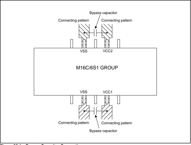
Figure 28.1 Bypass Capacitor Connection
