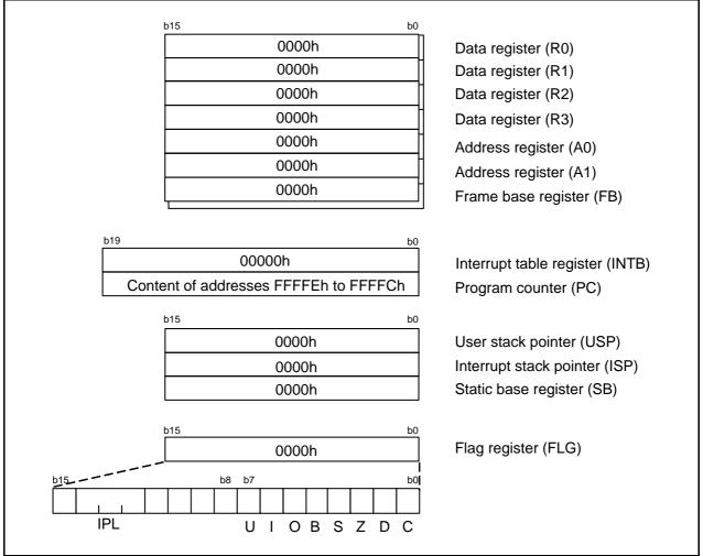
Figure 6.2 CPU Register Status after Reset
