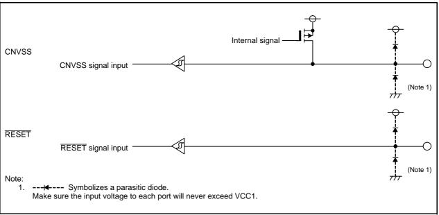
Figure 12.9 I/O Pins
