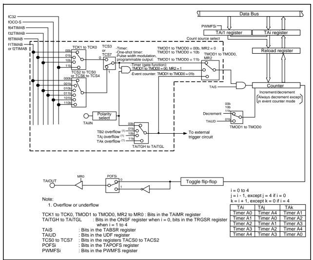
Figure 16.3 Timer A Block Diagram
