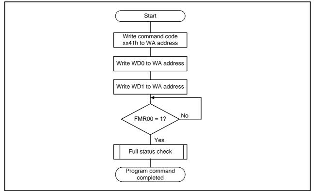
Figure 24.9 EW0 Mode Program Command (Suspend Function Disabled)
