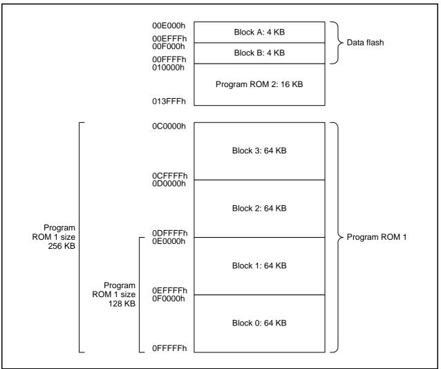
Figure 24.1 Flash Memory Block Diagram
