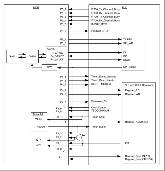
Figure 25.2 Connection between PLC modem Core and MCU
