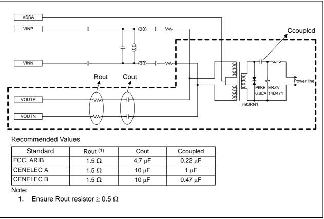
A recommended peripheral circuit for the transmitter is shown in Figure 26.3.
