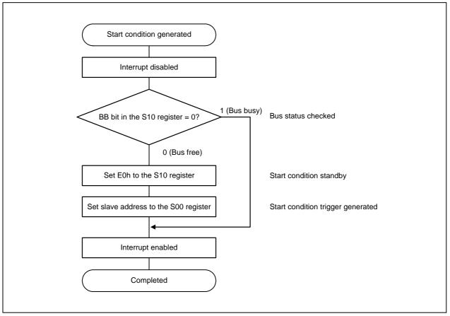
Figure 21.6 Procedure to Generate a Start Condition
