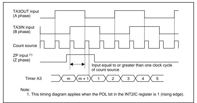
Figure 16.9 Relationship between the Two-Phase Pulse (A-Phase and B-Phase) and the Z-Phase
