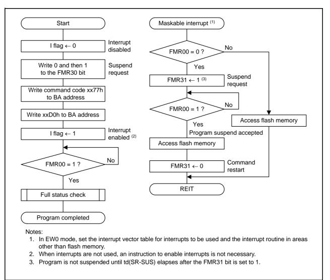
Figure 24.19 Lock Bit Program Flowchart in EW0 Mode (Suspend Function Enabled)
