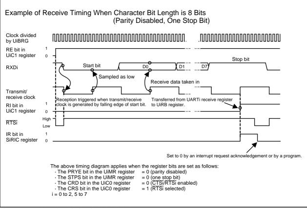
Figure 19.13 Receive Timing in UART Mode
