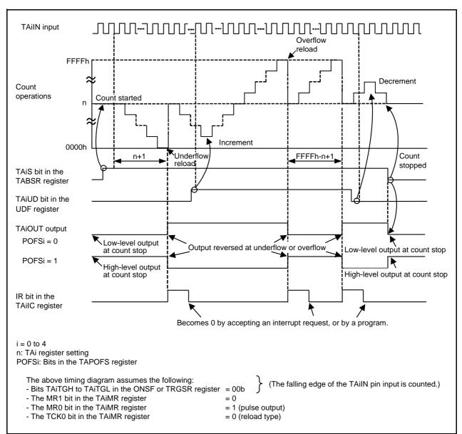
Figure 16.6 Operation Example in Event Counter Mode
