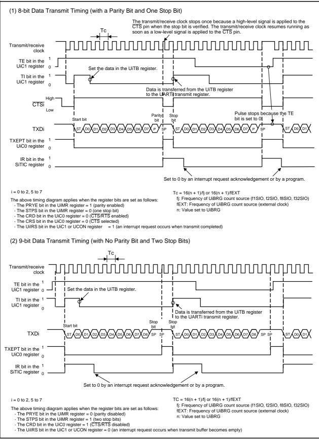
Figure 19.12 Transmit Timing in UART Mode
