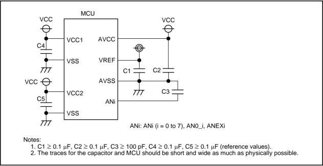
Figure 28.13 Example of Pin Configuration
