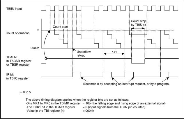
Figure 17.5 Operation Example in Event Counter Mode
