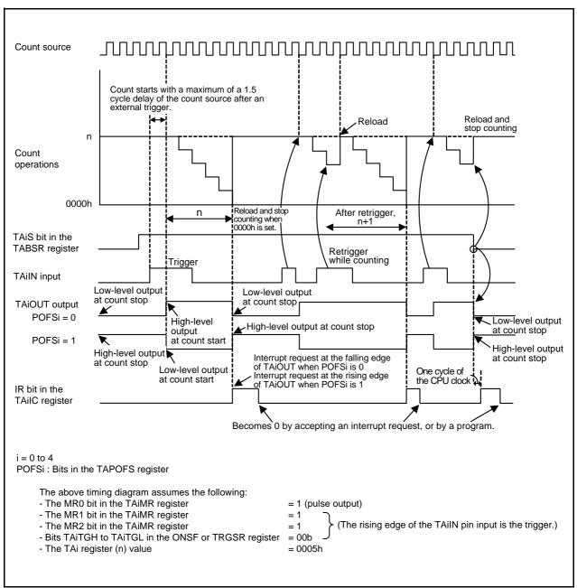
Figure 16.10 Operation Example in One-Shot Timer Mode
