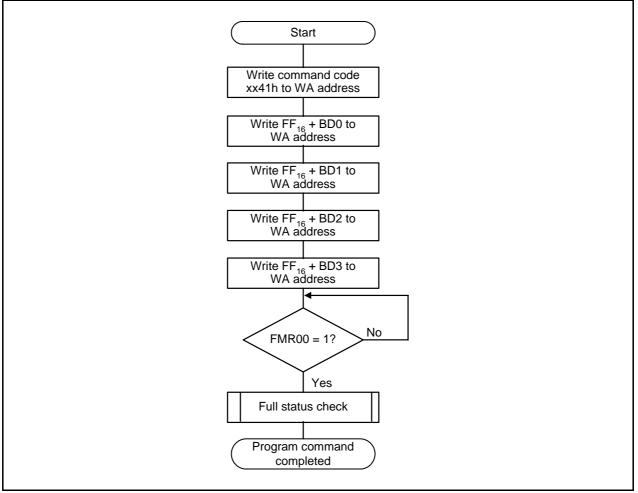
Figure 24.10 EW1 Mode Program Command (Suspend Function Disabled)
