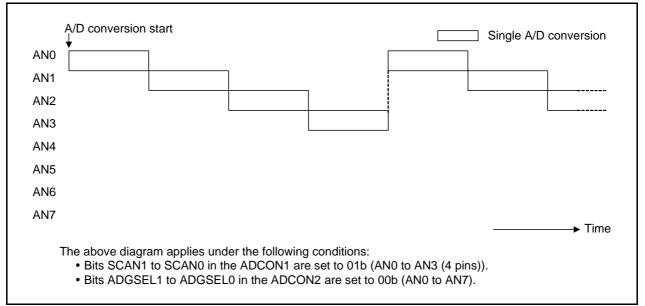
Figure 22.13 Operation Example in Repeat Sweep Mode 0
