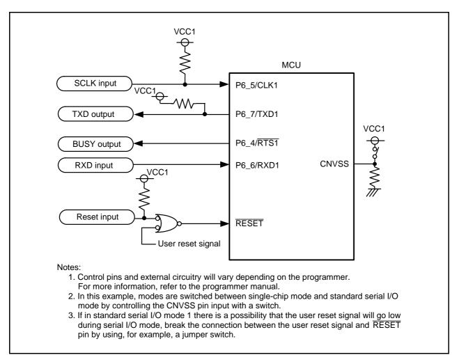
Figure 24.27 Circuit Application in Standard Serial I/O Mode 1
