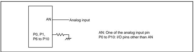
Figure 27.2 A/D Accuracy Measure Circuit
