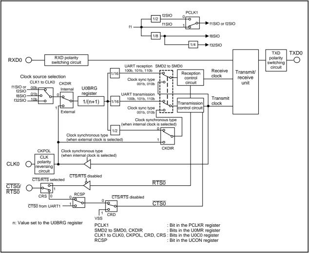
Figure 19.1 UART0 Block Diagram
