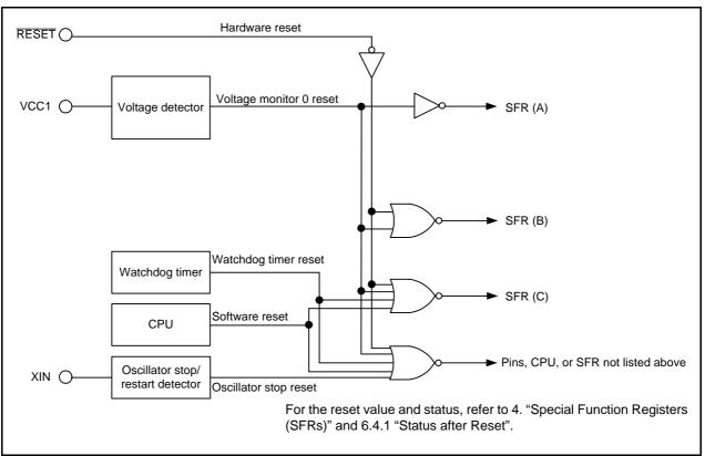
Figure 6.1 Reset Circuit Block Diagram
