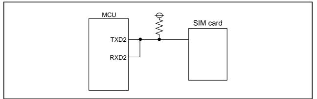
Figure 19.36 Example of SIM Interface Connection
