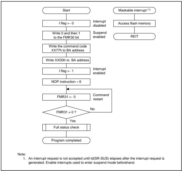
Figure 24.24 Lock Bit Program Flowchart in EW1 Mode (Suspend Function Enabled)
