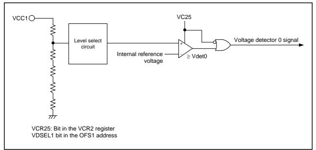
Figure 7.1 Voltage Detector Block Diagram
