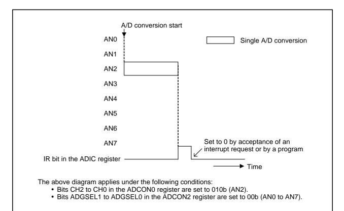
Figure 22.10 Operation Example in One-Shot Mode
