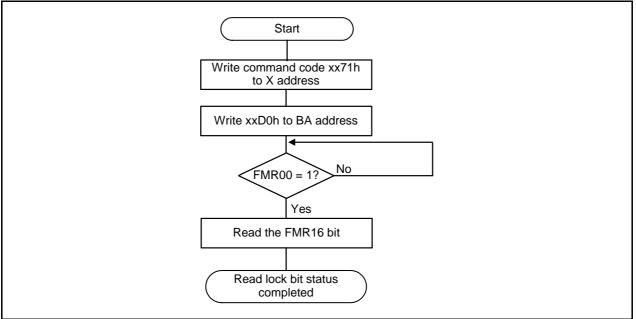
Figure 24.13 Read Lock Bit Status Command
