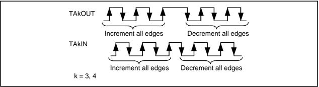
Figure 16.8 Multiply-by-4 Processing
