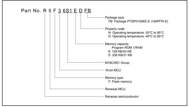
Figure 1.1 Part No., with Memory Size and Package
