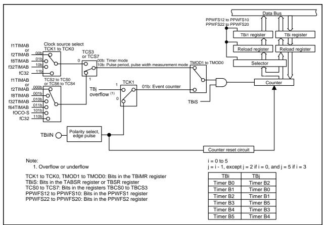
Figure 17.3 Timer B Block Diagram
