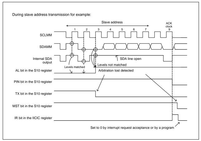
Figure 21.12 Operation Example When Arbitration Lost is Detected
