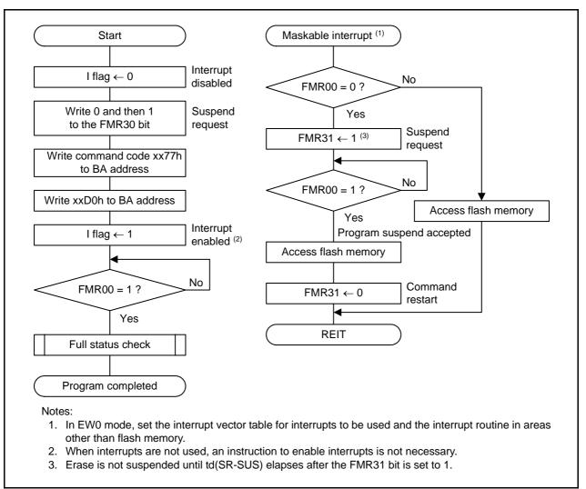
Figure 24.18 Block Erase Flowchart in EW0 Mode (Suspend Function Enabled)
