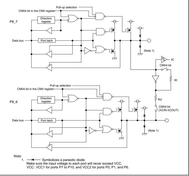
Figure 12.8 I/O Ports (8/8)
