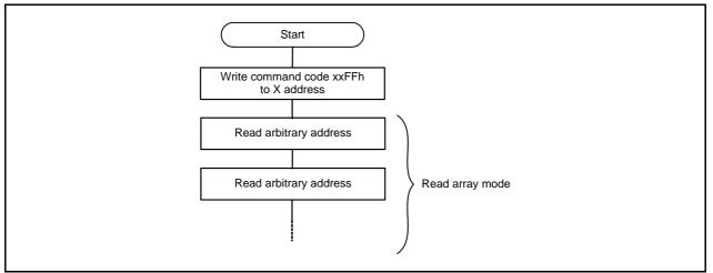
Figure 24.6 Read Array Command
