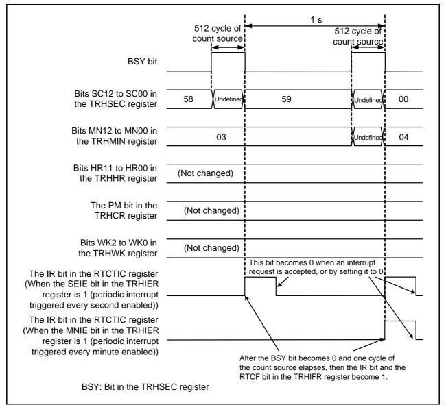
Figure 18.3 Real-Time Clock Basic Operating Example
