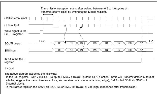
Figure 20.4 shows SI/Oi Operation Timing (Internal Clock).
