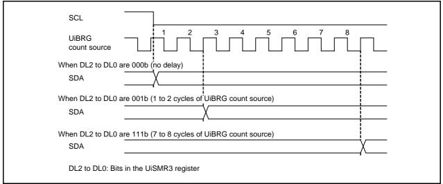
Figure 19.29 SDA Output Selection by Setting Bits DL2 to DL0
