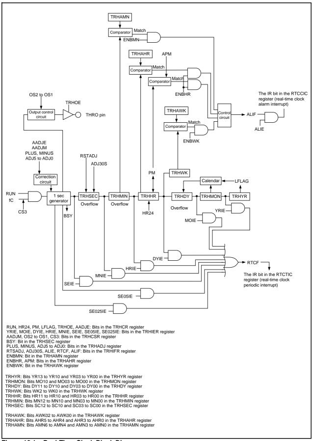
Figure 18.1 Real-Time Clock Block Diagram
