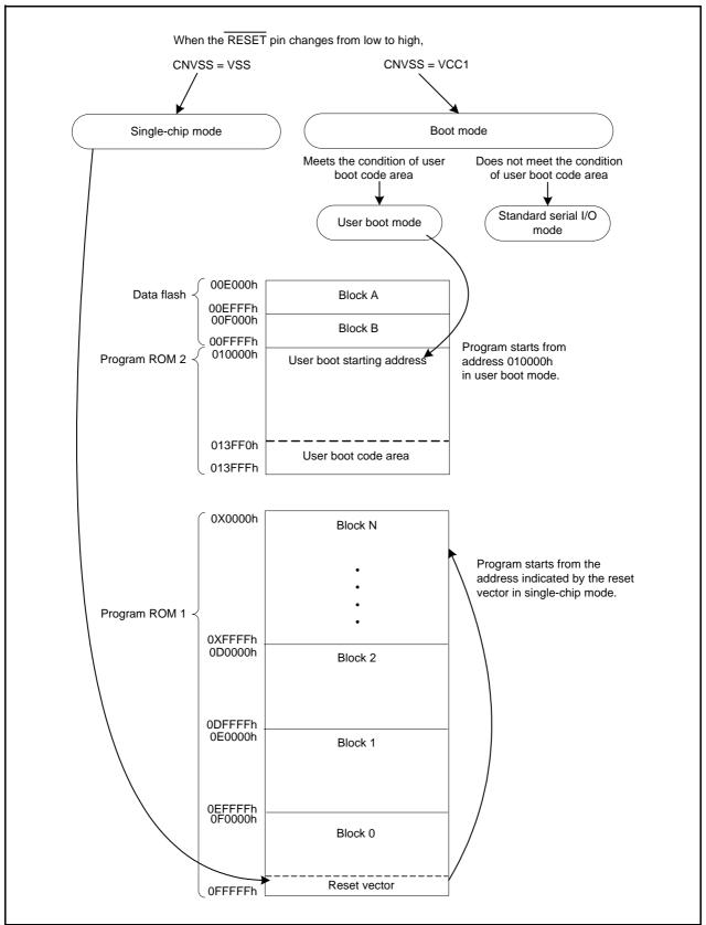
Figure 24.4 Program Starting Address in User Boot Mode
