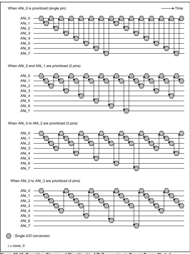
Figure 22.15 Transition Diagram of Pins Used in A/D Conversion in Repeat Sweep Mode 1
