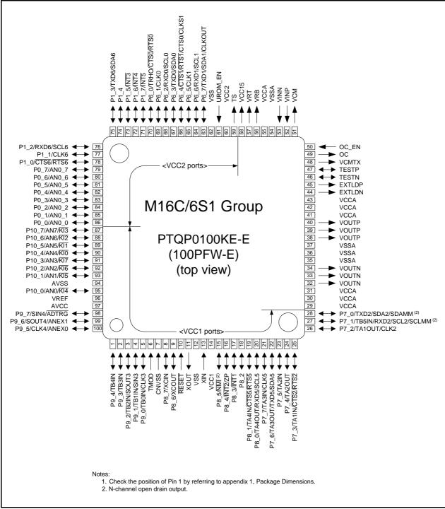
Figure 1.3 Pin Assignment (Top View)
