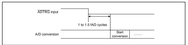
Figure 22.5 A/D conversion Start Timing When External Trigger Input
