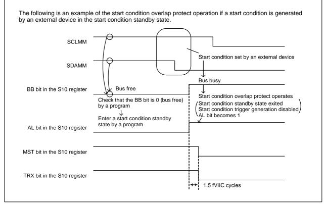
Figure 21.10 Start Condition Overlap Protect Operation
