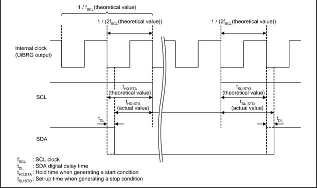
Figure 19.39 Setup and Hold Times When Generating Start and Stop Conditions
