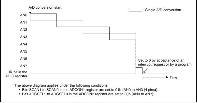
Figure 22.12 Operation Example in Single Sweep Mode
