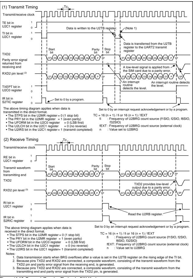
Figure 19.35 Transmit/Receive Timing in SIM Mode
