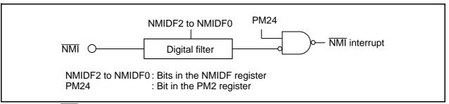
Figure 13.10 NMI Interrupt Block Diagram
