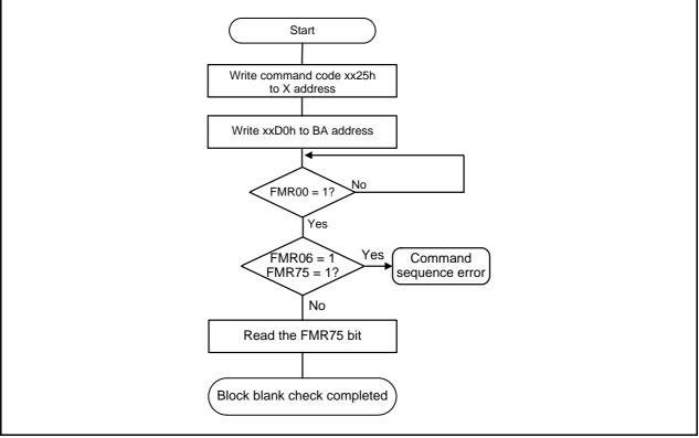
Figure 24.14 Block Blank Check Command
