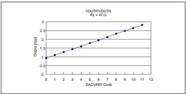
Figure 26.4 DACVREFF and Line Driver Output Amplitude Characteristics
