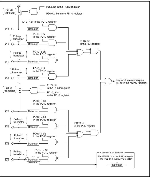
Figure 13.11 Block Diagram of Key Input Interrupt
