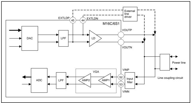
Figure 26.1 Analog Front End Circuit Block Diagram
