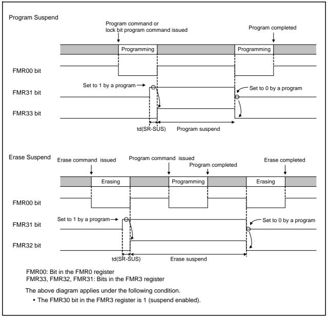
Figure 24.20 Suspend Operation Example in EW0 Mode
