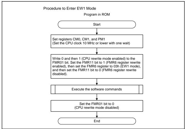
Figure 24.21 Setting and Resetting of EW1 Mode
