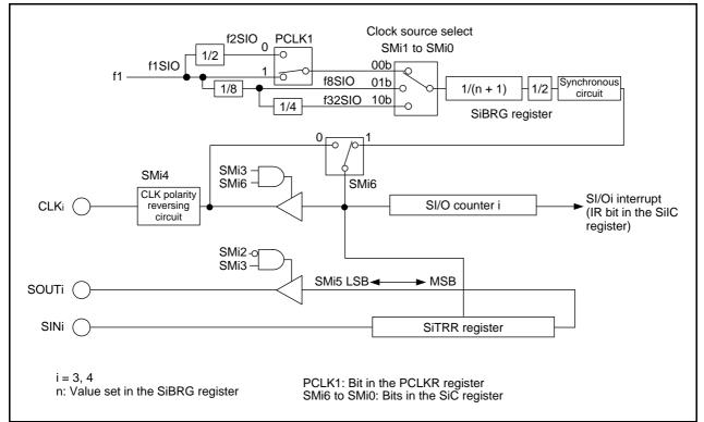
Figure 20.1 SI/O3 and SI/O4 Block Diagram
