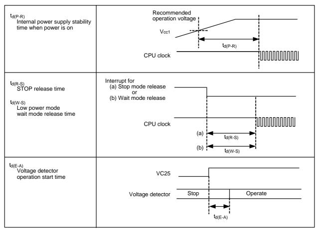
Figure 27.3 Power Supply Circuit Timing Diagram
