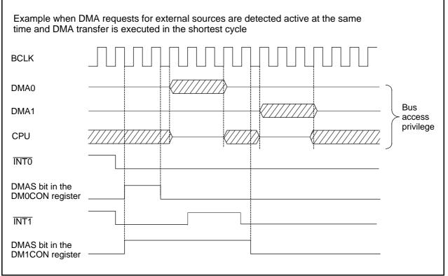
Figure 15.5 DMA Transfer by External Sources
