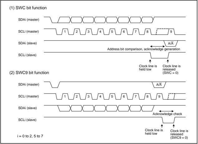
Figure 19.24 Inserting Wait-States Using Bits SWC and SWC9
