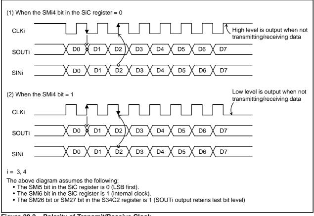
Figure 20.2 Polarity of Transmit/Receive Clock
