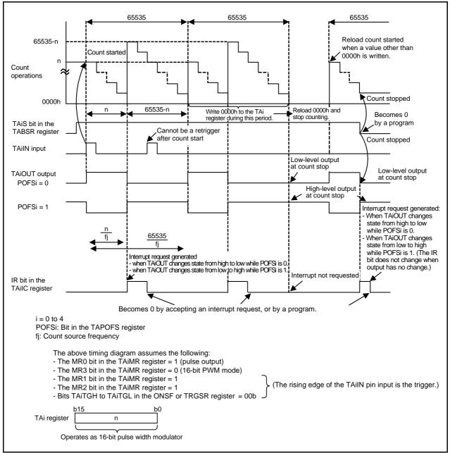
Figure 16.11 Operation Example in 16-Bit Pulse Width Modulation Mode
