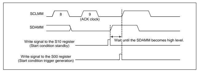
Figure 21.9 Restart Condition Generation Timing
