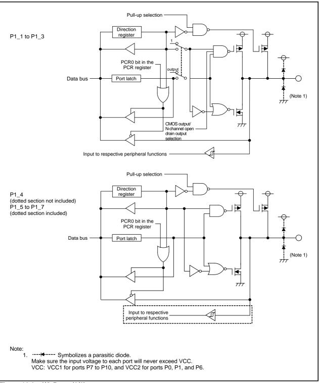
Figure 12.2 I/O Ports (2/8)
