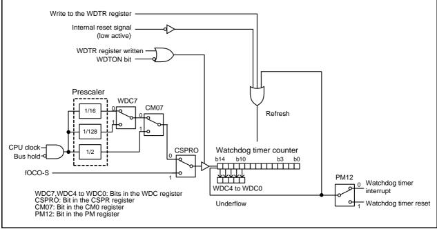
Figure 14.1 Watchdog Timer Block Diagram
