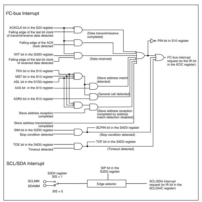
Figure 21.21 I<sup>2</sup>C Interface Interrupts
