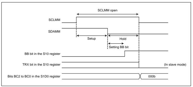
Figure 21.13 Start Condition Detection
