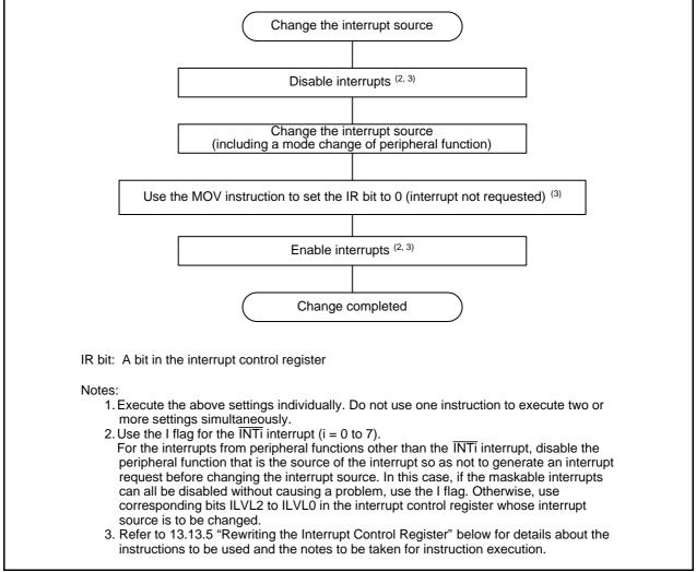
Figure 13.12 Procedure for Changing the Interrupt Generate Factor
