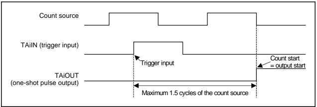
Figure 16.4 Output Example of One-Shot Timer Mode
