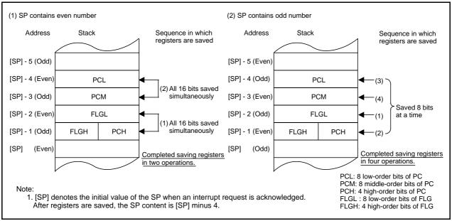
Figure 13.6 Register Save Operation
