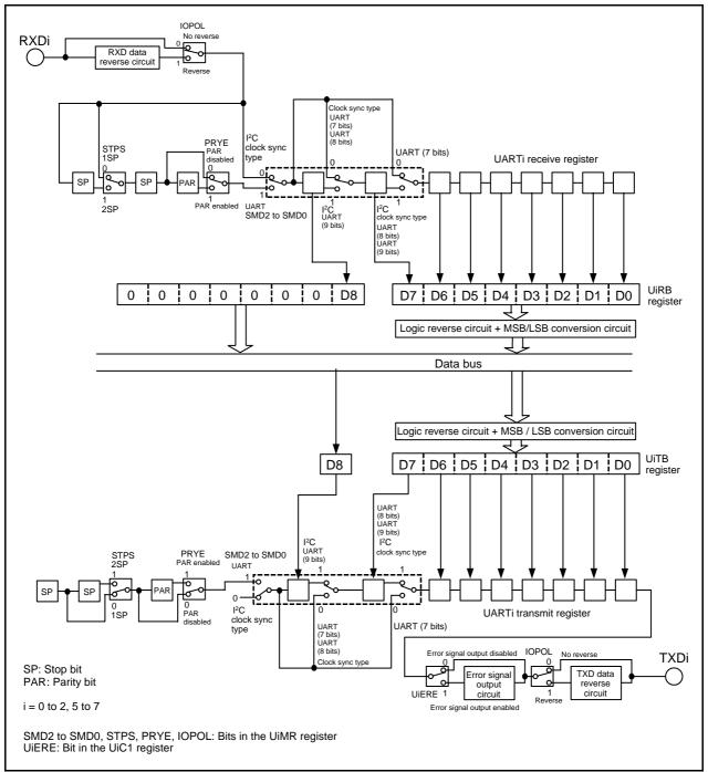
Figure 19.4 UARTi Transmit/Receive Unit Block Diagram
