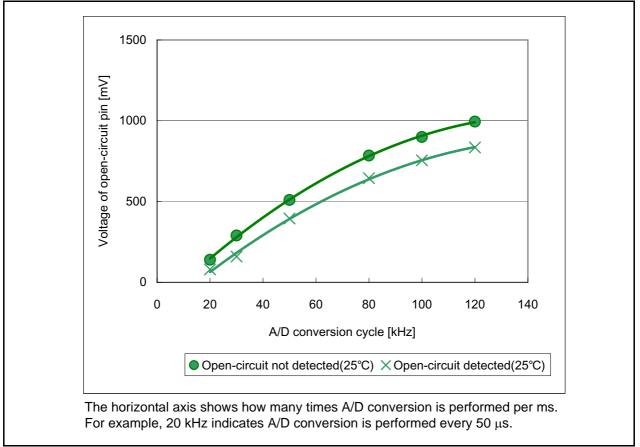
Figure 22.9 A/D Open-Circuit Detection (Discharge) Characteristics (Standard Characteristics)
