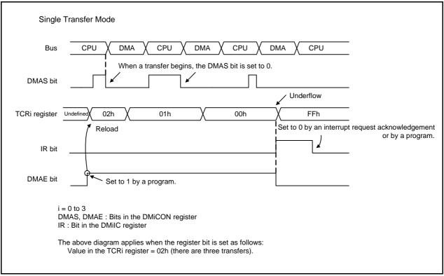
Figure 15.3 Operation Example in Single Transfer Mode
