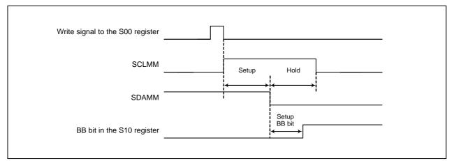
Figure 21.7 Start Condition Generation Timing
