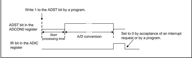
Figure 22.18 ADST Bit Operation
