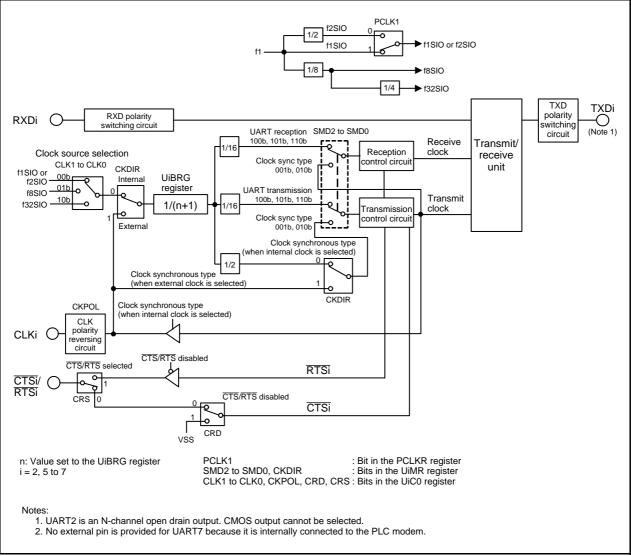
Figure 19.3 Block Diagram of UART2, and UART5 to UART7
