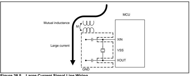
Figure 28.5 Large Current Signal Line Wiring
