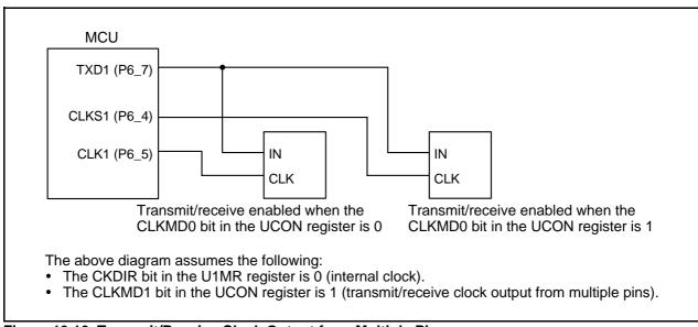
Figure 19.10 Transmit/Receive Clock Output from Multiple Pins
