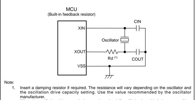
When the oscillation drive capacity is set to low, check if oscillation is stable in low status. Also, place a feedback resistor between XIN and XOUT if the oscillator manufacturer recommends placing the resistor externally.
