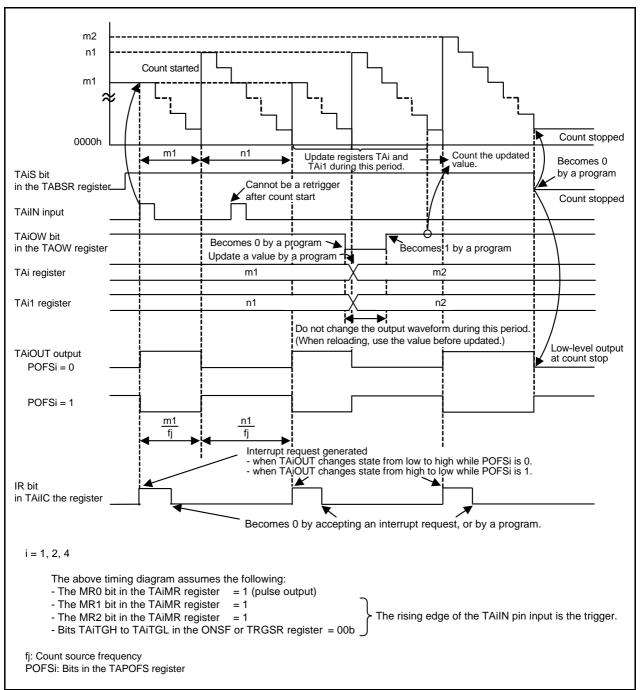
Figure 16.13 Operation Example in Programmable Output Mode
