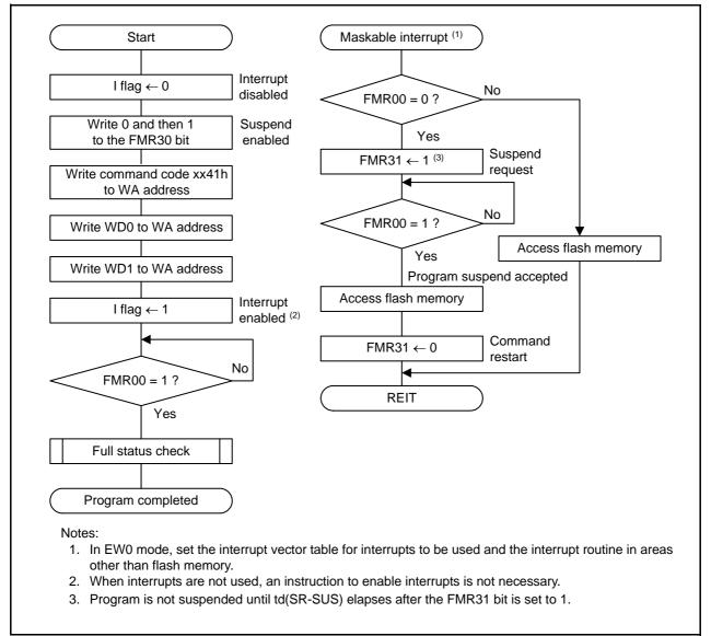
Figure 24.17 Program Flowchart in EW0 Mode (Suspend Function Enabled)
