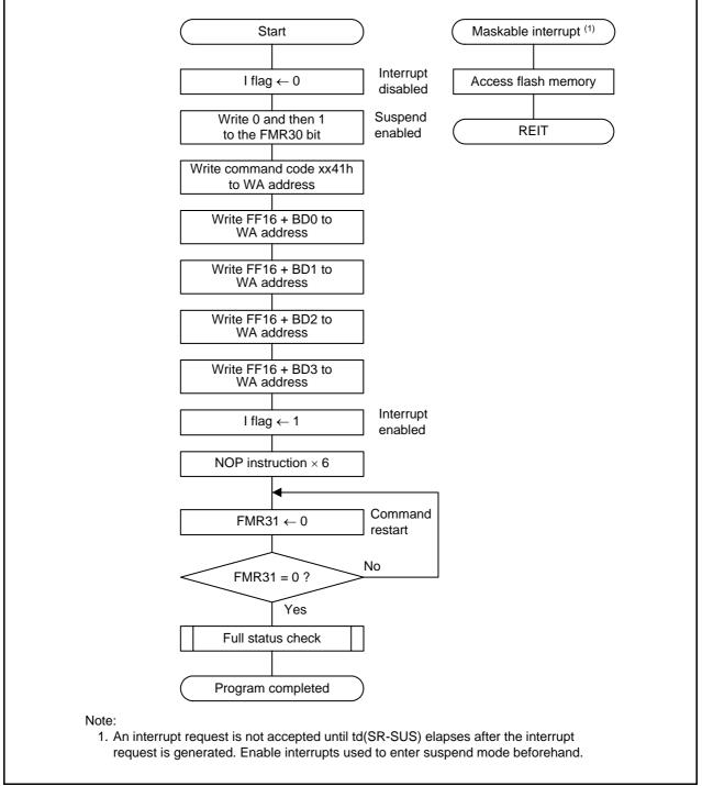
Figure 24.22 Program Flowchart in EW1 Mode (Suspend Function Enabled)
