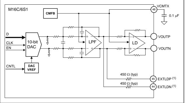
Figure 26.2 AFE Transmitter Circuit
