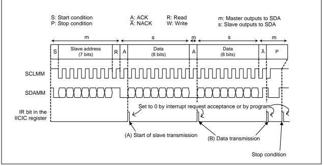
Figure 21.20 Example of Slave Transmission
