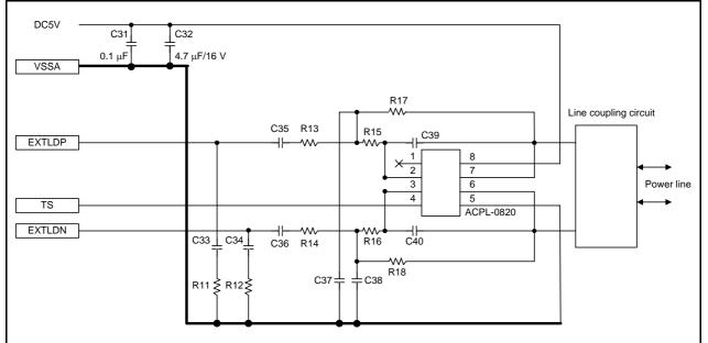
Figure 26.6 External Line Driver Connection Example (LSI in the figure is ACPL-0820 by AVAGO Technologies)
