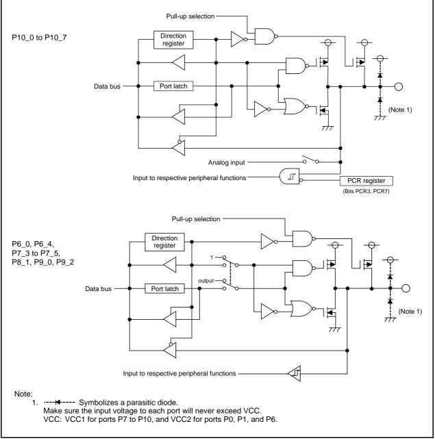
Figure 12.3 I/O Ports (3/8)
