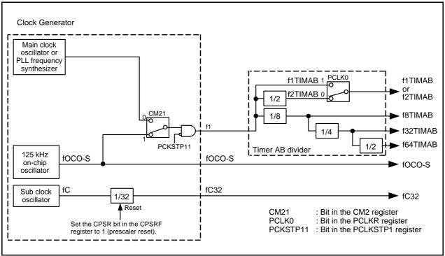
Figure 17.1 Timer A and B Count Sources
