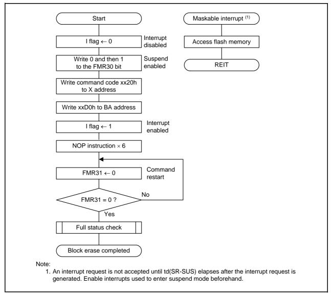
Figure 24.23 Block Erase Flowchart in EW1 Mode (Suspend Function Enabled)
