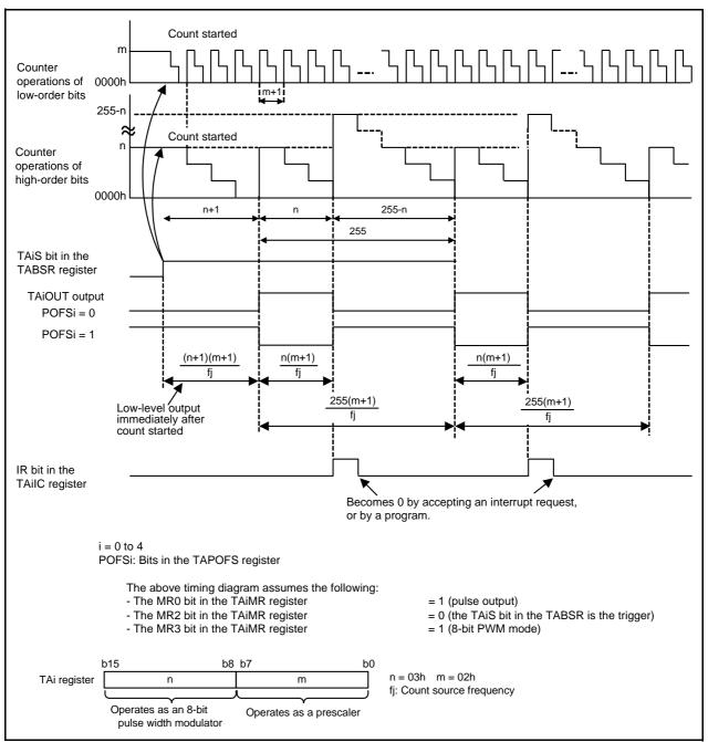
Figure 16.12 Operation Example in 8-Bit Pulse Width Modulation Mode
