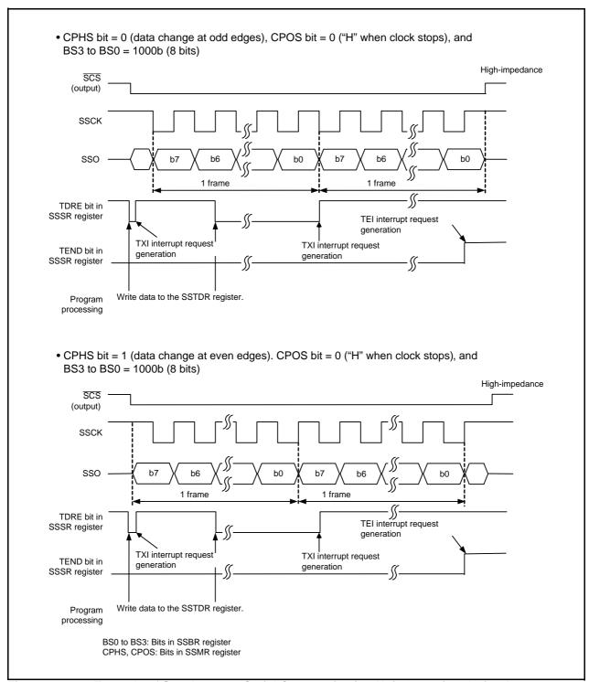
Figure 22.11 Example of Synchronous Serial Communication Unit Operation during Data
