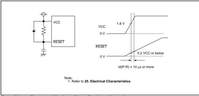
Figure 5.4 Example of Hardware Reset Circuit and Operation
