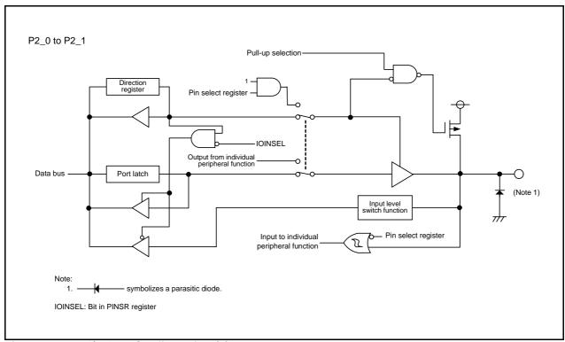
Figure 7.1 I/O Port Configuration (1)
