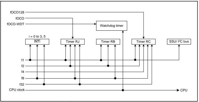
Figure 9.2 Peripheral Function Clock
