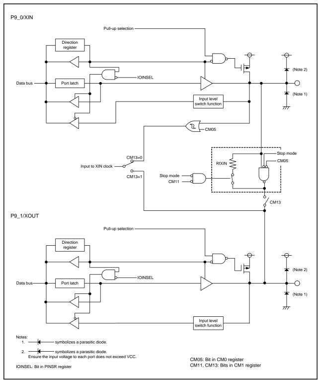
Figure 7.4 I/O Port Configuration (4)
