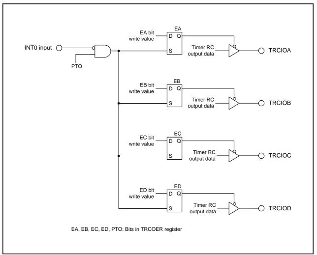
Figure 18.6 Forced Cutoff of Pulse Output
