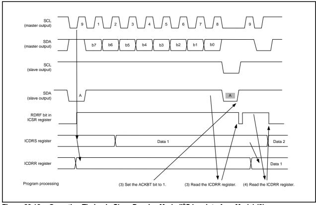
Figure 23.12 Operating Timing in Slave Receive Mode (I<sup>2</sup>C bus Interface Mode) (2)
