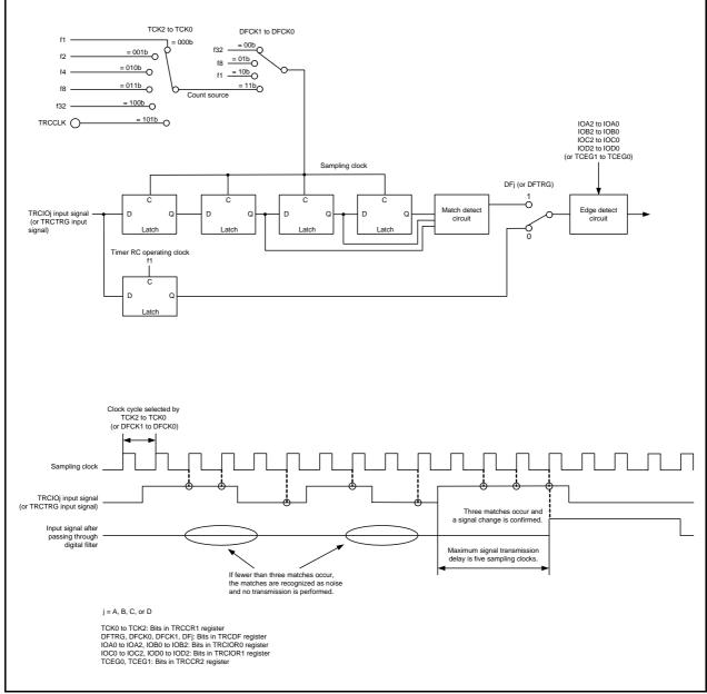
Figure 18.5 Block Diagram of Digital Filter
