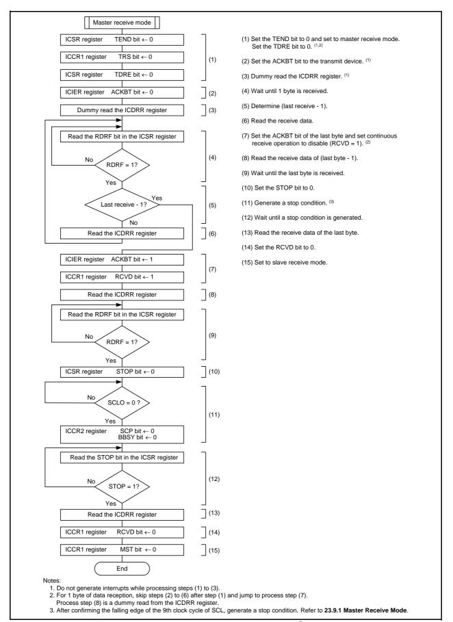
Figure 23.17 Register Setting Example in Master Receive Mode (I<sup>2</sup>C bus Interface Mode)
