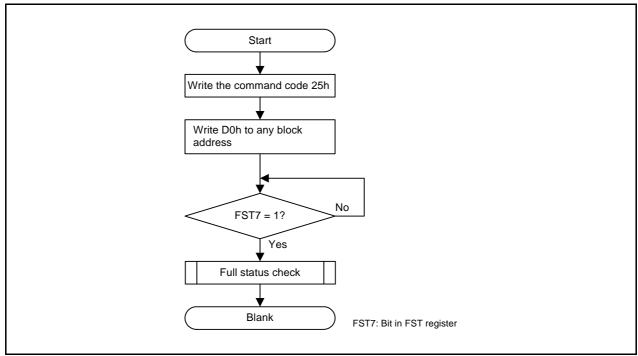
Figure 24.19 Block Blank Check Flowchart
