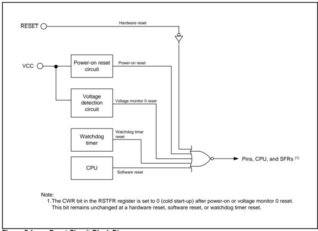
Figure 5.1 Reset Circuit Block Diagram
