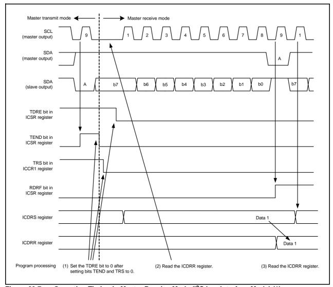
Figure 23.7 Operating Timing in Master Receive Mode (I<sup>2</sup>C bus Interface Mode) (1)
