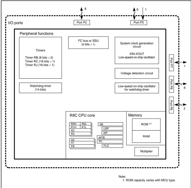
Figure 1.2 Block Diagram of R8C/LAPS Group
