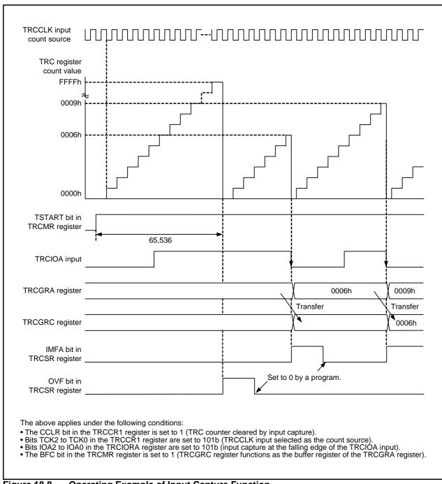
Figure 18.8 Operating Example of Input Capture Function
