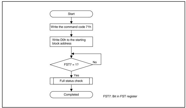
Figure 24.18 Read Lock Bit Status Flowchart
