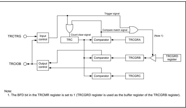
Figure 18.16 Block Diagram of PWM2 Mode
