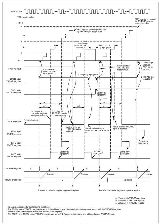
Figure 18.18 Operating Example in PWM2 Mode (TRCTRG Trigger Input Enabled)
