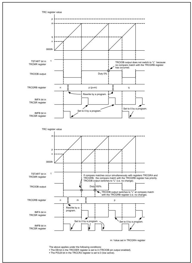
Figure 18.15 Operating Example in PWM Mode (Duty 0% and Duty 100%)
