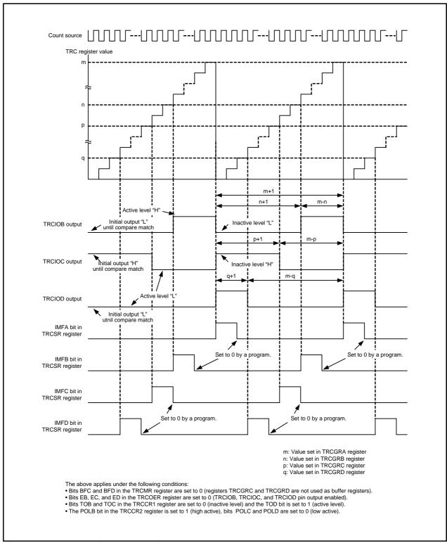
Figure 18.14 Operating Example in PWM Mode
