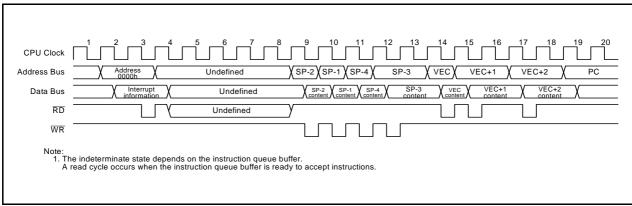
Figure 12.3 Time Required for Executing Interrupt Sequence
