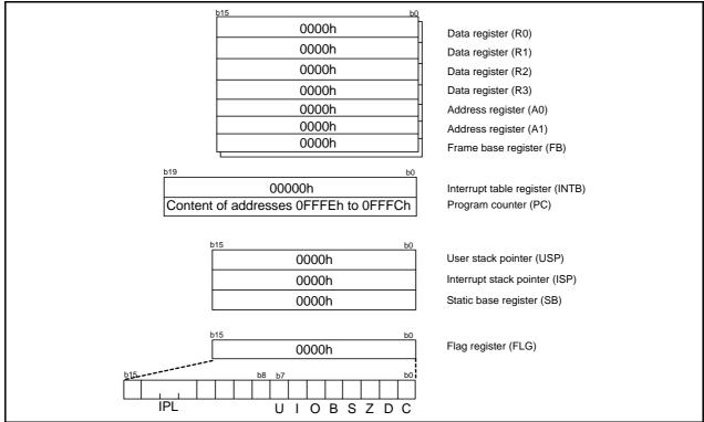
Figure 5.2 CPU Register Status after Reset
