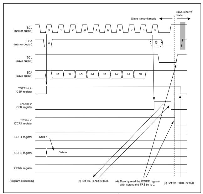
Figure 23.10 Operating Timing in Slave Transmit Mode (I<sup>2</sup>C bus Interface Mode) (2)
