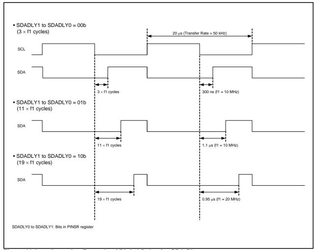
Figure 23.3 Operating Example of Digital Delay for SDA Pin
