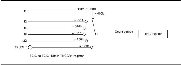
Figure 18.2 Count Source Block Diagram
