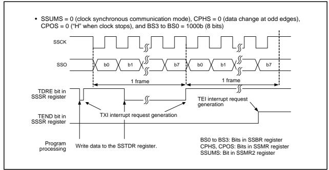
Figure 22.5 Example of Synchronous Serial Communication Unit Operation during Data
