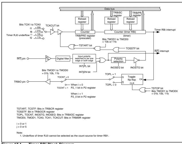
Figure 17.1 Timer RBi Block Diagram
