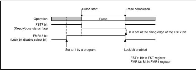
Figure 24.8 FMR13 Bit Operation Timing
