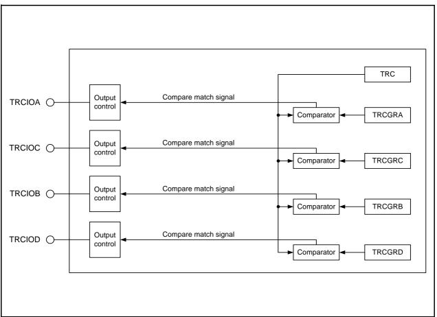
Figure 18.9 Block Diagram of Output Compare Function
