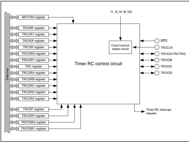
Figure 18.1 Timer RC Block Diagram
