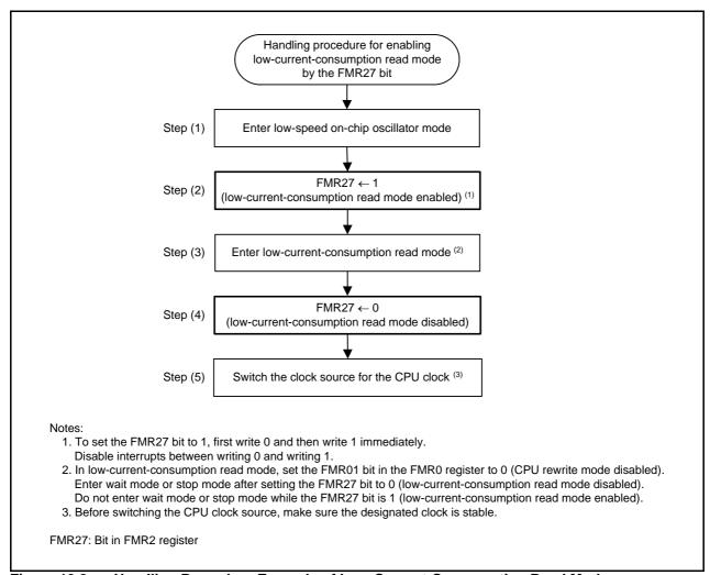
Figure 10.8 Handling Procedure Example of Low-Current-Consumption Read Mode
