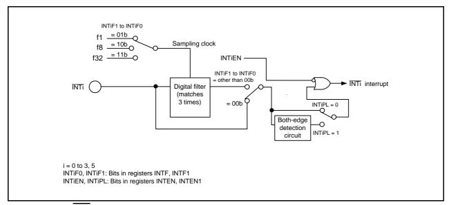
Figure 12.9 INTi Input Filter Configuration
