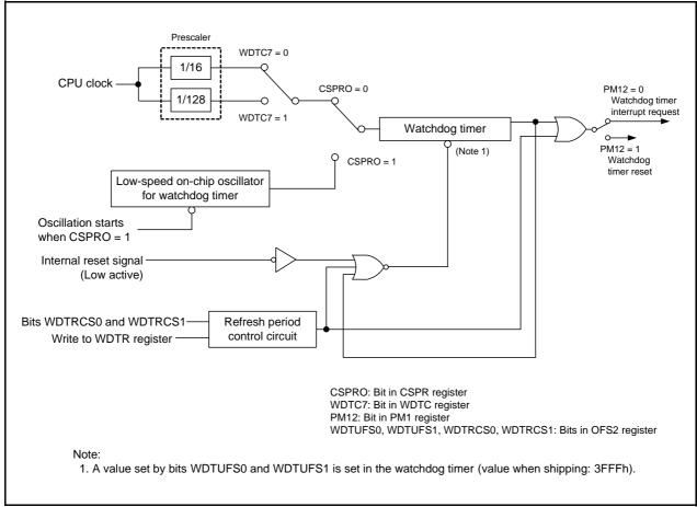
Figure 15.1 Watchdog Timer Block Diagram
