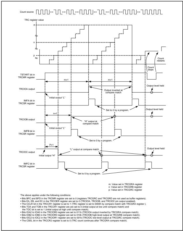
Figure 18.10 Operating Example of Output Compare Function
