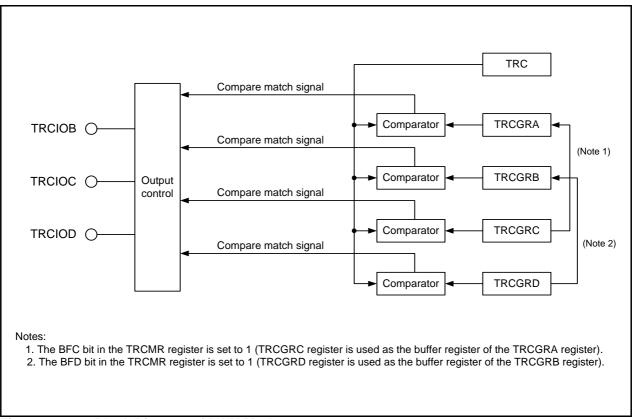
Figure 18.13 Block Diagram of PWM Mode
