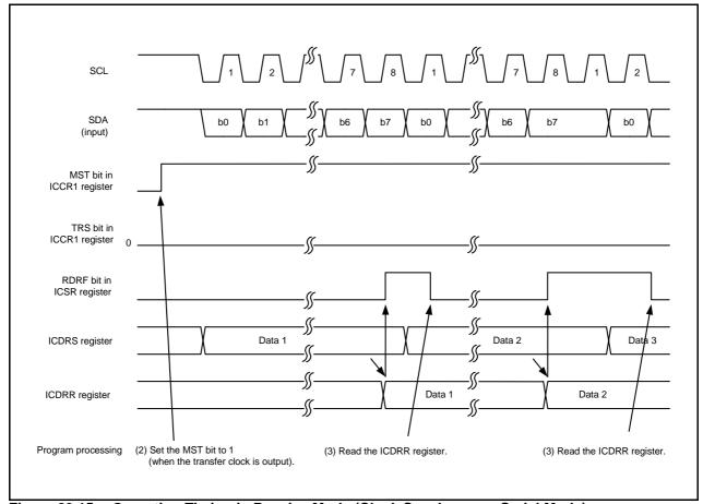
Figure 23.15 Operating Timing in Receive Mode (Clock Synchronous Serial Mode)
