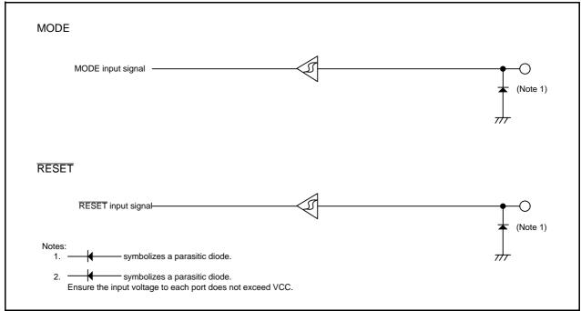
Figure 7.5 Pin Configuration
