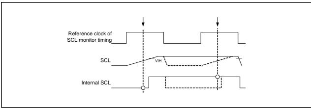
Figure 23.21 Bit Synchronization Circuit Timing
