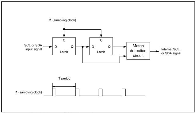
Figure 23.20 Block Diagram of Noise Canceller
