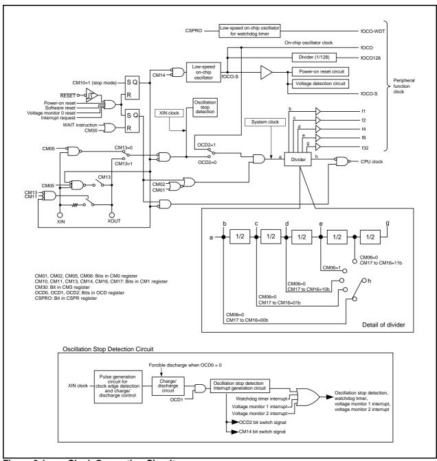
Figure 9.1 Clock Generation Circuit
