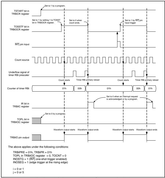
Figure 17.4 Operating Example in Programmable One-Shot Generation Mode
