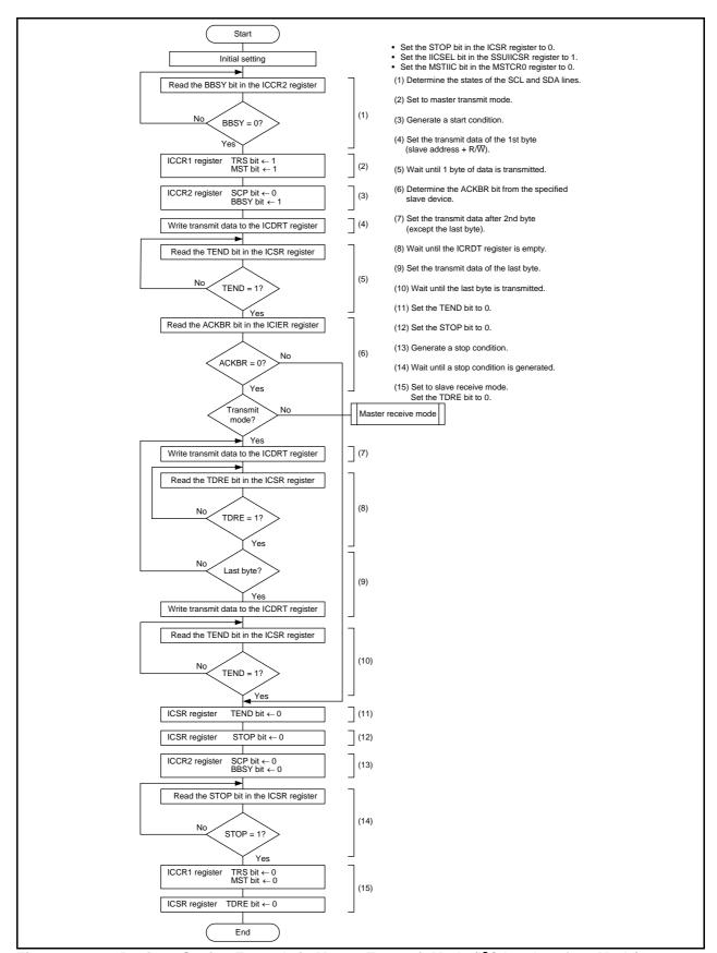
Figure 23.16 Register Setting Example in Master Transmit Mode (I<sup>2</sup>C bus Interface Mode)
