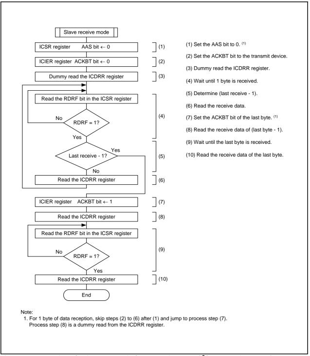
Figure 23.19 Register Setting Example in Slave Receive Mode (I<sup>2</sup>C bus Interface Mode)
