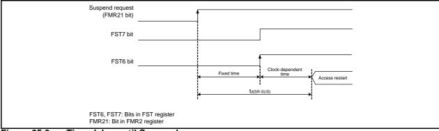
Figure 25.2 Time delay until Suspend
