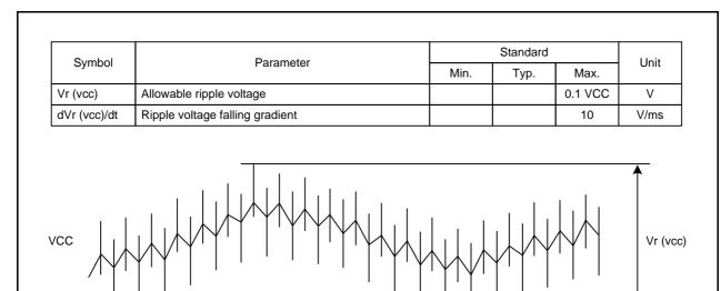
Figure 26.2 Definition of Ripple Voltage
