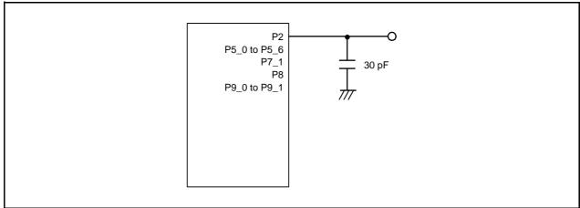
Figure 25.1 Ports P2, P5\_0 to P5\_6, P7\_1, P8, and P9\_0 to P9\_1 Timing Measurement Circuit
