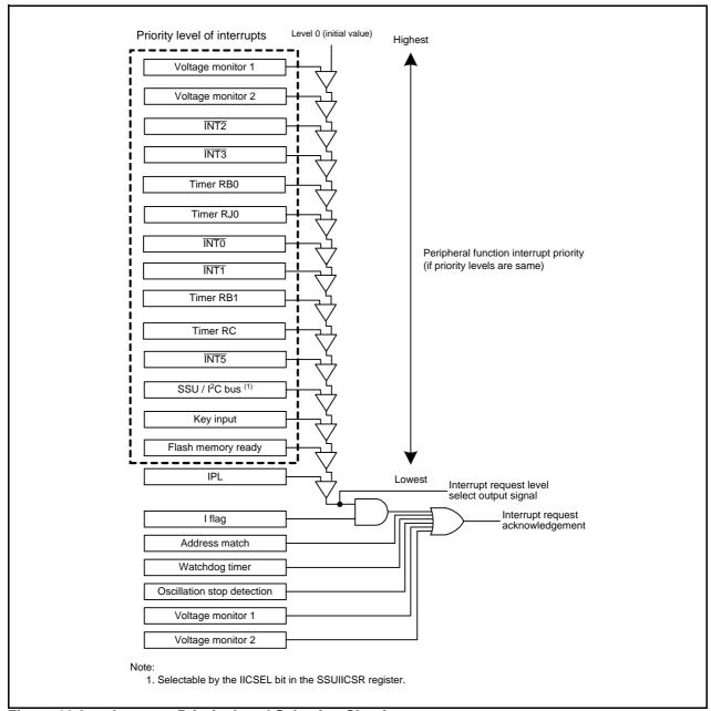
Figure 12.8 Interrupt Priority Level Selection Circuit
