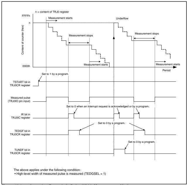
Figure 19.3 Operating Example in Pulse Width Measurement Mode
