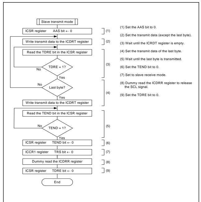
Figure 23.18 Register Setting Example in Slave Transmit Mode (I<sup>2</sup>C bus Interface Mode)
