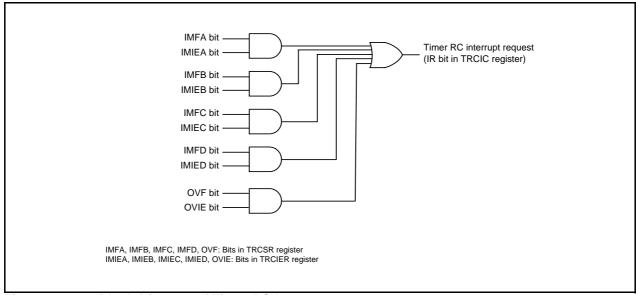
Figure 18.20 Block Diagram of Timer RC Interrupt
