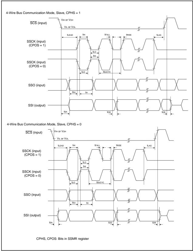
Figure 25.5 I/O Timing of Synchronous Serial Communication Unit (SSU) (Slave)
