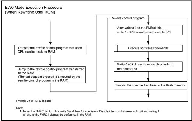
Figure 24.6 How to Set and Exit EW0 Mode
