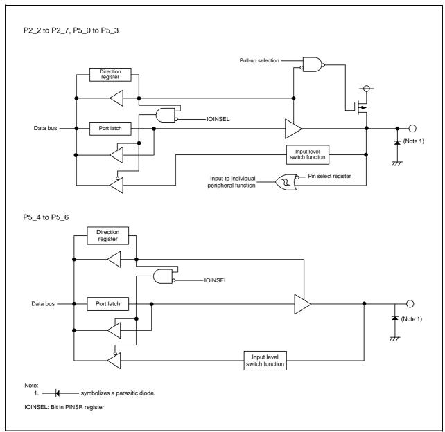
Figure 7.2 I/O Port Configuration (2)
