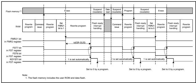
Figure 24.4 Erase-Suspend Operation Timing in EW0 Mode
