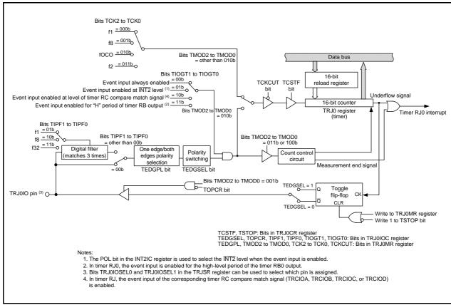
Figure 19.1 Timer RJ0 Block Diagram
