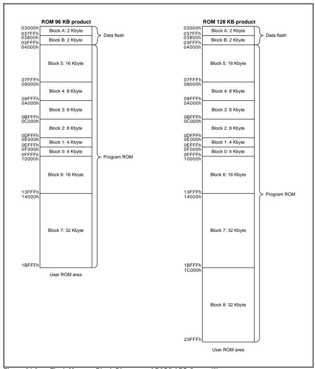
Figure 24.2 Flash Memory Block Diagrams of R8C/LAPS Group (2)
