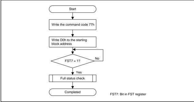
Figure 24.17 Lock Bit Program Flowchart
