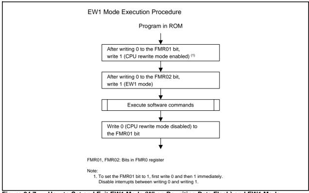
Figure 24.7 How to Set and Exit EW1 Mode (When Rewriting Data Flash) and EW1 Mode
