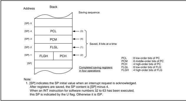
Figure 12.6 Register Saving Operation
