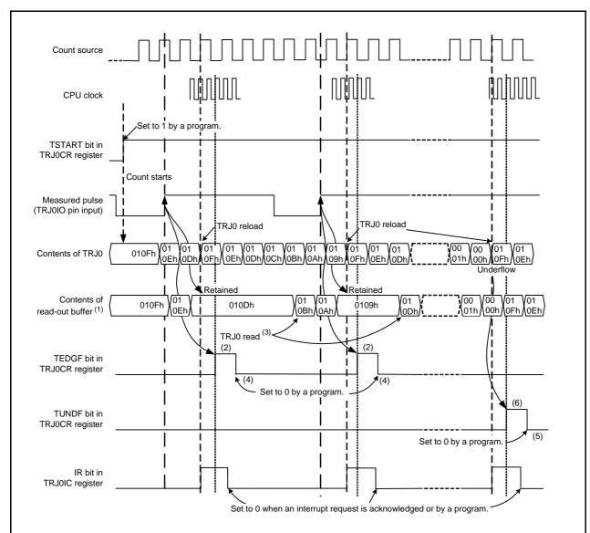
The above applies when the initial value in the TRJ0 register is set to 010Fh and the period from one rising edge to the next rising edge of the measurement pulse is measured (TEDGSEL = 0).
