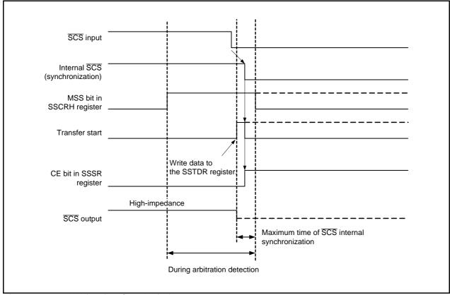
Figure 22.13 Arbitration Check Timing
