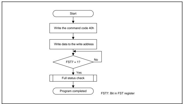
Figure 24.9 Program Flowchart (Flash Ready Status Interrupt Disabled)
