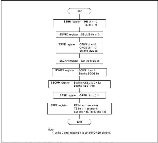
Figure 22.4 Initialization in Clock Synchronous Communication Mode
