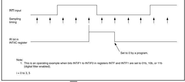
Figure 12.10 Operating Example of INTi Input Filter
