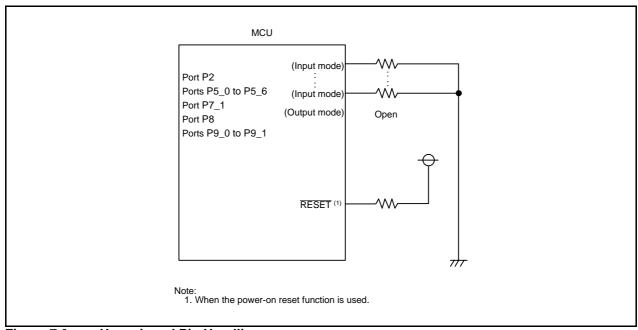
Figure 7.6 Unassigned Pin Handling
