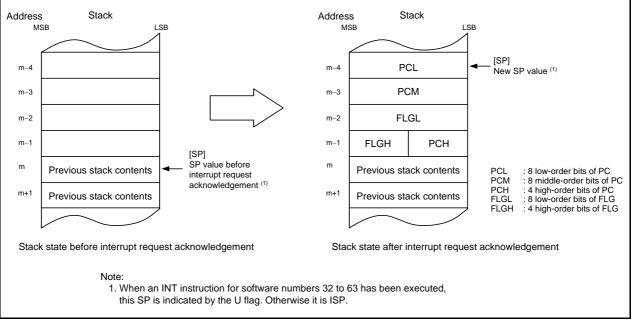
Figure 12.5 Stack State Before and After Acknowledgement of Interrupt Request
