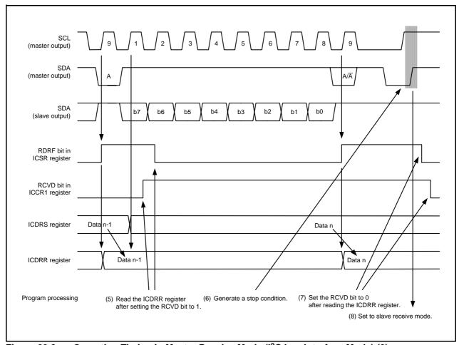
Figure 23.8 Operating Timing in Master Receive Mode (I<sup>2</sup>C bus Interface Mode) (2)
