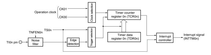
Figure 6-61. Block Diagram of Operation as Delay Counter
