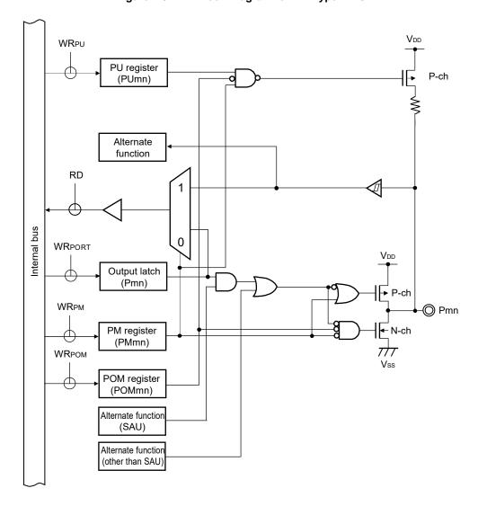
Figure 2-5. Pin Block Diagram for Pin Type 7-1-9
