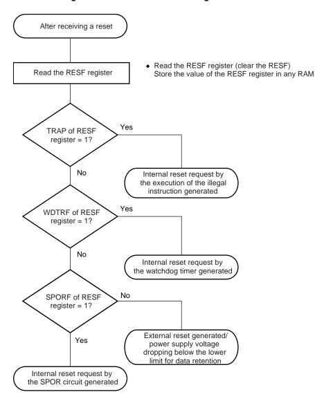
Figure 16-6. Procedure for Checking Reset Source
