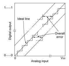
Figure 10-16. Quantization Error
