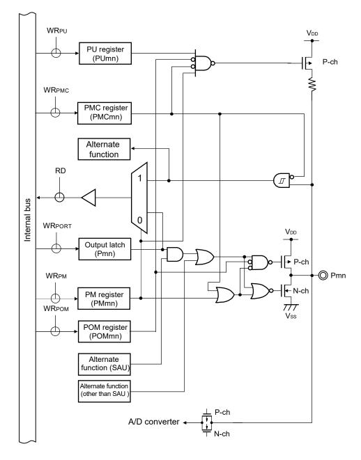
Figure 2-7. Pin Block Diagram for Pin Type 7-3-2
