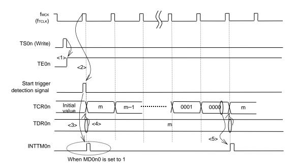
Figure 6-25. Operation Timing (In Interval Timer Mode)
