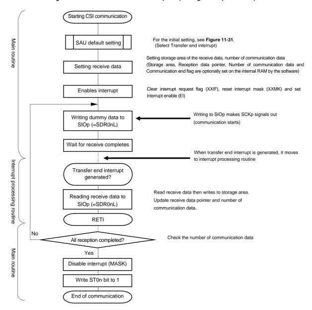
Figure 11-35. Flowchart of Master Reception (in Single-Reception Mode)
