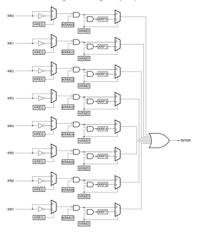
Figure 14-1. Block Diagram of Key Interrupt
