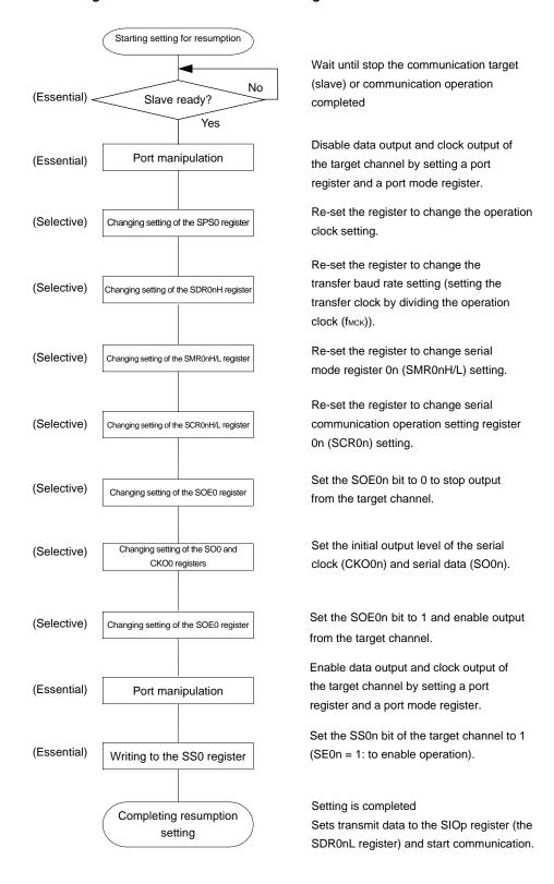
Figure 11-25. Procedure for Resuming Master Transmission
