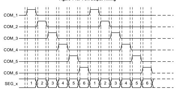
Figure 4-10. Port Output Timing
