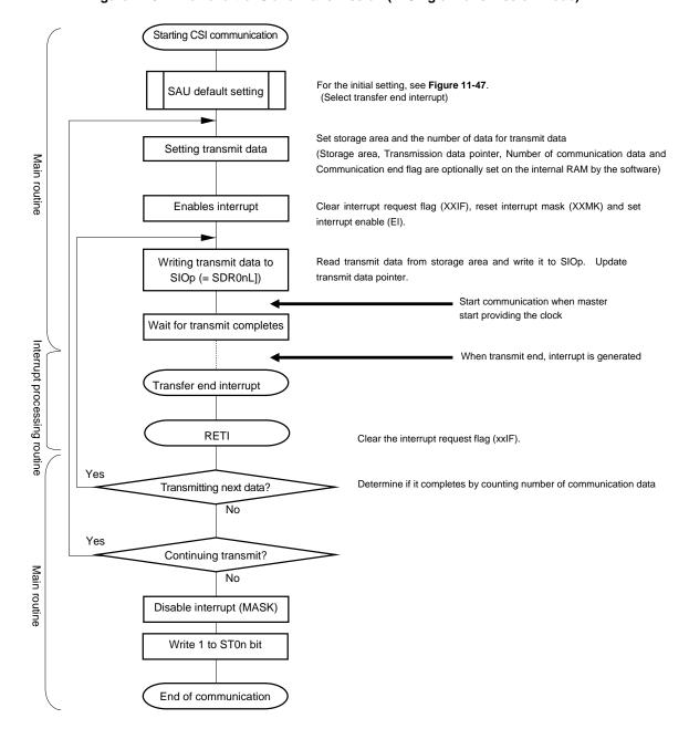
Figure 11-51. Flowchart of Slave Transmission (in Single-Transmission Mode)
