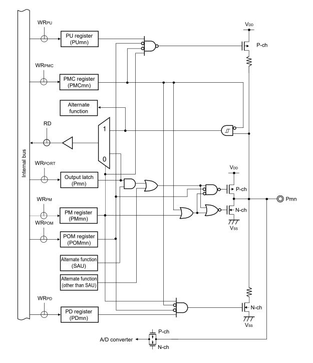
Figure 2-9. Pin Block Diagram for Pin Type 19-3-1
