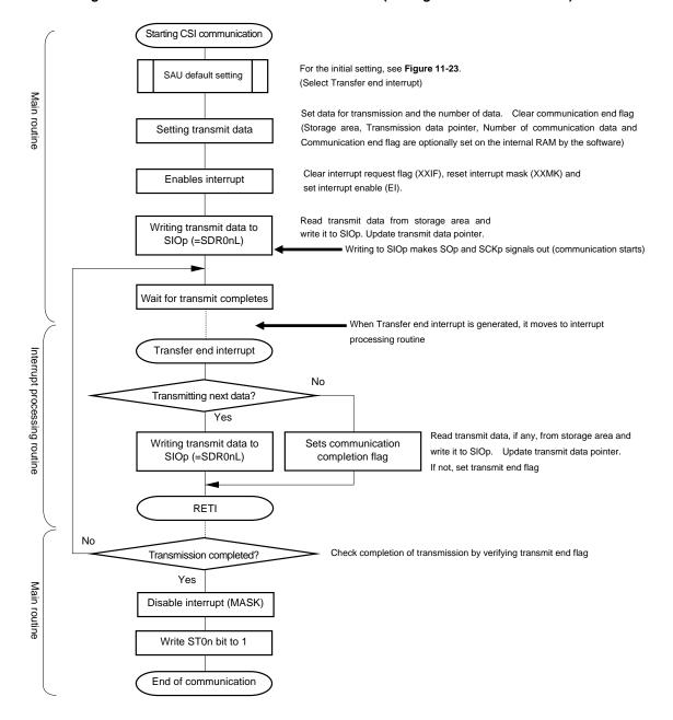
Figure 11-27. Flowchart of Master Transmission (in Single-Transmission Mode)
