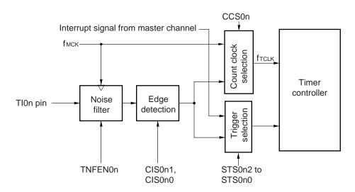
Figure 6-39. Input Circuit Configuration
