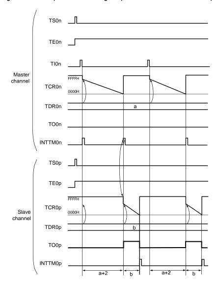
Figure 6-66. Example of Basic Timing of Operation for One-shot Pulse Output
