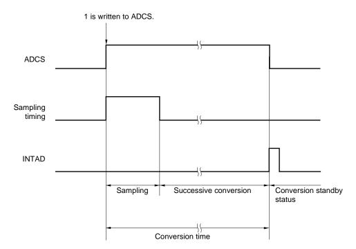
Figure 10-5. A/D Converter Sampling and A/D Conversion Timing
