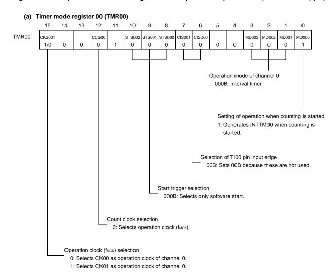
Figure 6-82. Example of Set Contents of Registers for Multiple PWM Output Function (Master Channel) (2/2)
