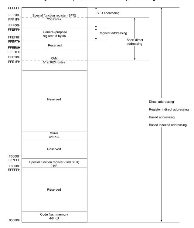
Figure 3-3. Correspondence Between Data Memory and Addressing
