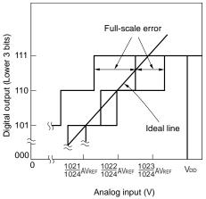
Figure 10-19. Integral Linearity Error
