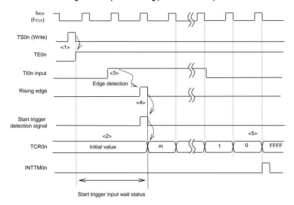
Figure 6-28. Operation Timing (In One-count Mode)
