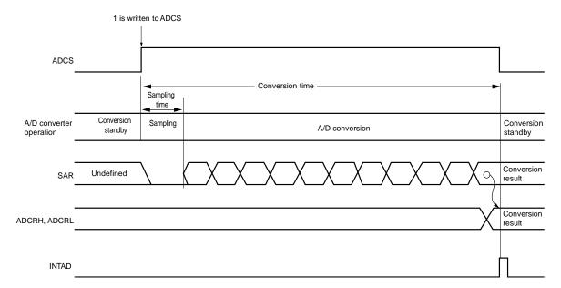
Figure 10-11. Conversion Operation of A/D Converter
