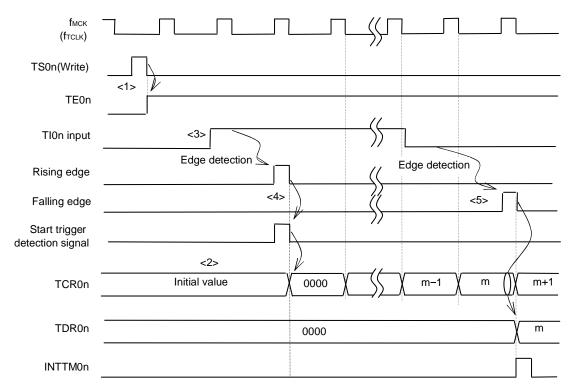
Remark Figure 6-29 shows the timing when the noise filter is not used. When the noise filter is on-state, the edge detection is delayed by two cycles of the operating clock (fmck) from the TI0n input (totally 3 to 4 cycles). The error of one cycle is due to the asynchronous timing between the TI0n input and operating clock (fmck).
