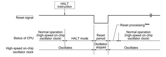
Note For the reset processing time, see CHAPTER 16 RESET FUNCTION. For the reset processing time of the SPOR circuit, see CHAPTER 17 SELECTABLE POWER-ON-RESET CIRCUIT.
