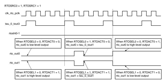
Figure 12-9. Output Timing
