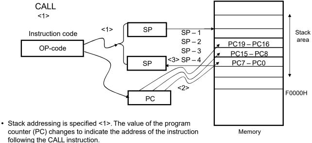
• The values of PC bits 19 to 16, 15 to 8, and 7 to 0 are stored in addresses SP – 2, SP – 3, and SP – 4, respectively <2>.
