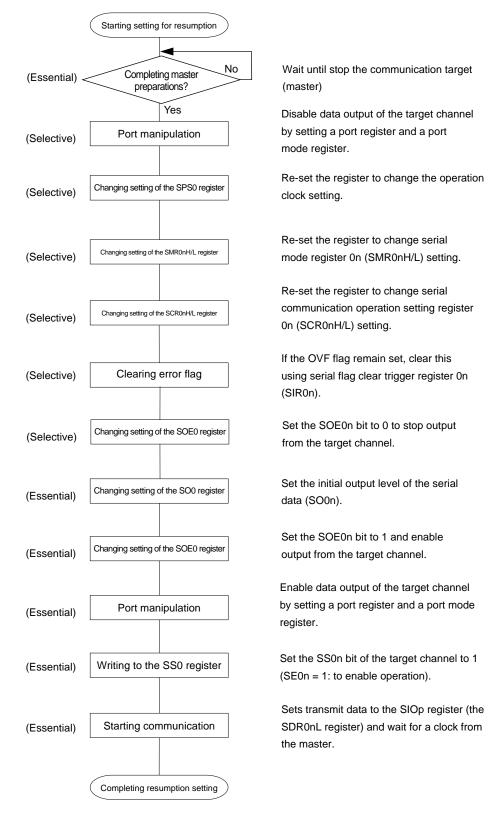
Figure 11-49. Procedure for Resuming Slave Transmission
