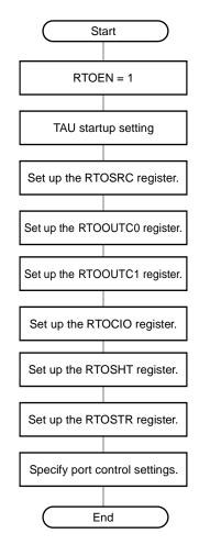
Figure 12-8. Initial Register Setup Flow
