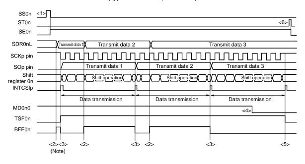
**Note** If transmit data is written to the SDR0nL register while the BFF0n bit of serial status register 0n (SSR0n) is 1 (valid data is stored in serial data register 0n (SDR0nL)), the transmit data is overwritten.
