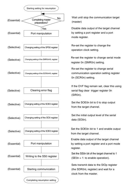
Figure 11-63. Procedure for Resuming Slave Transmission/Reception
