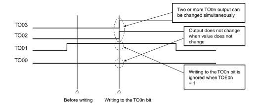
Figure 6-37. TO0n Pin Statuses by Collective Manipulation of TO0n Bit
