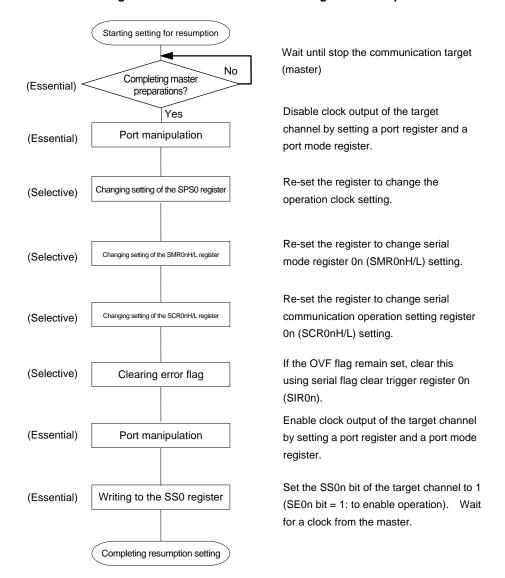
Figure 11-57. Procedure for Resuming Slave Reception
