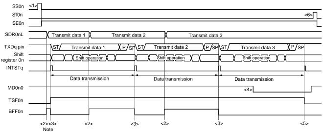
**Note** If transmit data is written to the SDR0nL register while the BFF0n bit of serial status register 0n (SSR0n) is 1 (valid data is stored in serial data register 0n (SDR0nL)), the transmit data is overwritten.
