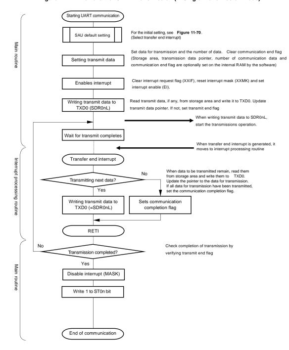
Figure 11-74. Flowchart of UART Transmission (in Single-Transmission Mode)
