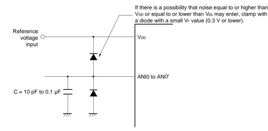
Figure 10-21. Analog Input Pin Connection
