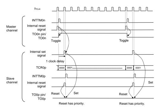
Remarks 1. Internal reset signal: TO0n pin reset/toggle signal Internal set signal: TO0n pin set signal
