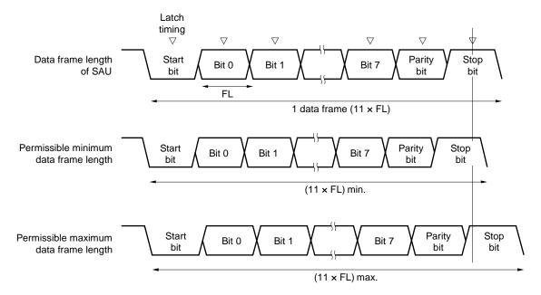
As shown in Figure 11-83 the timing of latching receive data is determined by the division ratio set by bits 7 to 1 of serial data register 0nH (SDR0nH) after the start bit is detected. If the last data (stop bit) is received before this latch timing, the data can be correctly received.
