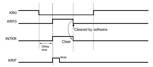
Note Acknowledgment of vectored interrupt request or bit cleared by software
