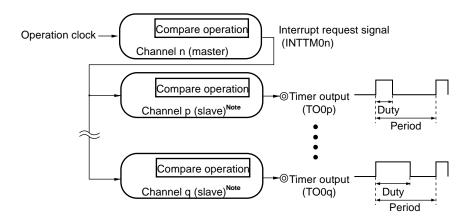
**Note** This operation can be obtained with the lower 8-bit timer of channel 1 or 3.
