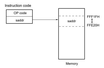
Remark SADDR and SADDRP are used to describe the values of addresses FE20H to FF1FH with 16-bit immediate data (higher 4 bits of actual address are omitted), and the values of addresses FFE20H to FFF1FH with 20bit immediate data.
