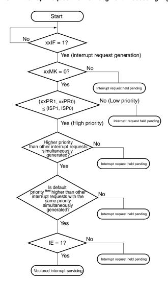
Figure 13-7. Interrupt Request Acknowledgment Processing Algorithm
