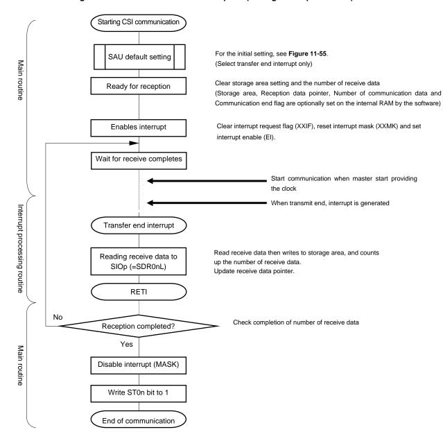
Figure 11-59. Flowchart of Slave Reception (in Single-Reception Mode)
