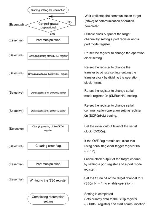
Figure 11-33. Procedure for Resuming Master Reception
