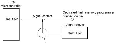
In the flash memory programming mode, a signal output by another device will conflict with the signal output by the dedicated flash memory programmer. Therefore, isolate the signal of another device.
