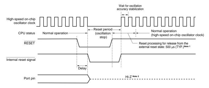
Figure 16-2. Timing of Reset by RESET Input
