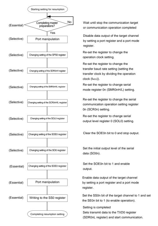
Figure 11-72. Procedure for Resuming UART Transmission
