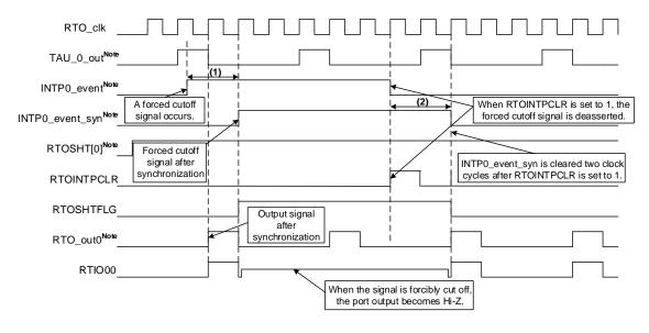
Figure 12-10. Timing of Entering and Exiting the Output Cutoff State by Using INTPO
