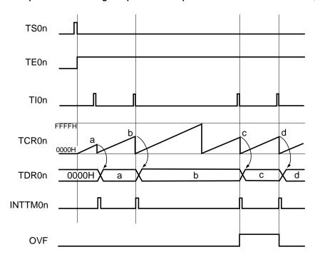
Figure 6-54. Example of Basic Timing of Operation as Input Pulse Interval Measurement (MD0n0 = 0)
