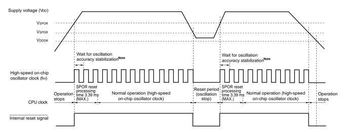
Figure 17-2. Timing of Internal Reset Signal Generation
