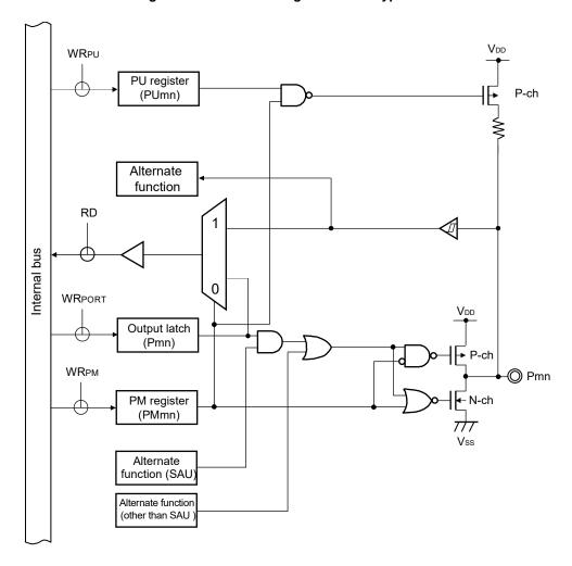
Figure 2-3. Pin Block Diagram for Pin Type 7-1-1
