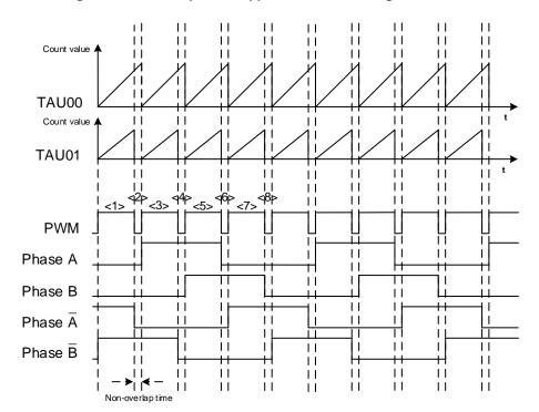
Figure 12-15. Example of Stepper Motor Controlling Waveforms
