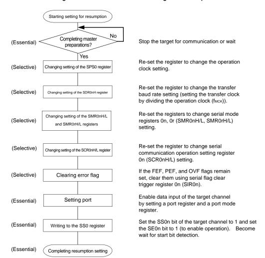
Figure 11-80. Procedure for Resuming UART Reception
