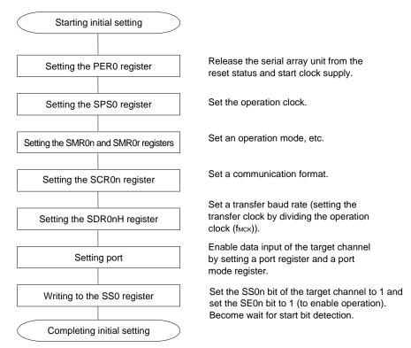
Caution After setting the RXE0n bit of SCR0n register to 1, be sure to set SS0n to 1 after 4 or more fclk clocks have elapsed.
