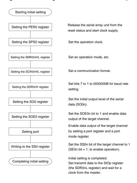
Caution Be sure to set transmit data to the SIOp register before the clock from the master is started.
