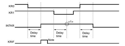
Note Acknowledgment of vectored interrupt request or bit cleared by software
