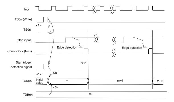
Figure 6-26. Operation Timing (In Event Counter Mode)
