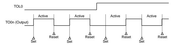
Remarks 1. Set: The output signal of the TO0n pin changes from inactive level to active level.
