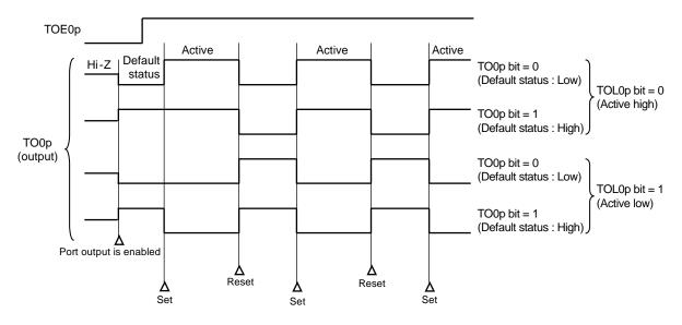
Figure 6-33. TO0p Pin Output Status at PWM Output (TOM0p = 1)
