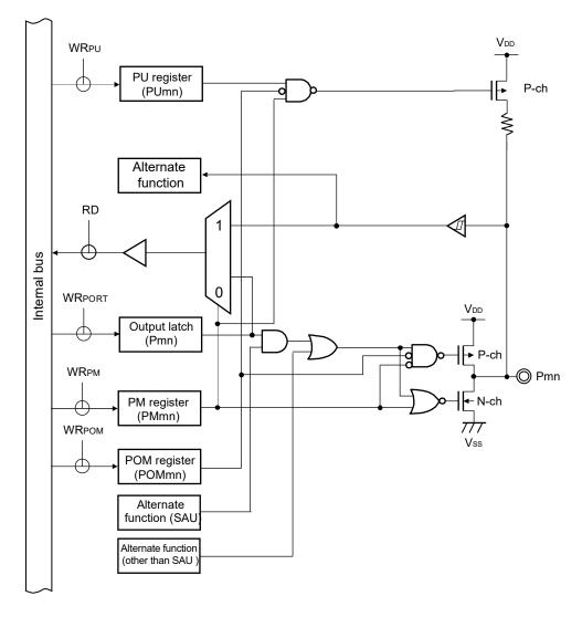
Figure 2-4. Pin Block Diagram for Pin Type 7-1-2
