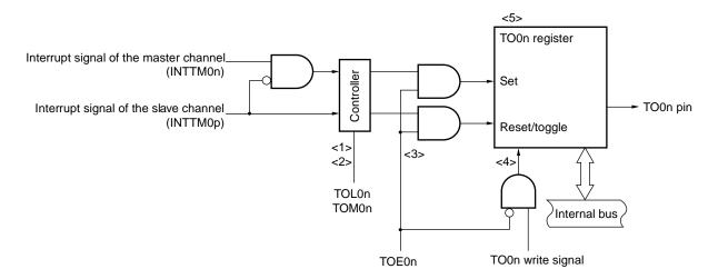
The following describes the TO0n pin output circuit.
