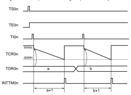
Figure 6-62. Example of Basic Timing of Operation as Delay Counter
