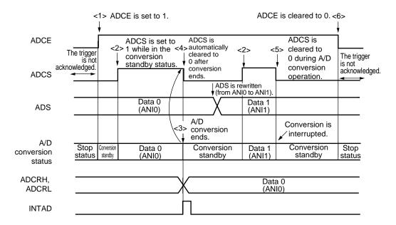
Figure 10-13. Example of Operation Timing
