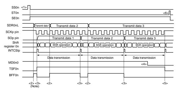
**Note** If transmit data is written to the SDR0nL register while the BFF0n bit of serial status register 0n (SSR0n) is 1 (valid data is stored in serial data register 0n (SDR0nL)), the transmit data is overwritten.
