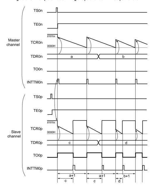
Figure 6-76. Example of Basic Timing of Operation as PWM Output Function
