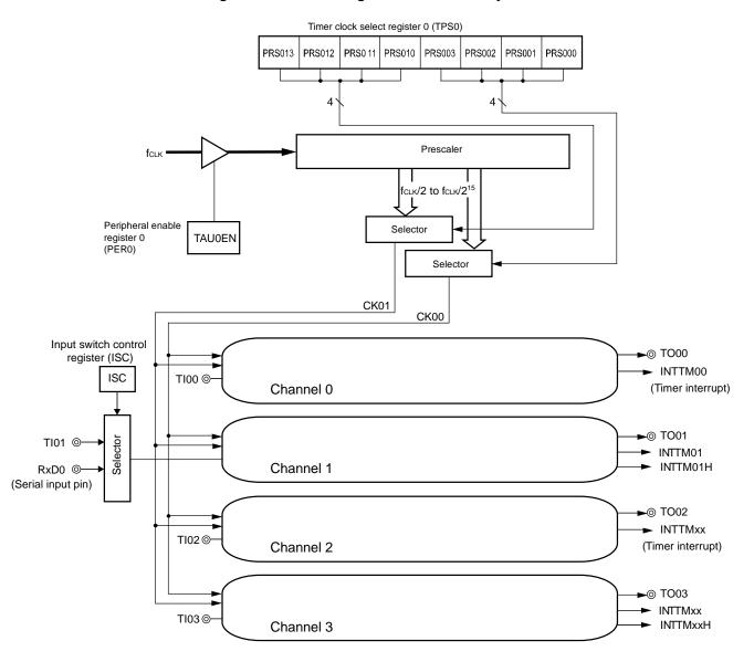
Figure 6-1. Entire Configuration of Timer Array Unit
