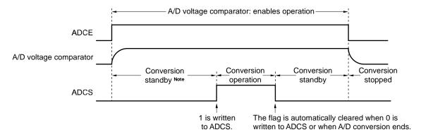
Note It requires at least 0.1  $\mu$ s to stabilize the internal circuit until the A/D conversion operation is started (ADCS = 1) after the operation of the A/D voltage comparator is enabled (ADCE = 1). If the ADCS bit is set to 1 without waiting for at least 0.1  $\mu$ s, ignore data of the first conversion.
