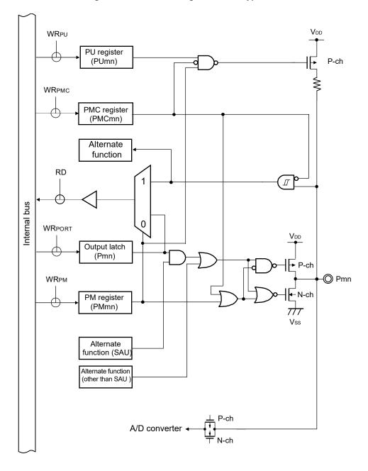
Figure 2-6. Pin Block Diagram for Pin Type 7-3-1
