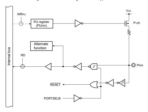
Figure 2-2. Pin Block Diagram for Pin Type 3-1-1
