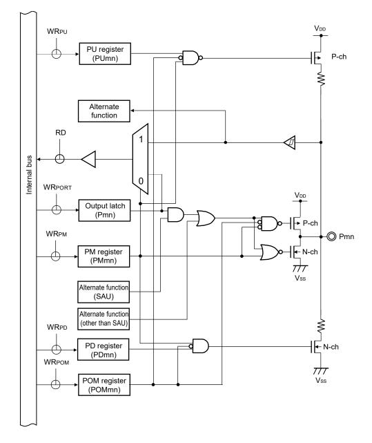
Figure 2-8. Pin Block Diagram for Pin Type 19-1-1
