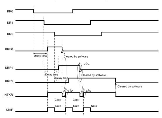
Figure 14-8. Operation of INTKR Signal When Key Interrupts Are Input to Multiple Channels (When KRMD = 1 and KREG = 0)
