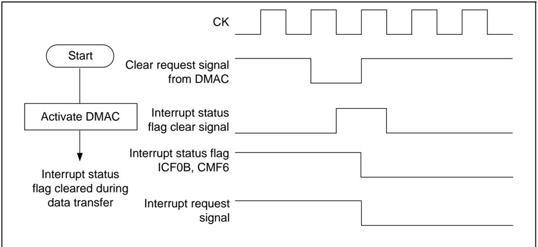
**Figure 11.43 Procedure and Timing for Clearing by DMAC**
