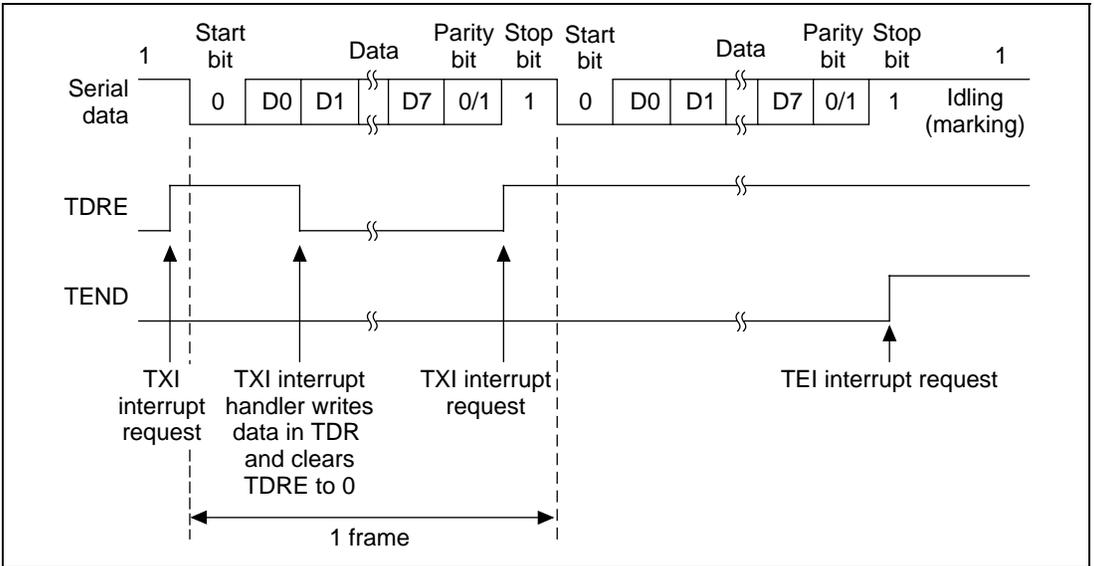
**Figure 15.6 SCI Transmit Operation in Asynchronous Mode
