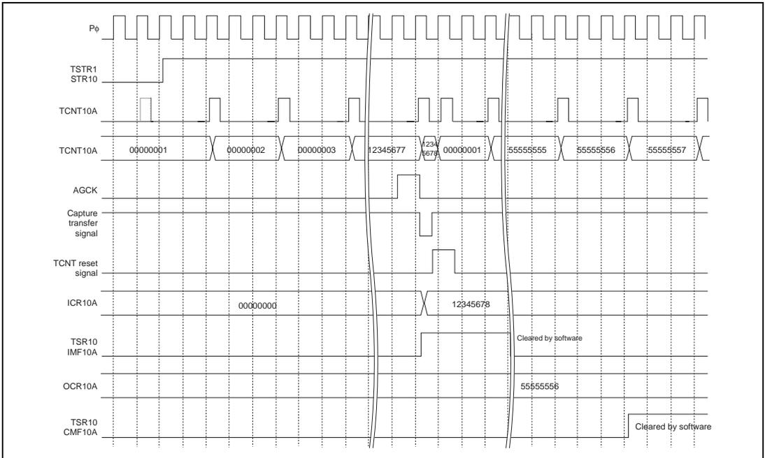
**Figure 11.28 TCNT10A Capture Operation and Compare-Match Operation**
