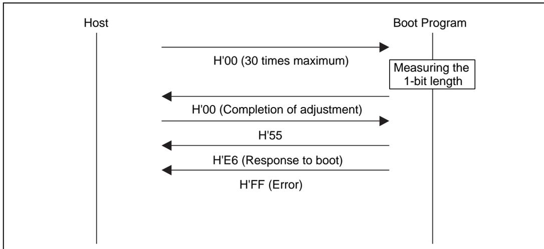
**Figure 23.27 Bit-Rate-Adjustment Sequence**
