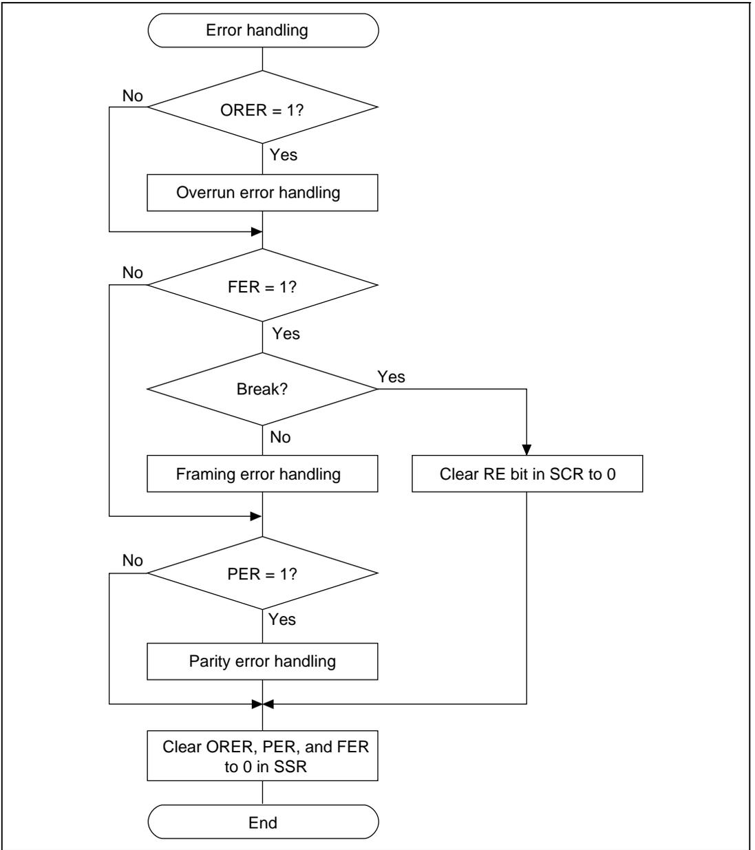
Figure 15.8 Sample Flowchart for Receiving Serial Data (2)
