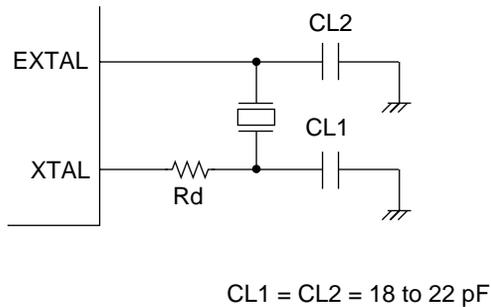
Figure 5.4 Connection of Crystal Oscillator (Example)
