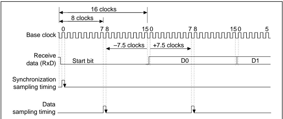
**Figure 15.24 Receive Data Sampling Timing in Asynchronous Mode**
