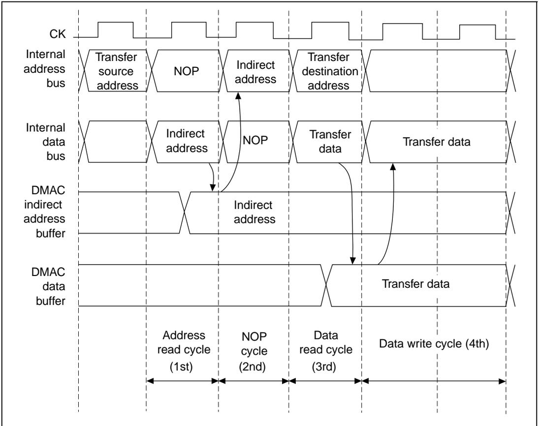
**Figure 10.7 Dual Address Mode and Indirect Address Transfer Timing Example 2
