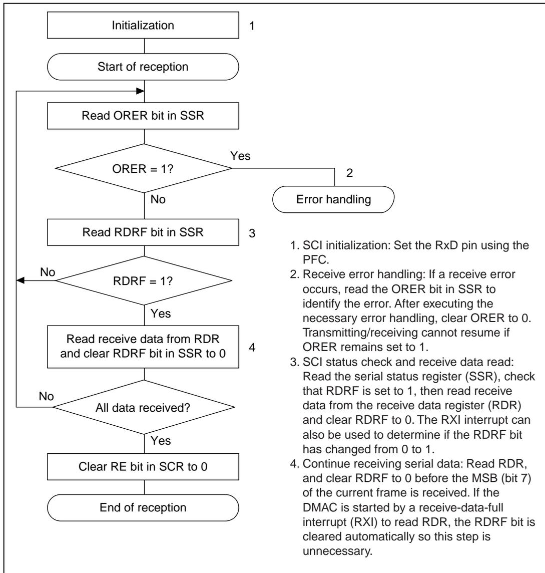
**Figure 15.20 Sample Flowchart for Serial Receiving (1)**
