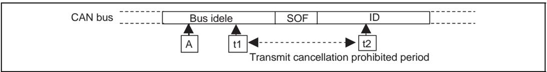
When the transmission setting (TXPR) is made to a mailbox at the point A shown in the above figure and then transmit cancellation setting (TXCR) is made at the timing between t1 and t2, transmission may be performed to the CAN bus regardless of the fact that a flag is set in the abort acknowledge register. (The transmit acknowledge (TXACK) of the transmitted mailbox is set.)
