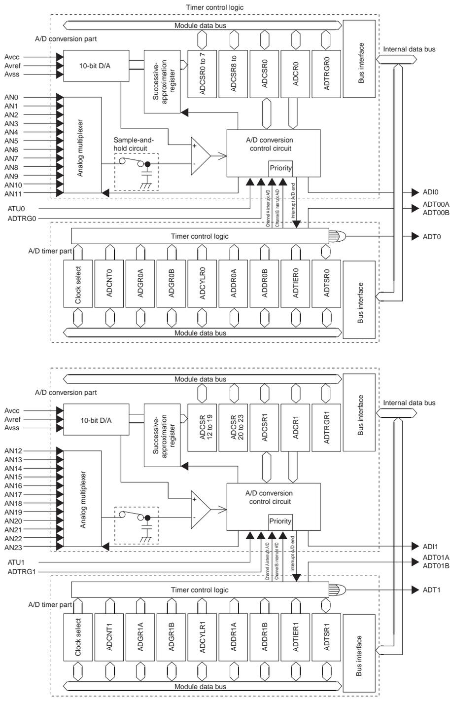
**Figure 18.1 Simplified Block Diagram of Multi-Trigger A/D Converter**
