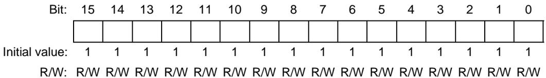
GR10G is initialized to H'FFFF by a power-on reset, and in hardware standby mode and software standby mode.
