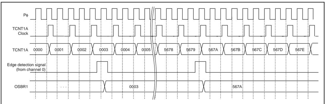
**Figure 11.20 Twin-Capture Operation**
