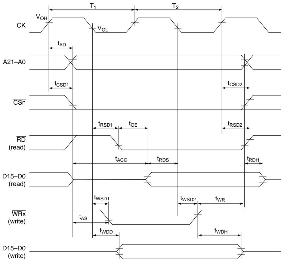
Note: t<sub>RDH</sub>: Specified from the negate timing of A21-A0, CS<sub>n</sub>, or RD, whichever is first.
