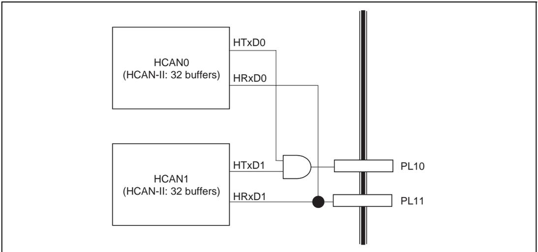
1. When a message is transmitted to the CAN bus without connecting to other nodes, an ACK error will not occur. For example, when a message is transmitted from HCAN0 in the above figure, HCAN1 transmits ACK in the ACK field.
