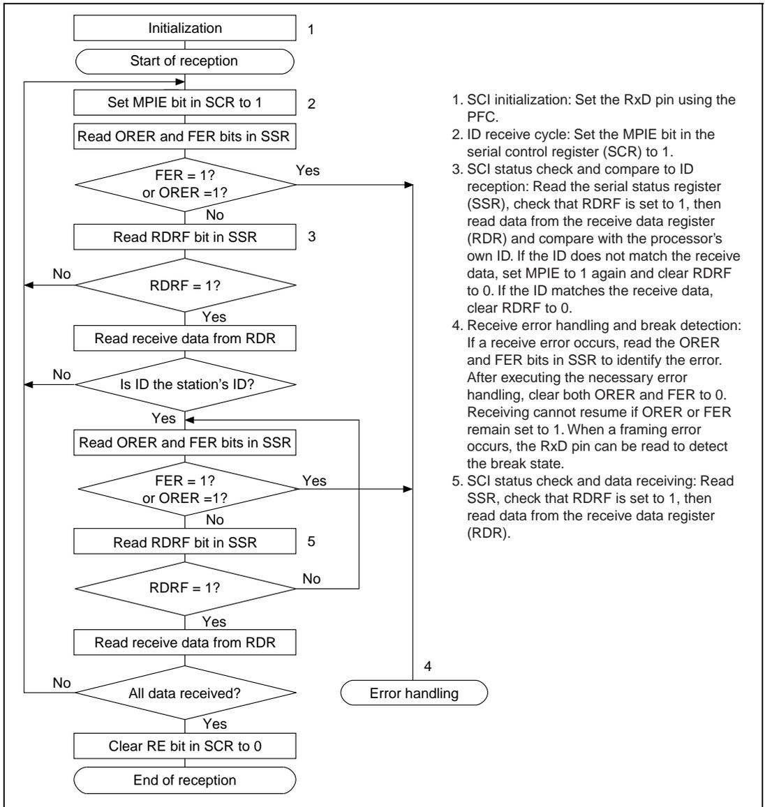
1. SCI initialization: Set the RxD pin using the PFC.
