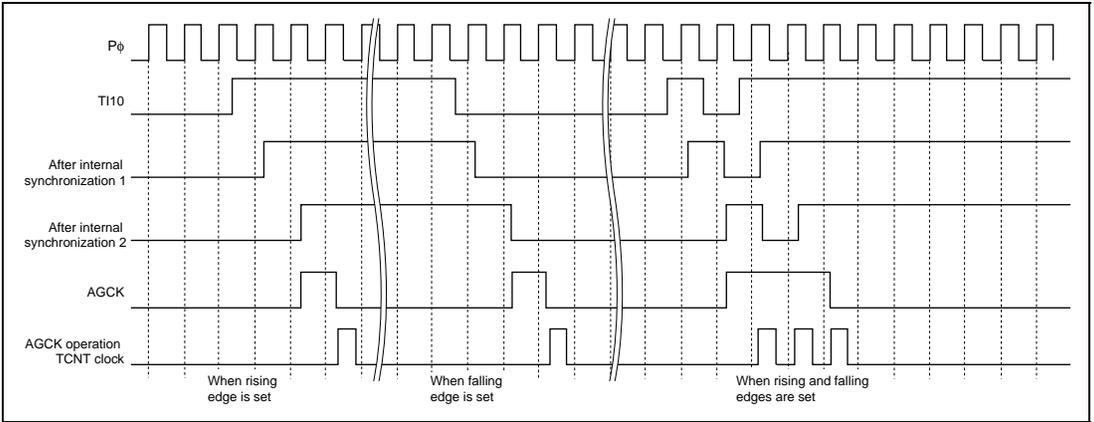
**Figure 11.26 Edge Input Operation (Without Noise Cancellation)**
