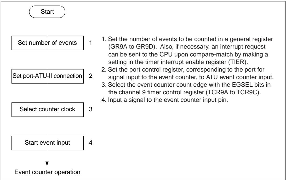
**Figure 11.61 Sample Setup Procedure for Event Counter Operation**
