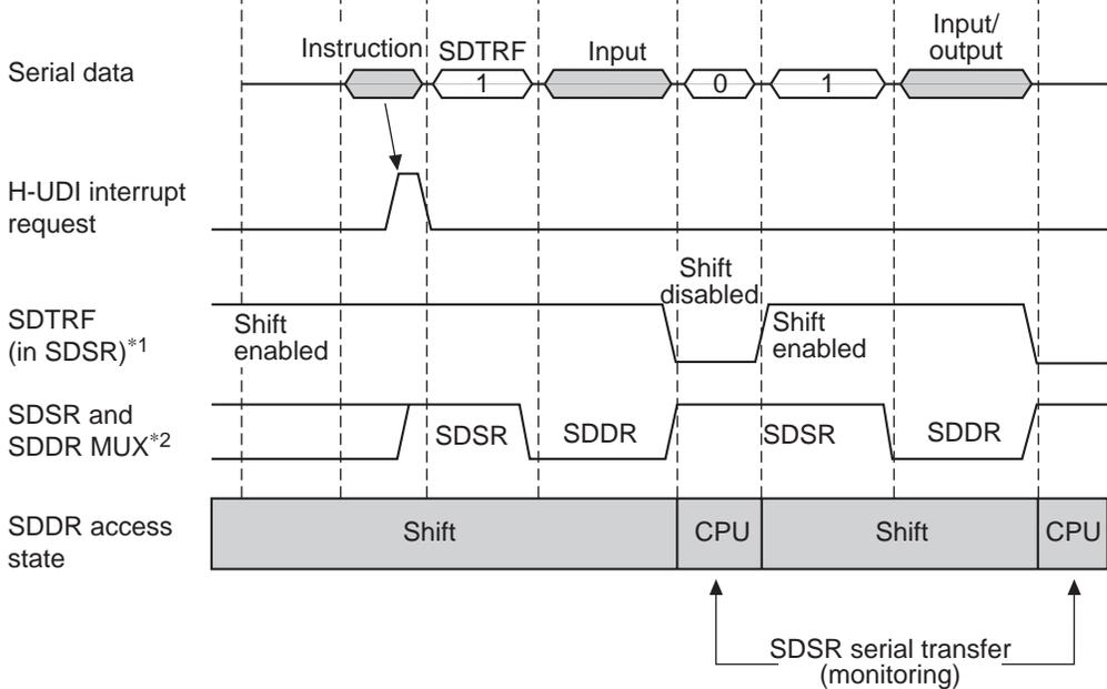
Notes: 1. SDTRF flag (in SDRS): Indicates whether SDDR access by the CPU or serial transfer data input/output to SDDR is possible.
