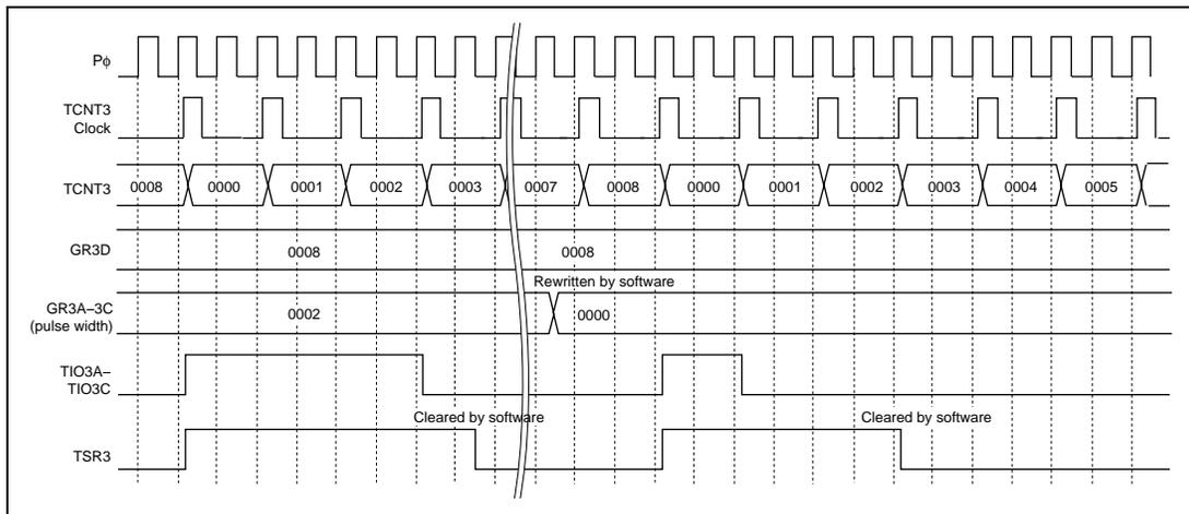
**Figure 11.23 Channel 3 to 5 PWM Mode Operation**
