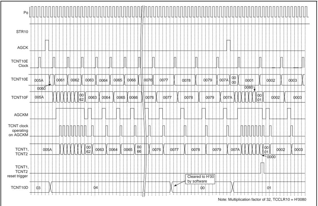
**Figure 11.35 TCNT10F Operation (End of Cycle, Acceleration, Deceleration)**
