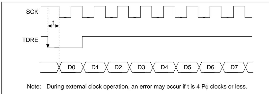
**Figure 15.25 Example of Synchronous Transmission with DMAC**
