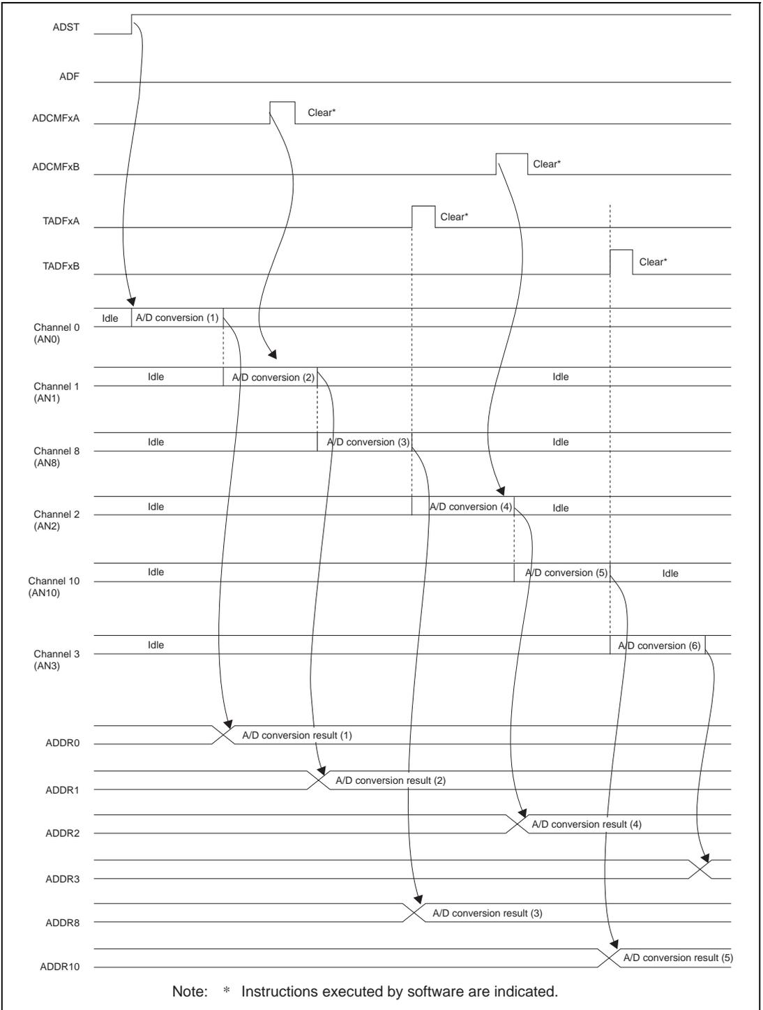
**Figure 18.3 Example of Multi-Trigger A/D Converter Operation**
