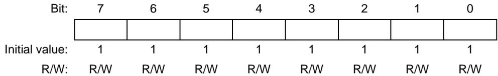
OCR10B is initialized to H'FF by a power-on reset, and in hardware standby mode and software standby mode.
