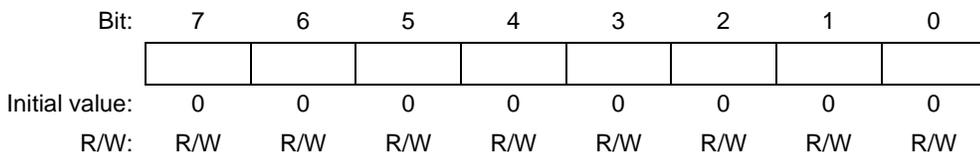
TCNT10B can only be accessed by a byte read or write.
