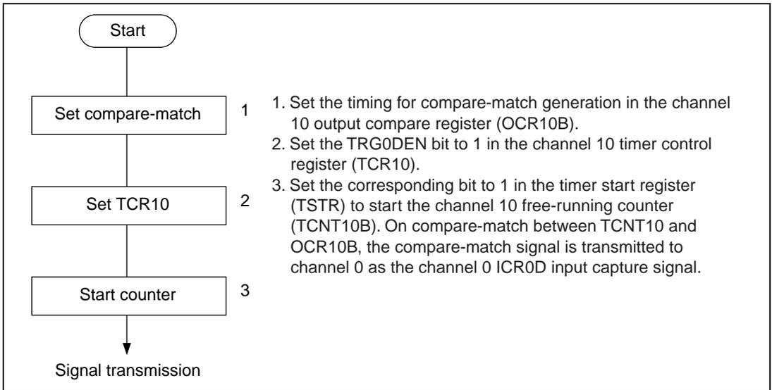
**Figure 11.55 Sample Setup Procedure for Compare-Match Signal Transmission**
