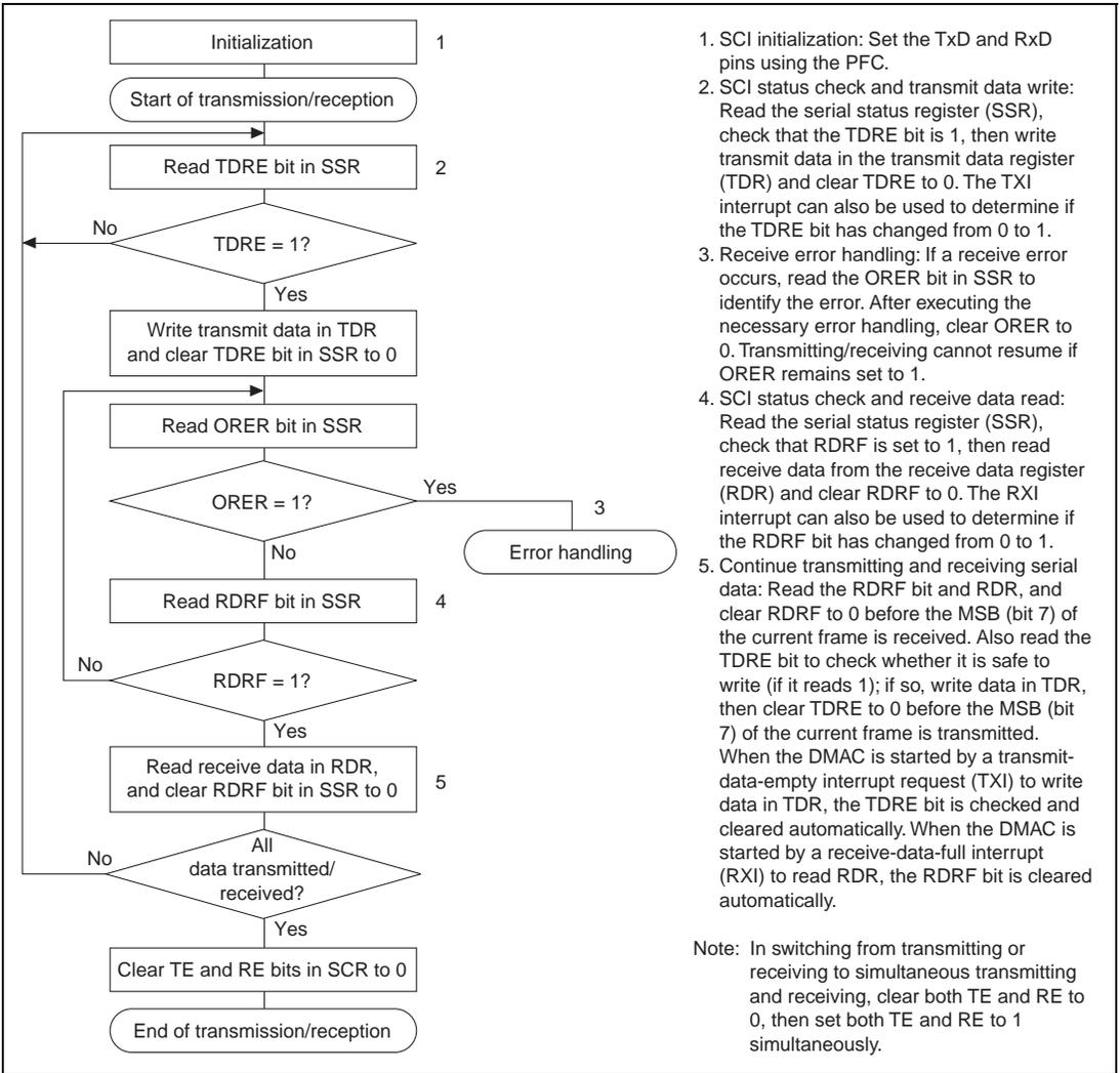
1. SCI initialization: Set the Tx/D and Rx/D pins using the PFC.
