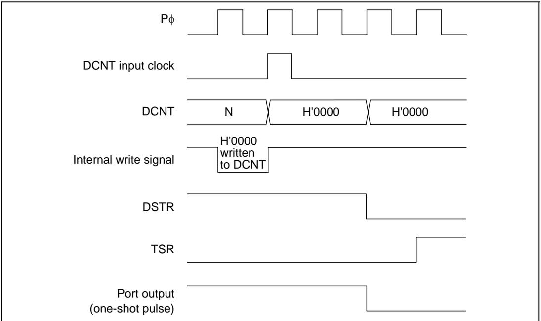
**Figure 11.70 Halting of a Down-Counter by the CPU**
