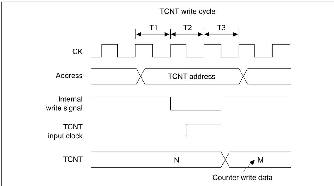
**Figure 13.8 Contention between TCNT Write and Increment**
