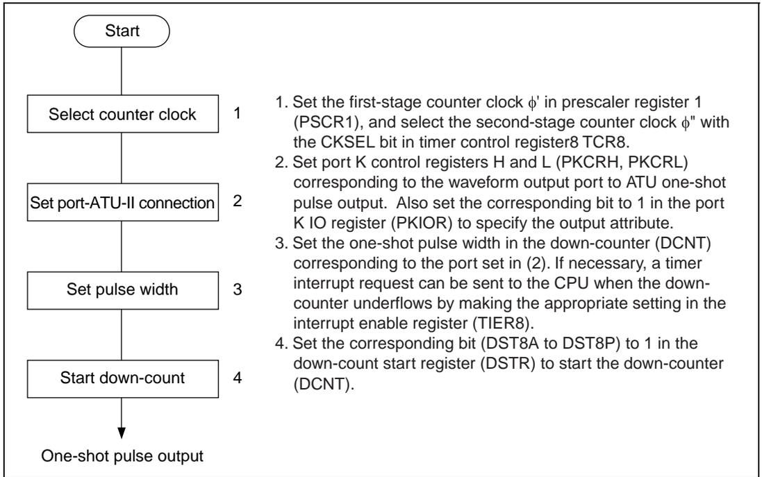
**Figure 11.56 Sample Setup Procedure for One-Shot Pulse Output**
