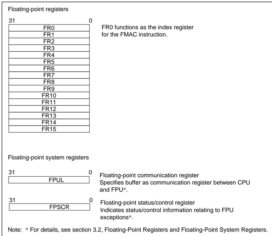
**Figure 3.1 Overview of Register Configuration
