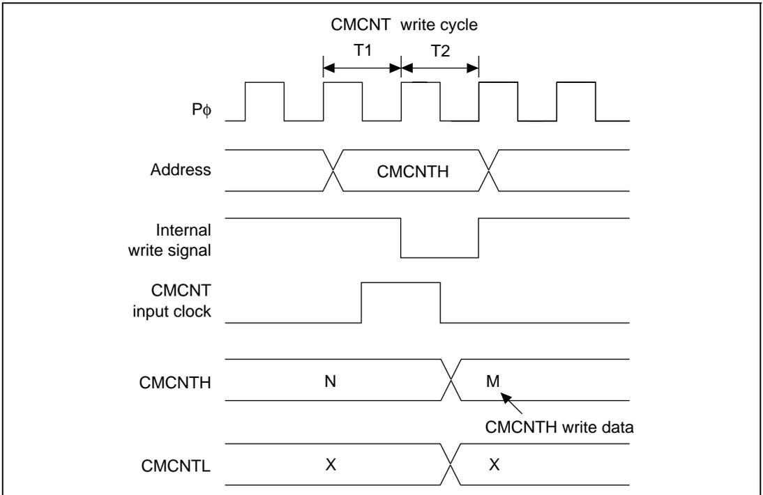
Figure 14.8 CMCNT Byte Write and Increment Contention
