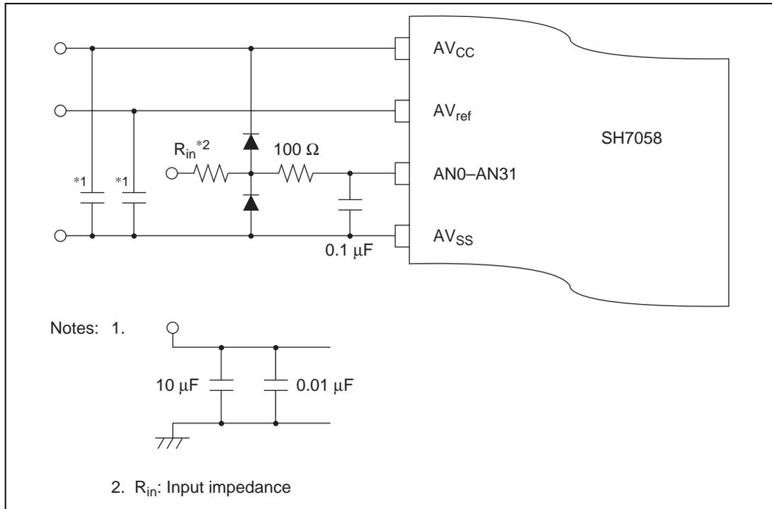
**Figure 17.9 Example of Analog Input Pin Protection Circuit**
