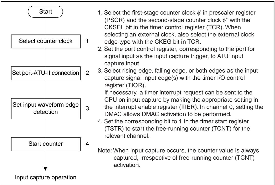
**Figure 11.53 Sample Setup Procedure for Input Capture**
