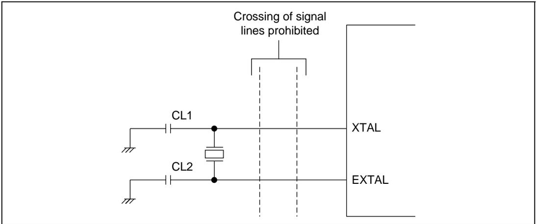
**Figure 5.8 Precautions for Oscillator Circuit System Board Design**
