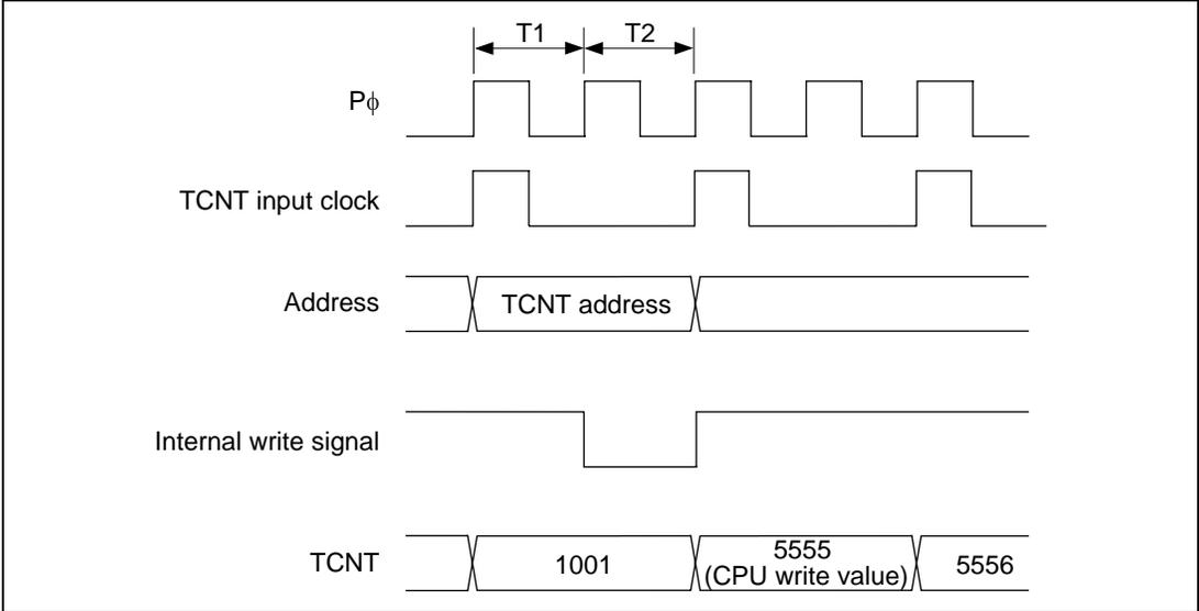
**Figure 11.65 Contention between TCNT Write and Increment**
