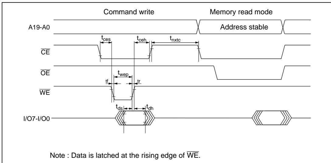
**Figure 23.32 Memory Read Timing after Command Write**
