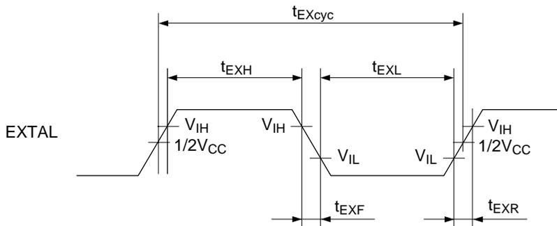
Note: EXTAL pin is  $V_{CC} = 3.3\text{ V} \pm 0.3\text{ V}$  power supply circuit.
