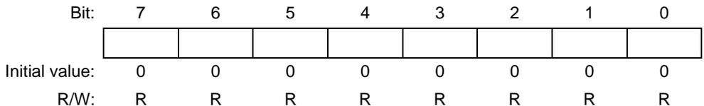
The receive data register (RDR) stores serial receive data. The SCI completes the reception of one byte of serial data by moving the received data from the receive shift register (RSR) into RDR for storage. RSR is then ready to receive the next data. This double buffering allows the SCI to receive data continuously.
