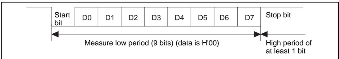
**Figure 23.7 Automatic Adjustment Operation of SCI Bit Rate**
