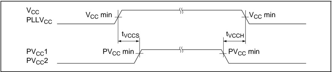
**Figure 27.1 Power-On/Off Timing**
