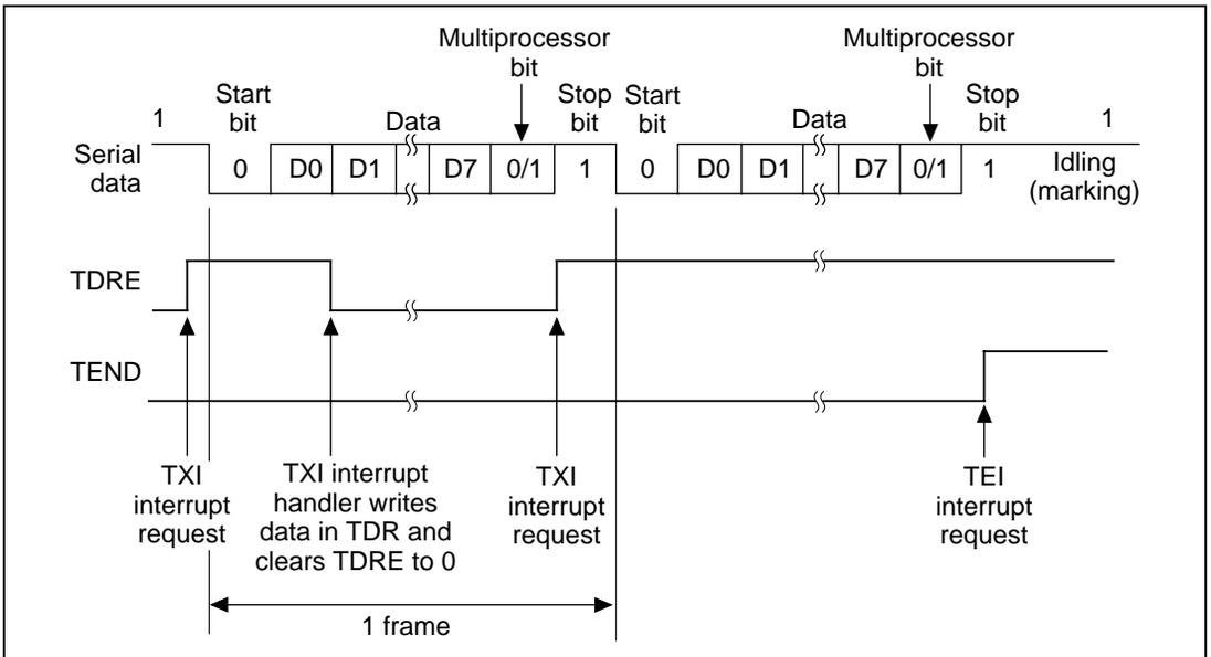
**Figure 15.12 SCI Multiprocessor Transmit Operation**
