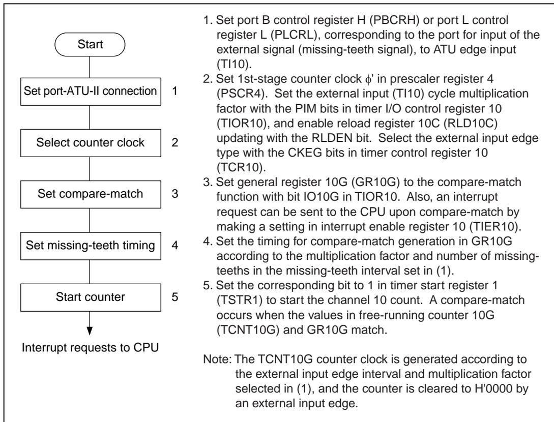
**Figure 11.63 Sample Setup Procedure for Missing-Teeth Detection**
