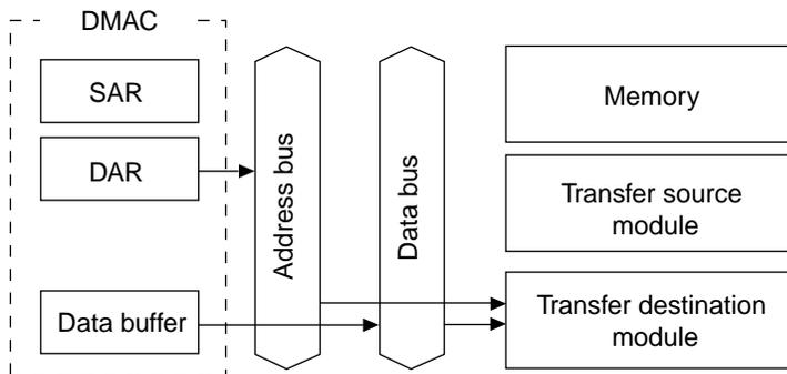
The DAR value is taken as the address, and data stored in the DMAC's data buffer is written to the transfer destination module.
