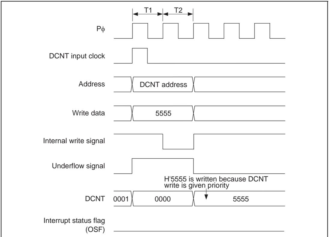
**Figure 11.72 Contention between DCNT Write and Underflow**
