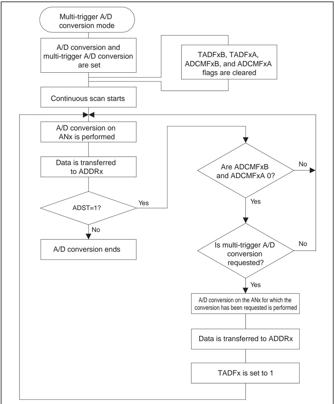
**Figure 18.4 Flowchart of Multi-Trigger A/D Converter Operation**
