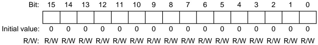
TCCLR10 is initialized to H'0000 by a power-on reset, and in hardware standby mode and software standby mode.
