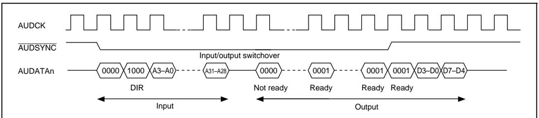
**Figure 20.5 Example of Read Operation (Byte Read)**
