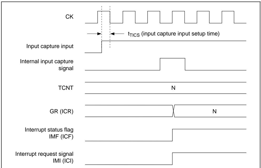
**Figure 11.37 IMF (ICF) Setting Timing in Input Capture**
