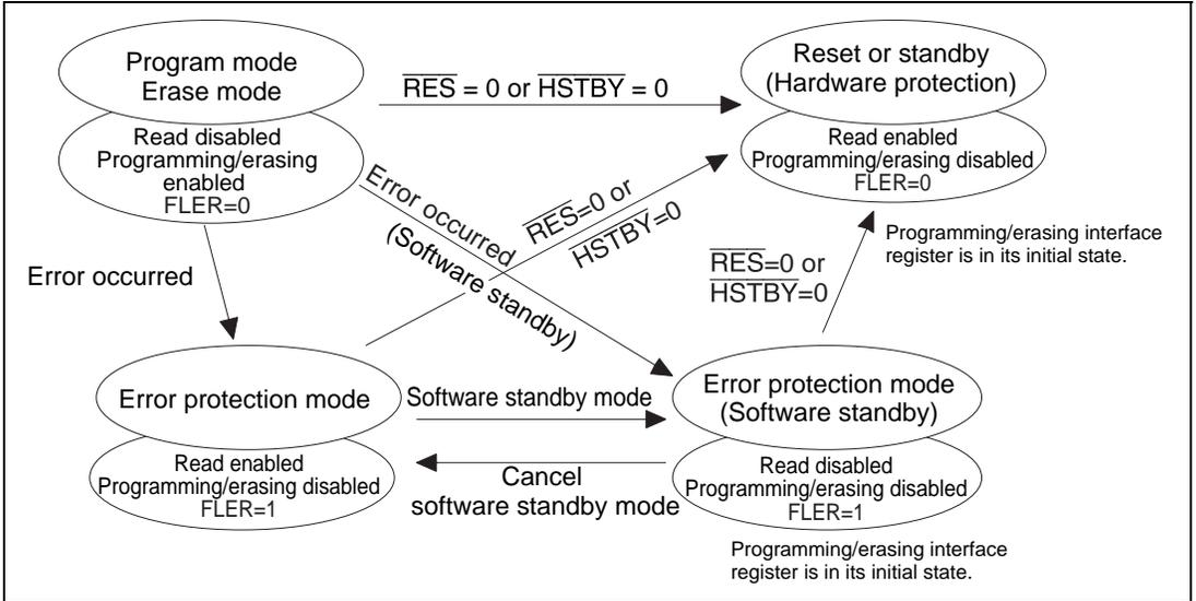
**Figure 23.16 Transitions to and from Error Protection State**
