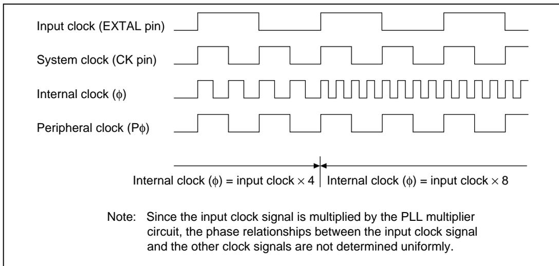
**Figure 5.2 Frequencies and Phases of Clock Signals**
