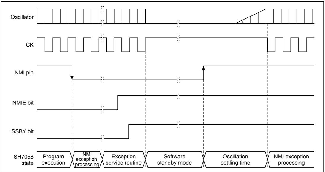
**Figure 25.3 Software Standby Mode NMI Timing (Application Example)**
