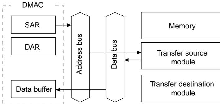
The SAR value is taken as the address, and data is read from the transfer source module and stored temporarily in the DMAC.
