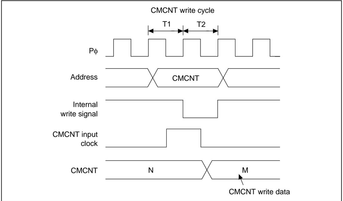
Figure 14.7 CMCNT Word Write and Increment Contention
