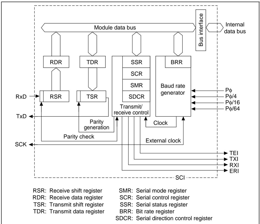
Figure 15.1 SCI Block Diagram
