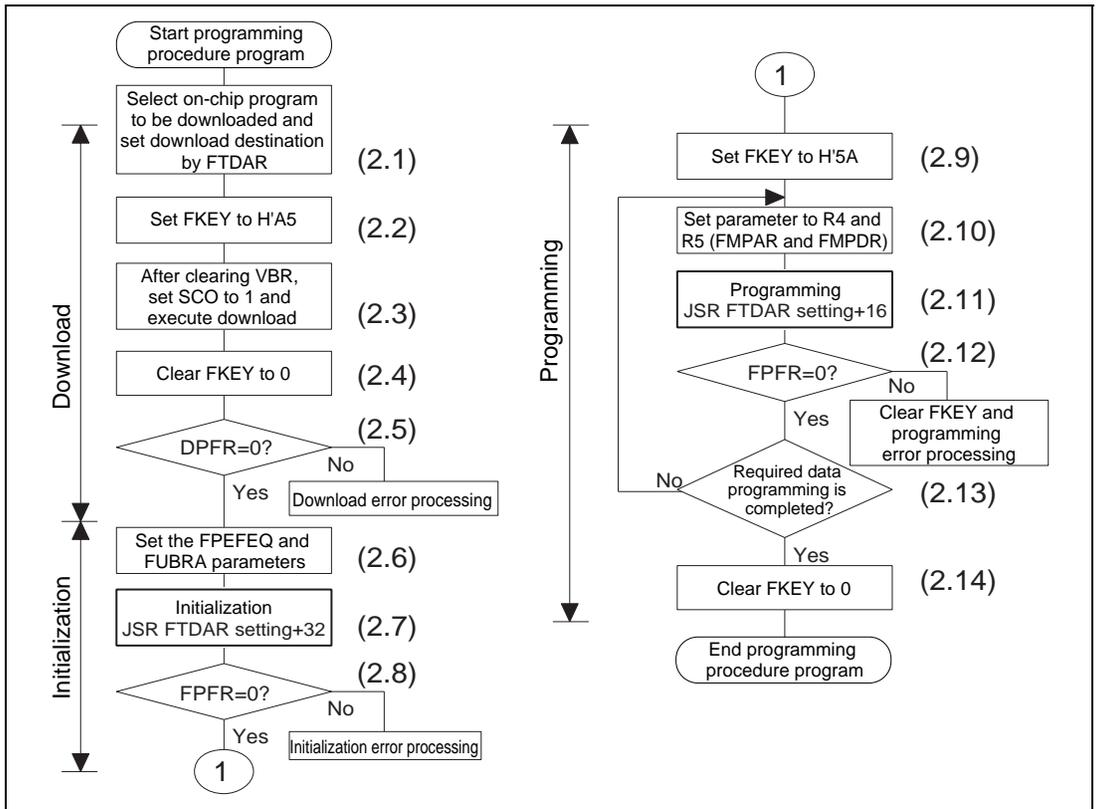
**Figure 23.11 Programming Procedure**
