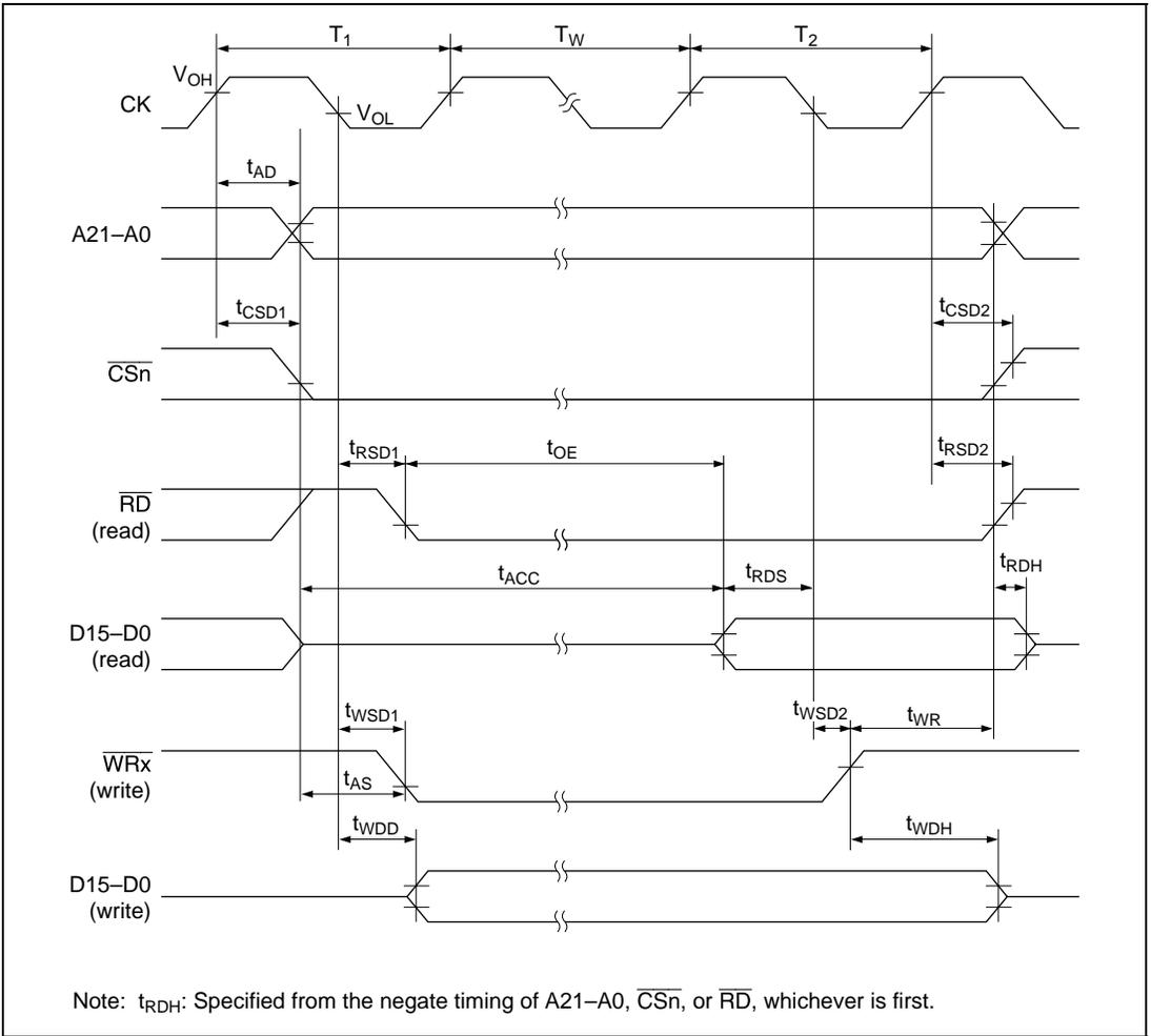
**Figure 27.10 Basic Cycle (One Software Wait)**
