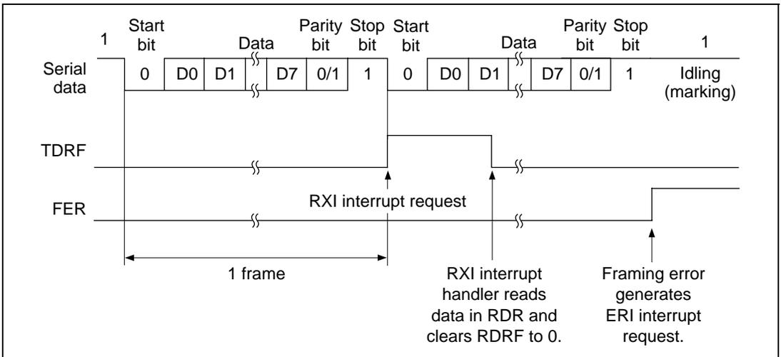
**Figure 15.9 SCI Receive Operation**
