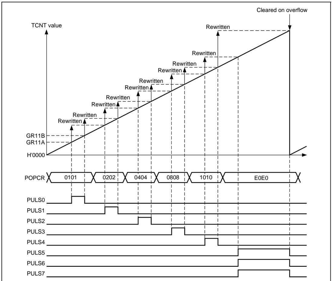
**Figure 12.4 Example of Advanced Pulse Controller Output Operation**
