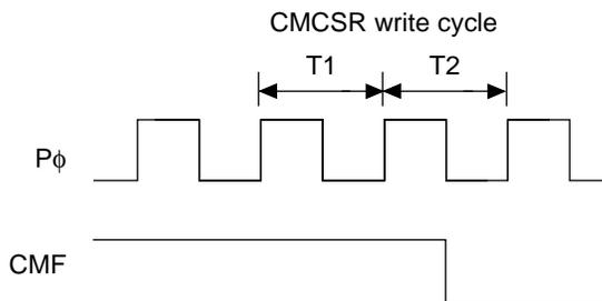
**Figure 14.5 Timing of CMF Clear by the CPU**
