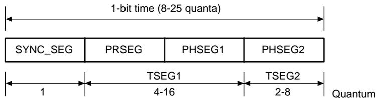
**SYNC\_SEG:** Segment for establishing synchronization of nodes on the CAN bus. (Normal bit edge transitions occur in this segment.)
