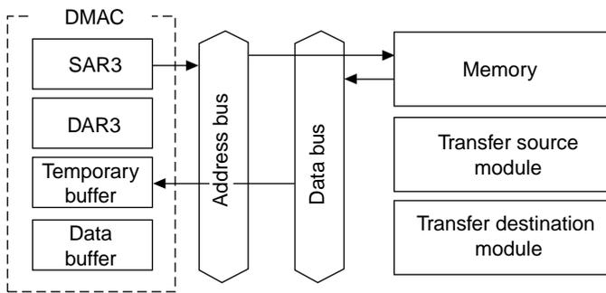
The SAR3 value is taken as the address, memory data is read, and the value is stored in the temporary buffer. Since the value read at this time is used as the address, it must be 32 bits. If data bus is 16 bits wide when accessed to an external memory space, two bus cycles are necessary.
