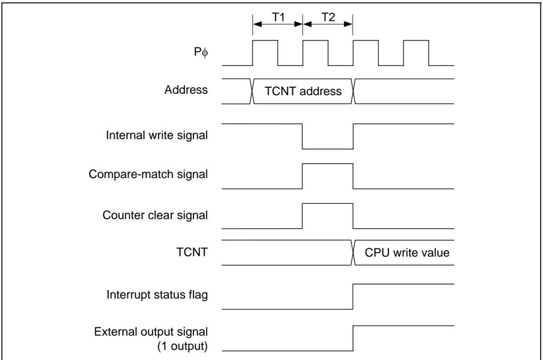
**Figure 11.64** Contention between TCNT Write and Clear
