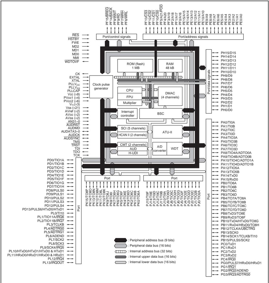
**Figure 1.1 Block Diagram**
