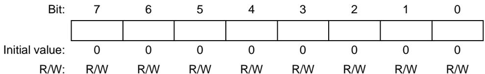
TCNT10H is initialized to H'00 by a power-on reset, and in hardware standby mode and software standby mode.
