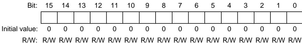
RLDR8 is a 16-bit readable/writable register. When reload is enabled (by a setting in RL DENR) and DSTR8I to DSTR8P are set to 1 by the channel 2 compare-match signal one-shot pulse start trigger, the reload register value is transferred to DCNT8I to DCNT8P before the down-count is started. The reload register value is not transferred when the one-shot pulse function is used independently, without linkage to channel 2, or when down-counters DCNT8I to DCNT8P are running.
