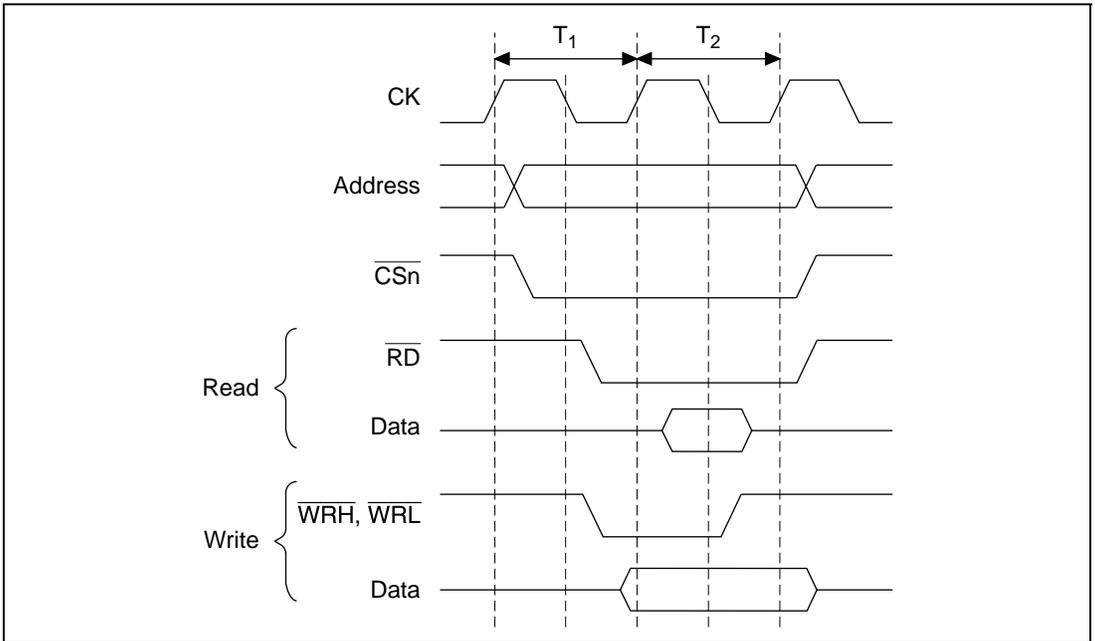
Figure 9.3 Basic Timing of External Space Access
