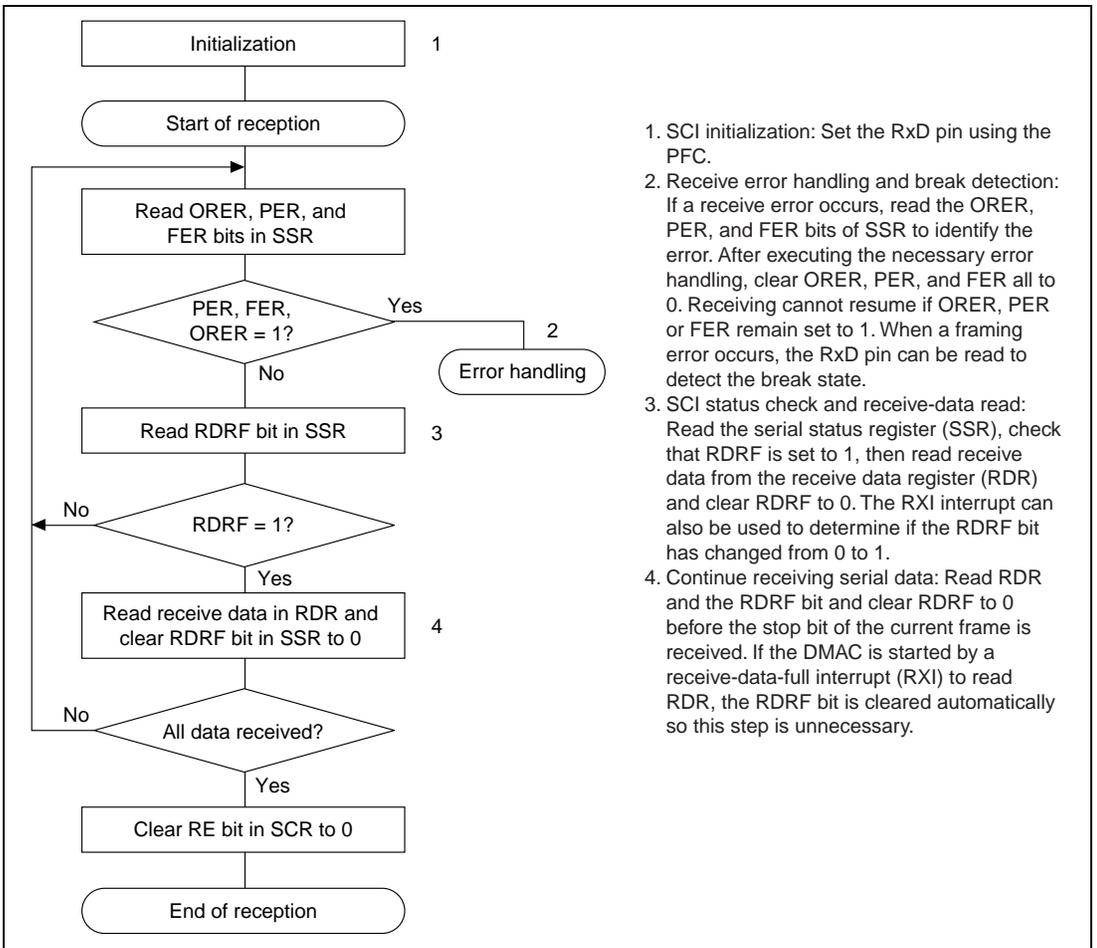
1. SCI initialization: Set the RxD pin using the PFC.
