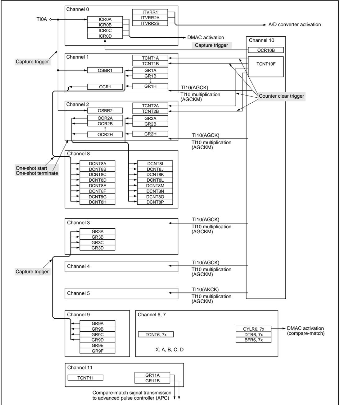
**Figure 11.11 Inter-Module Communication Signals**
