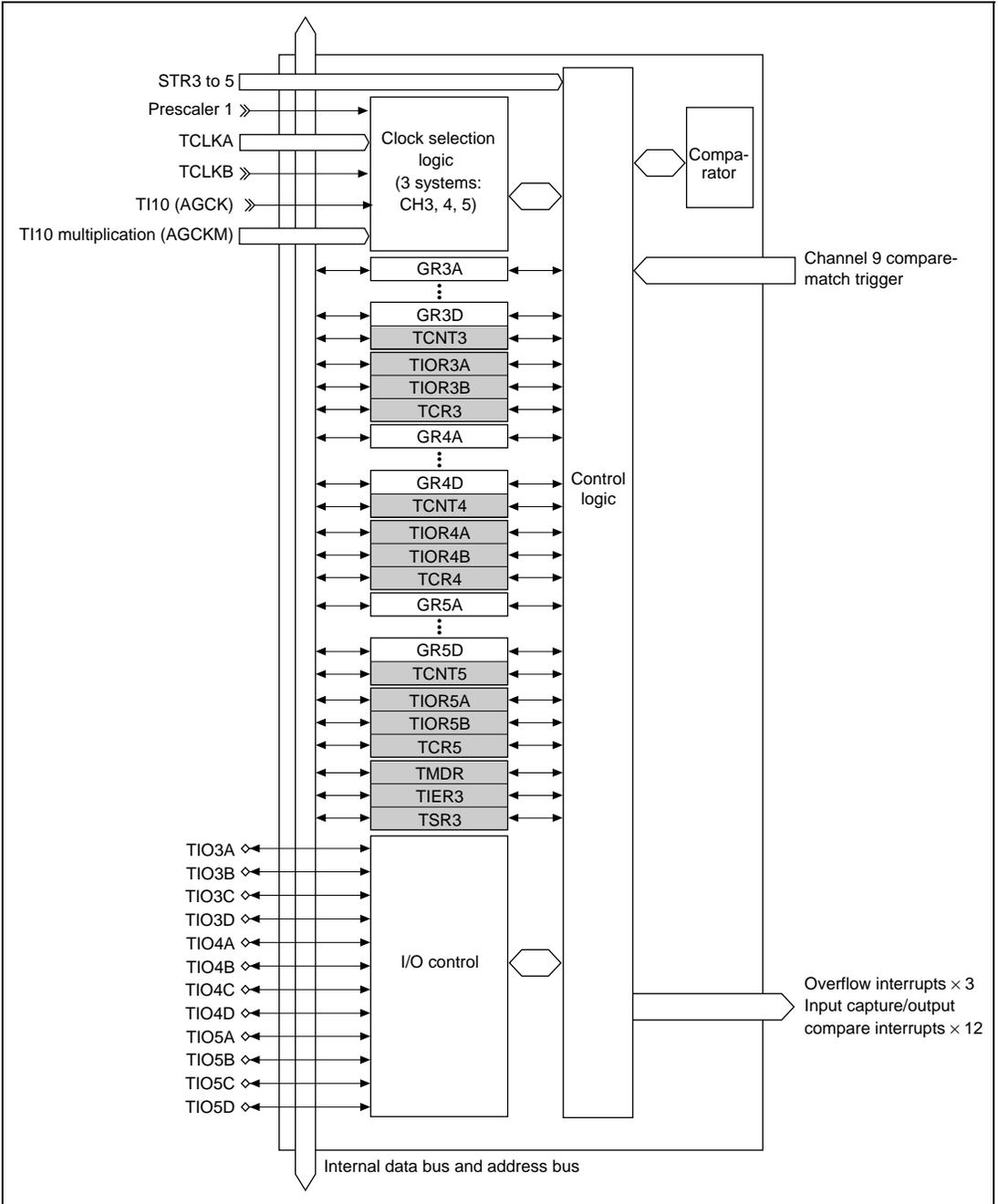
**Figure 11.5 Block Diagram of Channels 3 to 5**
