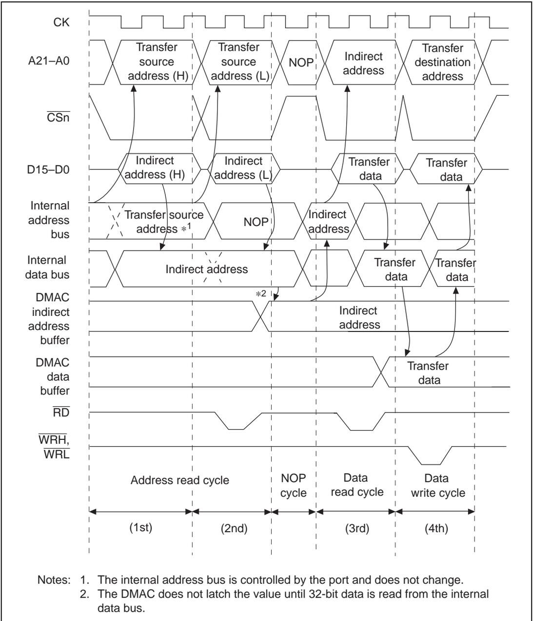
**Figure 10.6 Dual Address Mode and Indirect Address Transfer Timing Example 1**
