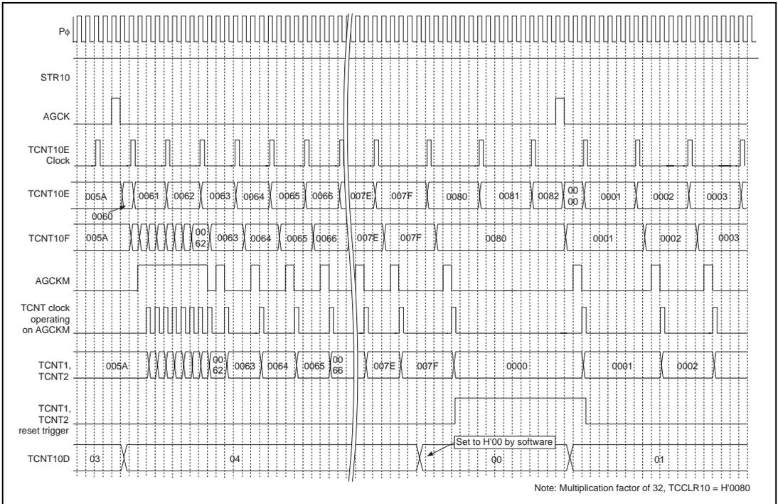
**Figure 11.36 TCNT10F Operation (End of Cycle, Steady-State)**
