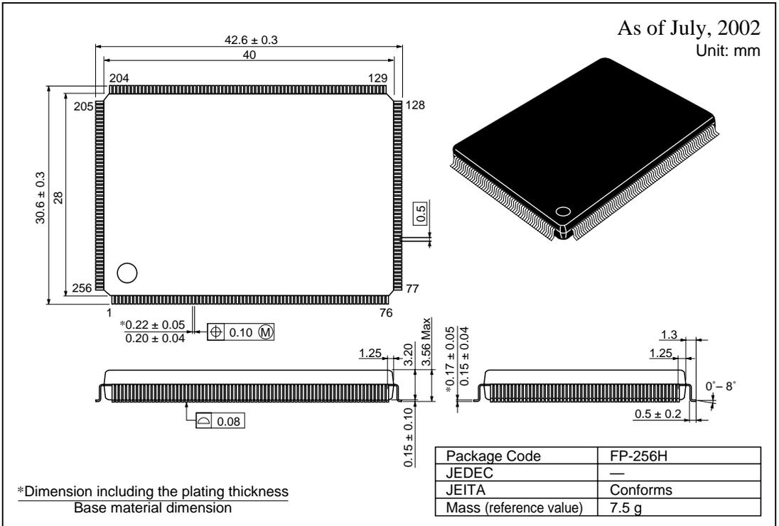
**Figure D.1 SH7058 Package Dimensions (FP-256H)**
