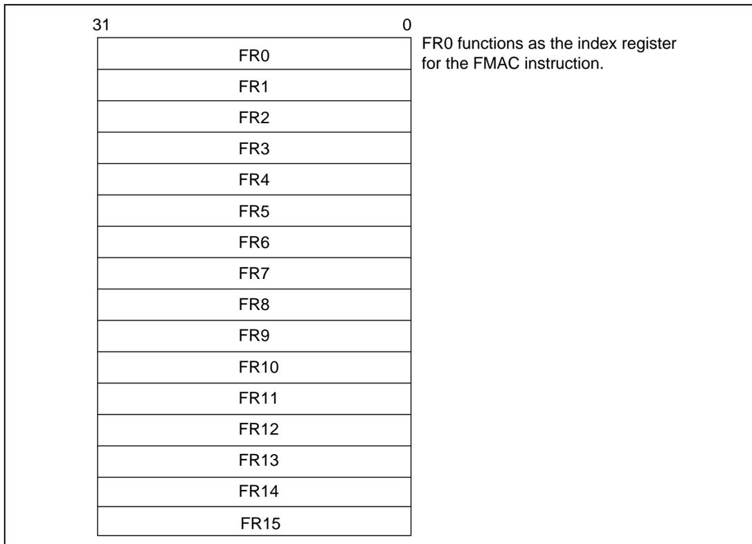
**Figure 2.4 Floating-Point Registers**
