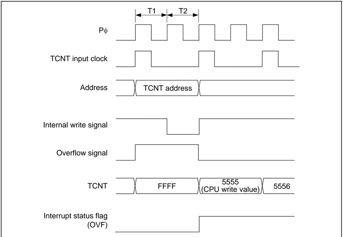
**Figure 11.66 Contention between TCNT Write and Overflow**
