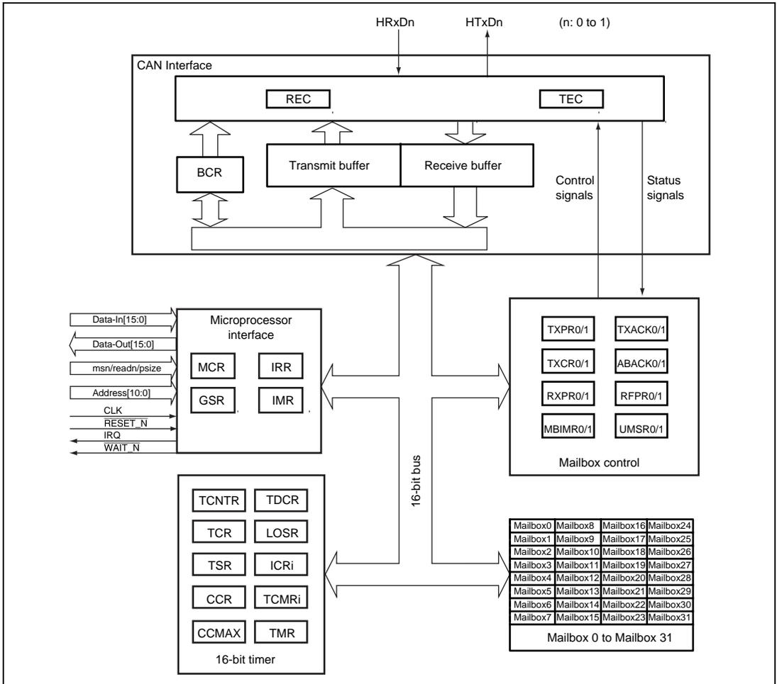
Figure 16.1 Block Diagram of HCAN-II (for One Channel)
