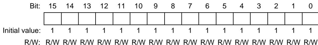
The DTR registers are 16-bit readable/writable registers used for PWM duty storage.
