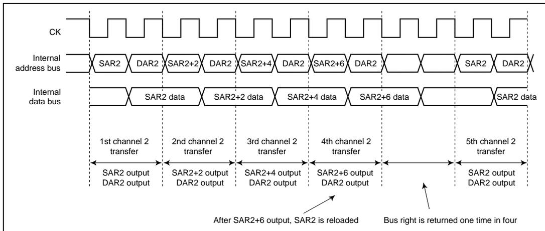
**Figure 10.11 Source Address Reload Function Timing Chart**
