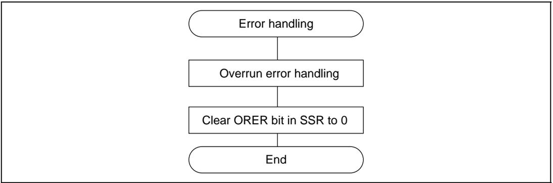
**Figure 15.21 Sample Flowchart for Serial Receiving (2)**
