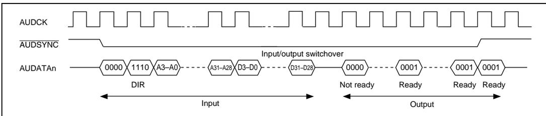
**Figure 20.6 Example of Write Operation (Longword Write)**
