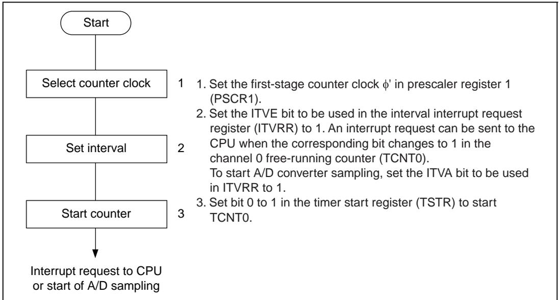
**Figure 11.58 Sample Setup Procedure for Interval Timer Operation**
