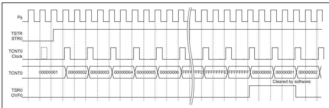
**Figure 11.13 Free-Running Counter Operation and Overflow Timing**
