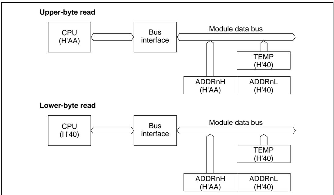
Figure 17.2 A/D Data Register Access Operation (Reading H'AA40)
