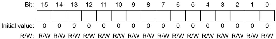
RLD10C is initialized to H'0000 by a power-on reset, and in hardware standby mode and software standby mode.
