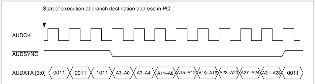
**Figure 20.2 Example of Data Output (32-Bit Output)**
