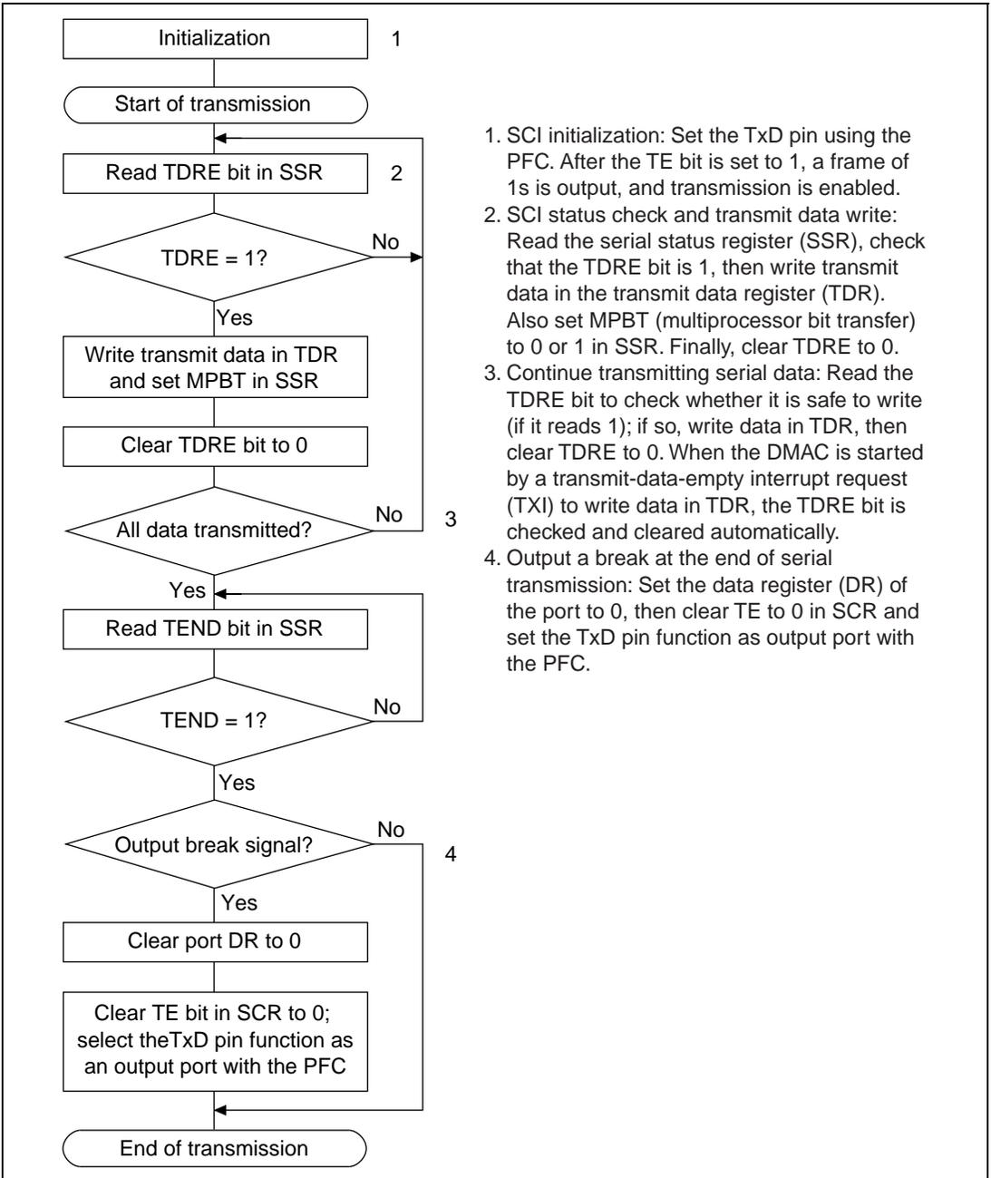
1. SCI initialization: Set the TxD pin using the PFC. After the TE bit is set to 1, a frame of 1s is output, and transmission is enabled.
