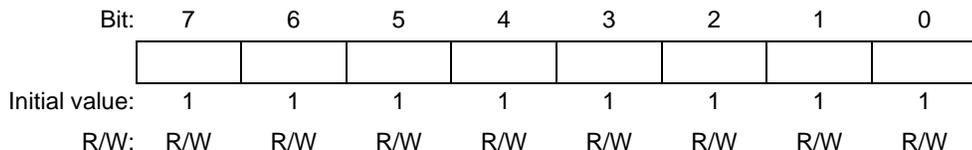
The bit rate register (BRR) is an 8-bit register that, together with the baud rate generator clock source selected by the CKS1 and CKS0 bits in the serial mode register (SMR), determines the serial transmit/receive bit rate.
