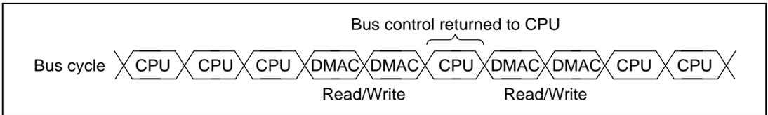
**Figure 10.8 DMA Transfer Timing Example in Cycle-Steal Mode**
