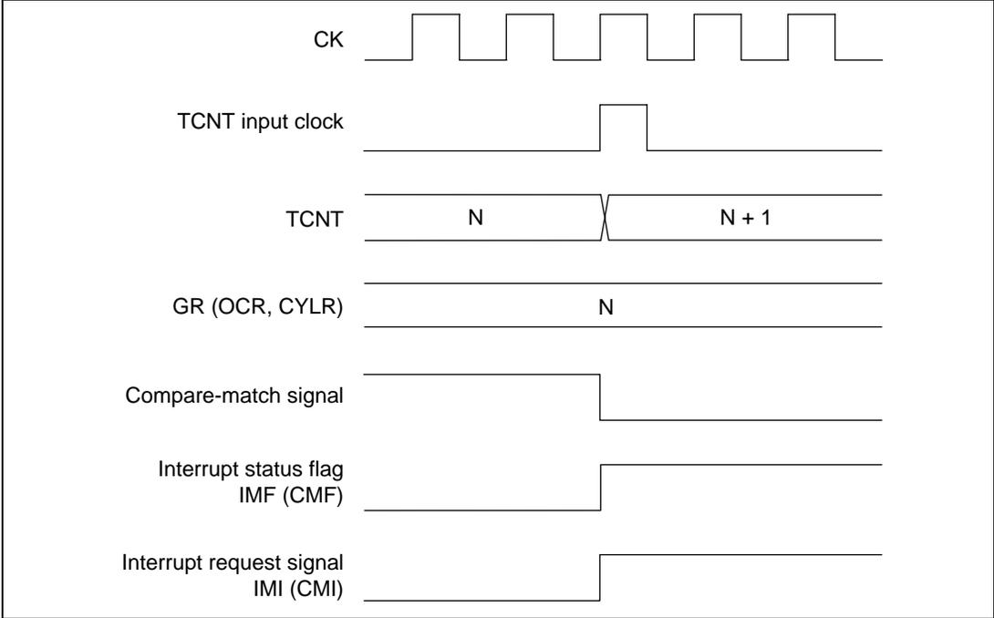
**Figure 11.38 IMF (CMF) Setting Timing in Compare-Match**
