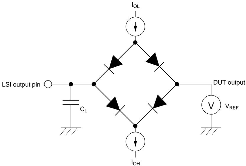
$C_L$  is a total value that includes the measuring instrument capacitance.
