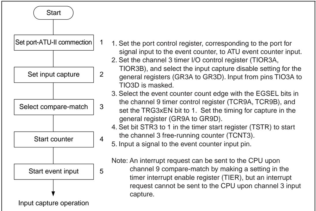
**Figure 11.62 Sample Setup Procedure for Compare-Match Signal Transmission**
