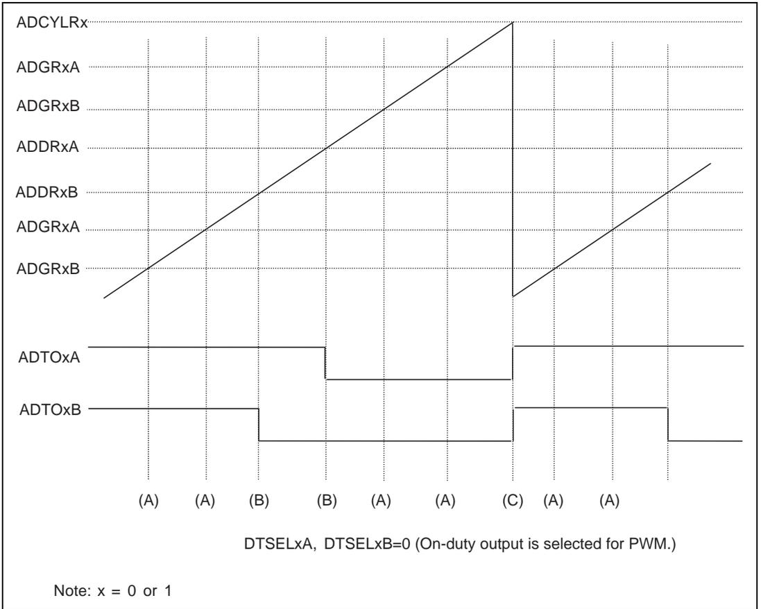
**Figure 18.5 Example of Output Waveform from MTAD PWM**
