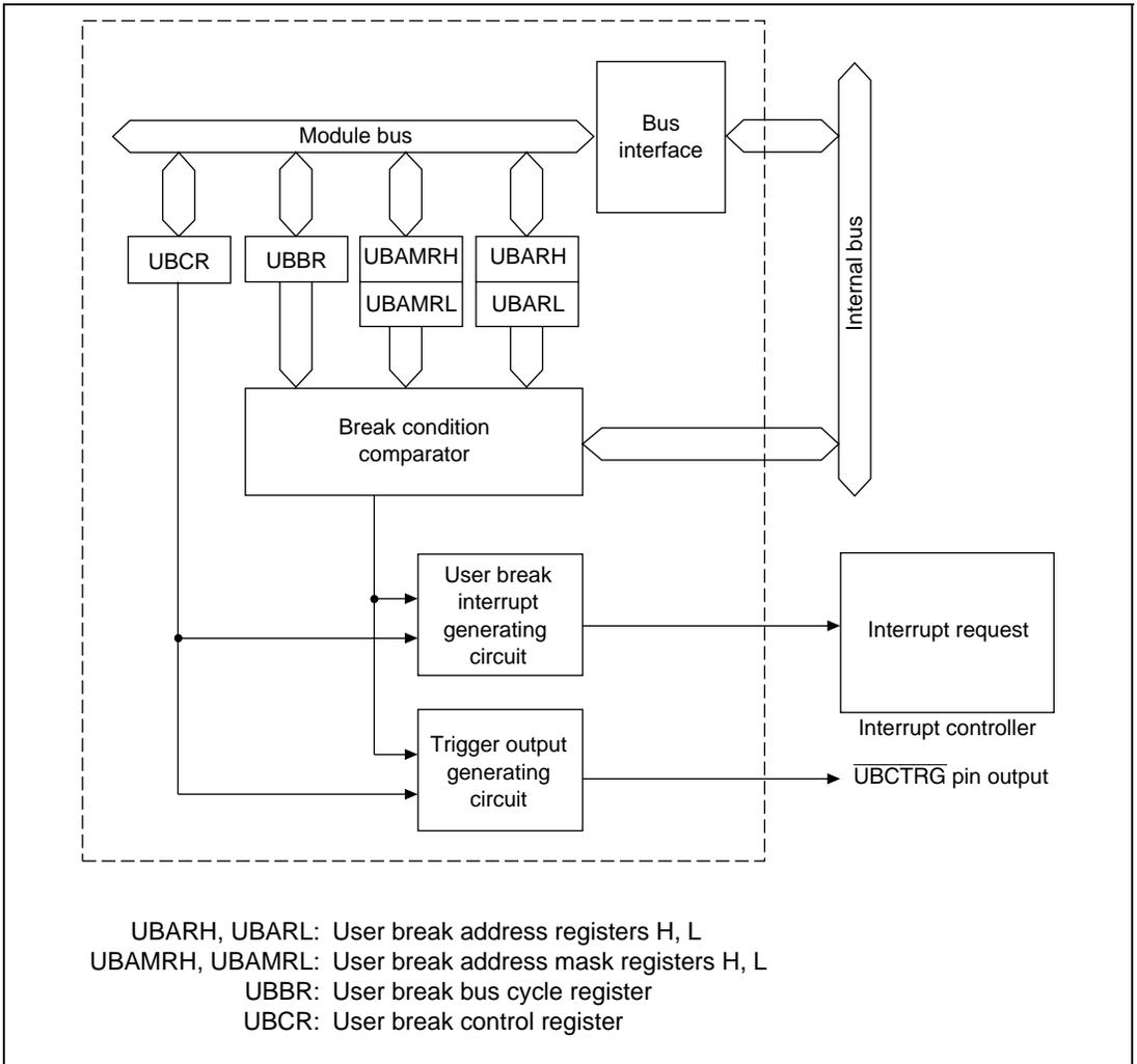
**Figure 8.1 User Break Controller Block Diagram**
