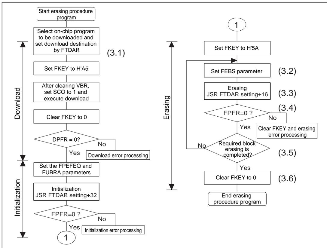
**Figure 23.12 Erasing Procedure**
