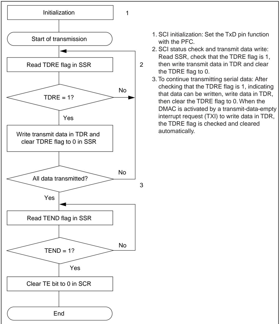
1. SCI initialization: Set the TxD pin function with the PFC.
