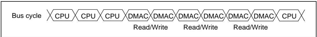
**Figure 10.9 DMA Transfer Timing Example in Burst Mode**
