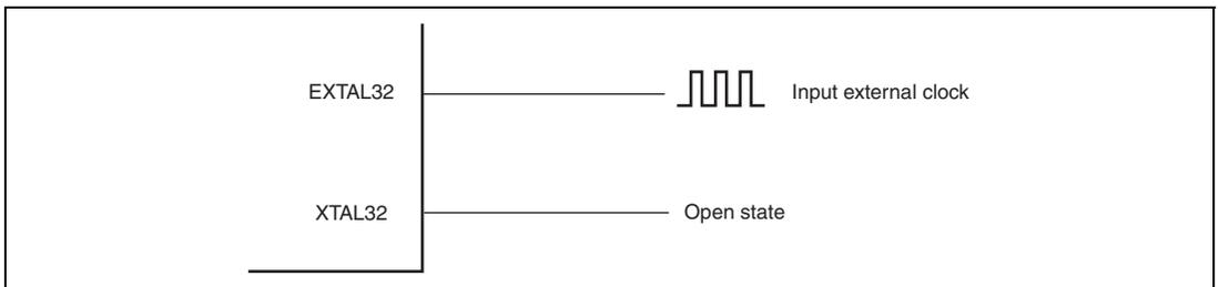
**Figure 5.6 Example of Connecting an External Clock**
