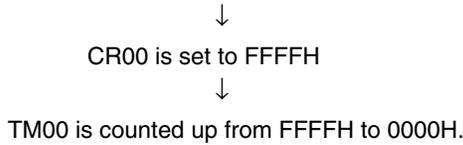
**Figure 8-36. Operation Timing of OVF00 Flag**
