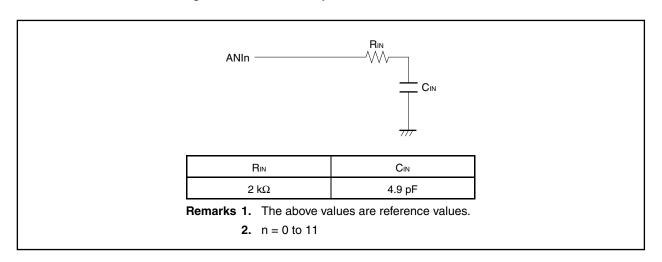
Figure 13-14. Internal Equivalent Circuit of ANIn Pin
