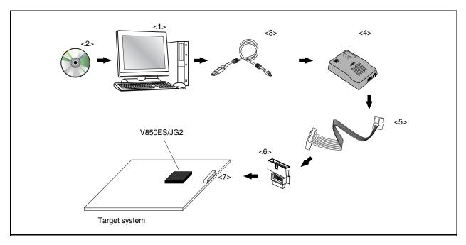
Figure A-3. On-Chip Emulation System Configuration
