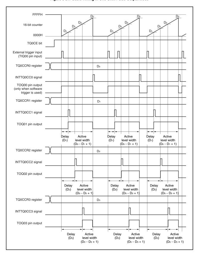
Figure 8-21. Basic Timing in One-Shot Pulse Output Mode
