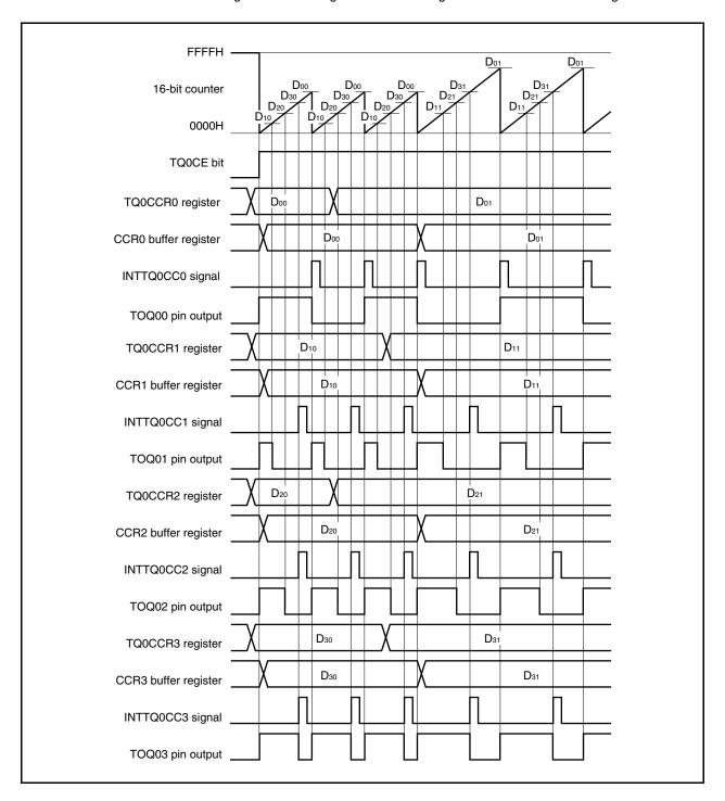
To transfer data from the TQ0CCRm register to the CCRm buffer register, the TQ0CCR1 register must be written
