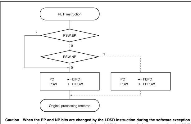
Caution When the EP and NP bits are changed by the LDSR instruction during the software exception processing, in order to restore the PC and PSW correctly during recovery by the RETI instruction, it is necessary to set the EP bit back to 1 and the NP bit back to 0 using the LDSR instruction immediately before the RETI instruction.
