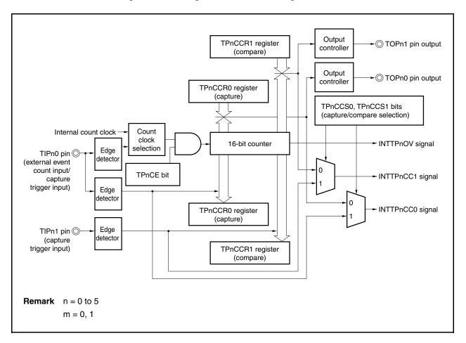
Figure 7-28. Configuration in Free-Running Timer Mode
