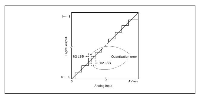
Figure 13-17. Quantization Error
