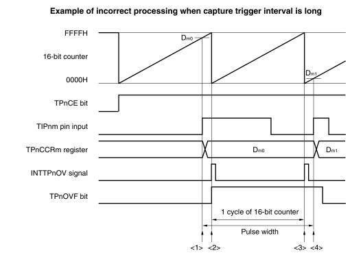
The following problem may occur when long pulse width is measured in the free-running timer mode.
