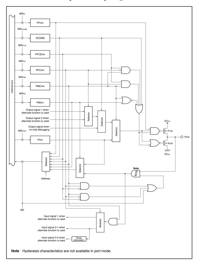
Figure 4-23. Block Diagram of Type U-7
