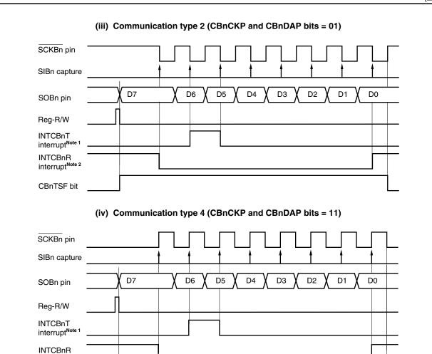
**Notes 1.** The INTCBnT interrupt is set when the data written to the CBnTX register is transferred to the data shift register in the continuous transmission or continuous transmission/reception modes. In the single transmission or single transmission/reception modes, the INTCBnT interrupt request signal is not generated, but the INTCBnR interrupt request signal is generated upon end of communication.
