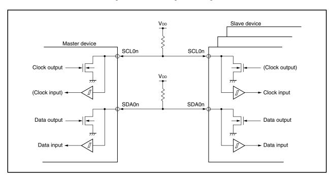
Figure 17-6. Pin Configuration Diagram
