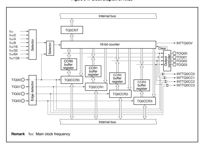
Figure 8-1. Block Diagram of TMQ0
