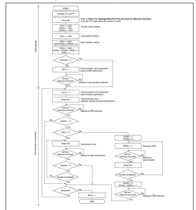
Figure 17-18. Master Operation in Single Master System
