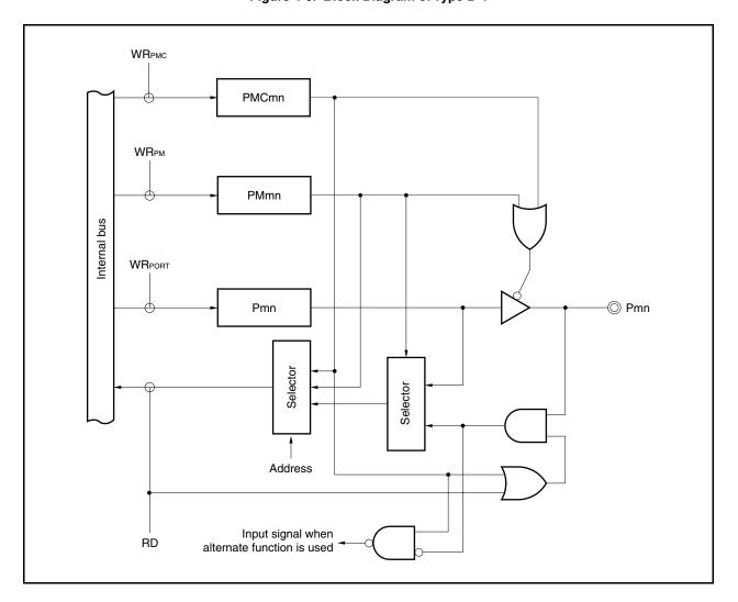
Figure 4-6. Block Diagram of Type D-1
