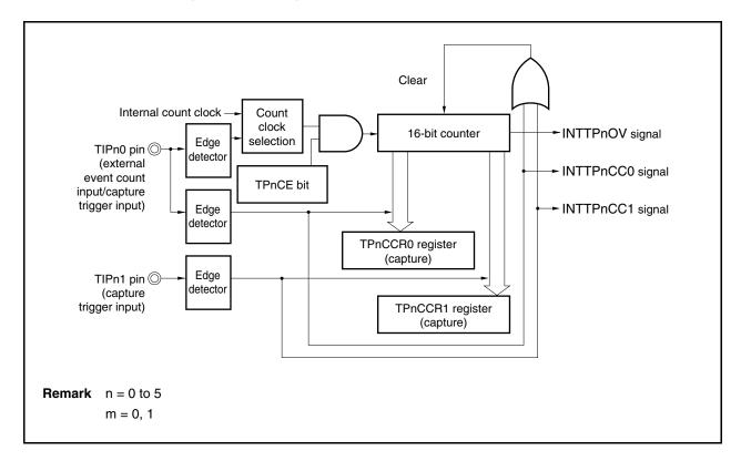
Figure 7-34. Configuration in Pulse Width Measurement Mode
