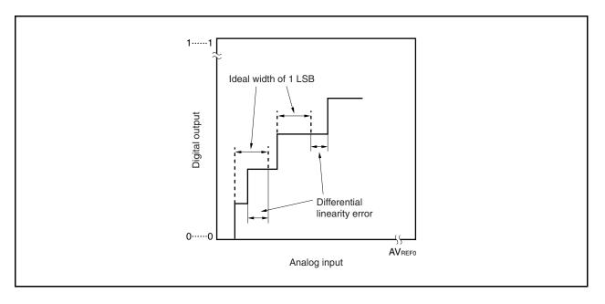
Figure 13-20. Differential Linearity Error
