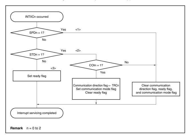
Figure 17-22. Slave Operation Flowchart (2)
