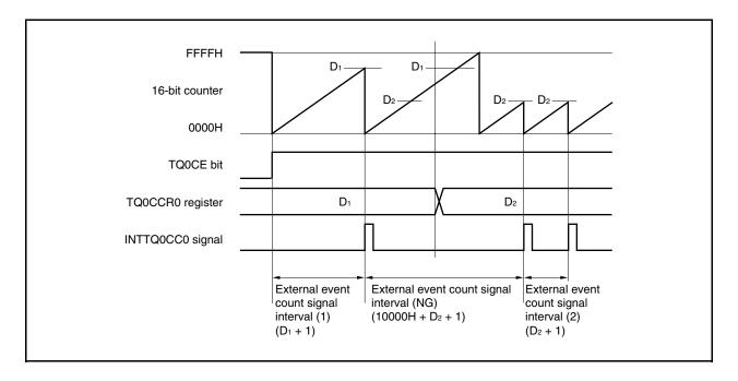
If the value of the TQ0CCR0 register is changed from  $D_1$  to  $D_2$  while the count value is greater than  $D_2$  but less than  $D_1$ , the count value is transferred to the CCR0 buffer register as soon as the TQ0CCR0 register has been rewritten. Consequently, the value that is compared with the 16-bit counter is  $D_2$ .
