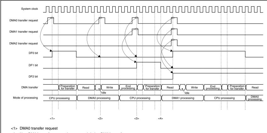
Figure 18-4. Period in Which DMA Transfer Request Is Ignored (2)
