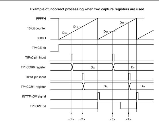
The following problem may occur when two pulse widths are measured in the free-running timer mode.
