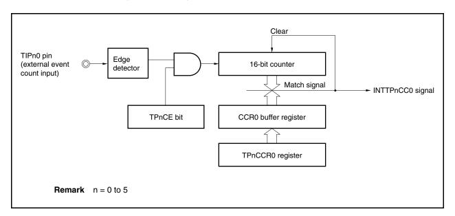
Figure 7-9. Configuration in External Event Count Mode
