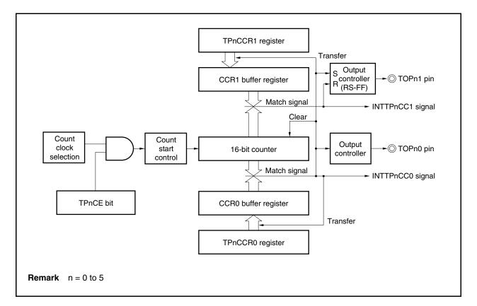
Figure 7-24. Configuration in PWM Output Mode
