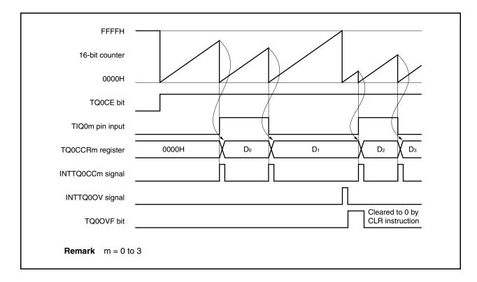
Figure 8-35. Basic Timing in Pulse Width Measurement Mode
