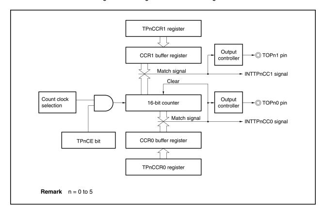
If the set value of the TPnCCR1 register is less than the set value of the TPnCCR0 register, the INTTPnCC1 signal is generated once per cycle. At the same time, the output of the TOPn1 pin is inverted. The TOPn1 pin outputs a square wave with the same cycle as that output by the TOPn0 pin.
