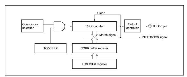
Figure 8-2. Configuration of Interval Timer
