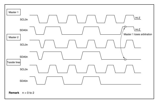
Figure 17-14. Arbitration Timing Example
