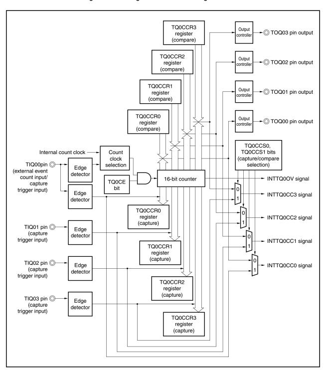
When the TQ0CE bit is set to 1, 16-bit timer/event counter Q starts counting, and the output signals of the TQ000 to TQQ03 pins are inverted. When the count value of the 16-bit counter later matches the set value of the TQ0CCRm register, a compare match interrupt request signal (INTTQ0CCm) is generated, and the output signal of the TQ00m pin is inverted.
