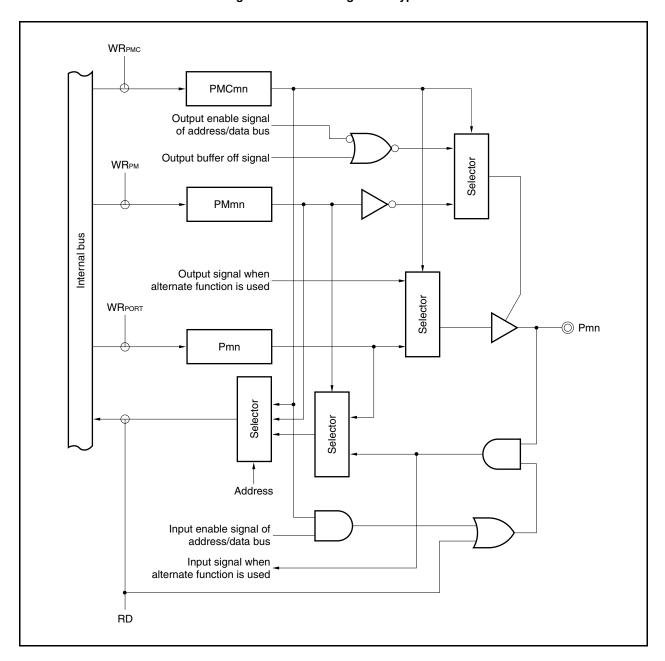
Figure 4-8. Block Diagram of Type D-3
