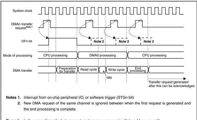
Figure 18-3. Period in Which DMA Transfer Request Is Ignored (1)
