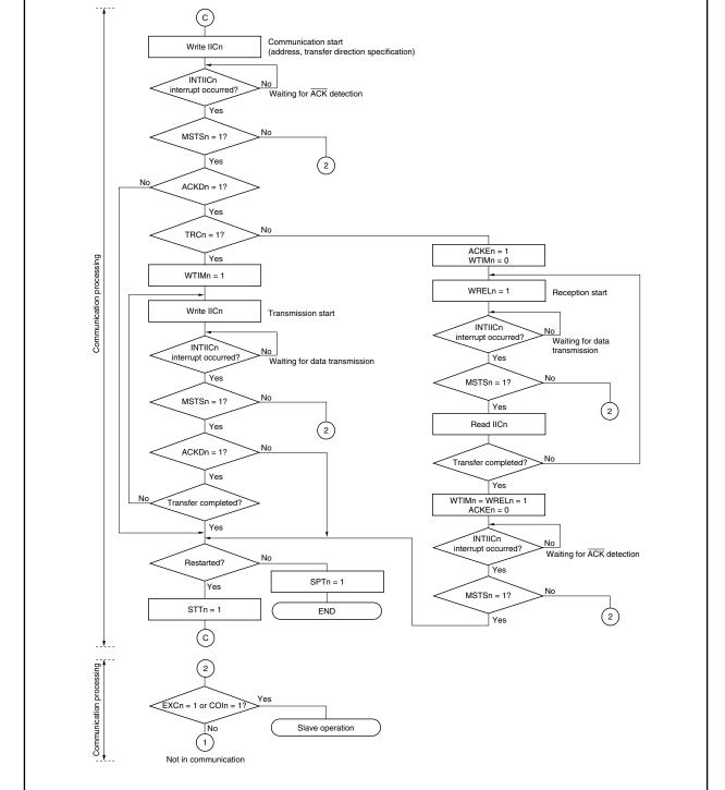
Figure 17-19. Master Operation in Multimaster System (3/3)
