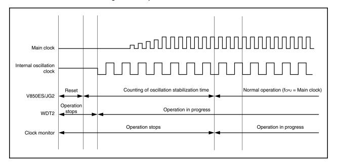
Figure 22-5. Operation After Reset Release
