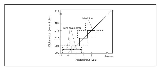
Figure 13-18. Zero-Scale Error
