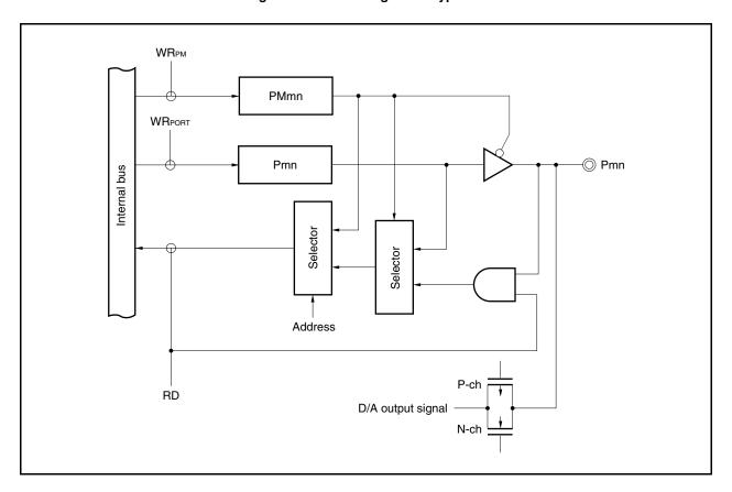
Figure 4-4. Block Diagram of Type A-2
