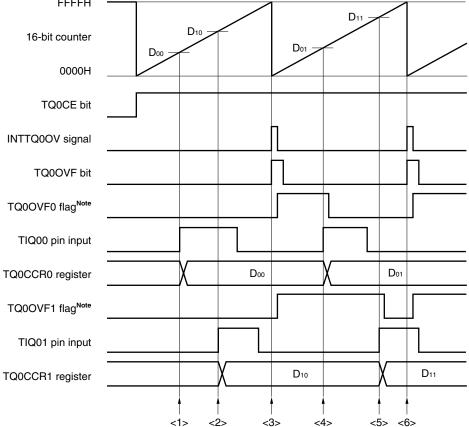
Note The TQ0OVF0 and TQ0OVF1 flags are set on the internal RAM by software.
