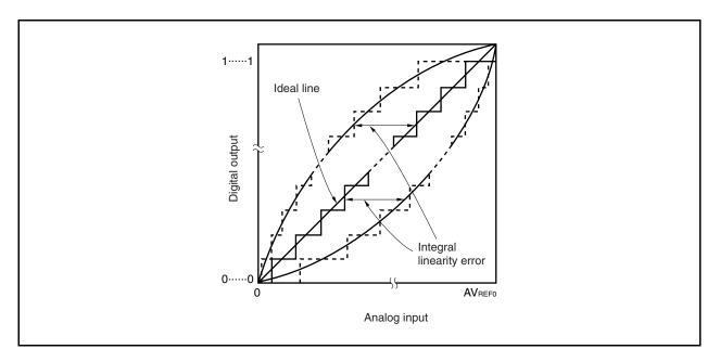
Figure 13-21. Integral Linearity Error
