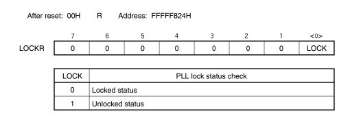
Caution The LOCK register does not reflect the lock status of the PLL in real time. The set/clear conditions are as follows.
