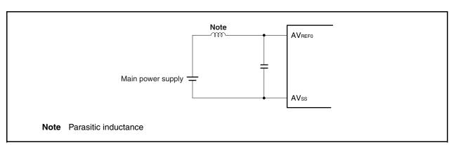
Figure 13-15. AVREFO Pin Processing Example
