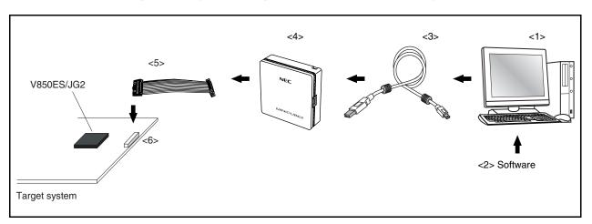
Figure A-4. System Configuration of On-Chip Emulation System
