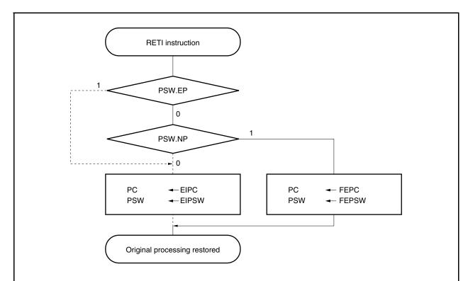
Caution When the EP and NP bits are changed by the LDSR instruction during non-maskable interrupt servicing, in order to restore the PC and PSW correctly during recovery by the RETI instruction, it is necessary to set the EP bit back to 0 and the NP bit back to 1 using the LDSR instruction immediately before the RETI instruction.
