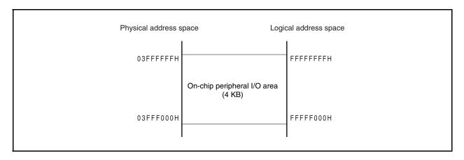
Peripheral I/O registers that have functions to specify the operation mode for and monitor the status of the on-chip peripheral I/O are mapped to the on-chip peripheral I/O area. Program cannot be fetched from this area.
