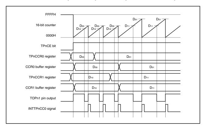
To transfer data from the TPnCCRm register to the CCRm buffer register, the TPnCCR1 register must be written.
