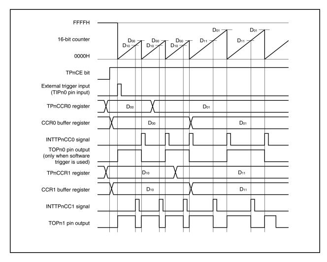
In order to transfer data from the TPnCCRm register to the CCRm buffer register, the TPnCCR1 register must be written.
