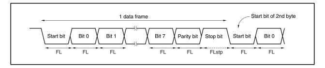
Assuming 1 bit data length: FL; stop bit length: FLstp; and base clock frequency: fuclk, we obtain the following equation.
