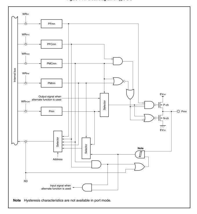
Figure 4-11. Block Diagram of Type G-2
