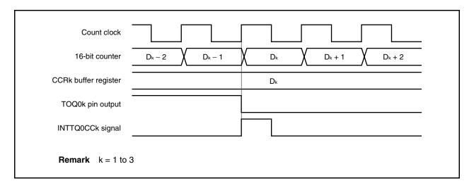
Usually, the INTTQ0CCk signal is generated in synchronization with the next counting up after the count value of the 16-bit counter matches the value of the TQ0CCRk register.
