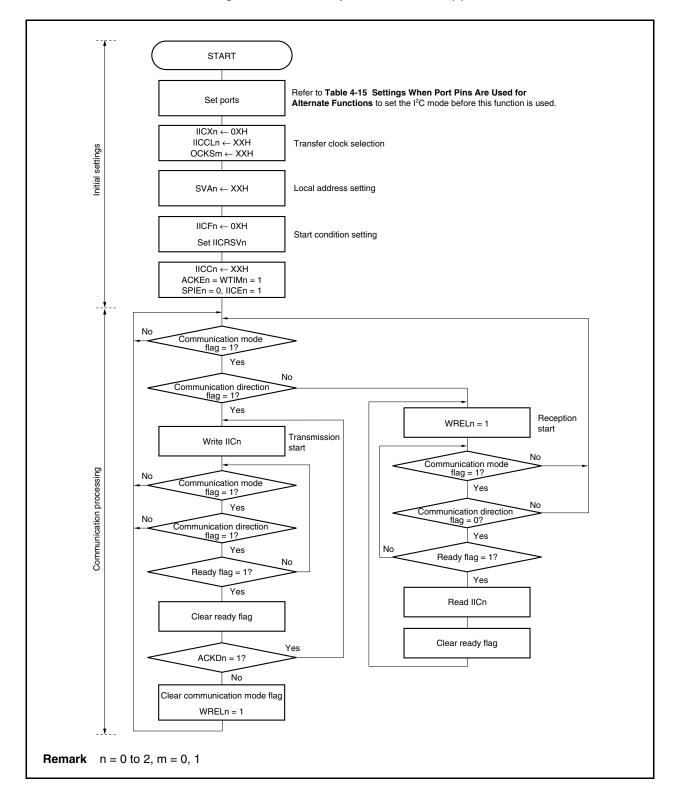
Figure 17-21. Slave Operation Flowchart (1)
