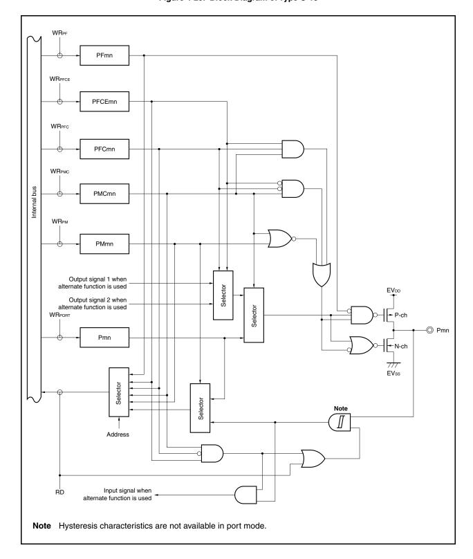
Figure 4-29. Block Diagram of Type U-13
