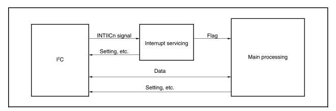
Figure 17-20. Software Outline During Slave Operation
