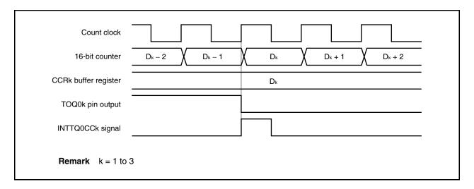
Usually, the INTTQ0CCk signal is generated in synchronization with the next count up after the count value of the 16-bit counter matches the value of the CCRk buffer register.
