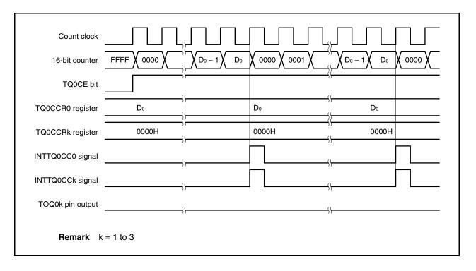
To output a 100% waveform, set a value of (set value of TQ0CCR0 register + 1) to the TQ0CCRk register. If the set value of the TQ0CCR0 register is FFFFH, 100% output cannot be produced.
