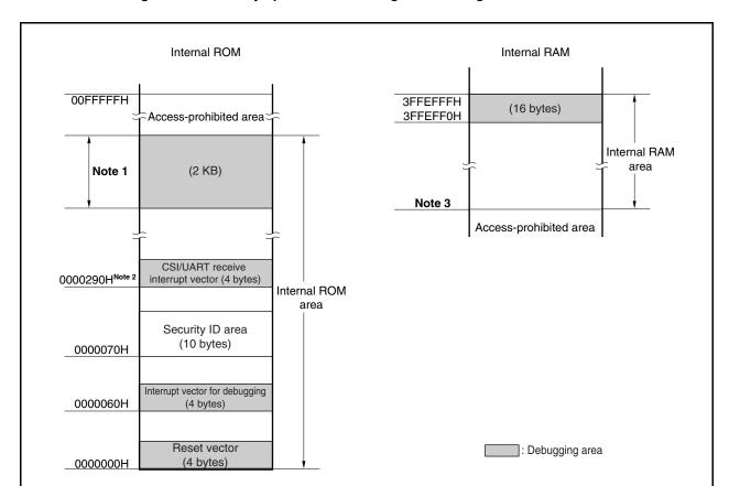
Figure 27-4. Memory Spaces Where Debug Monitor Programs Are Allocated
