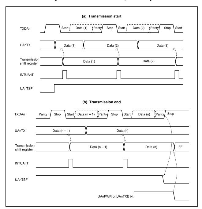
Figure 15-12. Continuous Transmission Operation Timing
