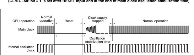
Figure 23-3. Clock Monitor Status After  $\overline{\text{RESET}}$  Input (CLM.CLME bit = 1 is set after  $\overline{\text{RESET}}$  input and at the end of main clock oscillation stabilization time)
