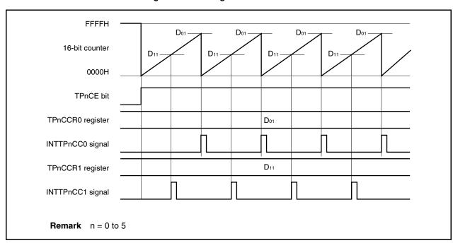
If the set value of the TPnCCR1 register is greater than the set value of the TPnCCR0 register, the INTTPnCC1 signal is not generated because the count value of the 16-bit counter and the value of the TPnCCR1 register do not match.
