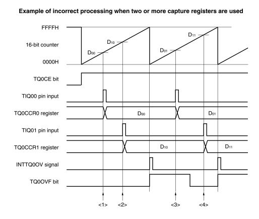
The following problem may occur when two pulse widths are measured in the free-running timer mode.
