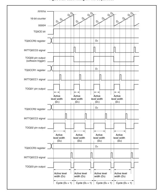
Figure 8-25. Basic Timing in PWM Output Mode
