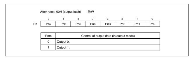
Data is written to or read from the Pn register as follows, regardless of the setting of the PMCn register.
