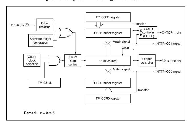
Figure 7-16. Configuration in External Trigger Pulse Output Mode
