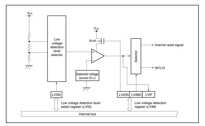
Figure 24-1. Block Diagram of Low-Voltage Detector
