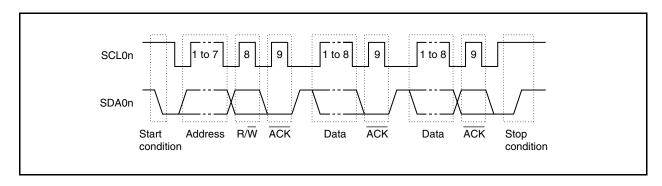
Figure 17-7. I<sup>2</sup>C Bus Serial Data Transfer Timing
