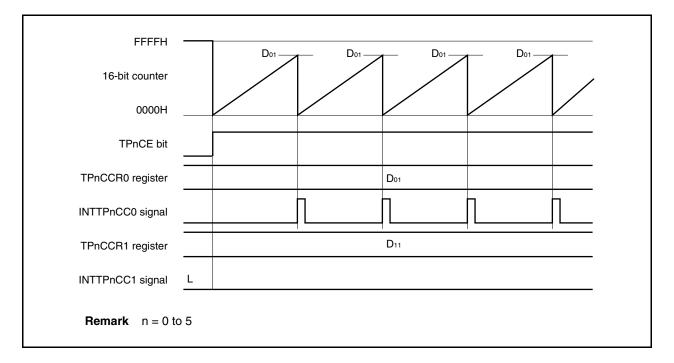
Figure 7-15. Timing Chart When D<sub>01</sub> < D<sub>11</sub>
