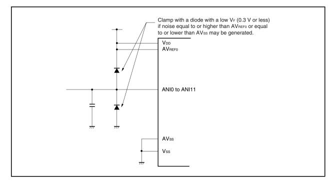
Figure 13-12. Processing of Analog Input Pin
