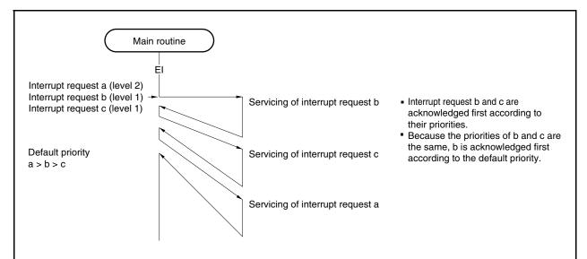
Caution To perform multiple interrupt servicing, the values of the EIPC and EIPSW registers must be saved before executing the EI instruction. When returning from multiple interrupt servicing, restore the values of EIPC and EIPSW after executing the DI instruction.
