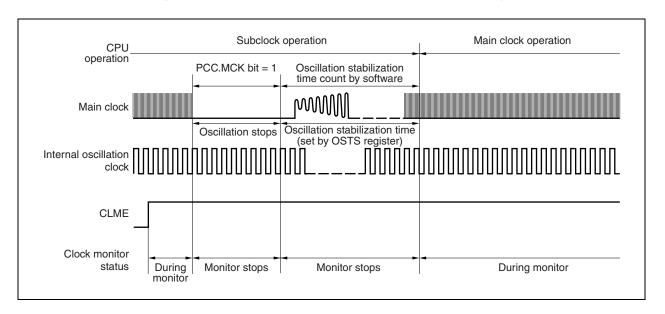
Figure 23-5. Operation When Main Clock Is Stopped (Arbitrary)
