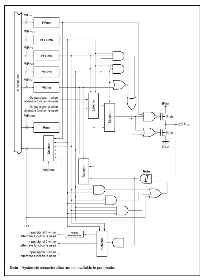
Figure 4-27. Block Diagram of Type U-11
