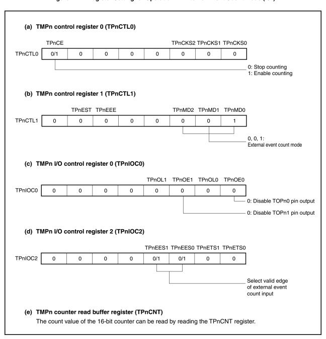
Figure 7-11. Register Setting for Operation in External Event Count Mode (2/2)
