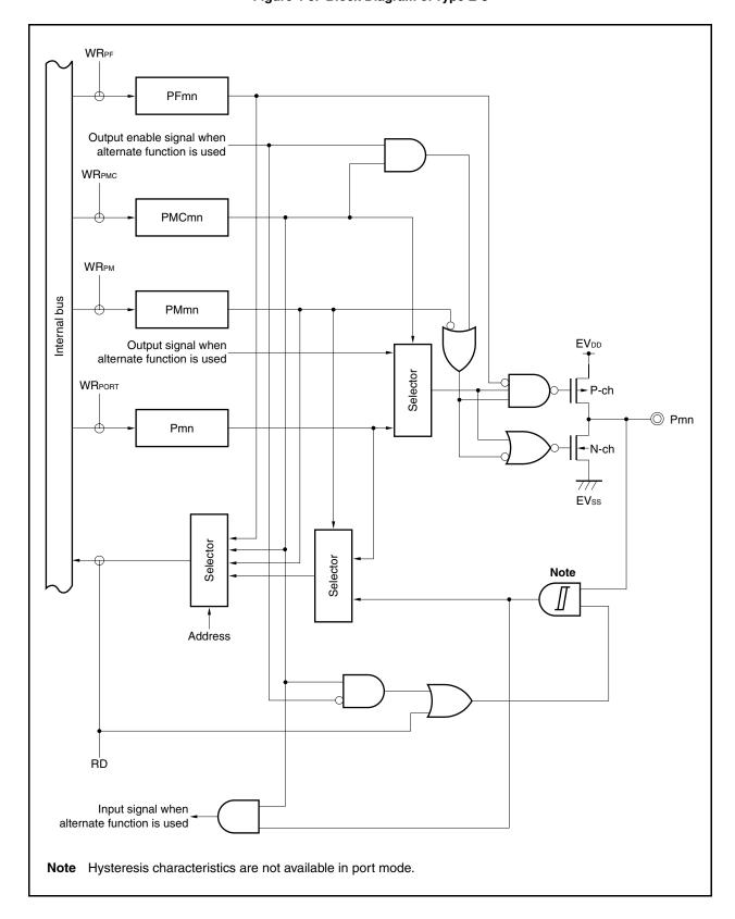
Figure 4-9. Block Diagram of Type E-3
