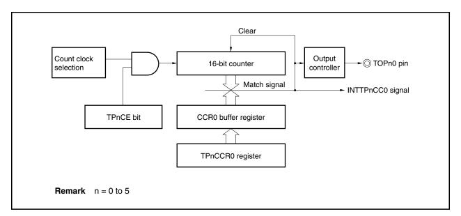
Figure 7-2. Configuration of Interval Timer
