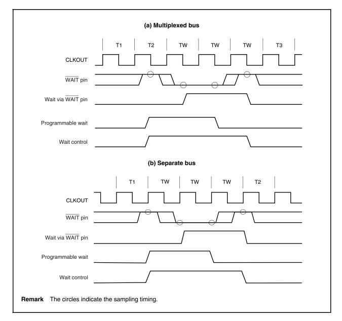
Figure 5-3. Inserting Wait Example
