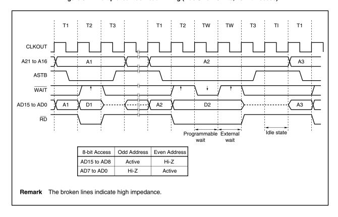
Figure 5-5. Multiplexed Bus Read Timing (Bus Size: 8 Bits)
