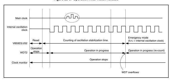
Figure 22-6. Operation After Reset Release
