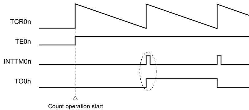
When MD0n0 is set to 1, a timer interrupt (INTTM0n) is output at count operation start, and TO0n performs a toggle operation.
