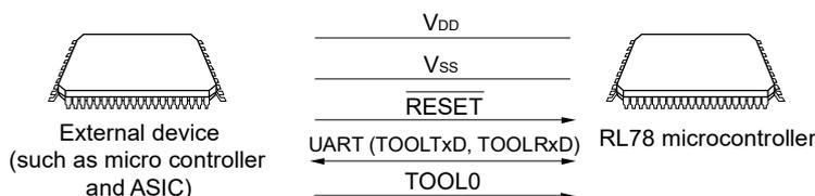
Processing to write data to or delete data from the RL78 microcontroller by using an external device is performed on-board. Off-board writing is not possible.
