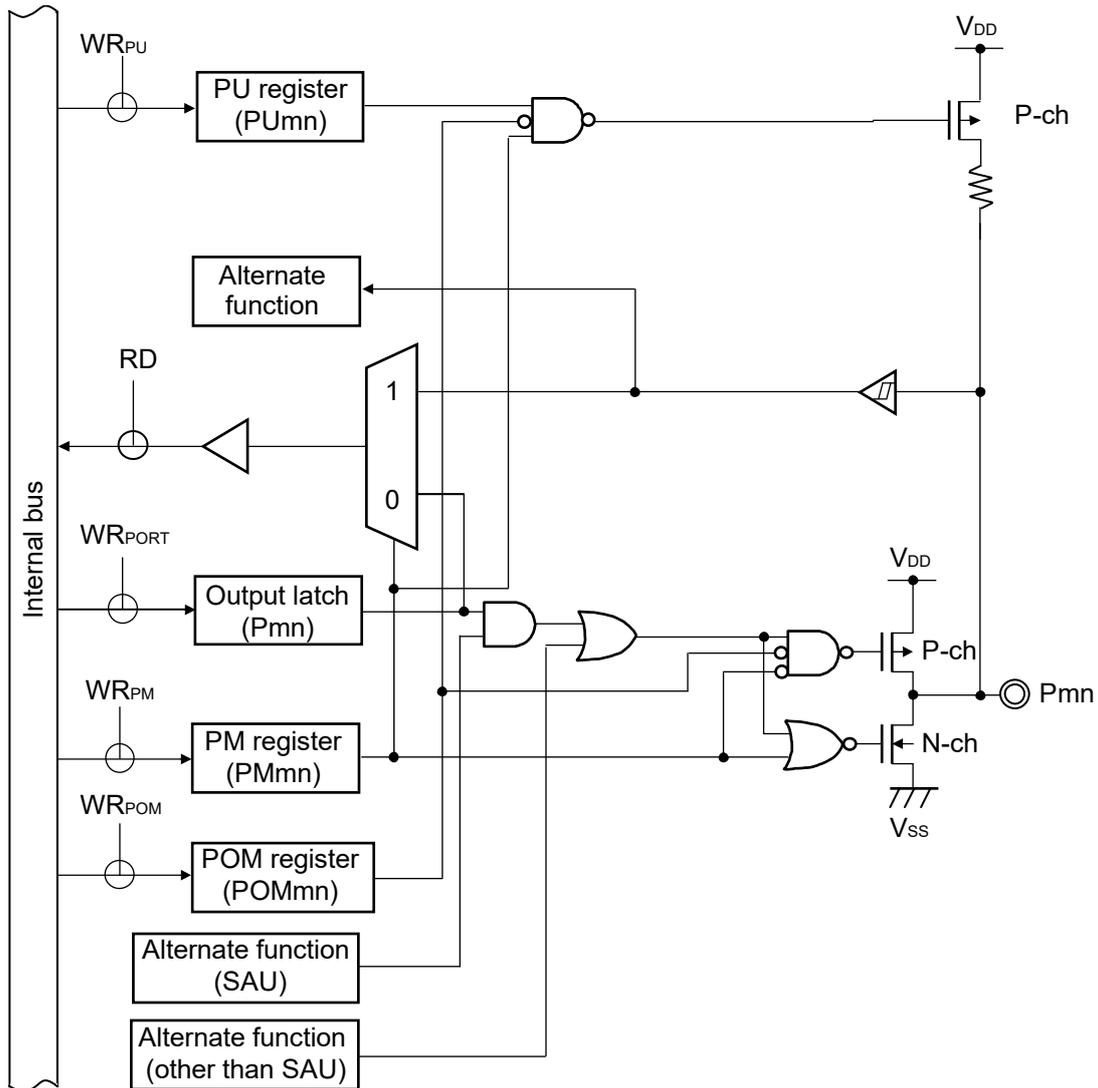
**Caution** The input buffer is enabled even if the type 7-1-2 pin is operating as an output when the N-ch open drain output mode is selected by the corresponding bit in the port output mode register (POM<sub>xx</sub>). This may lead to a through current flowing through the type 7-1-2 pin when the voltage level on this pin is intermediate. Changing the output level when the N-ch open drain output mode is selected may cause a glitch (EV<sub>DD</sub> level).
