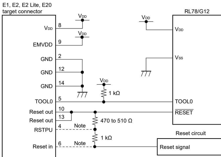
**Note** Connecting the dotted line is not necessary during flash programming.
