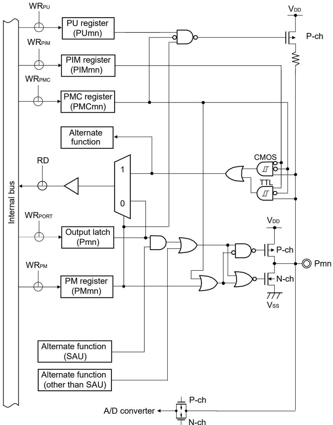
**Caution** When the type 8-3-1 pin is set to TTL input buffer by the corresponding bit in the port input mode register (PIM<sub>xx</sub>) and is driven high, a through current may flow through the type 8-3-1 pin due to the configuration of the TTL input buffer. Drive the type 8-3-1 pin low to prevent the through current.
