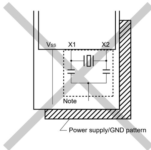
**Note** Do not place a power supply/GND pattern under the wiring section (section indicated by a broken line in the figure) of the X1 and X2 pins and the resonators in a multi-layer board or double-sided board. Do not configure a layout that will cause capacitance elements and affect the oscillation characteristics.
