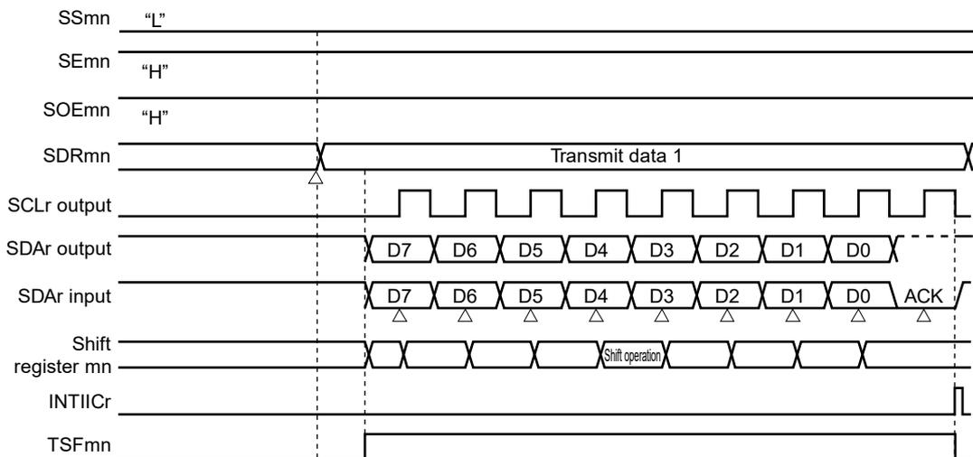
Figure 11-104. Flowchart of Simplified I<sup>2</sup>C Data Transmission
