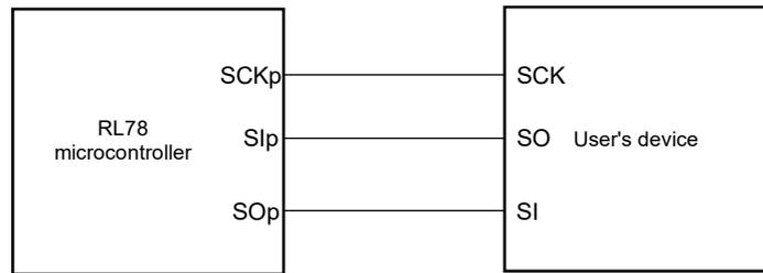
**Simplified SPI (CSI) mode serial transfer timing (during communication at same potential)
