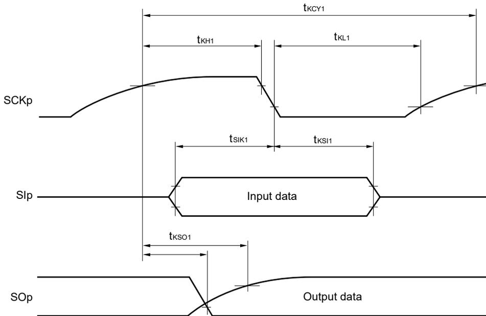
**(9) Communication at different potential (1.8 V, 2.5 V, 3 V) (simplified SPI (CSI) mode) (slave mode, SCKp... external clock input)****(T<sub>A</sub> = -40 to +85°C, 1.8 V ≤ V<sub>DD</sub> ≤ 5.5 V, V<sub>SS</sub> = 0 V)**
