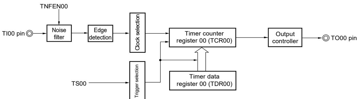
Figure 6-47. Example of Basic Timing of Operation as Frequency Divider (MD000 = 1)
