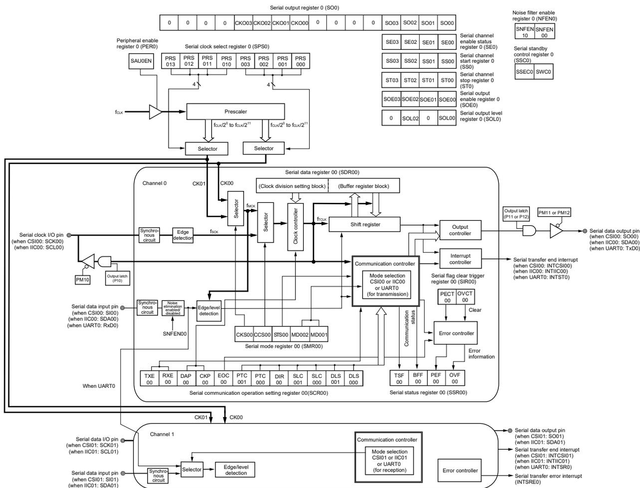
Figure 11-2. Block Diagram of Serial Array Unit 0 (30-pin products)
