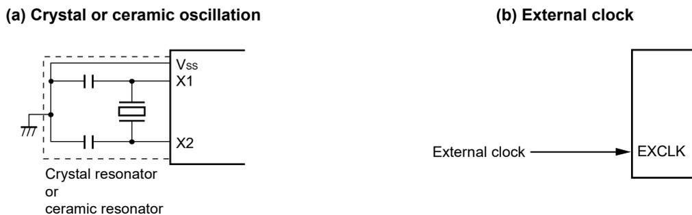
**Caution** When using the X1 oscillator, wire as follows in the area enclosed by the broken lines in the Figure 5-11 to avoid an adverse effect from wiring capacitance.
