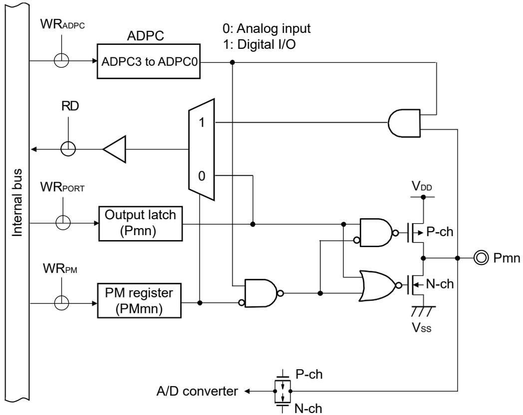
Figure 2-6. Pin Block Diagram for Pin Type 7-1-1
