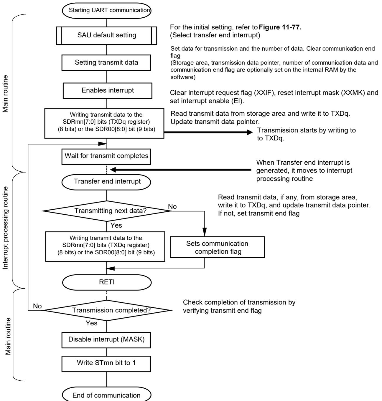
Figure 11-83. Flowchart of UART Transmission (in Continuous Transmission Mode)
