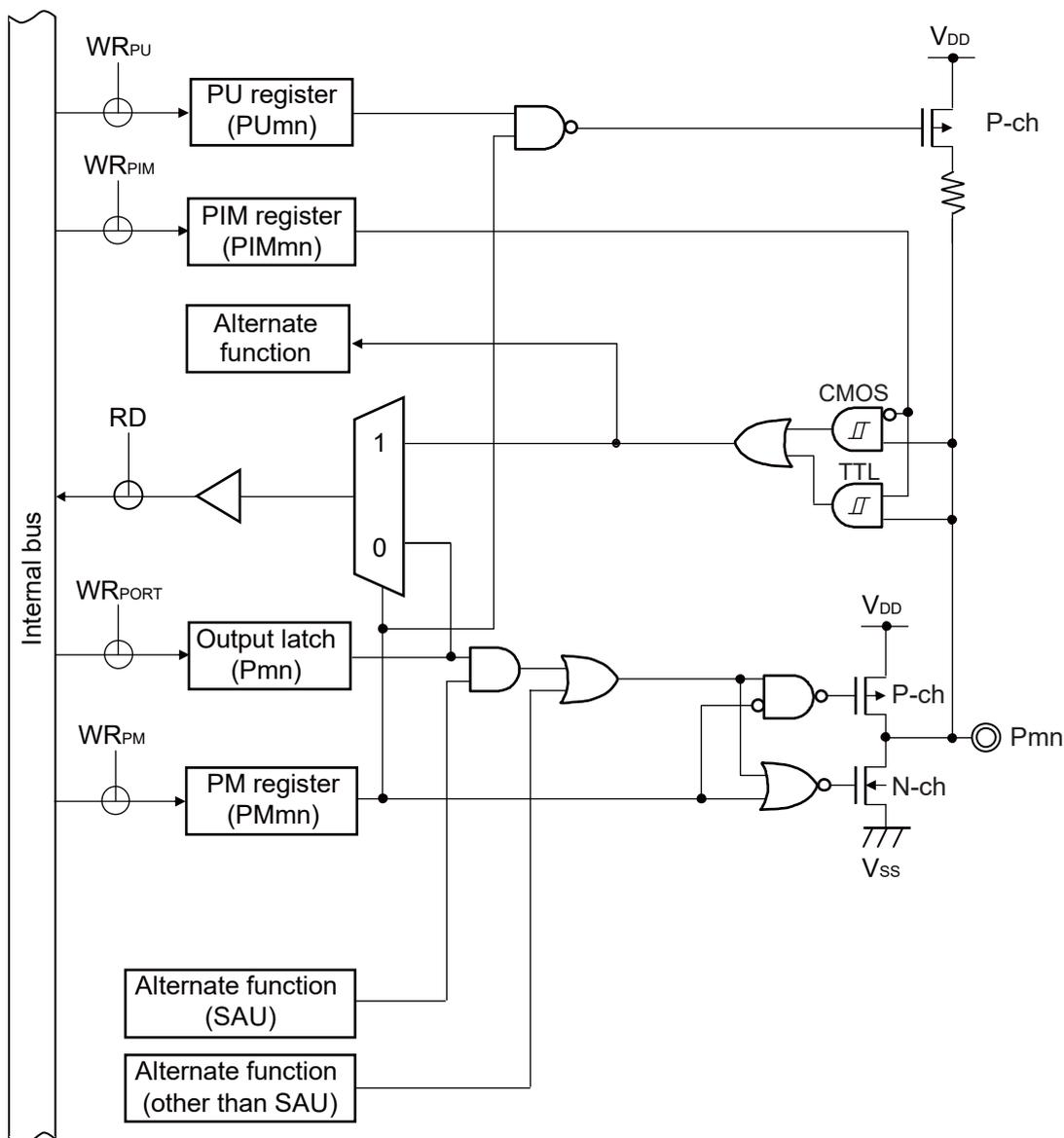
**Caution** When the type 8-1-1 pin is set to TTL input buffer by the corresponding bit in the port input mode register (PIMxx) and is driven high, a through current may flow through the type 8-1-1 pin due to the configuration of the TTL input buffer. Drive the type 8-1-1 pin low to prevent the through current.
