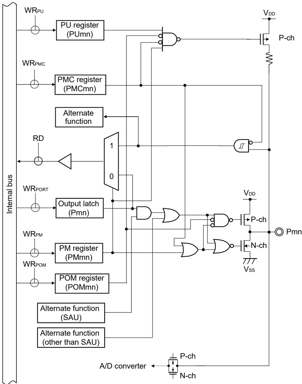
**Caution** The input buffer is enabled even if the type 7-3-2 pin is operating as an output when the N-ch open drain output mode is selected by the corresponding bit in the port output mode register (POMxx). This may lead to a through current flowing through the type 7-3-2 pin when the voltage level on this pin is intermediate. Changing the output level when the N-ch open drain output mode is selected may cause a glitch (EV<sub>DD</sub> level).
