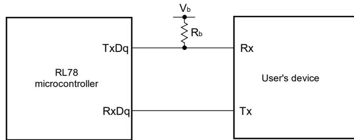
**UART mode bit width (during communication at different potential) (reference)**
