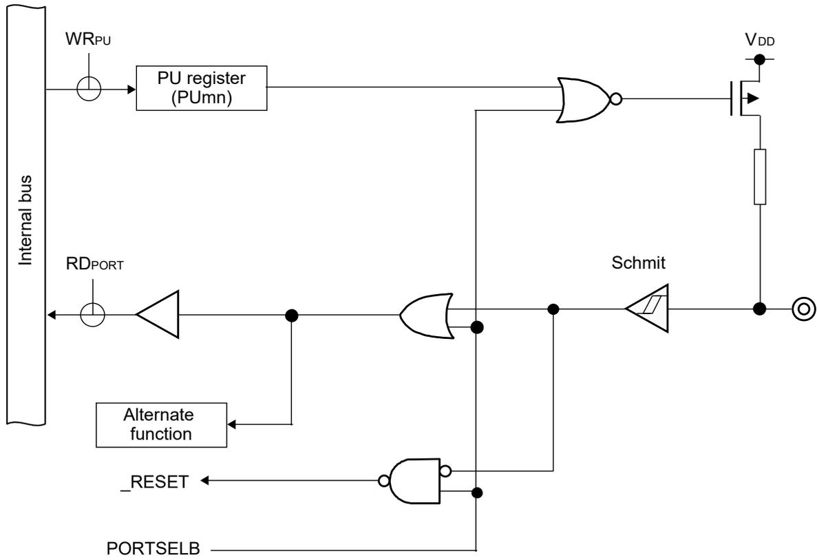
Figure 2-5. Pin Block Diagram for Pin Type 4-3-1
