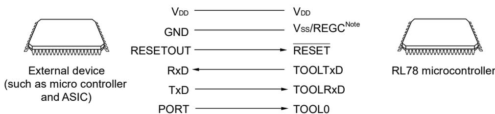
**Note** Connect the REGC pin to ground via a capacitor (0.47 to 1 μF) (30-pin products only).
