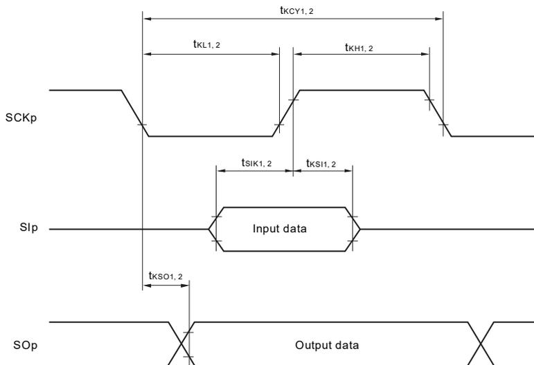
**Simplified SPI (CSI) mode serial transfer timing (during communication at same potential)
