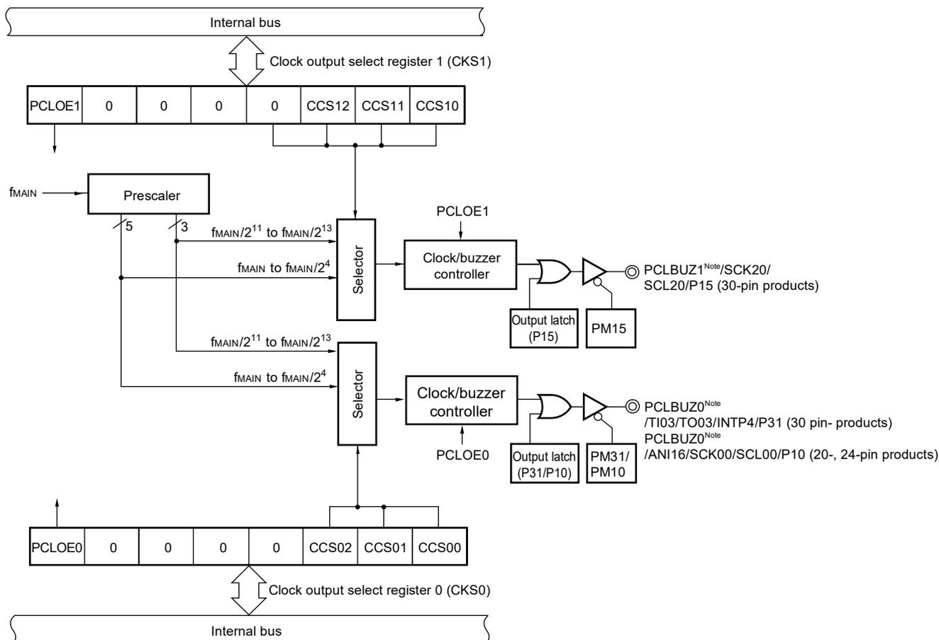
**Note** For output frequencies available from PCLBUZ0 and PCLBUZ1, refer to 28.4 or 29.4 AC Characteristics. PCLBUZ1 output function is available only in 30-pin products.
