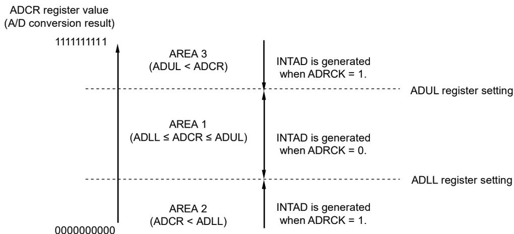
**Remark** If INTAD does not occur, the A/D conversion result is not stored in the ADCR or ADCRH register.
