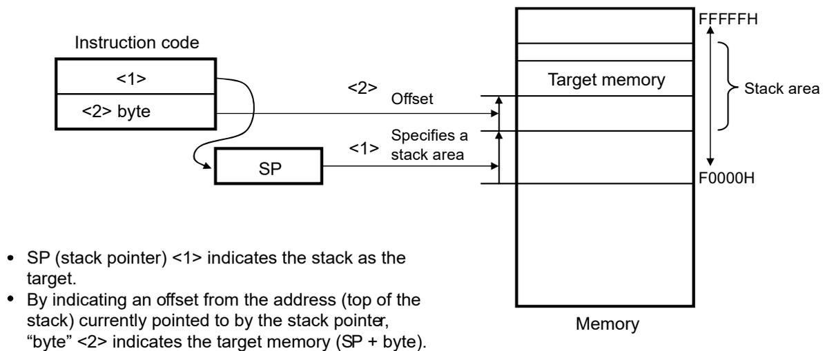
Figure 3-29. Example of [HL + byte], [DE + byte]
