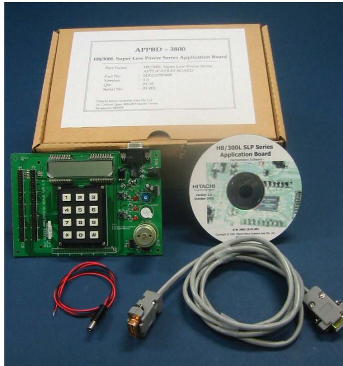
Figure 1.2 LCD Application Board [APPBD - LCD] Package
