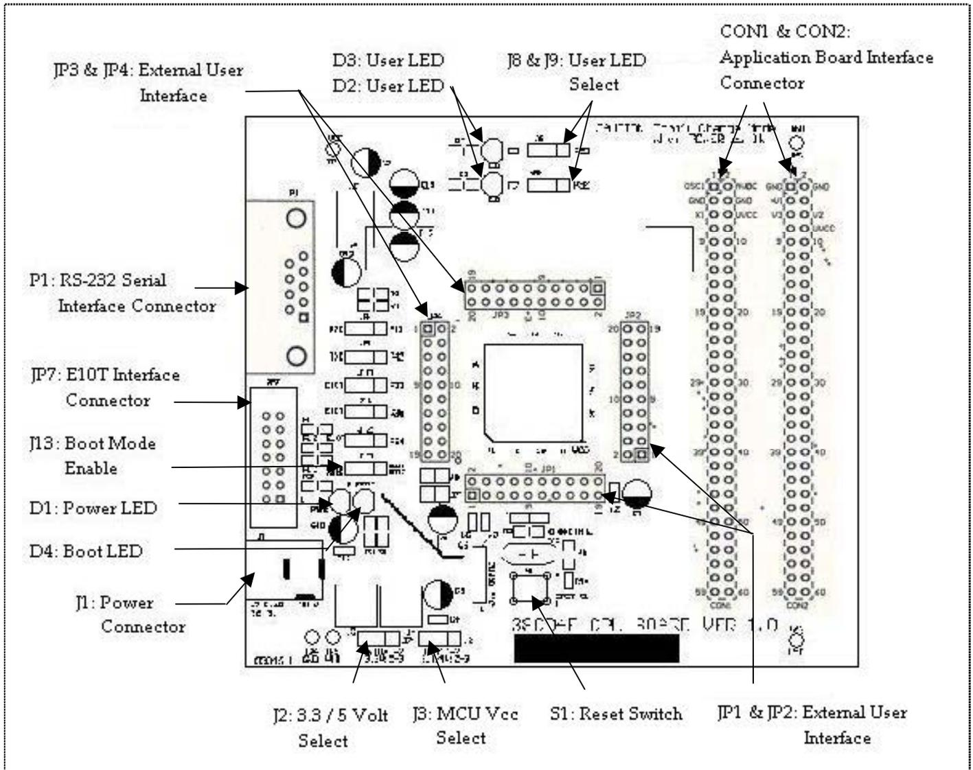
Figure 2.1 Names of Parts on CPU Board
