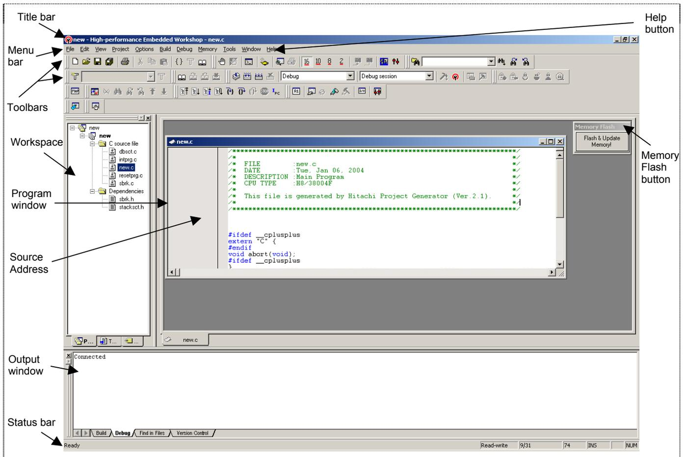
**Figure 4.1 High-Performance Embedded Workshop Window**
