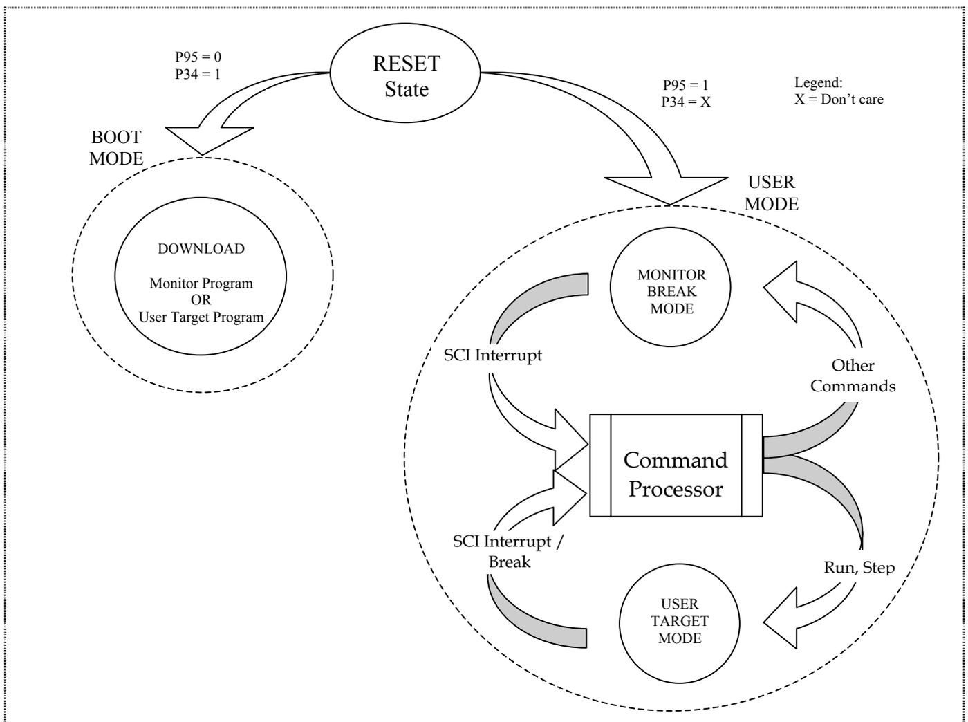
**Figure 7.1 Mode Transition Diagram**
