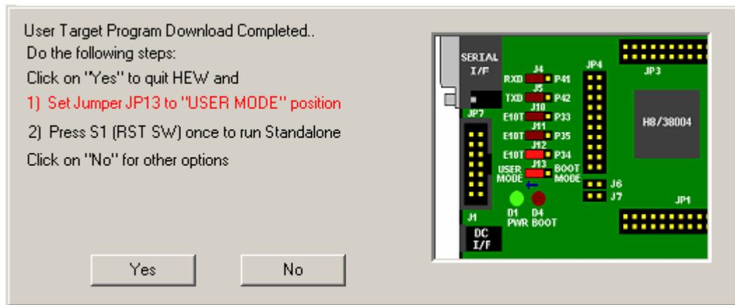
Figure 4.8 Dialogue box for running user target program
