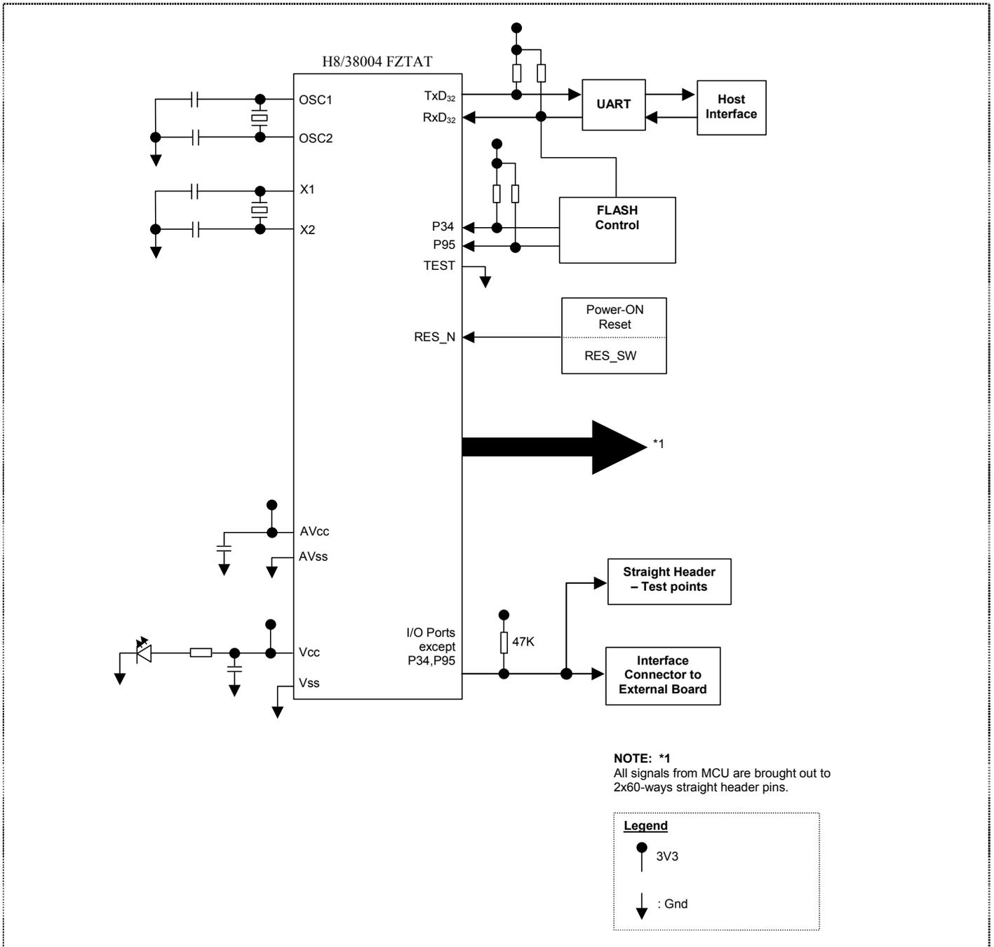
Figure 1.2 CPU Board Functional Blocks
