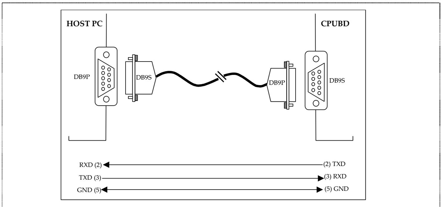
**Figure 2.2 Serial Communication connections**
