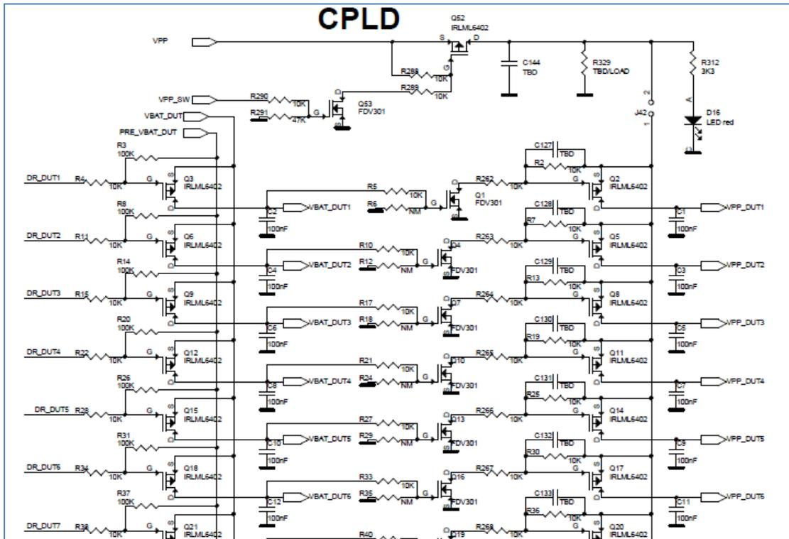
Figure 119: VBAT and VPP Control from CPLD
