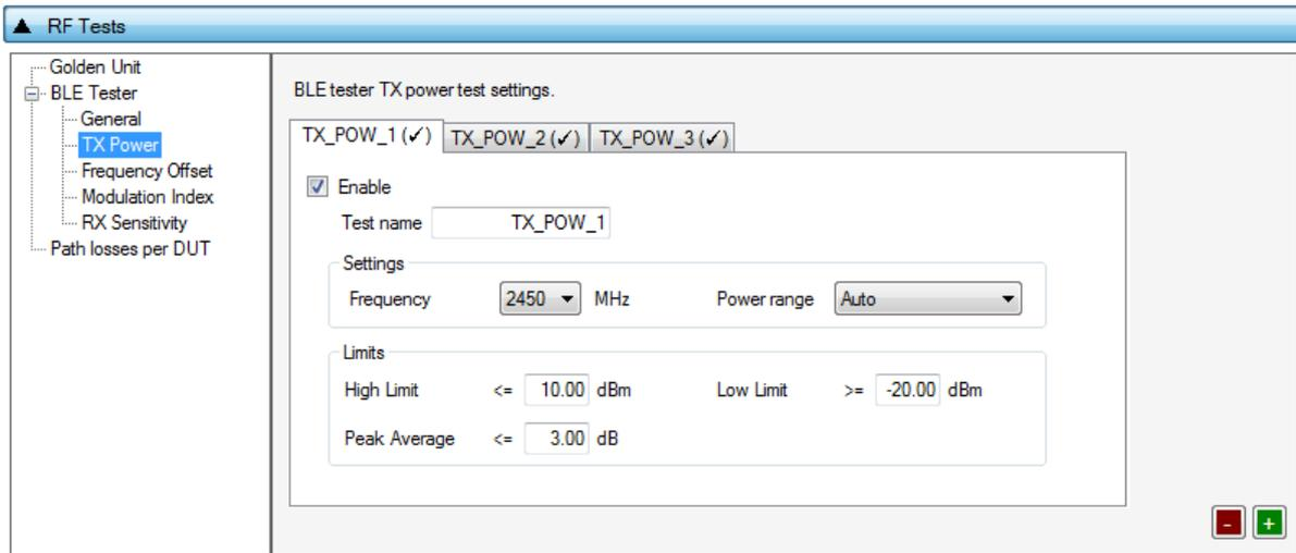
Figure 76: BLE Tester TX Power - DA1468x
