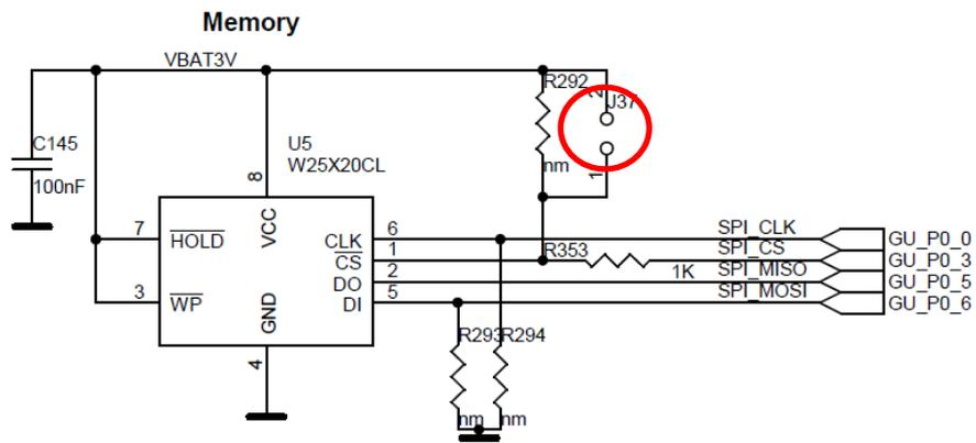
Figure 17: J37 - GU Programming Jumper Schematics
