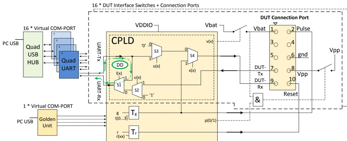
Figure 8: CPLD UART Loopback Data Stream
