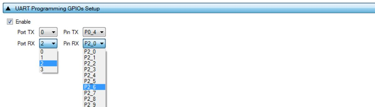
**Figure 47: UART Programming GPIOs Setup - DA1458x**
