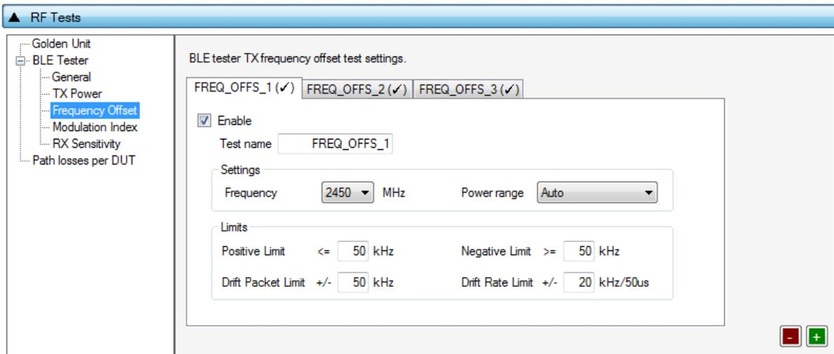
Figure 52: BLE Tester Frequency Offset - DA1458x
