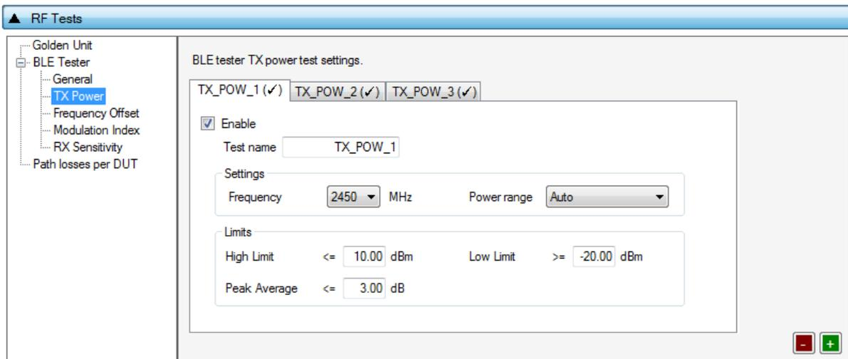
Figure 51: BLE Tester TX Power - DA1458x
