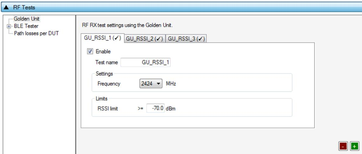
Figure 49: Golden Unit RF Tests - DA1458x
