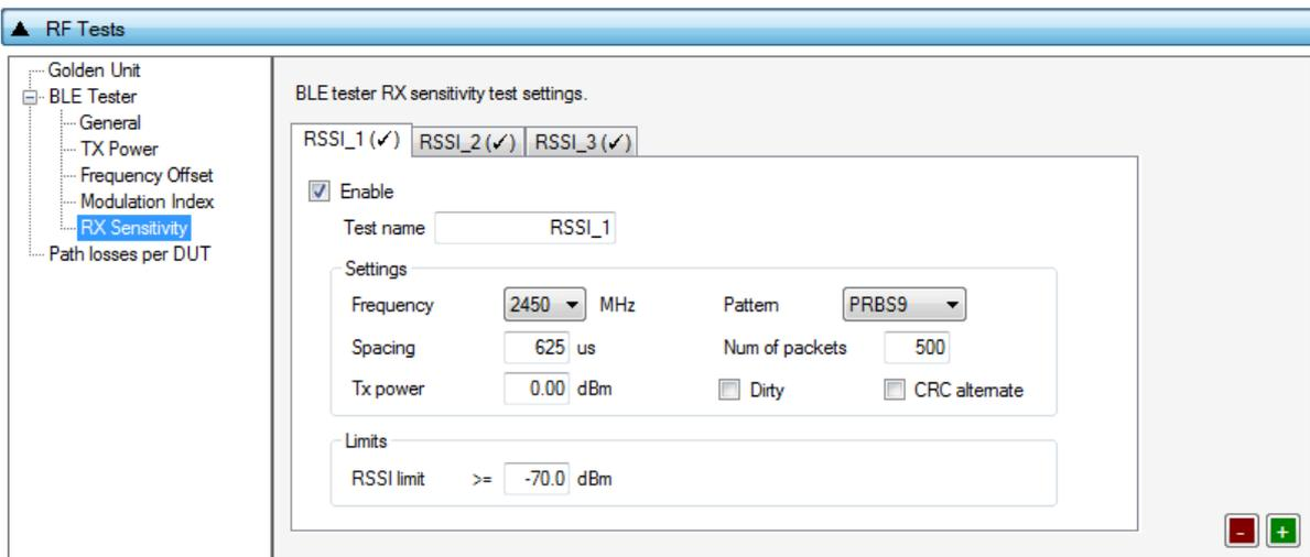
Figure 54: BLE Tester RX Sensitivity - DA1458x
