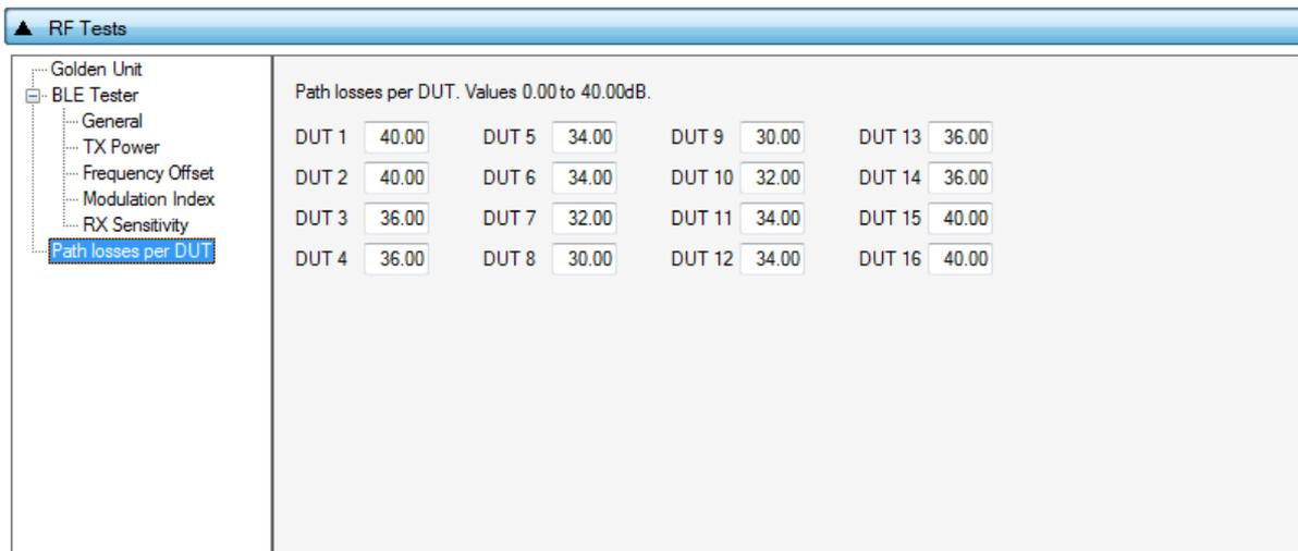
Figure 55: Path Losses per DUT - DA1458x
