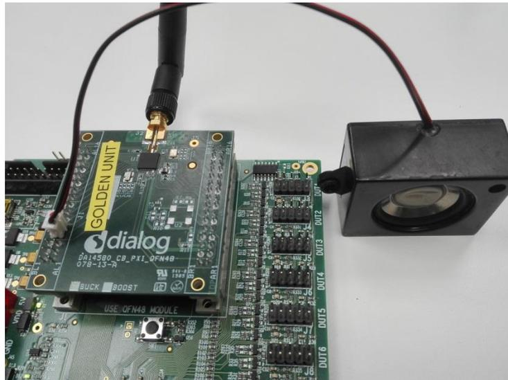
Figure 144: Speaker Connection for Audio Test.
