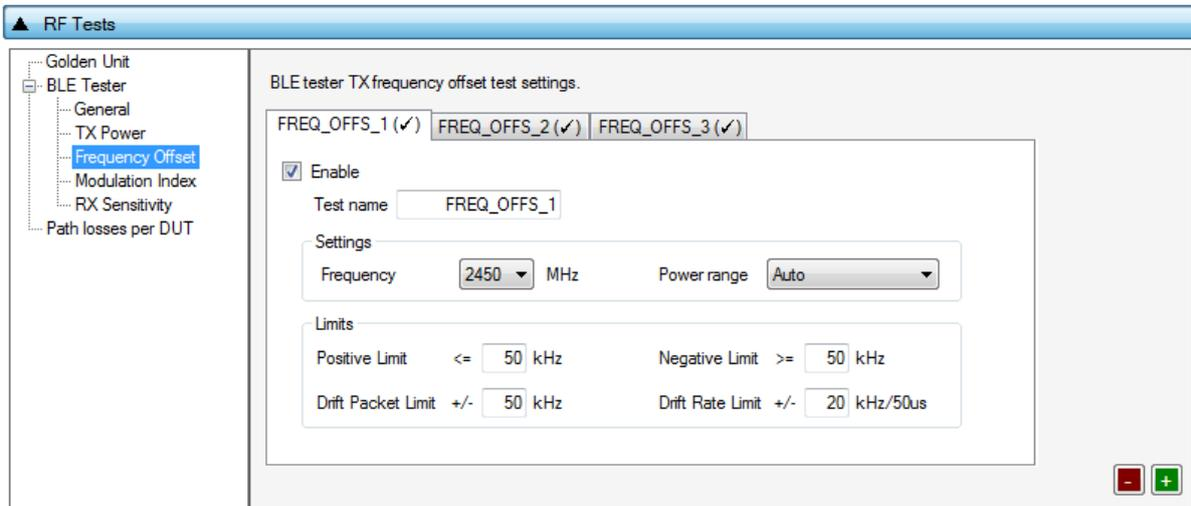
Figure 77: BLE Tester Frequency Offset - DA1468x
