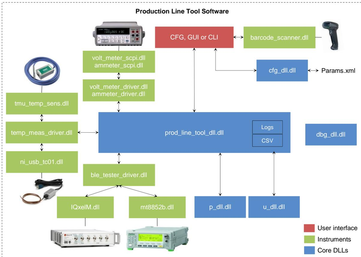
Figure 20: Production Line Tool Software Block Diagram
