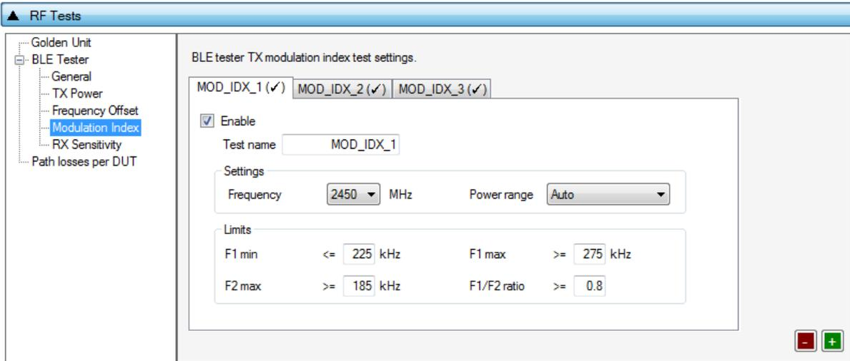
Figure 78: BLE Tester Modulation Index - DA1468x
