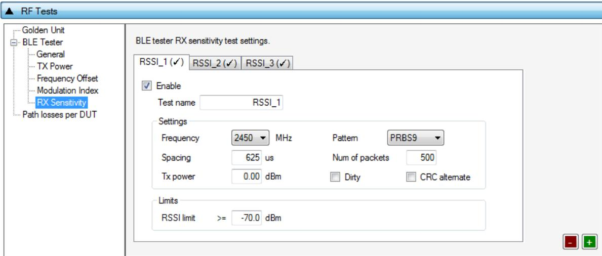
Figure 79: BLE Tester RX Sensitivity - DA1468x
