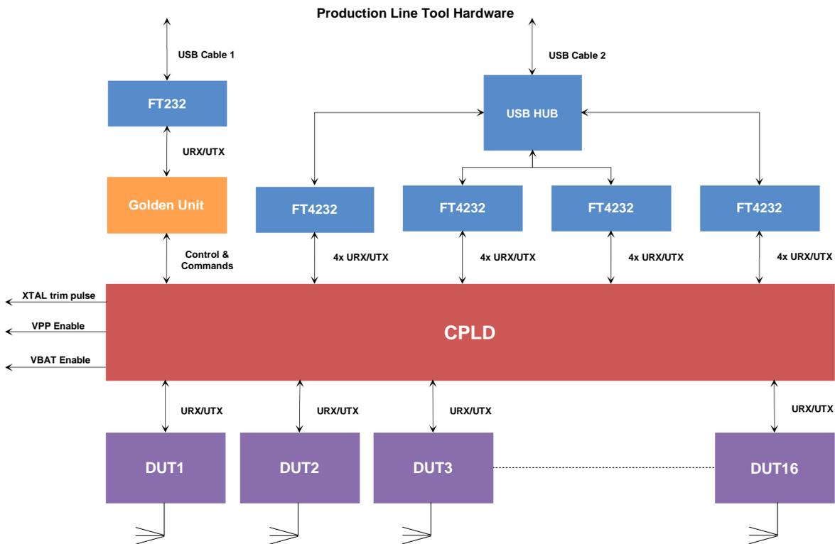
Figure 2: Production Line Tool Hardware Board Block Diagram
