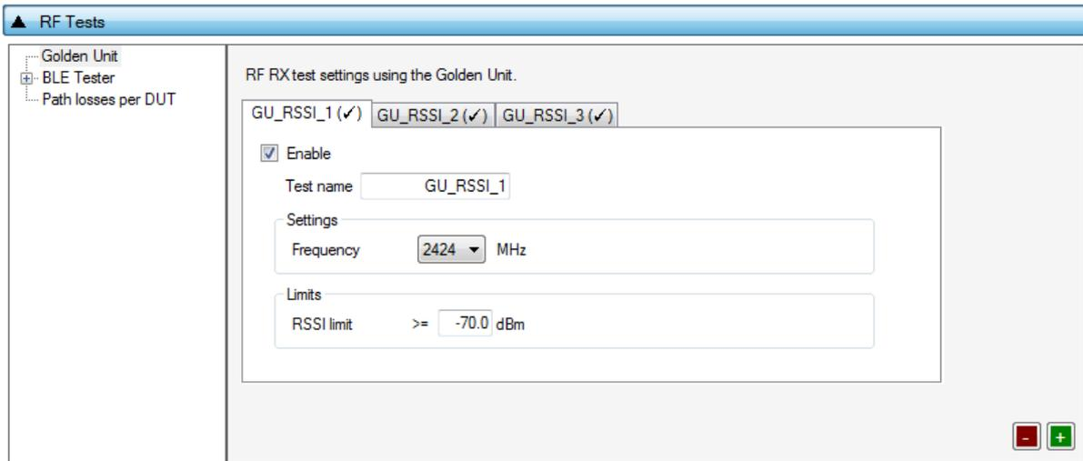
Figure 74: Golden Unit RF Tests - DA1468x
