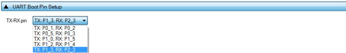
Figure 71: UART Boot Pins Setup - DA1468x
