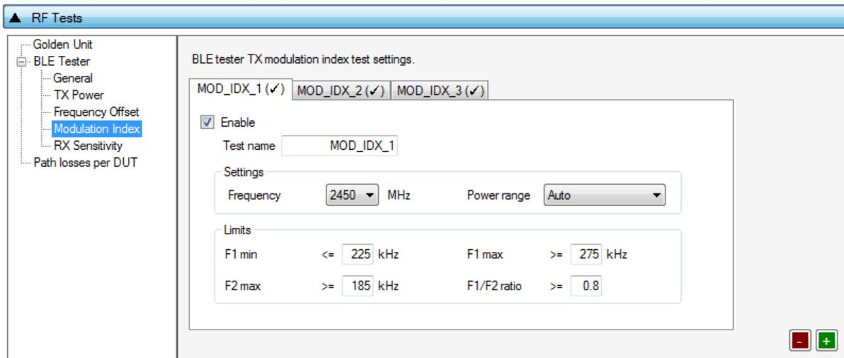
Figure 53: BLE Tester Modulation Index - DA1458x
