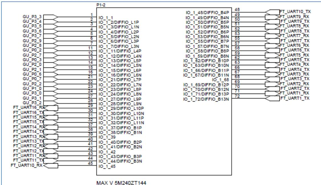
Figure 121: CPLD FTDI and GU Control Connections
