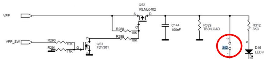
Figure 13: VPP Control Circuit Schematic
