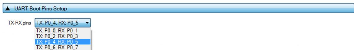
**Figure 45: UART Boot Pins Setup - DA1458x**
