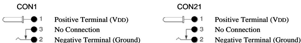
**Note:** Maximum Input 5.0 volts at CON1 and CON2.
