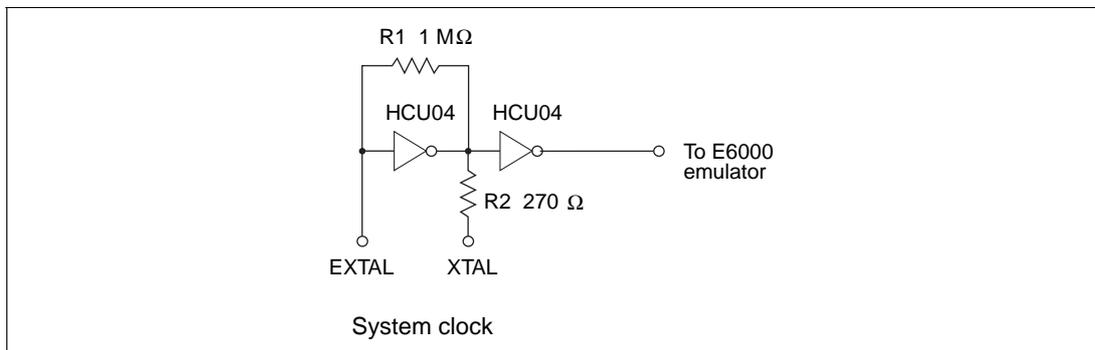
**Figure 9 Oscillator Circuit**
