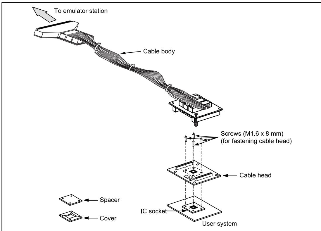
**Figure 1 HS2238RECB62H User System Interface Cable**
