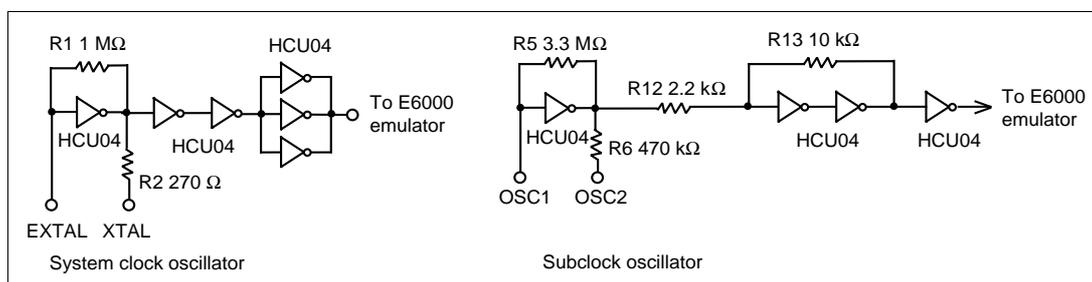
**Figure 11 Oscillator Circuit**
