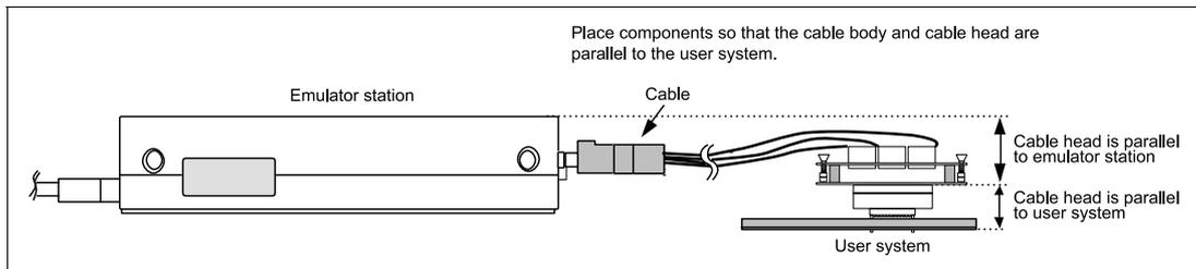
**Figure 12 User System Interface Cable Location Example**
