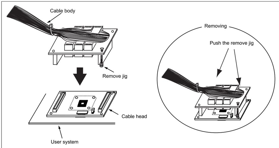
**Figure 6 Fastening Cable Body**
