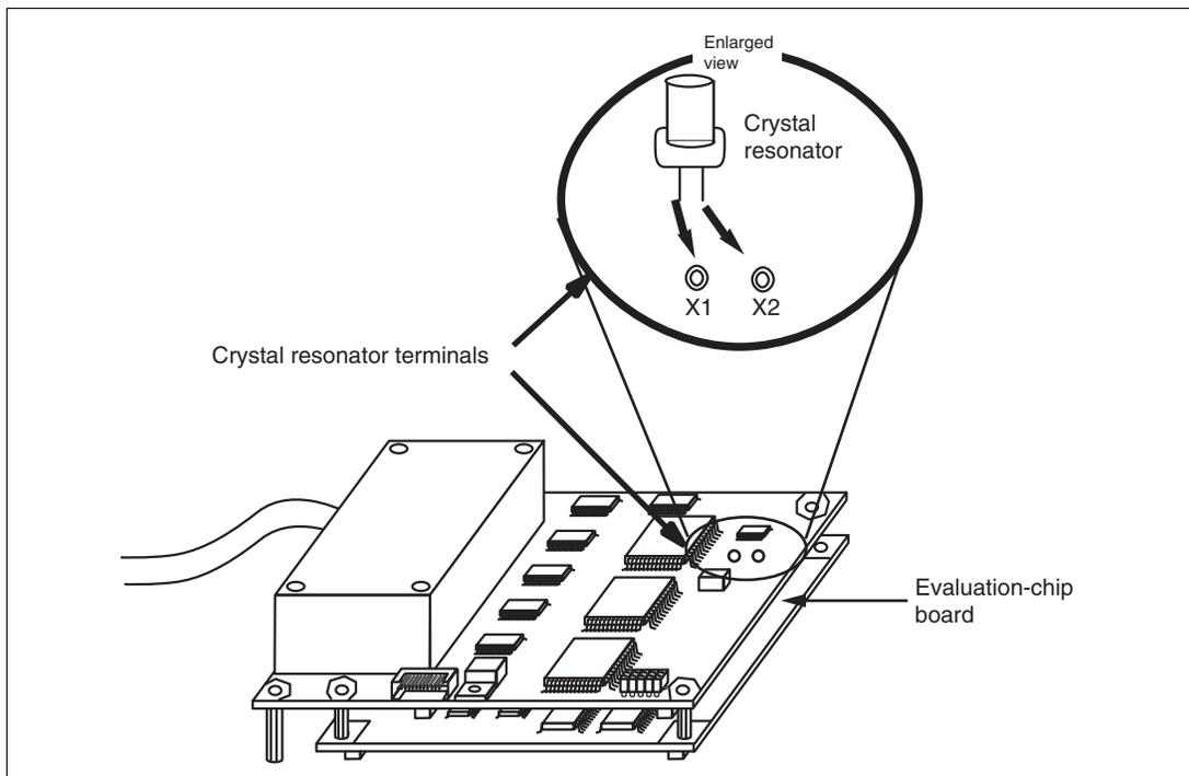
**Figure 19 Mounting the Crystal Resonator**
