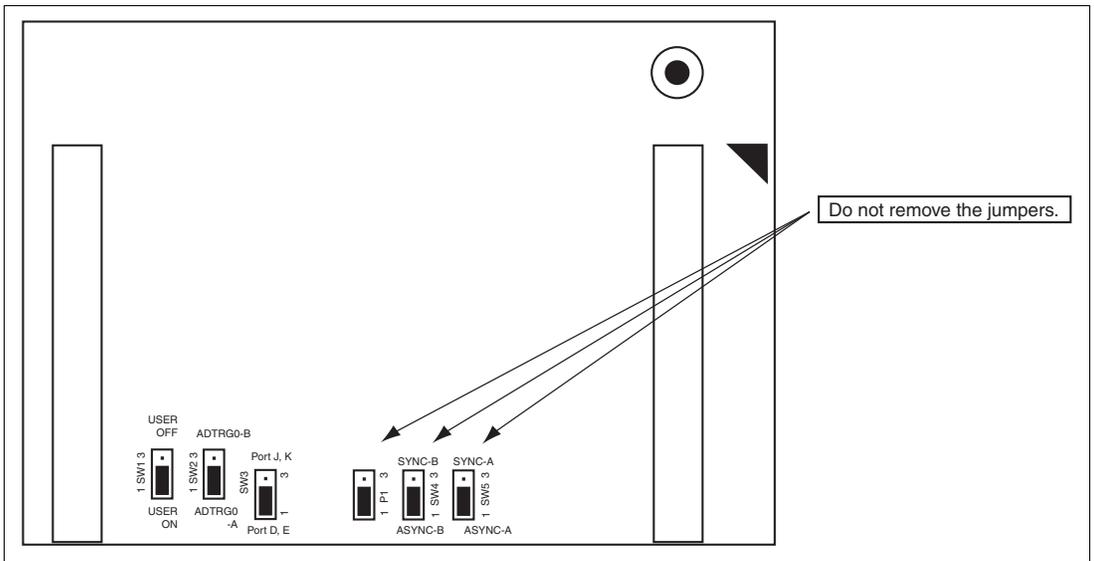
**Figure 20 P1, SW4, and SW5 Jumper Sockets**
