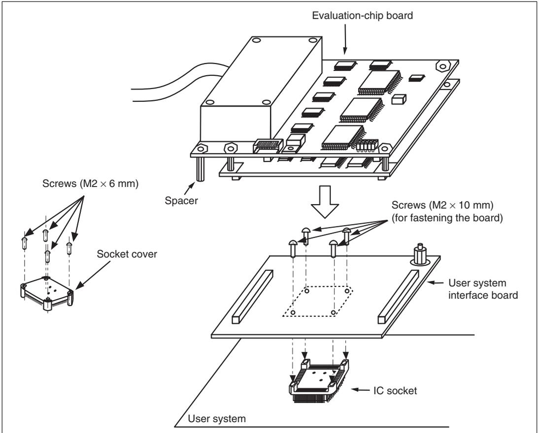
**Figure 1 H8SX/1668R PLQP0144KA-A User System Interface Board**
