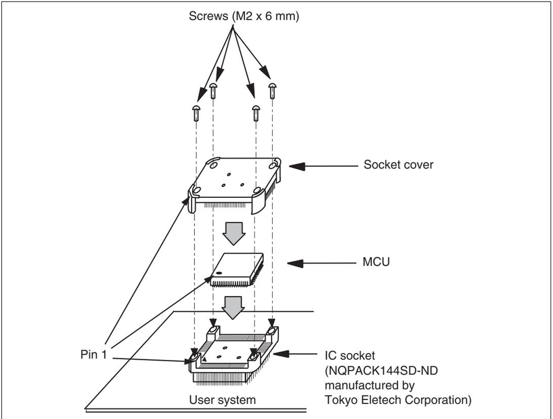
**Figure 11 Installing MCU to User System**
