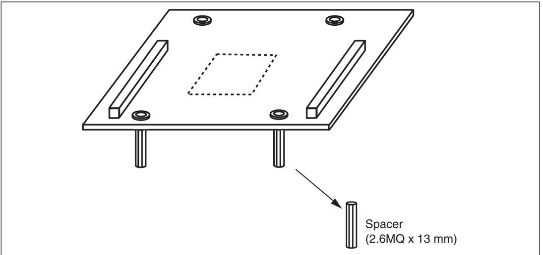
**Figure 10 Attaching Spacers**
