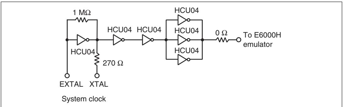
**Figure 18 Clock Oscillator**
