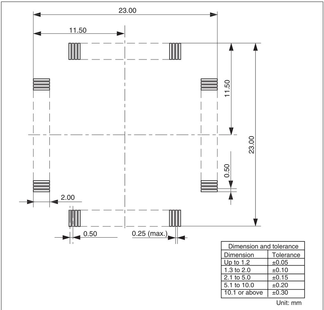
**Figure 6 Recommended Dimensions for the Mounting Pad**
