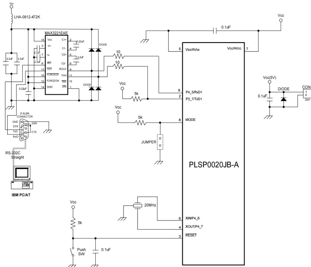
Figure 2 Circuit Using the RS-232C Cable (R8C/28, 29 Groups)
