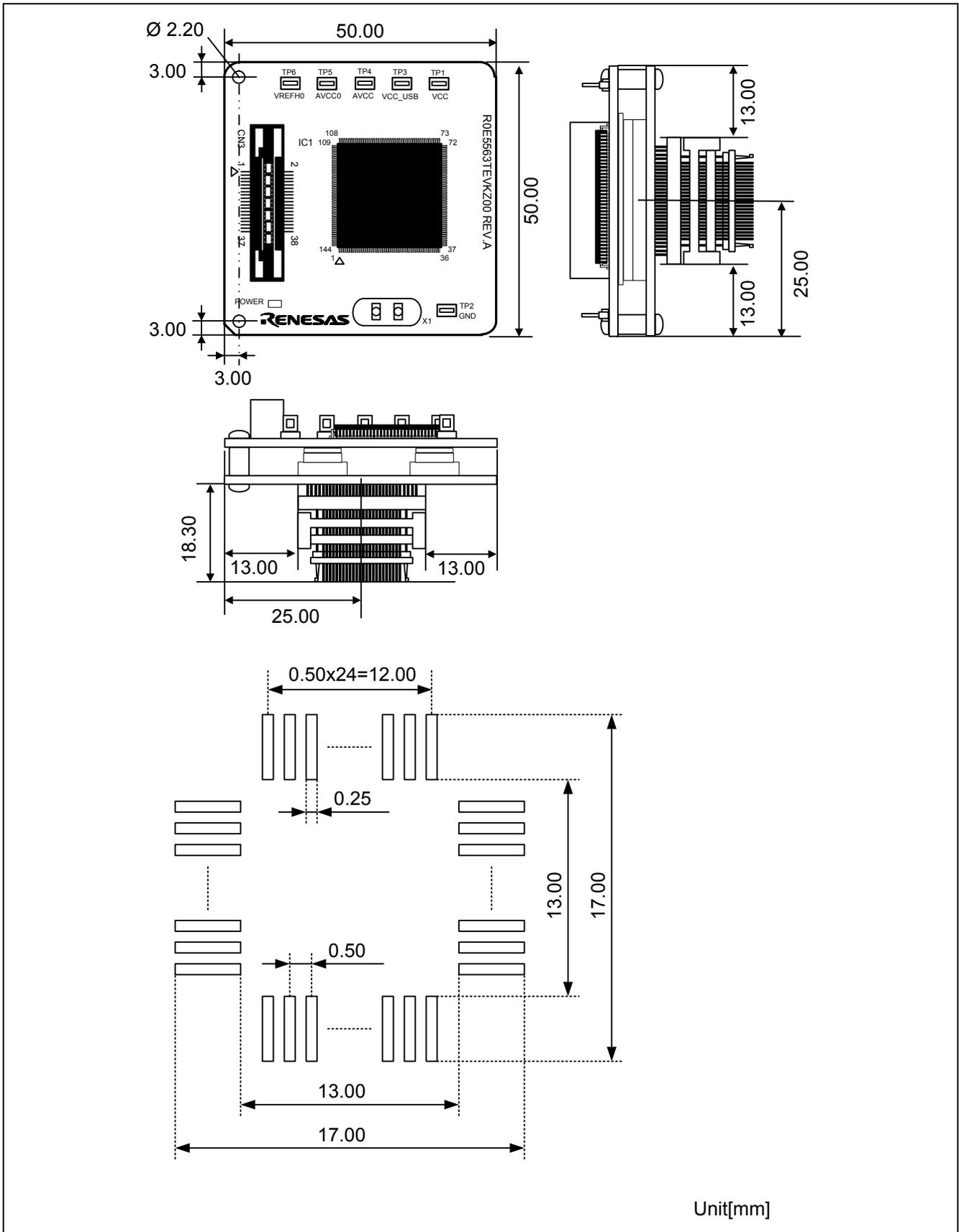
Figure 4 Reference Foot Pattern and Dimensions of This Product (R0E5563TEDMB02)
