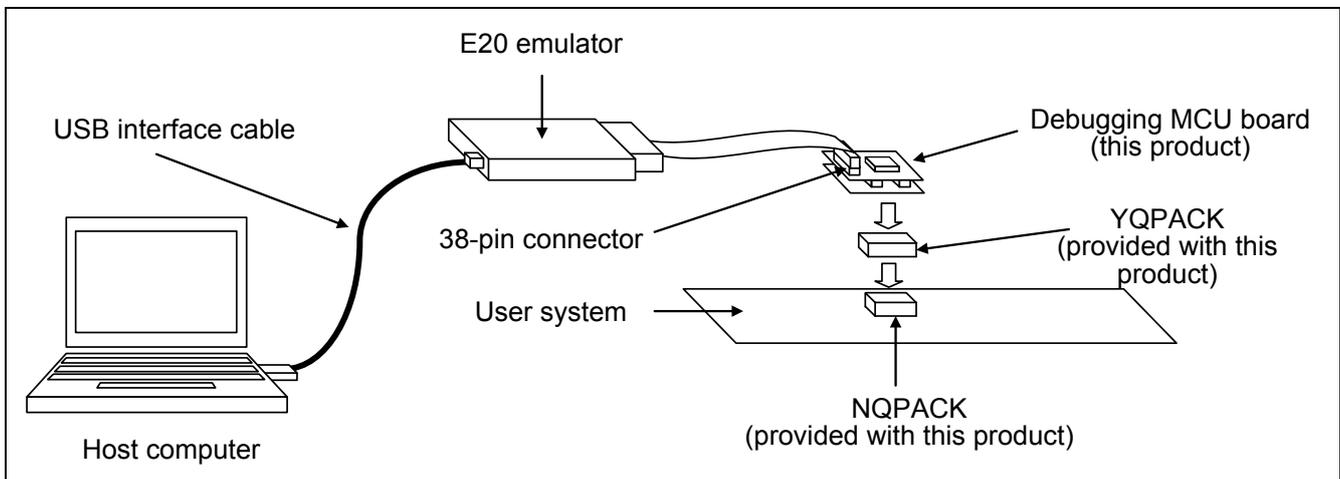
Figure 1 System Configuration
