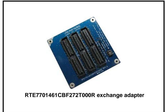
Figure 1 External View of the RTE7701461CBF272T000R
