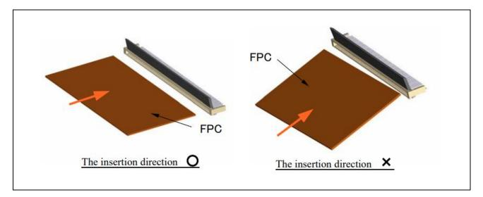
Figure 3.5 Caution When Connecting SMARC JTAG Adaptor to Connector
