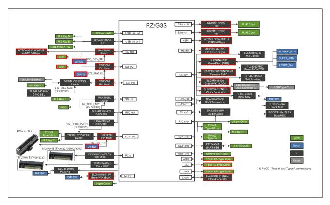
Figure 2.3 G3S SMARC EVK Block Diagram
