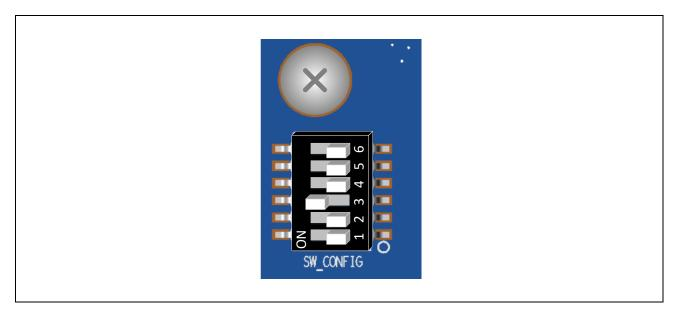
Figure 2.4 The Location and the Default Setting of the SW\_CONFIG
