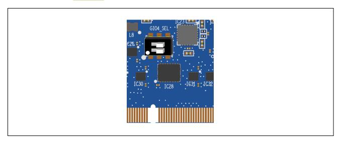
Figure 2.5 The Location and the Default Setting of the GPIO4\_SEL
