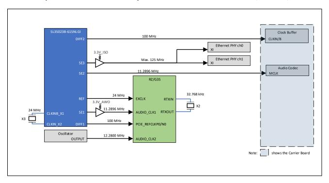
Figure 3.2 Clock Architecture of G3S SMARC EVK
