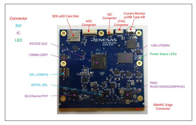
Figure 2.1 RZ/G3S SMARC Module Board Top View
