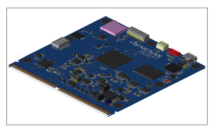
Figure 1.1 RZ/G3S SMARC Module Board
