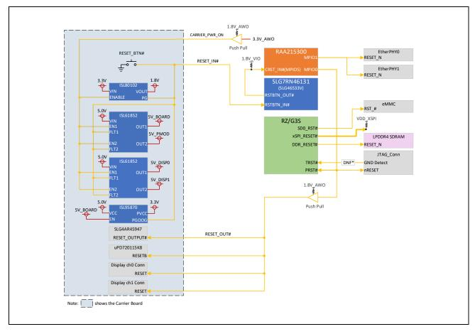
Figure 3.3 Reset Architecture of G3S SMARC EVK
