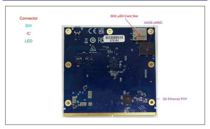
Figure 2.2 RZ/G3S SMARC Module Board Bottom View
