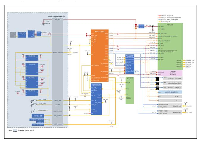
Figure 3.1 Power System Circuitry of G3S SMARC EVK
