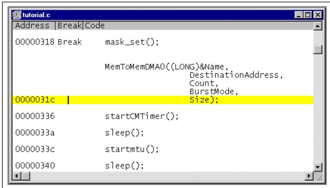
**Figure 4.23 Program Window after Executing the Step Out Command**
