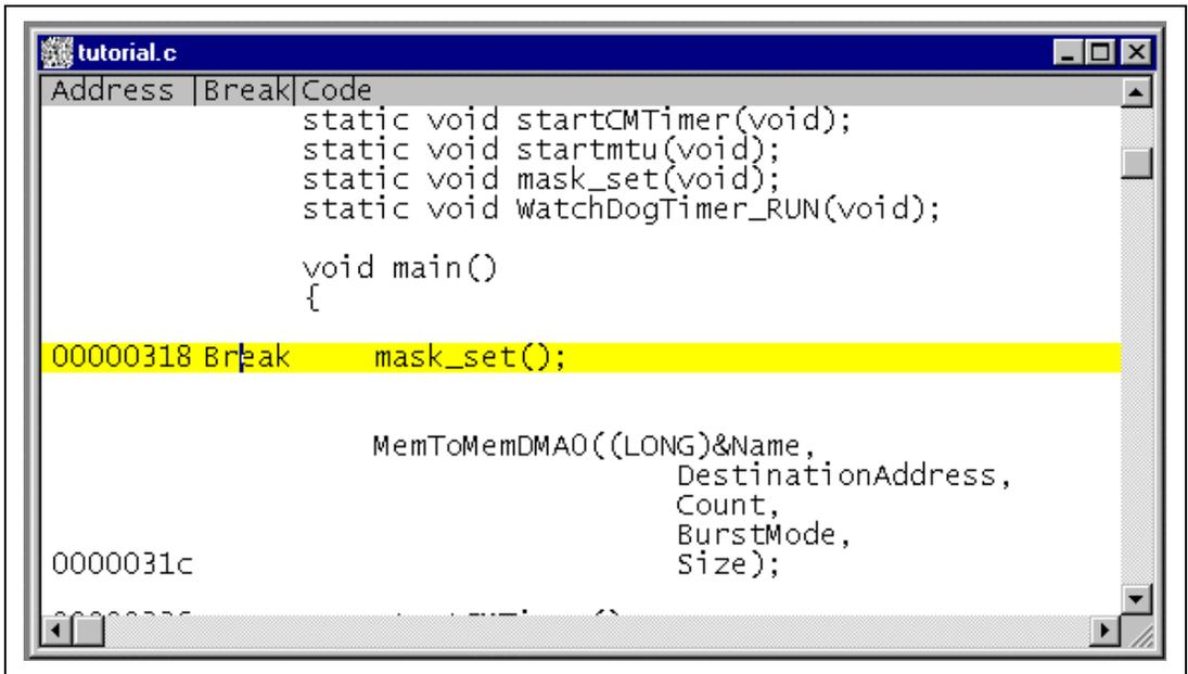
**Figure 4.21 Program Window after Executing the Step In Command (1)**
