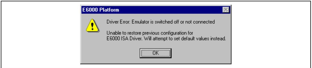
**Figure 2.21 Faulty Connection Message**
