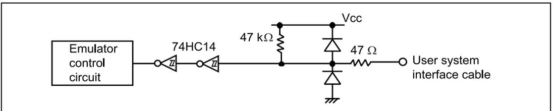
**Figure 3.8 User System Interface Circuit for RESET**
