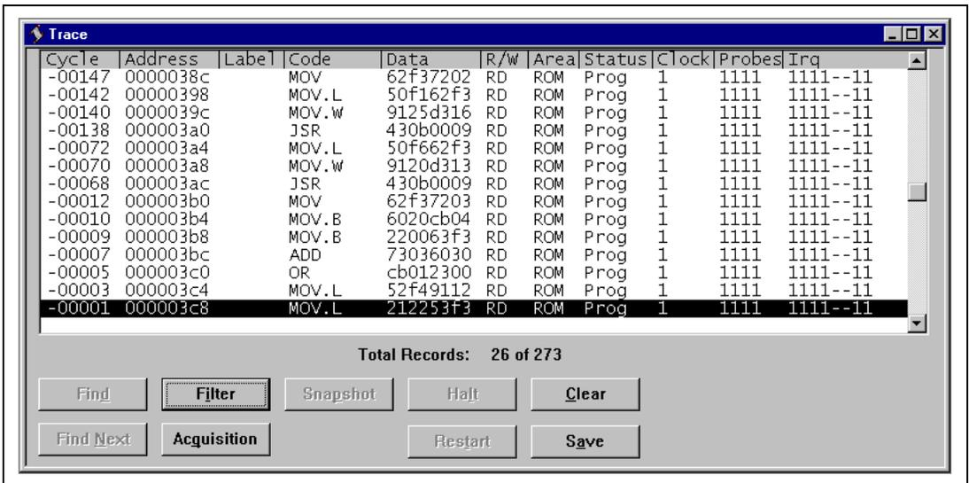
**Figure 4.35 Showing Trace Buffer Contents**
