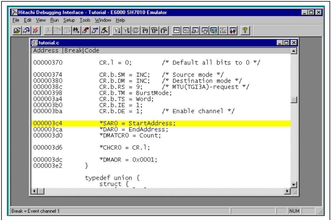
**Figure 4.31 Stopping the Program by a Breakpoint**
