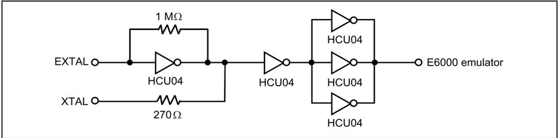
**Figure 3.11 Oscillator Circuit**
