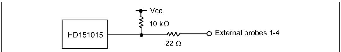
**Figure 3.13 Interface Circuit for External Probes 1-4**
