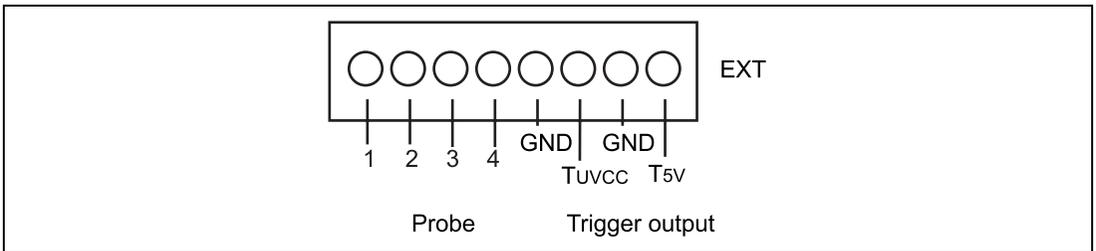
**Figure 3.12 External Probe Connector**
