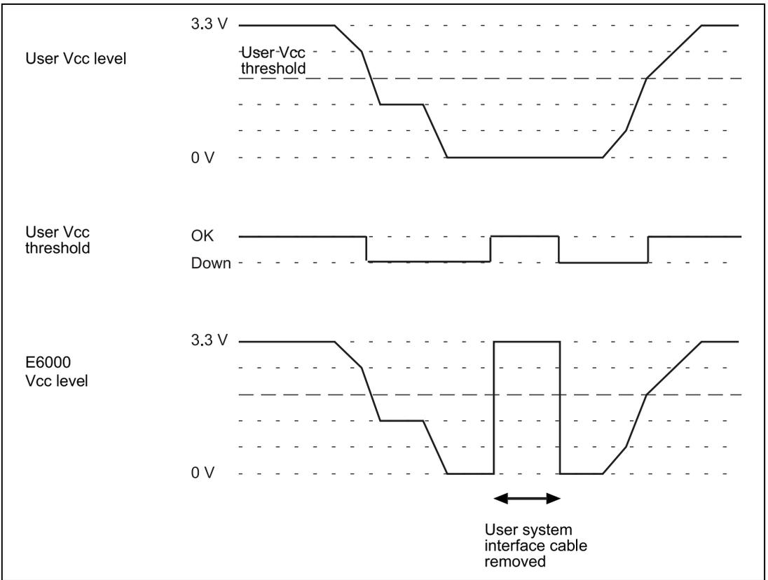
**Figure 3.14 Voltage Level Monitoring (Example for Vcc = 3.3 V)**
