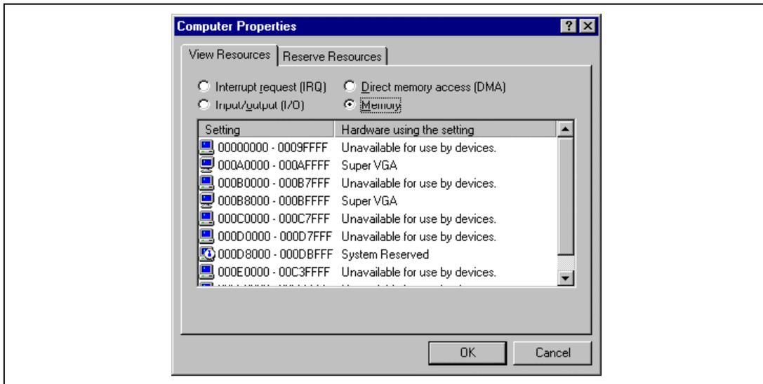
**Figure 2.3 Computer Properties Dialog Box (After Setting)**
