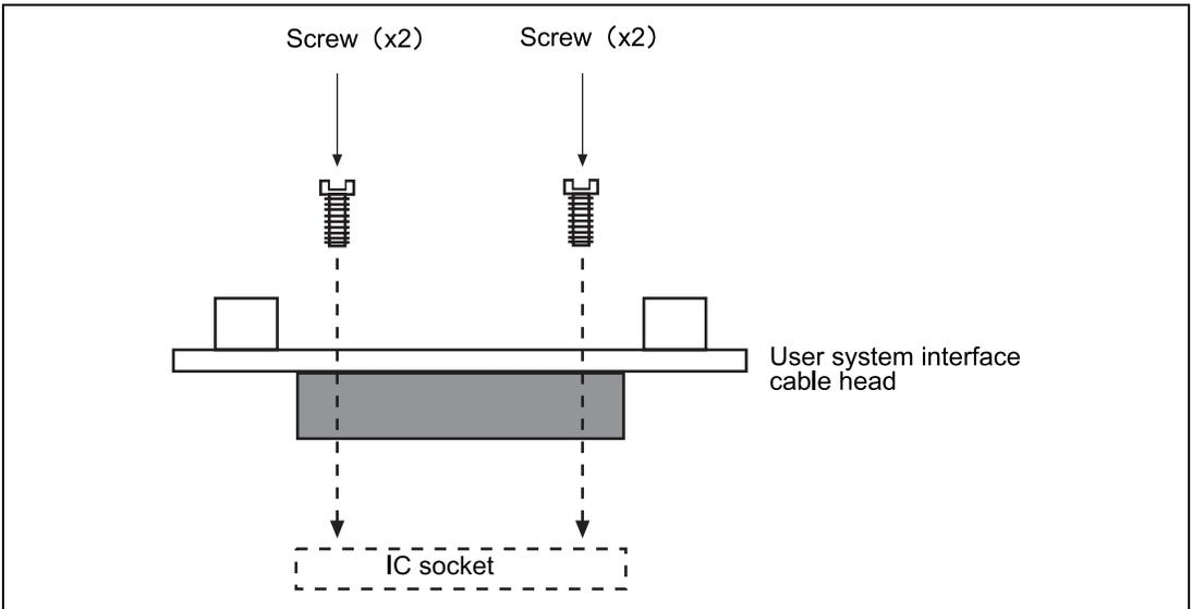
**Figure 3.2 Example of Connecting User System Interface Cable Head to User System**
