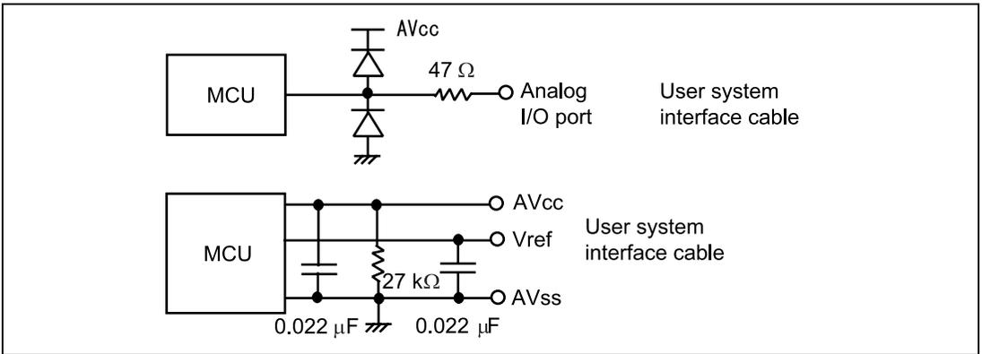
**Figure 3.9** User System Interface Circuit for Analog Port Control Signals
