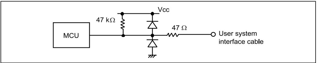
**Figure 3.6 User System Interface Circuit for General Ports**
