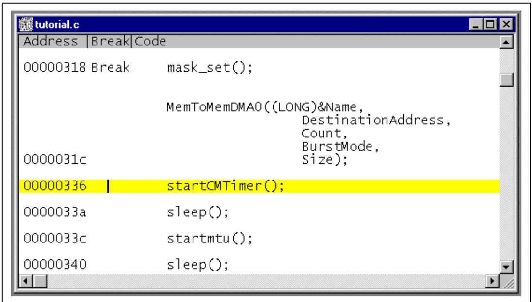
Figure 4.24 Program Window after Executing the Step Over Command
