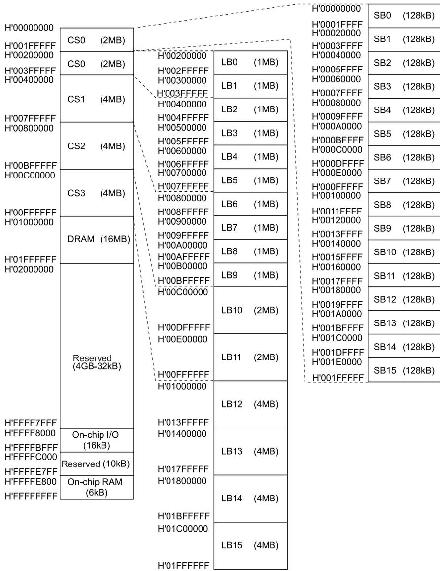
Figure 4.5 Memory Block in Extended Mode without ROM
