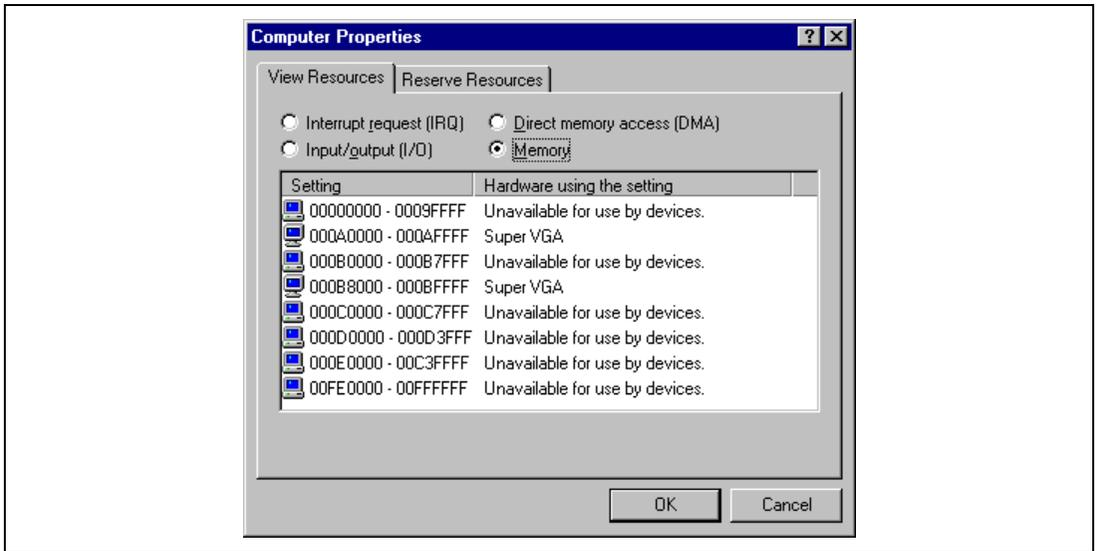
Figure 2.1 Computer Properties Dialog Box (Before Setting)
