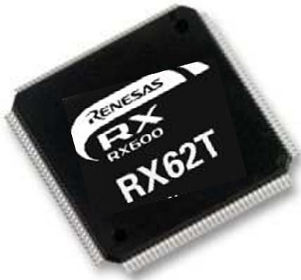
100MHz, MAC, FPU enable complex algo. & full support of Matlab/Scilab equations
