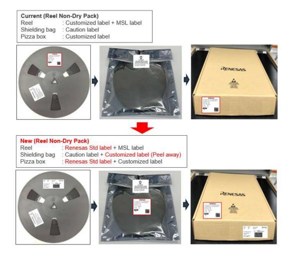
Note: Customized label can be peeled off from Shielding bag and pasted on the Reel
