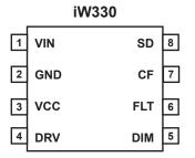
Figure 4.1 : 8-Lead SOIC Package
