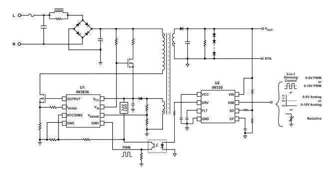
Figure 3.1 : iW330 Typical Application Circuit
