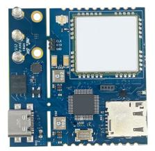
monoZ is a strategic partner for 1NCE, a global MVNO offering managed connectivity services for low-bandwidth IoT applications. monoZ:Jet is a 1NCE compatible compact low-power solderable System-on-Module (SOM) that enables secure IoT connectivity to user system. monoZ:Jet acts as data pump that push the incoming data from host system to the monoZ:Link IoT cloud platform. It is a ready to use device with preloaded application firmware and can be integrated in different user systems.
