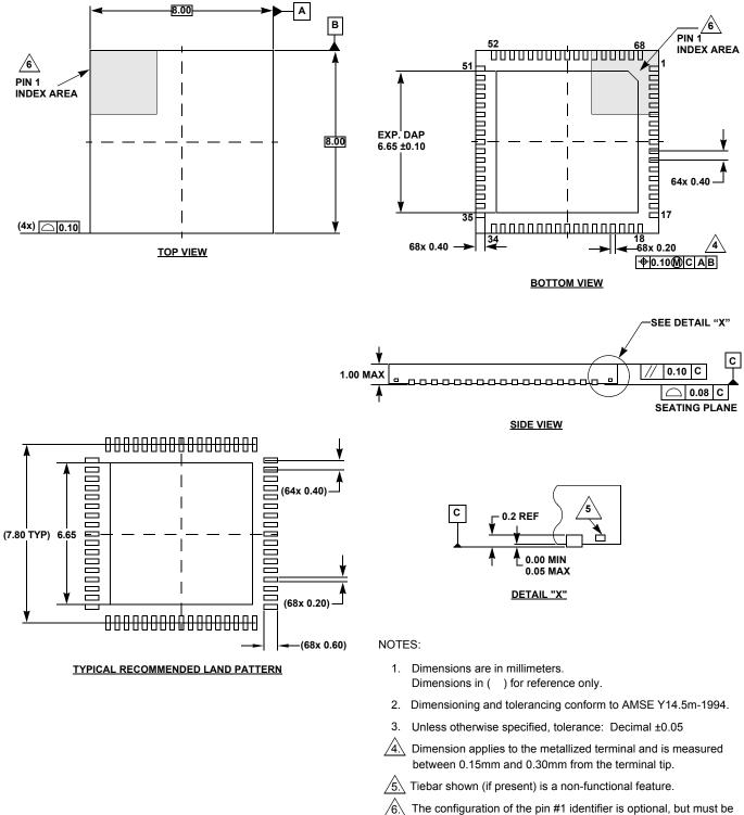
The configuration of the pin #1 identifier is optional, but must be located within the zone indicated. The pin #1 identifier may be either a mold or mark feature.
