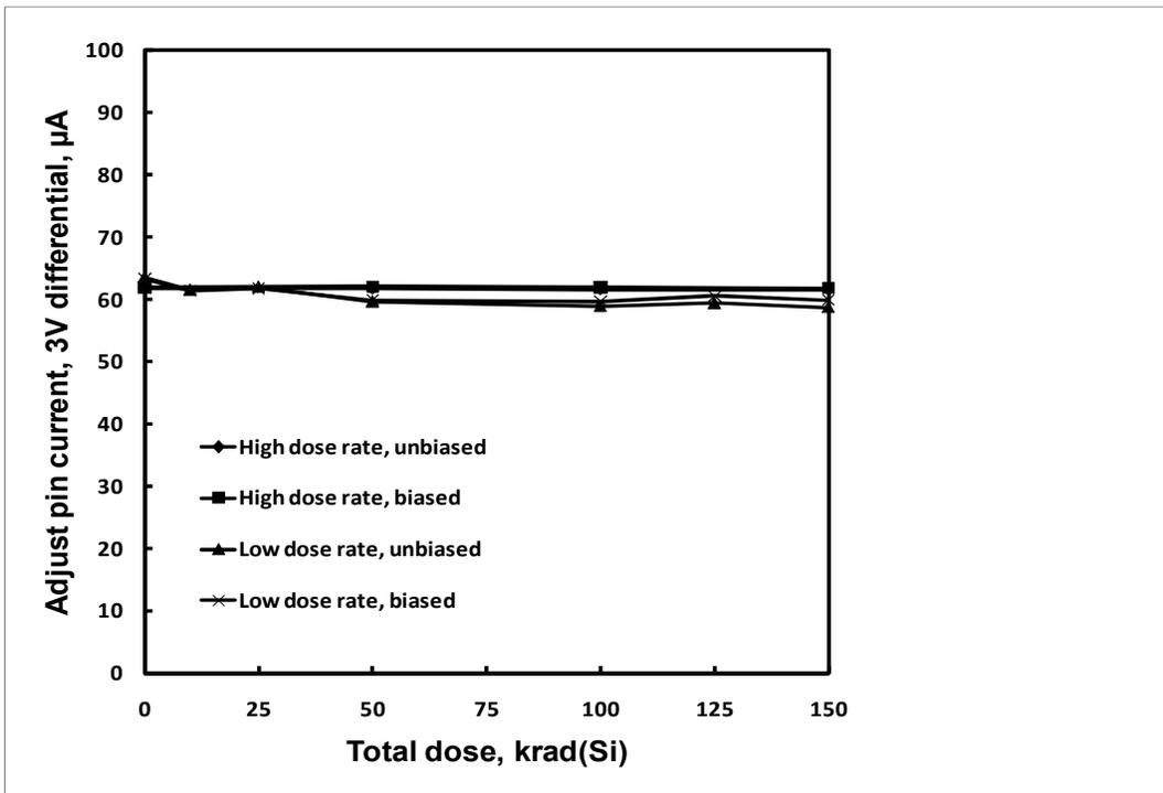
**Figure 6:** HS-117RH adjust pin current at 3V differential as a function of total dose irradiation at low and high dose rate for the unbiased and biased cases. The post-irradiation SMD limit is 100µA.
