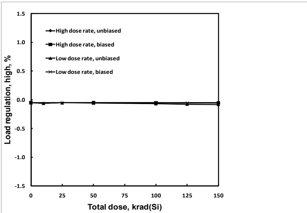
**Figure 10:** HS-117RH load regulation, 5mA to 1.25A, as a function of total dose irradiation at low and high dose rate for the unbiased and biased cases. The post-irradiation SMD limits are -1.5% to 1.5%.
