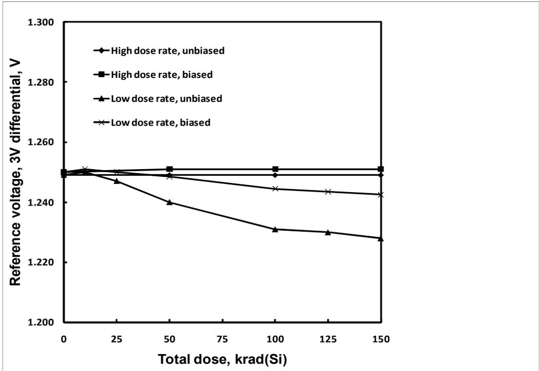
**Figure 3:** HS-117RH reference voltage at 3V differential voltage as a function of total dose irradiation at low and high dose rate for the unbiased (all pins grounded) and the biased (per Figure 2) cases. The low dose rate was 0.01rad(Si)/s and the high dose rate 55rad(Si)/s. Sample size for each cell was 5. The post-irradiation SMD limits are 1.2V to 1.3V.
