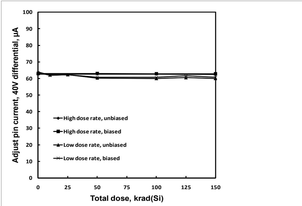
**Figure 7:** HS-117RH adjust pin current at 40V differential as a function of total dose irradiation at low and high dose rate for the unbiased and biased cases. The post-irradiation SMD limit is 100µA.
