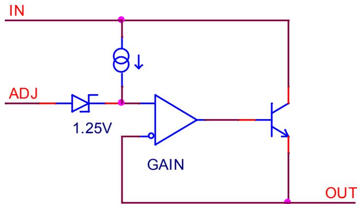
Figure 1: HS-117RH block diagram.
