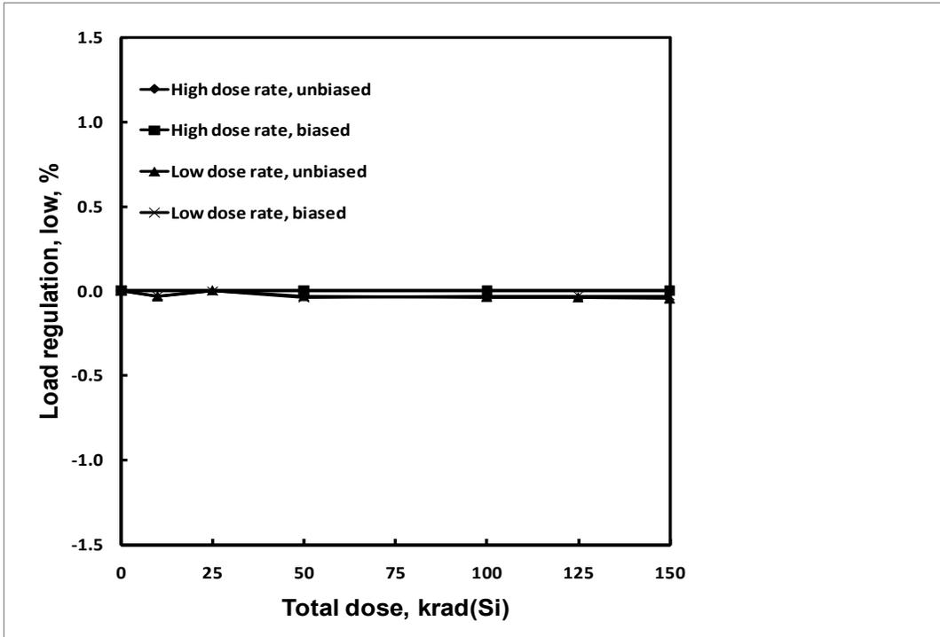
**Figure 9:** HS-117RH load regulation, 5mA to 500mA, as a function of total dose irradiation at low and high dose rate for the unbiased and biased cases. The post-irradiation SMD limits are -1.5% to 1.5%.
