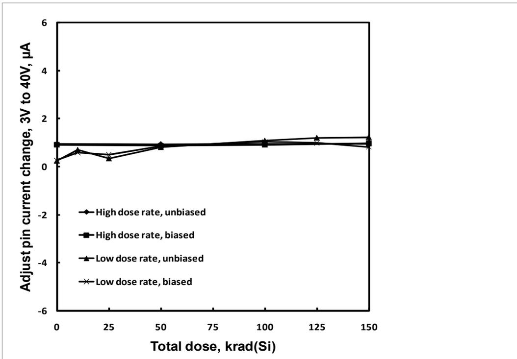
**Figure 8:** HS-117RH adjust pin current change, 3V to 40V differential, as a function of total dose irradiation at low and high dose rate for the unbiased and biased cases. The post-irradiation SMD limit is -6µA to 6µA.
