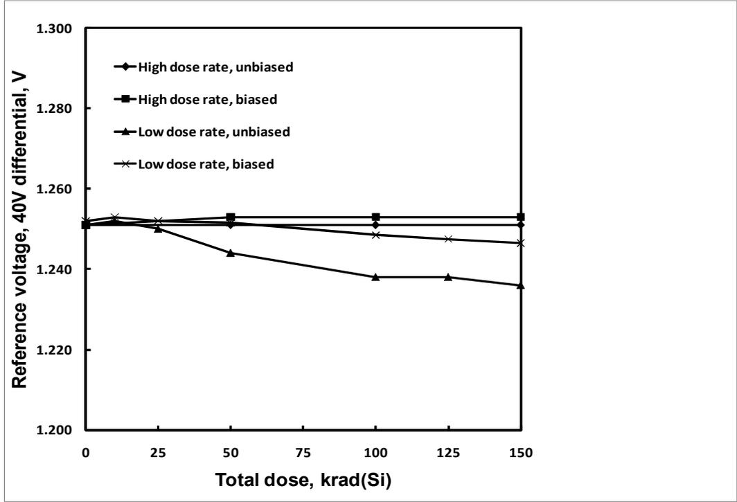
**Figure 4:** HS-117RH reference voltage at 40V differential voltage as a function of total dose irradiation at low and high dose rate for the unbiased (all pins grounded) and the biased (per Figure 2) cases. The low dose rate was 0.01rad(Si)/s and the high dose rate was 55rad(Si)/s. Sample size for each cell was 5. The post-irradiation SMD limits are 1.2 to 1.3V.
